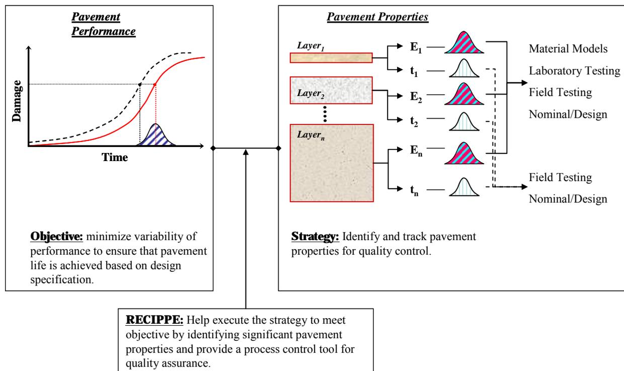
**Figure C.1 - Process of using RECIPPE to Ensure Uniform Pavement by Monitoring Pavement Layer Information**
