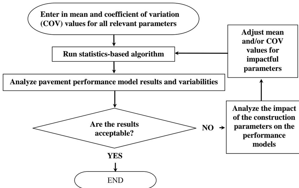
Figure A.3 - General Flow of Optimization Process
