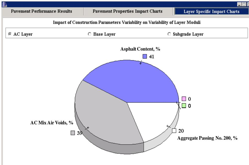
Figure 2.3 – Impact Charts for Design and Construction Parameters.
