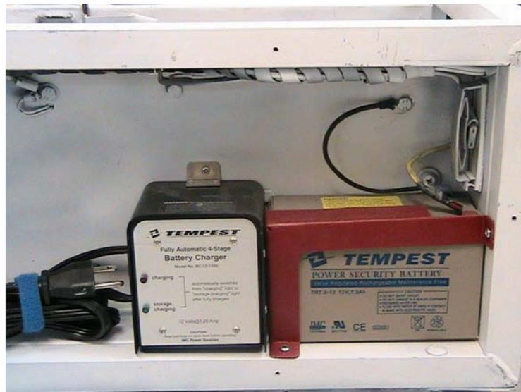
Figure 2.3 – SLA battery and automatic charger.
