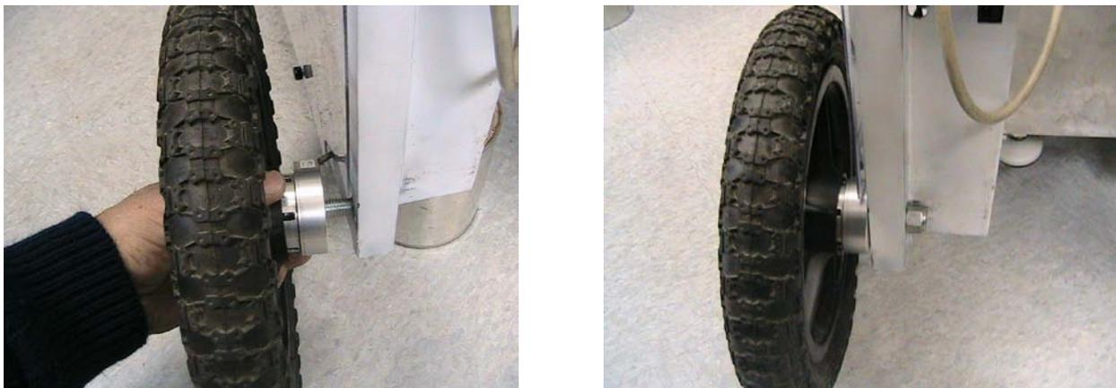
Figure 3.6 –Inserting the DMI in the wheel hub and DMI after installation
