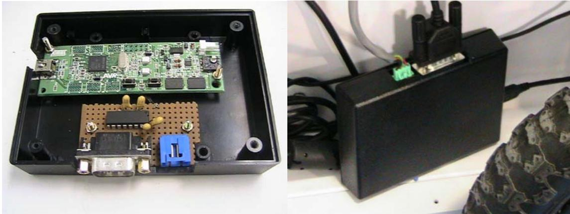
Figure 2.8 – Microcontroller and interconnect boards
