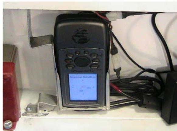
Figure 2.5 – GPS Holder outside and inside enclosure
