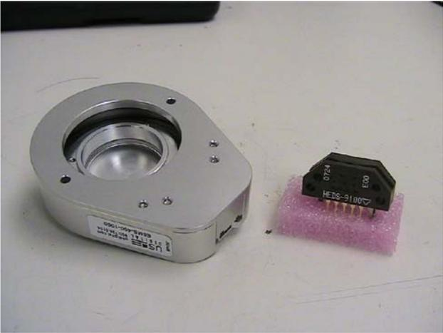
Figure 2.6 – Encoder wheel holder and encoder IC element
