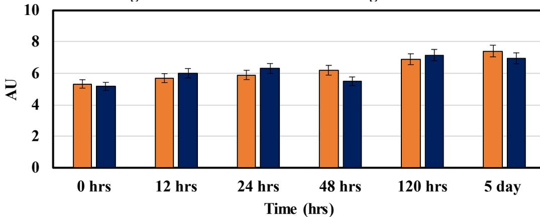
Figure 7.21. C=O Index results for change in PG Grade
