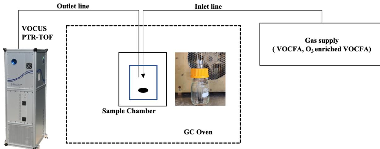
**Figure 7.34. Experimental setup for characterization of binders using Vocus PTR-TOF**
