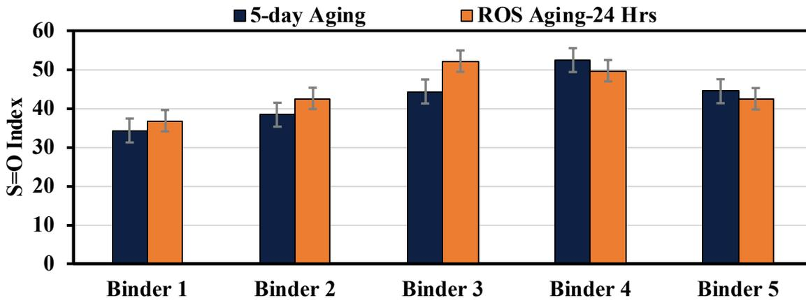
Figure 5.45. Sulfoxide Index of AC Binders Using Protocol 4
