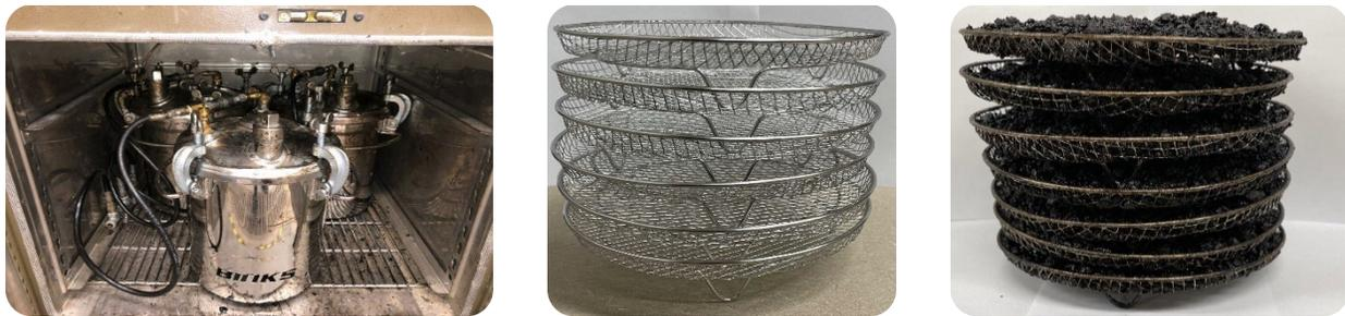
Figure 7.28. Pressure Device and Aging Racks
