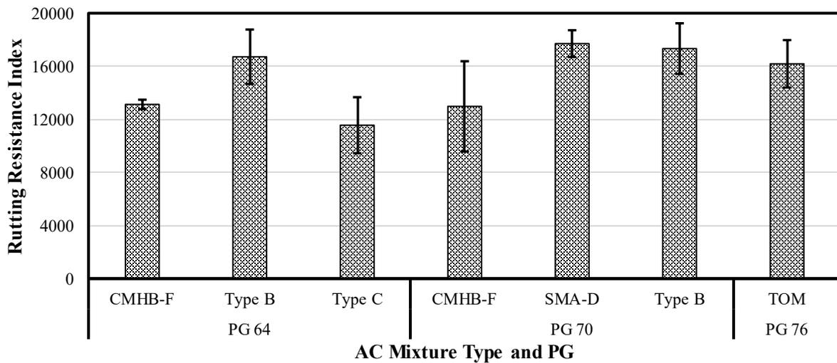
**Figure 3.5. Hamburg Wheel-Tracking Test Comparison of AC Mixtures**
