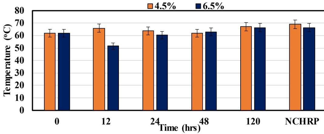
Figure 7.25. High PG Results for Change in Additive (64-22)
