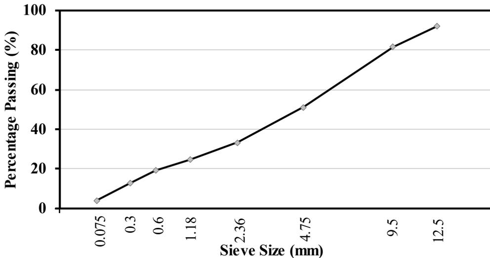
**Figure 5.42. Grading Curve of Mixtures Using Protocol 4**
