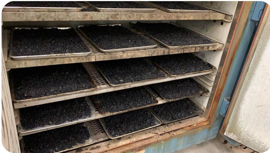
**Figure 6.2. Loose Mixture Aging in Oven (Protocol 1)**
