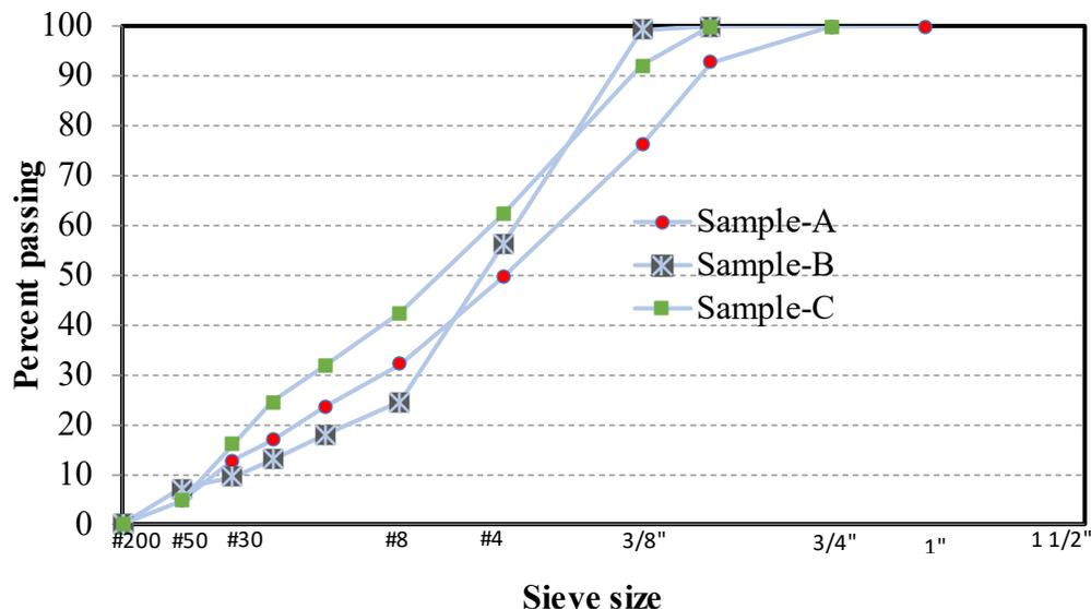
**Figure 7.33. Grading Curve of Mixtures used in the Study**
