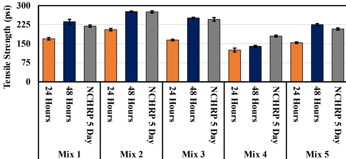
Figure 5.41. IDT Strength Comparison Using Protocol 3
