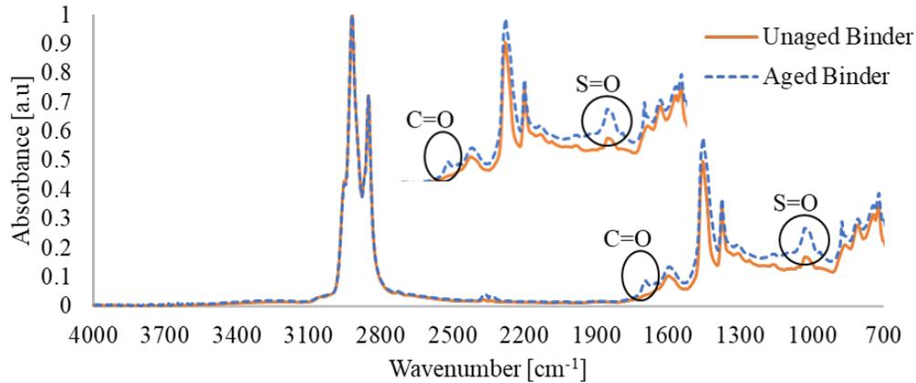
**Figure 5.17. Sample FTIR Spectra of an Aged and Unaged Binder**
