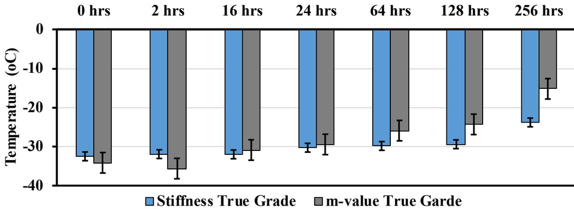
Figure 5.16. Low-Temperature PG for Mix 2 Using Protocol 1
