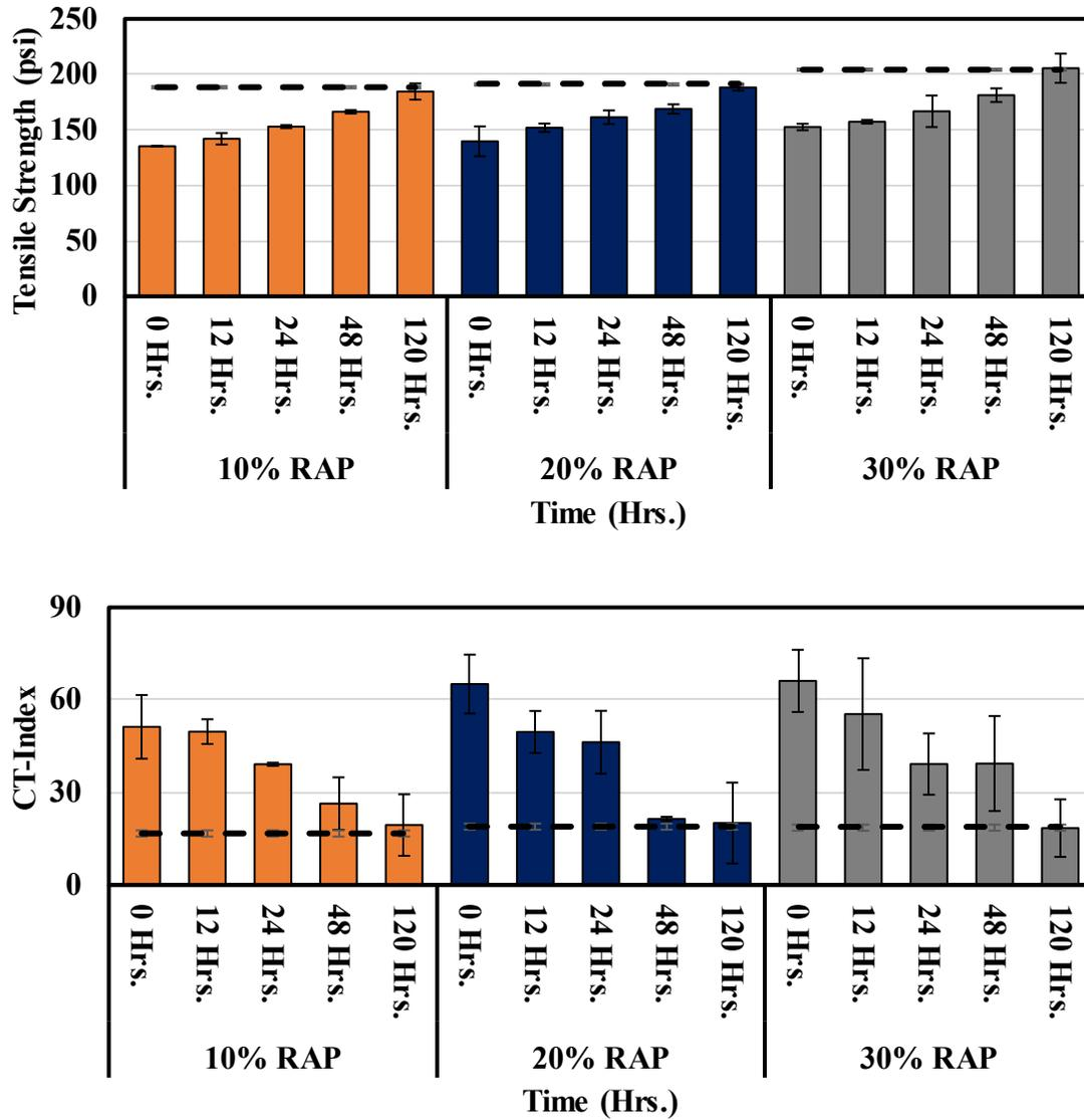
Figure 7.7. Tensile Strength and CT-Index Results for Change in RAP (Mix 1)
