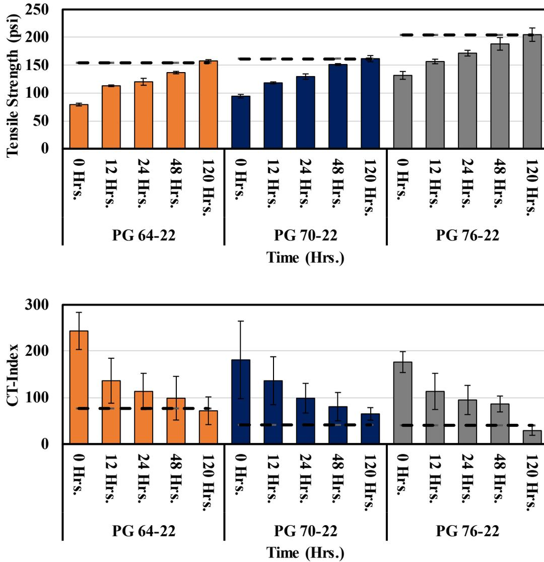
Figure 7.9. Tensile Strength and CT-Index Results for Change in PG (Mix 2)
