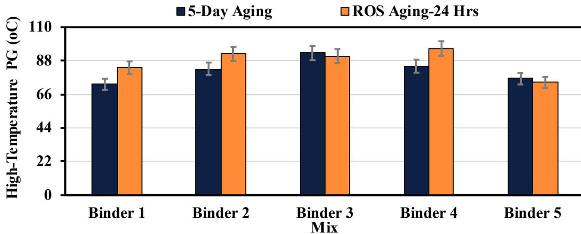
**Figure 5.48. High-Temperature PG of AC Binders Using Protocol 4**
