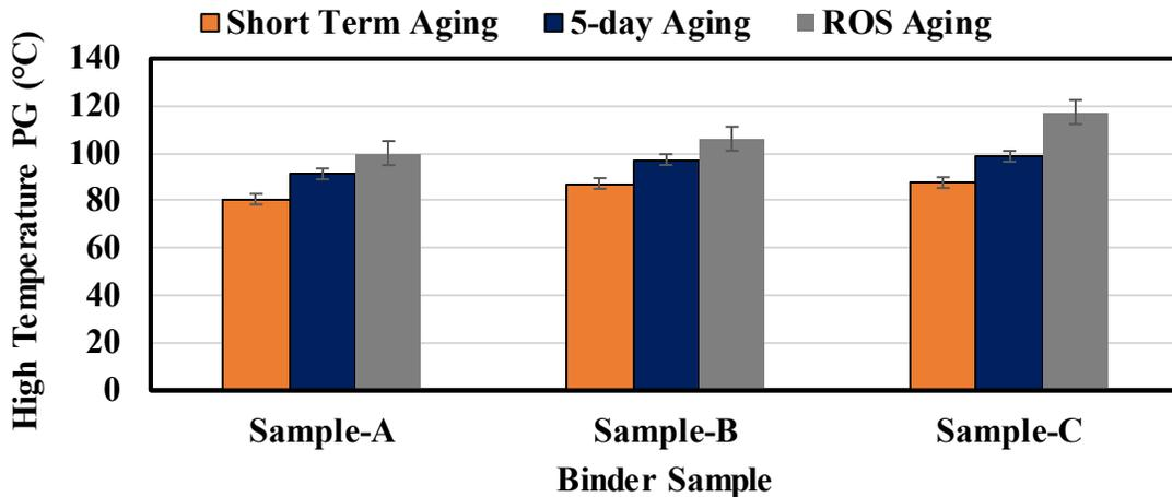
**Figure 7.39. High temperature PG of binders under the three aging protocols**
