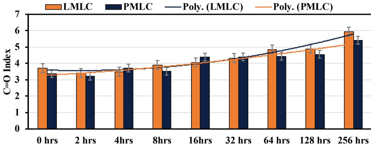
**Figure 5.18. C=O Index for Mix 1 Using Protocol 1**
