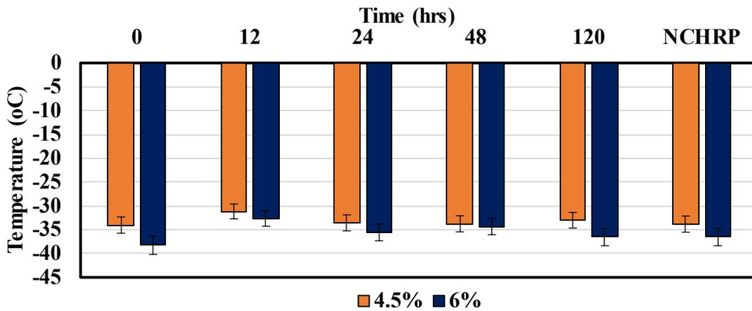
Figure 7.26. Low PG Results for Change in Additive (64-22)
