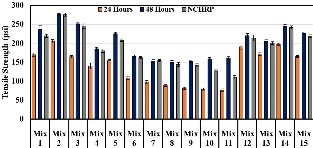
Figure 7.32. IDT Strength Comparison Using Protocol 3
