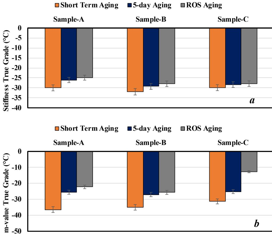
**Figure 7.40. Low temperature PG of binders under the three aging protocols (a) Stiffness true grade, (b) m-value true grade**
