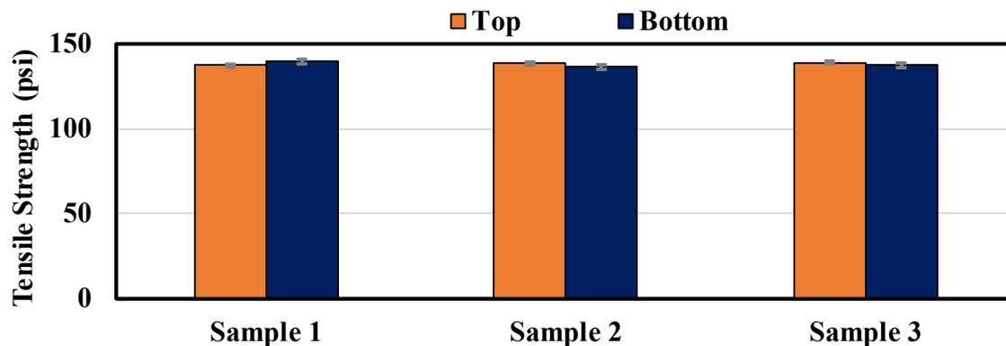
Figure 7.29. Tensile Strength Comparison Using Protocol 2
