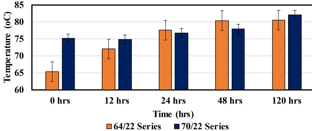
Figure 7.19. High PG results for change in PG grade
