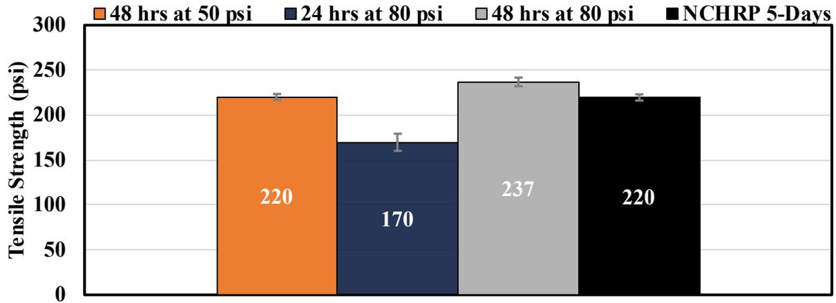
**Figure 5.39. IDT Strength Comparison Using Protocol 3**
