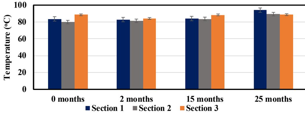
Figure 8.4. High temperature PG of extracted cores
