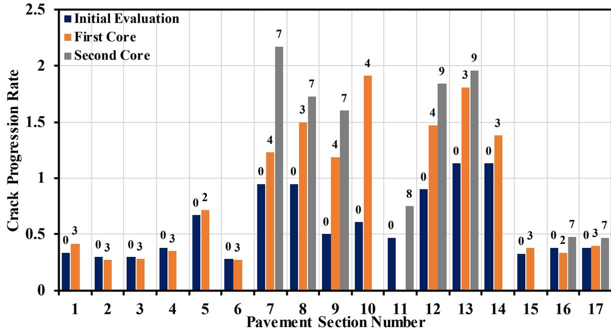
Figure 3.8. Mixture Cracking Performance Evaluation against Time
