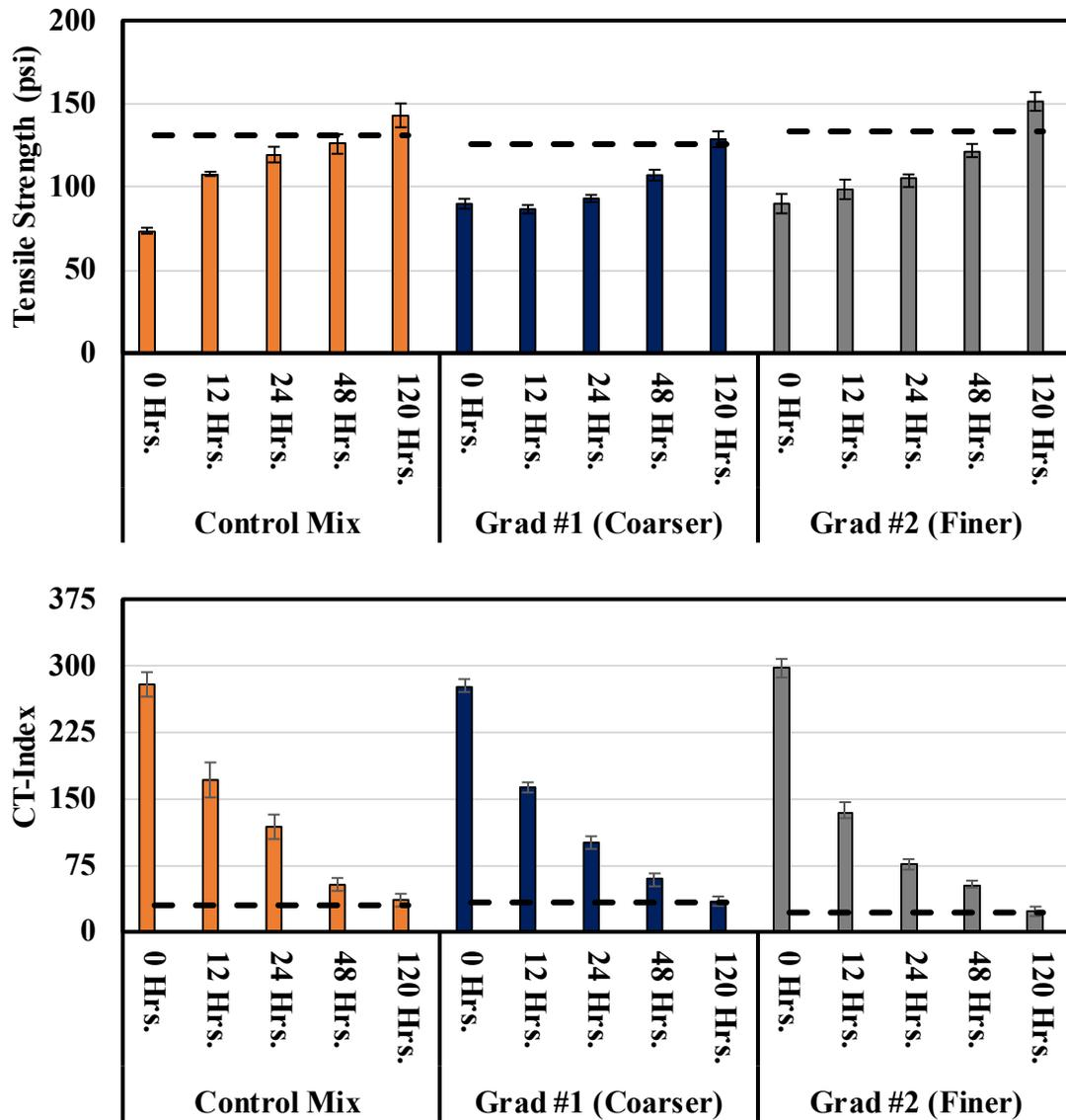
Figure 7.11. Tensile Strength and CT-Index Results for Change in Gradation (Mix 4)
