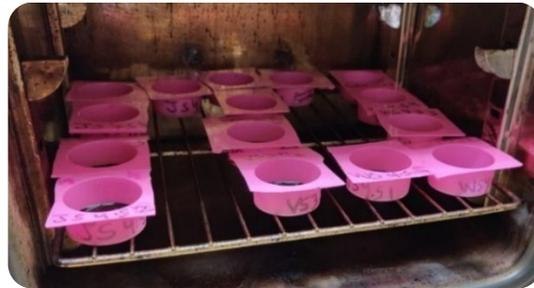
Figure 6.9. Binder Aging in Oven
