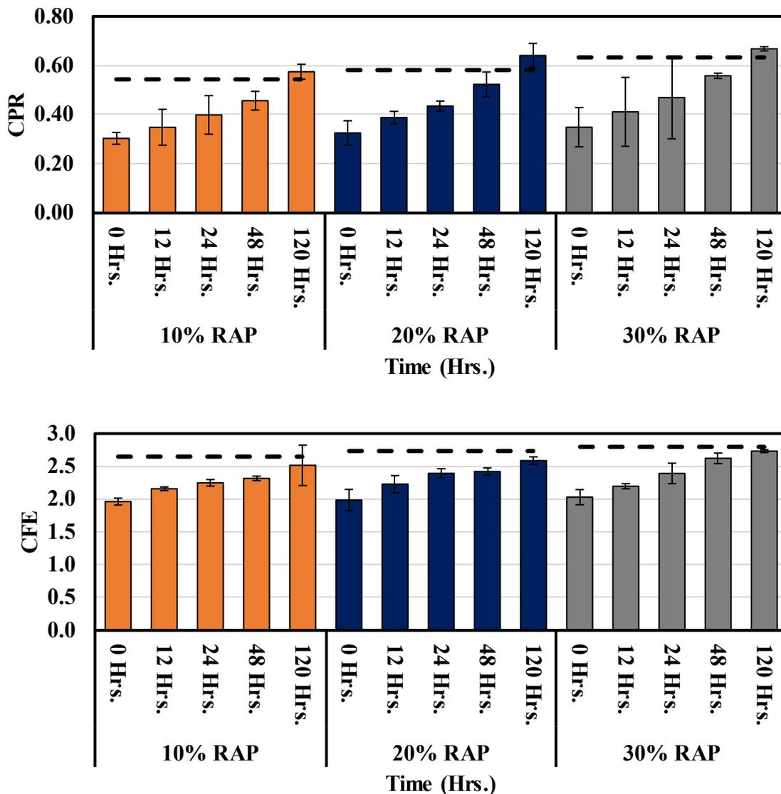
Figure 7.13. CPR and CFE Results for Change in RAP (Mix 1)
