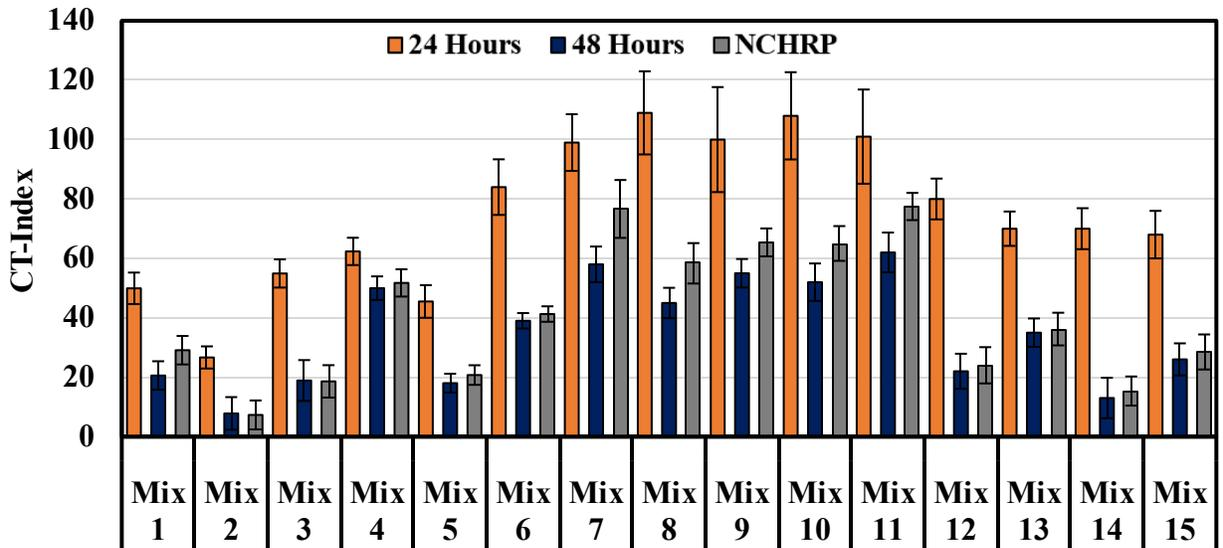
Figure 7.31. IDEAL-CT Index Value Comparison Using Protocol 3
