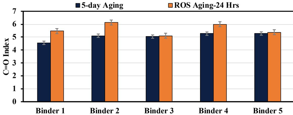
Figure 5.44. Carbonyl Index of AC Binders Using Protocol 4
