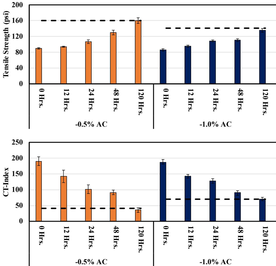
Figure 7.12. Tensile Strength and CT-Index Results for Change in Asphalt Content (Mix 4)
