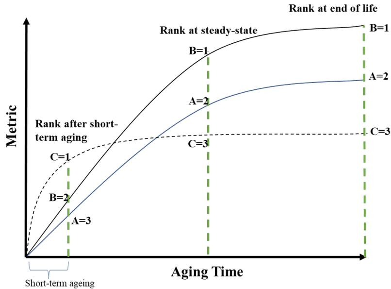
**Figure 6.5. Steady-State Aging of Asphalt Mixtures**
