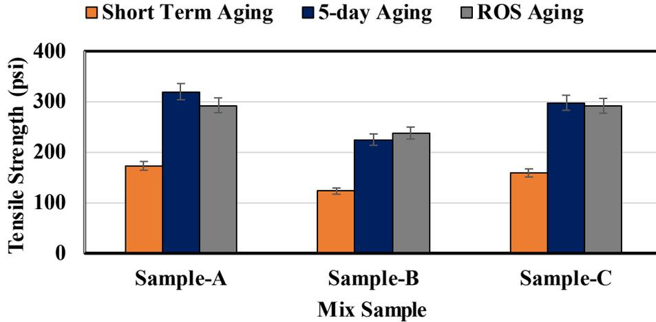
**Figure 7.38. Tensile strength of mixes aged under the three aging protocols**
