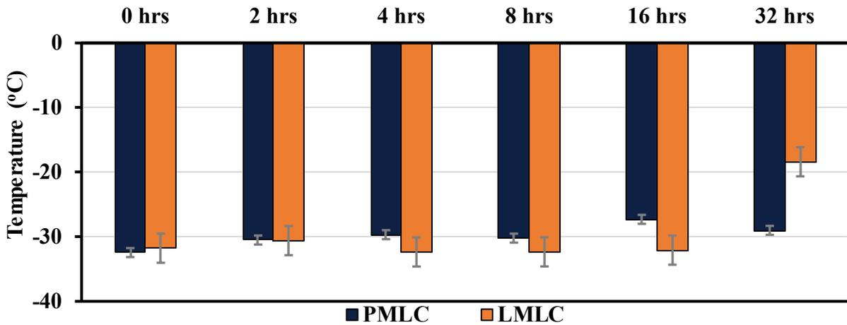
Figure 5.32. Stiffness Based True Low-Temperature PG for Mix 1 Using Protocol 2
