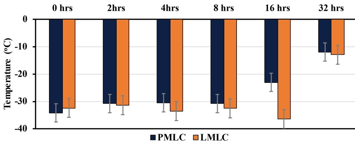
Figure 5.33. m-Value-Based True Low-Temperature Grade for Mix 1 Using Protocol 2
