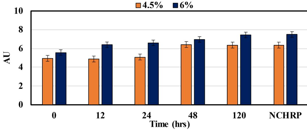
Figure 7.24. C=O Index Results for Change in Additive (70-22)
