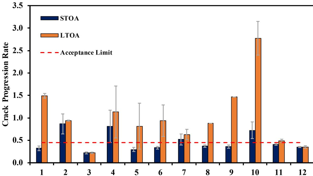
**Figure 3.9. Crack Progression Rate Results for Aged Mixtures**
