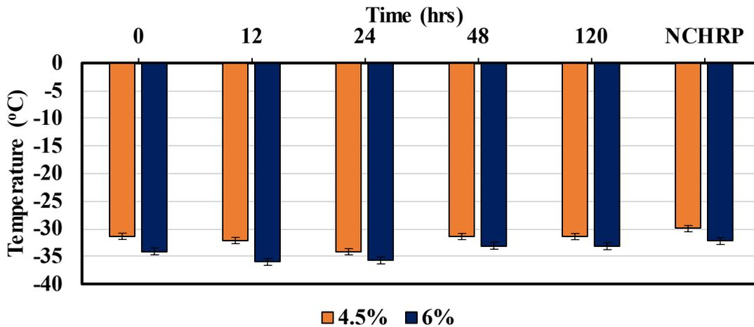
Figure 7.23. Low PG Results for Change in Additive (70-22)
