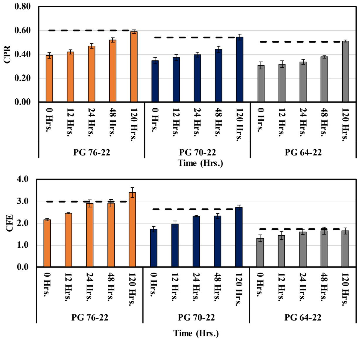
Figure 7.15. CPR and CFE Results for Change in PG (Mix 2)
