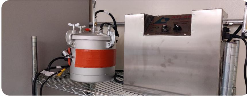
**Figure 6.4. Ozone Aging Device Setup (Protocol 3)**
