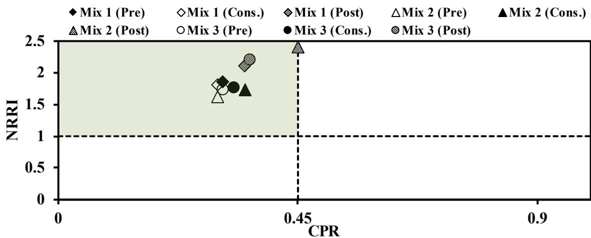
Figure 8.1. Interaction Performance Plot with a BMD Mix
