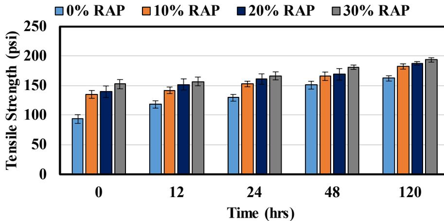
**Figure 6.6. Rank Order Comparison for IDT Tensile Strength**
