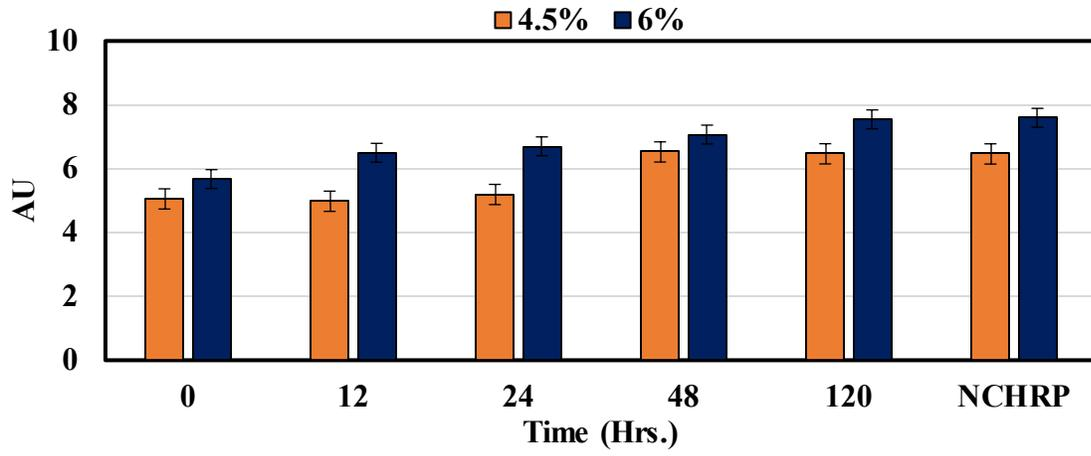
Figure 7.27. C=O Index Results for Change in Additive (64-22)
