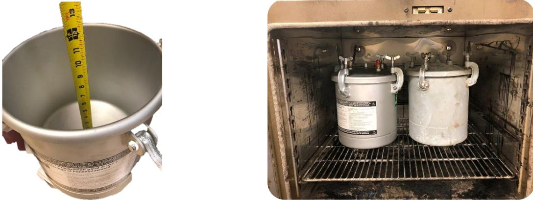
**Figure 4.6. Pressure Aging Chamber for Loose Mix (Protocol 3)**
