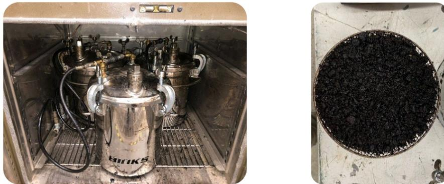
**Figure 6.3. Pressure Aging Device (Protocol 2)**
