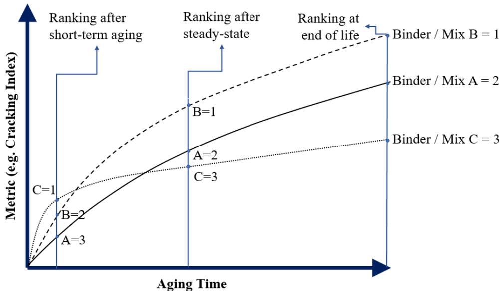
Figure 5.49. Steady-State Aging of Asphalt Mixtures
