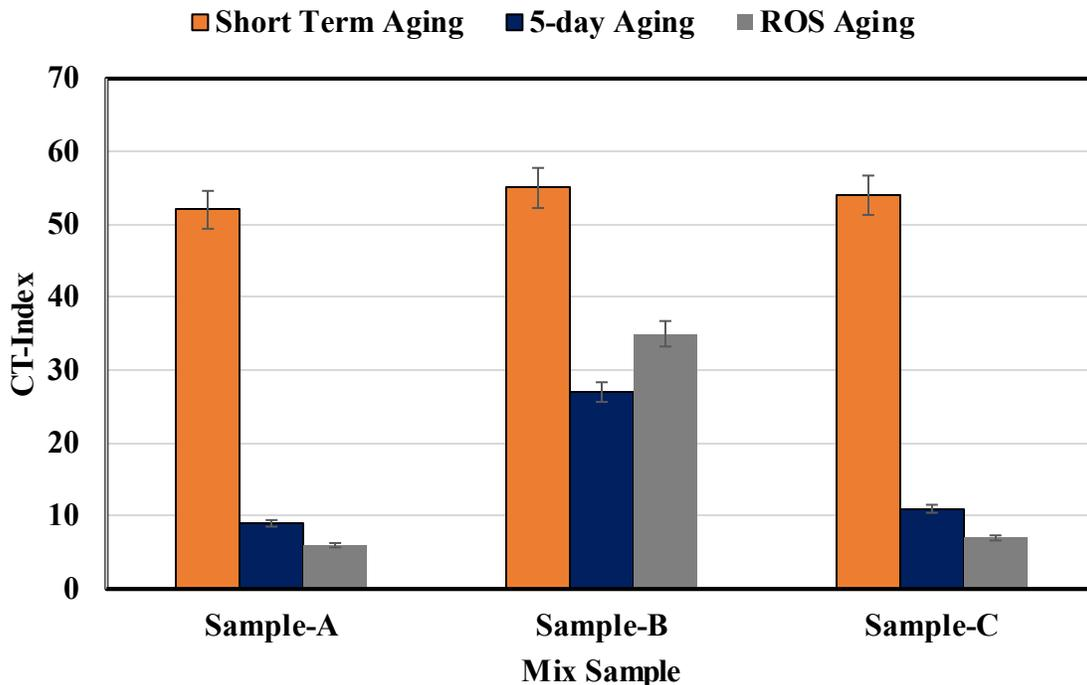
Figure 7.37. CT-index comparison of mixes aged under the three aging protocols
