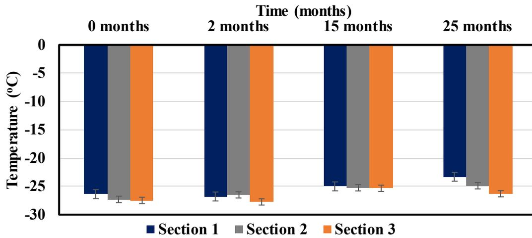
Figure 8.5. Low temperature PG- (Stiffness based) of extracted cores
