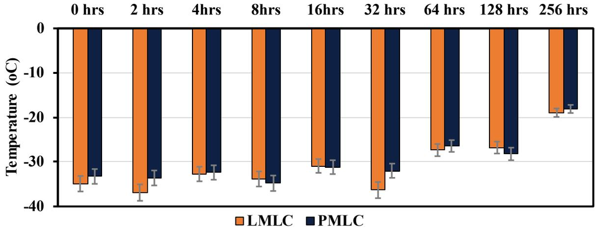
Figure 5.15. m-Value-Based True Low-Temperature Grade for Mix 1 Using Protocol 1
