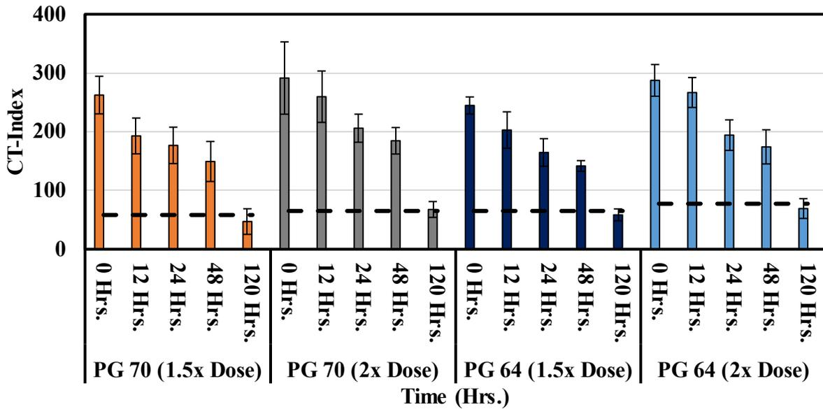
Figure 7.8. Tensile Strength and CT-Index Results for Change in Additives (Mix 2)
