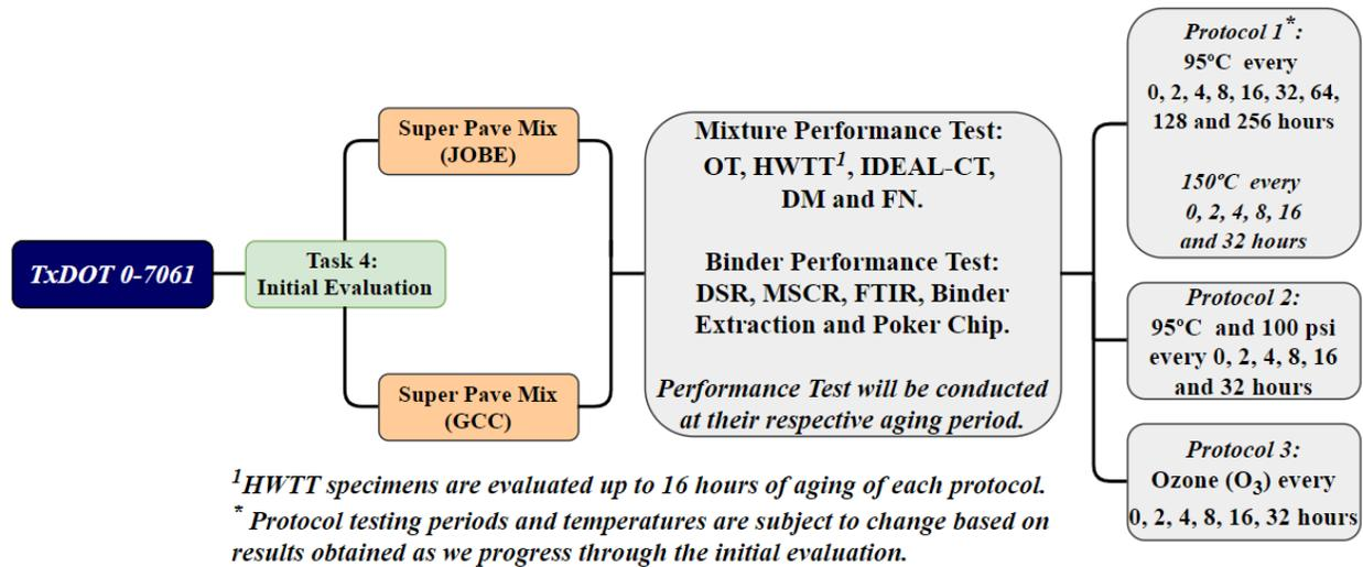
**Figure 4.1. Initial Evaluation Design Plan**
