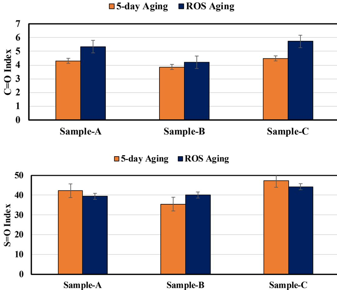
**Figure 7.41. Aging indices of long-term aged binders (a) Carbonyl Index, (b) Sulfoxide Index**
