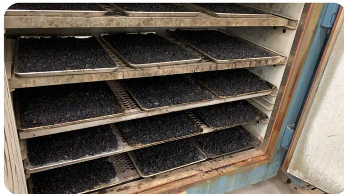
**Figure 4.5. Loose Mixture Aging in Oven (Protocol 1 and Protocol 2)**
