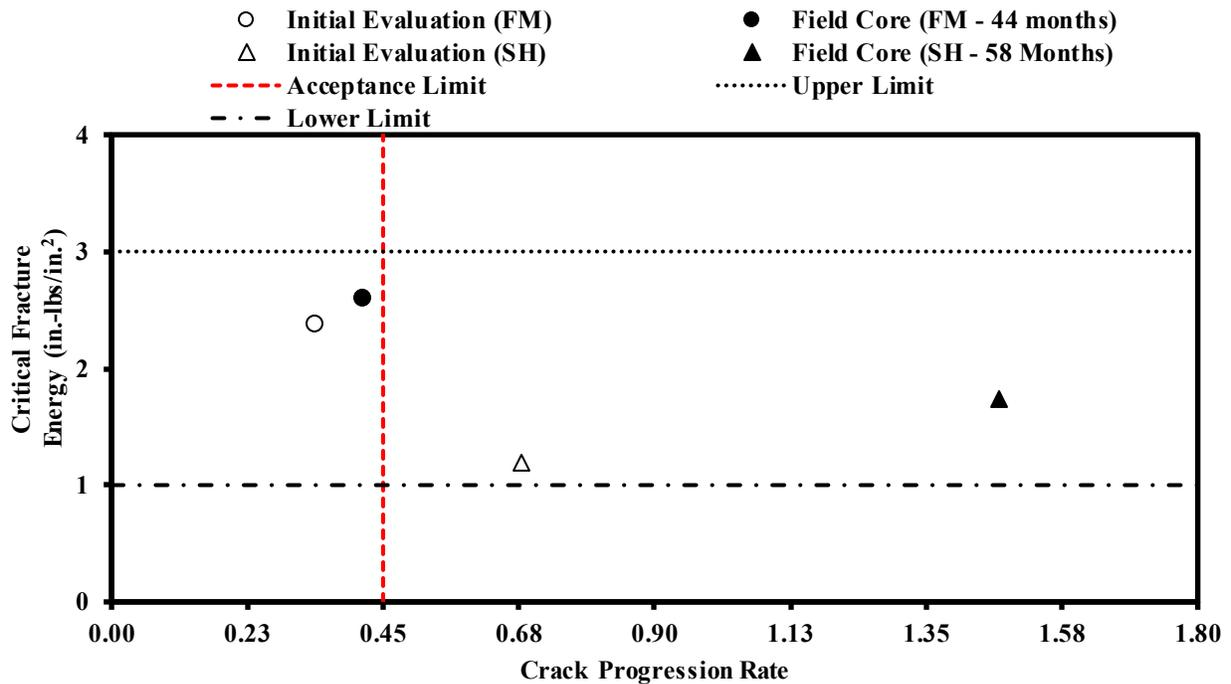
**Figure 3.6. Interaction Diagram Plot for Cracking Performance**
