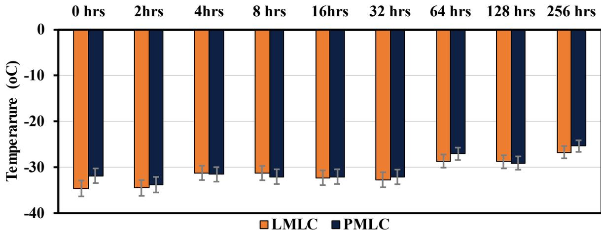
Figure 5.14. Stiffness-Based True Low-Temperature Grade for Mix 1 Using Protocol 1
