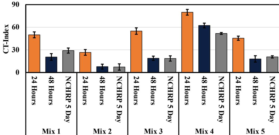
Figure 5.40. IDEAL-CT Index Value Comparison Using Protocol 3
