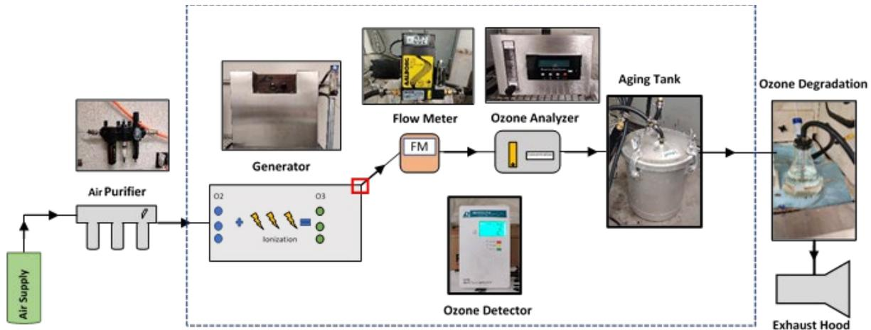
**Figure 5.43. Setup of the Accelerated Aging Procedure**
