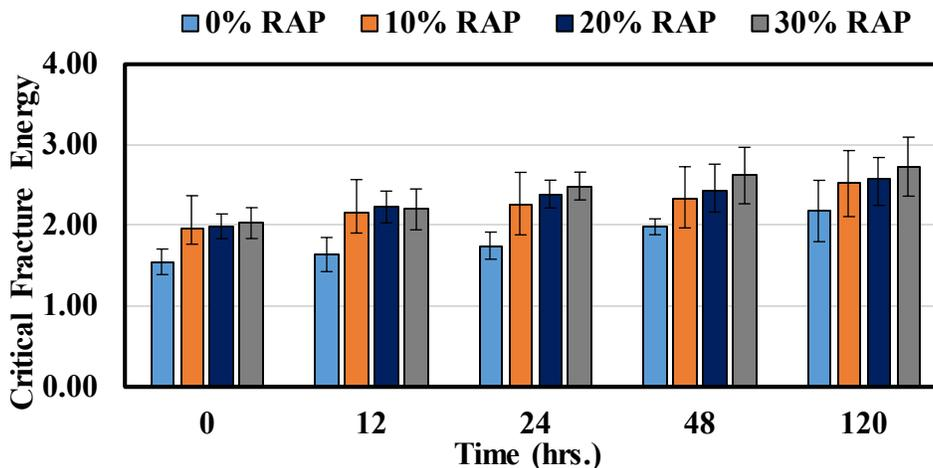
Figure 6.8. Rank Order Comparison for OT Critical Fracture Energy
