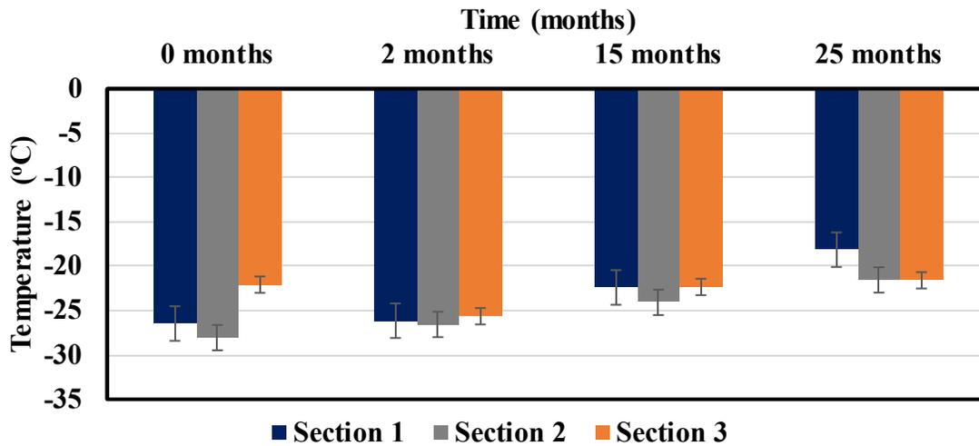
Figure 8.6. Low temperature PG (m-Value based) of extracted cores
