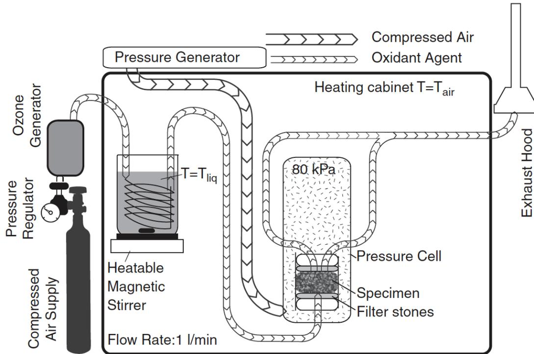
**Figure 2.2. Overview of VAPro Procedure (Steiner et al. 2016)**
