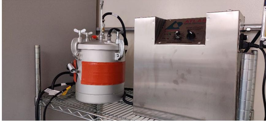
**Figure 4.8. Setup of the Ozone Based Aging Device (*Protocol 4*)**
