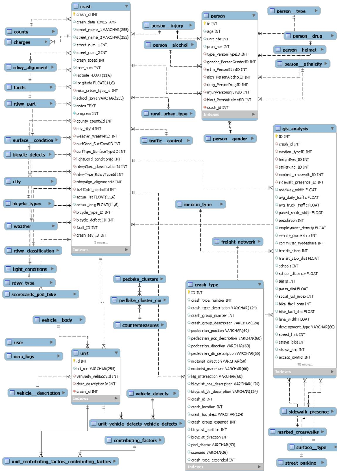
**Figure 6.2 Entity Relations Diagram for the Database.**
