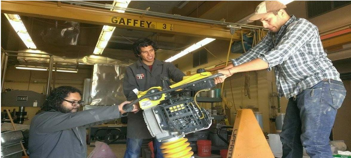
**Figure 4-2 Sample Preparation Using Vibratory Compactor**
