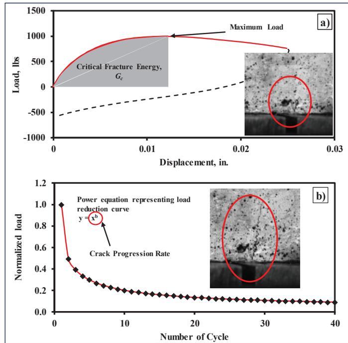
Figure 1 - Test Response Curves: a) Critical Fracture Energy (Crack Initiation) and b) Crack Progression Rate (Crack Propagation)
