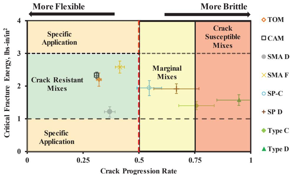
Figure 2 - Design Interaction Plot for Cracking Resistance of AC Mixes
