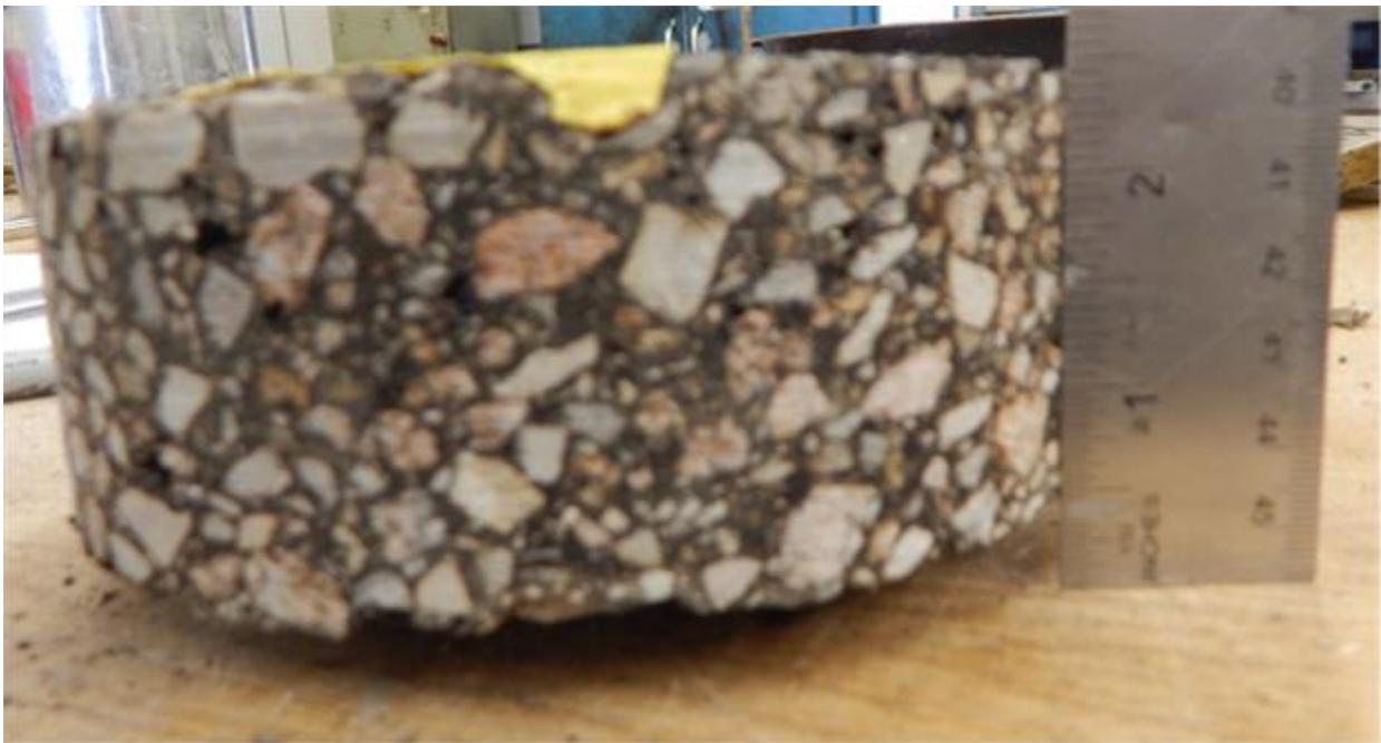
**Figure D10 - Field Core from Section 10**
