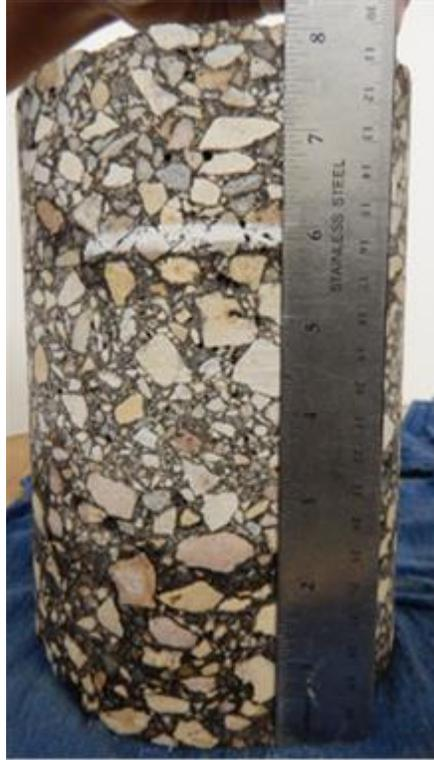
**Figure D5 - Field Core from Section 5**
