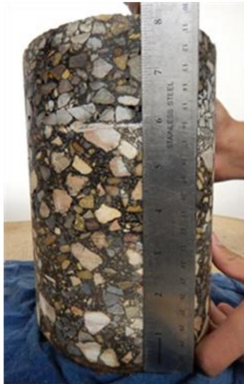
**Figure D2 - Field Core from Section 2**
