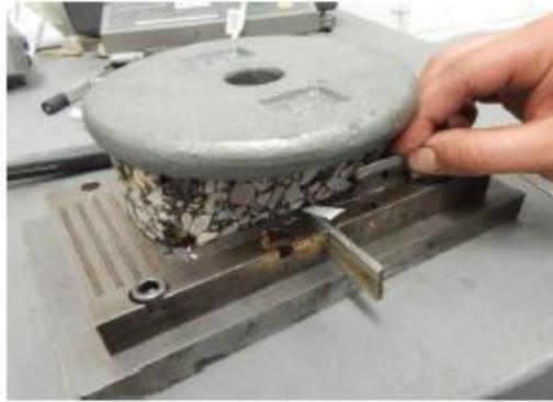
**Figure 12—Excess Epoxy Removed from Sides**
