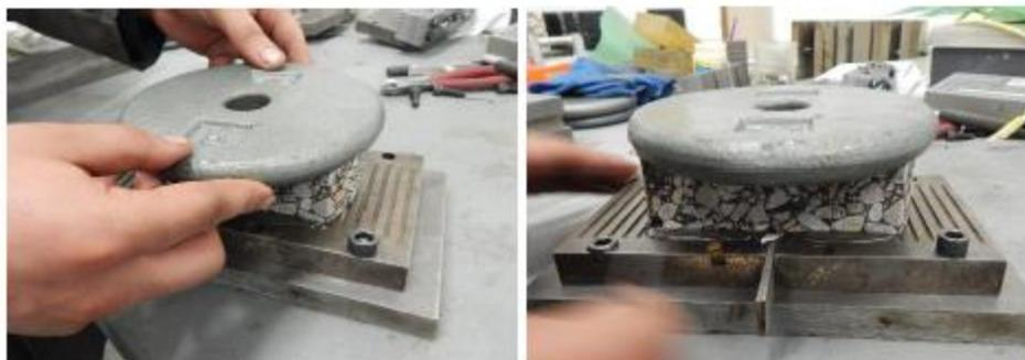
Figure 11—5-lb Weight on Top of Specimen
