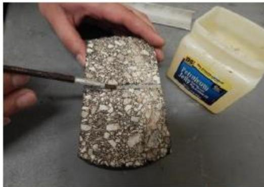
**Figure 7—Grease (Petroleum Jelly) on Specimen and Tape Placed on Center Line**
