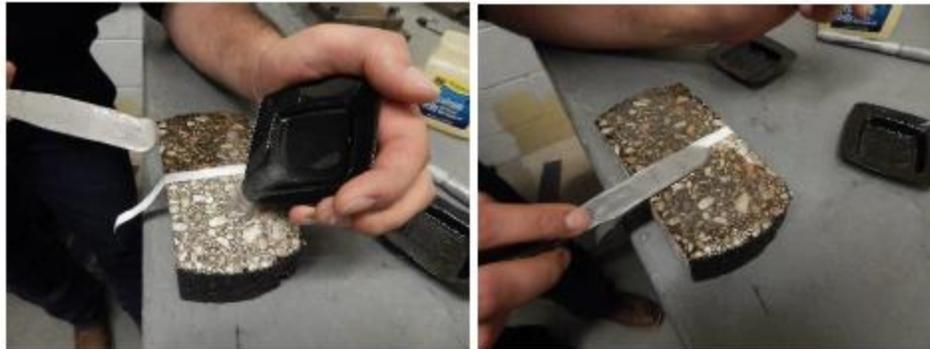
Figure 9—Pouring and Spreading Epoxy
