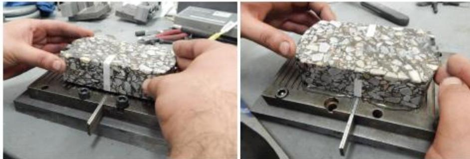
Figure 10—Centering and Alignment the Specimen
