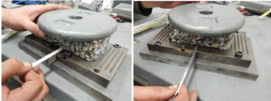
**Figure 13—Tape and Space Bar Removal**
