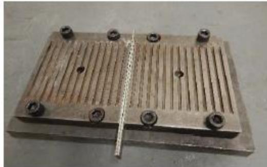
**Figure 5—Base Plates on Mounting Jig with Space Bar**
