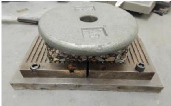
**Figure 14—Mounted Specimen**
