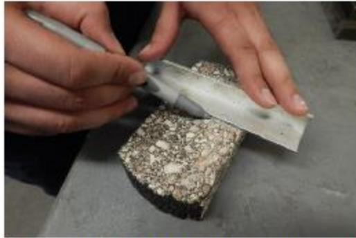
**Figure 6—Middle Line Drawn with Permanent Marker**
