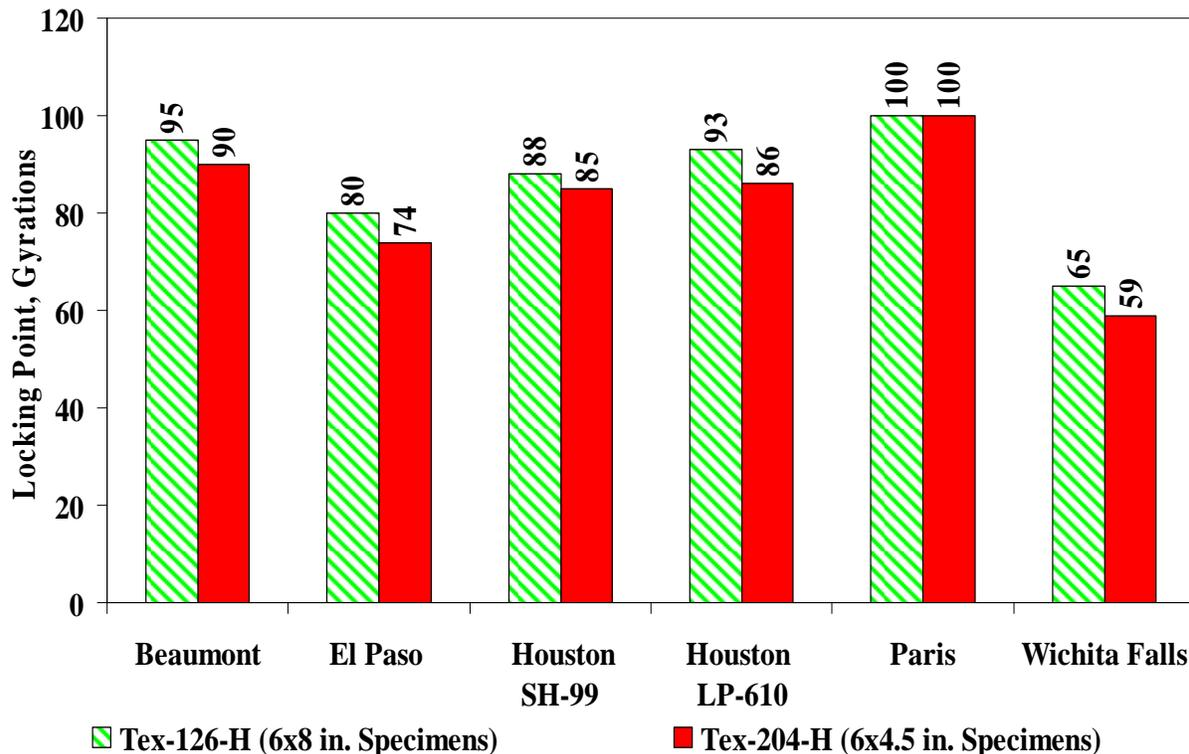
**Figure 5.5 – Locking Points for Tex-126-H and Tex-126-E Specimens**
