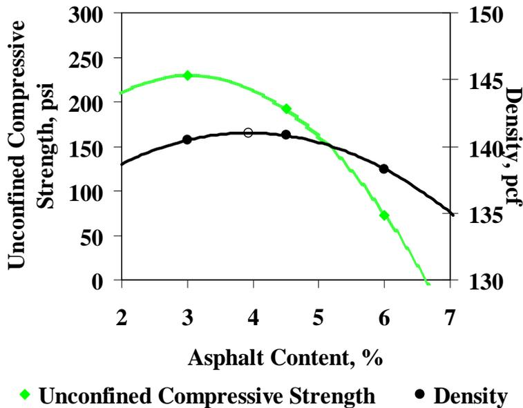
b) Asphalt Content–Density/Strength Curves
