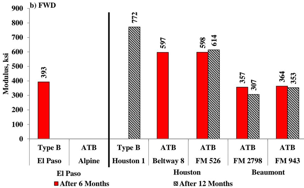
**Figure 7.7 – Comparison of PSPA and FWD Modulus for ATB and Type B Specimens**
