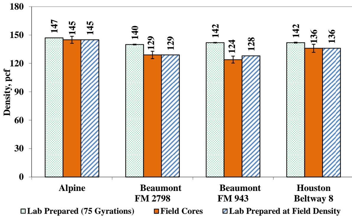
Figure 6.10 - Comparison between Densities of Laboratory Specimens and Field Cores.
