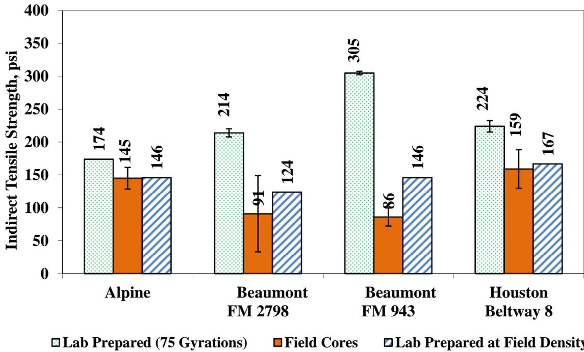
Figure 6.11 - IDT Comparison between Laboratory and Field Specimens.
