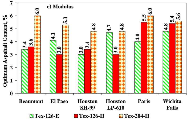
**Figure 4.8 – Comparison of Optimum Asphalt Contents Based on Density, Strength, and Modulus**
