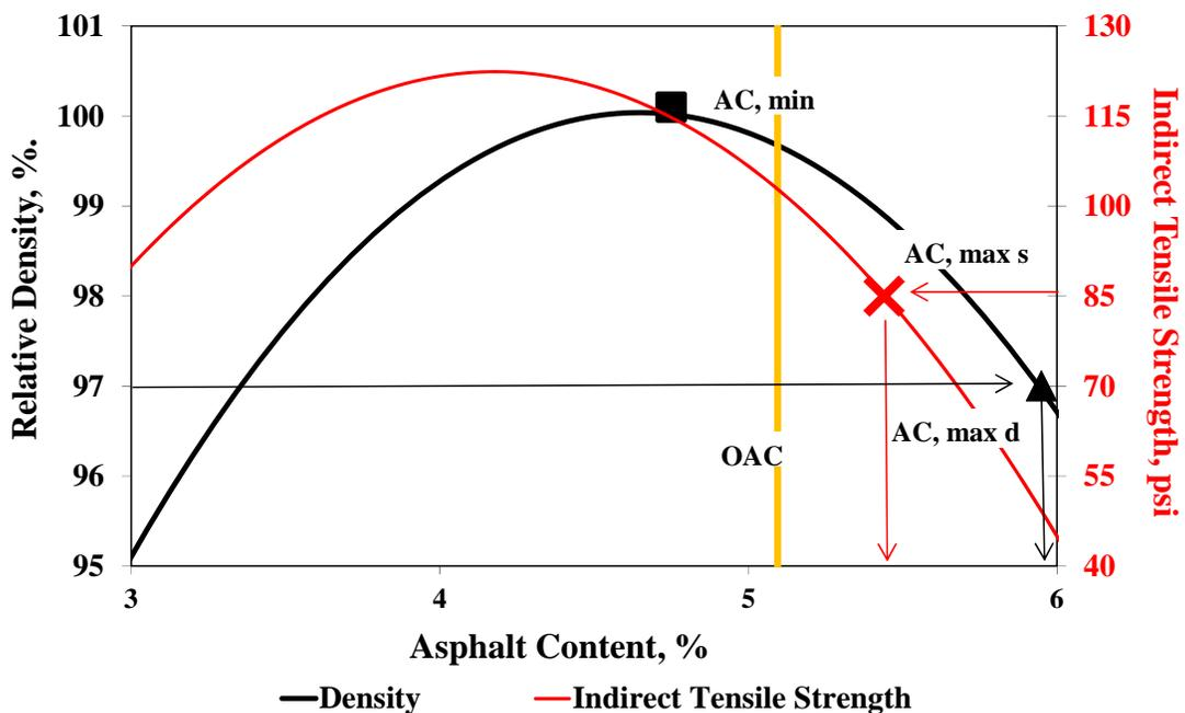
Figure 5.39 – Relative Density/IDT Asphalt Content Combined Curves
