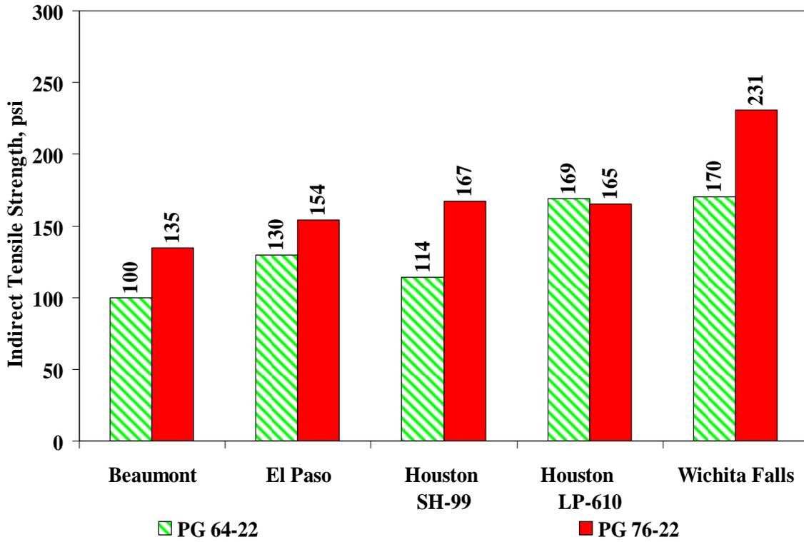
Figure 5.24 – Impact of Binder Grade on IDT Strength for Tex-204-H Protocol
