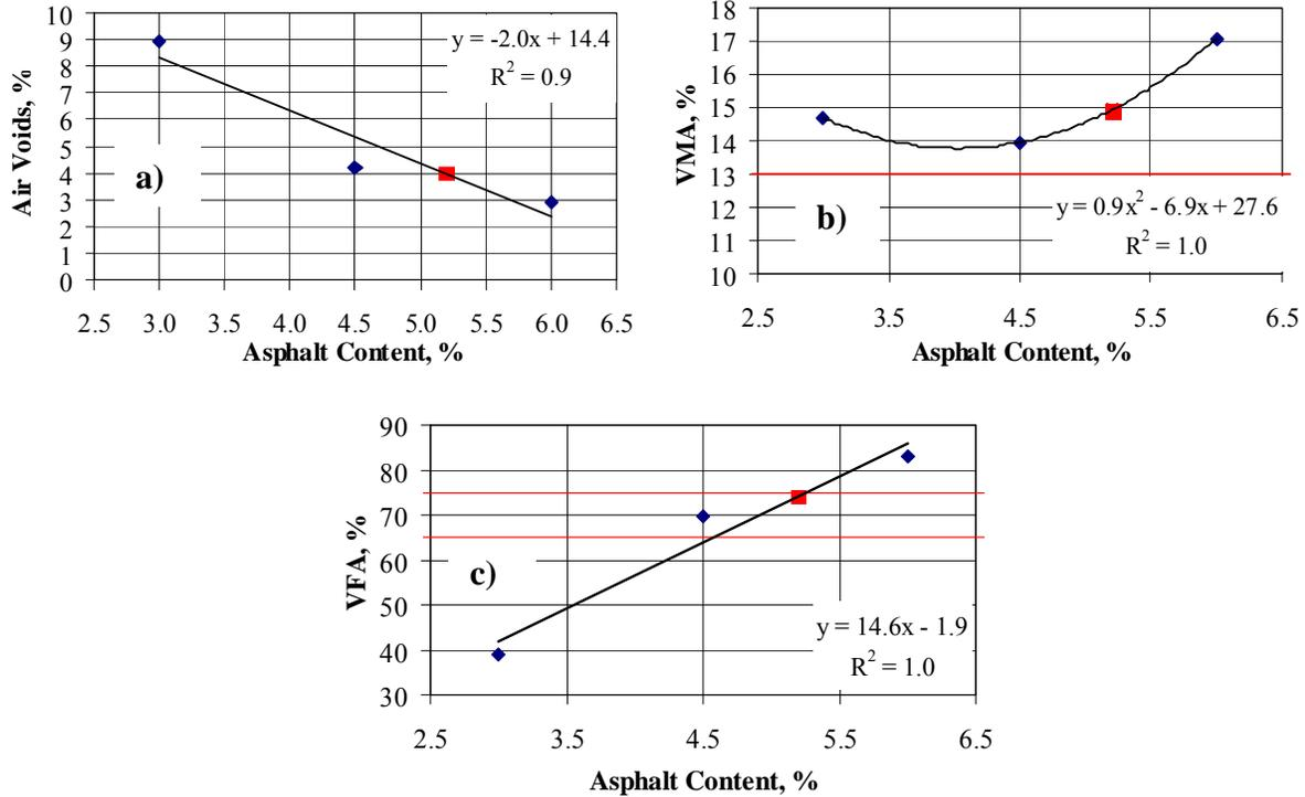
**Figure 4.7 – Volumetric Properties for El Paso Material**
