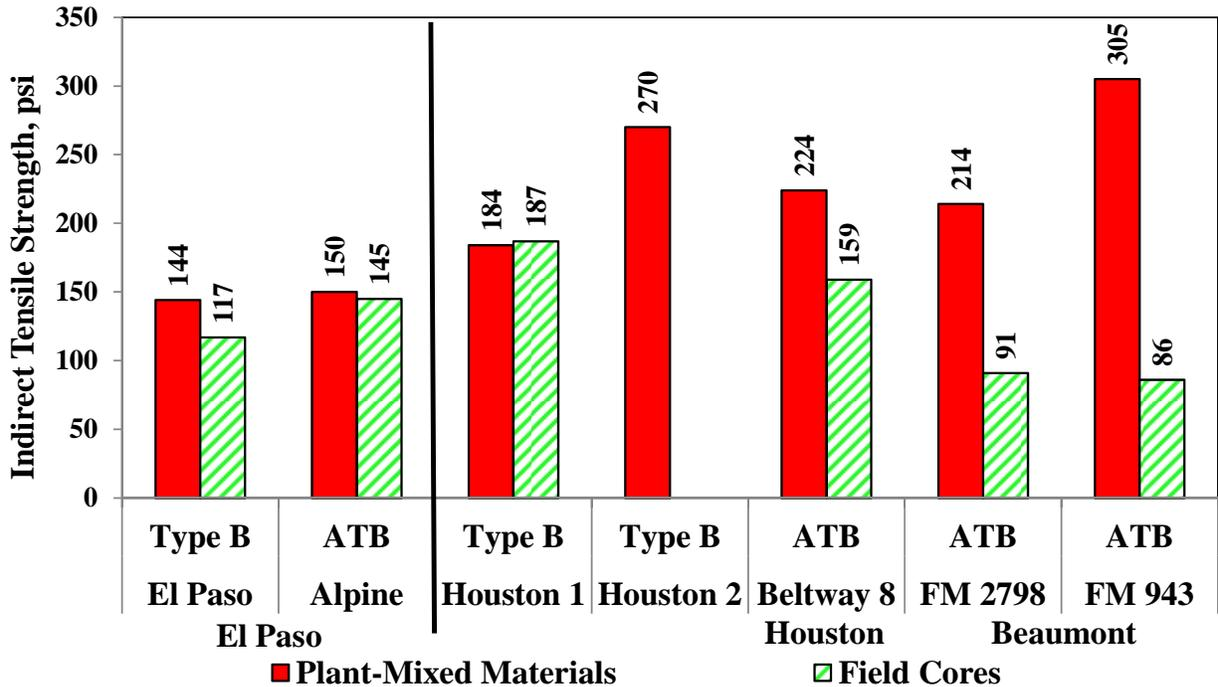
**Figure 7.4 – Comparison of Indirect Tensile Strength for ATB and Type B Specimens**
