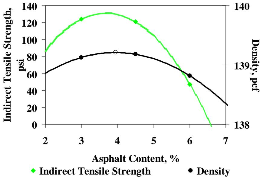
b) Asphalt Content-Density/Strength Curves
