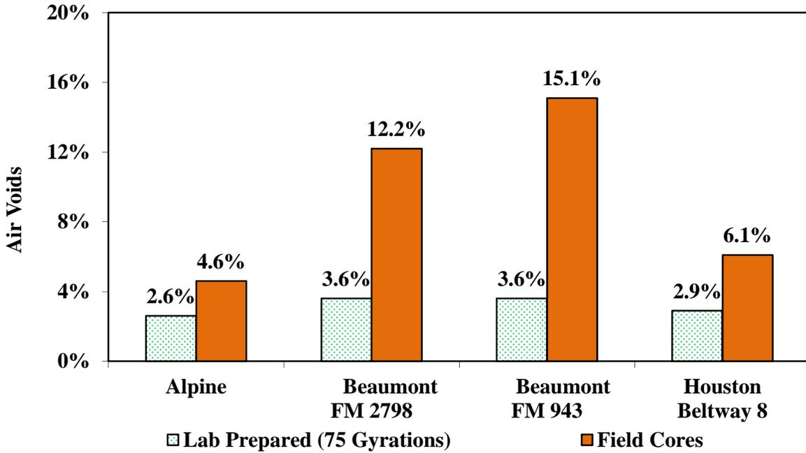
Figure 6.9 - Comparison between Air Voids of Laboratory Specimens and Field Cores
