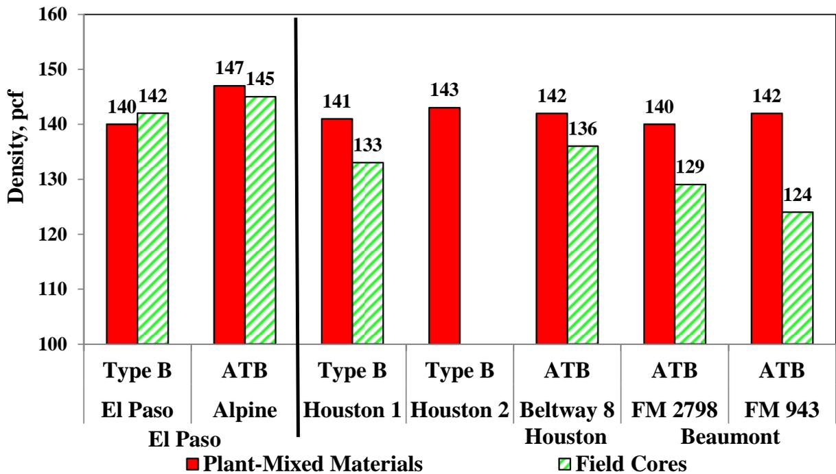
Figure 7.3 – Comparison of Density for ATB and Type B Specimens
