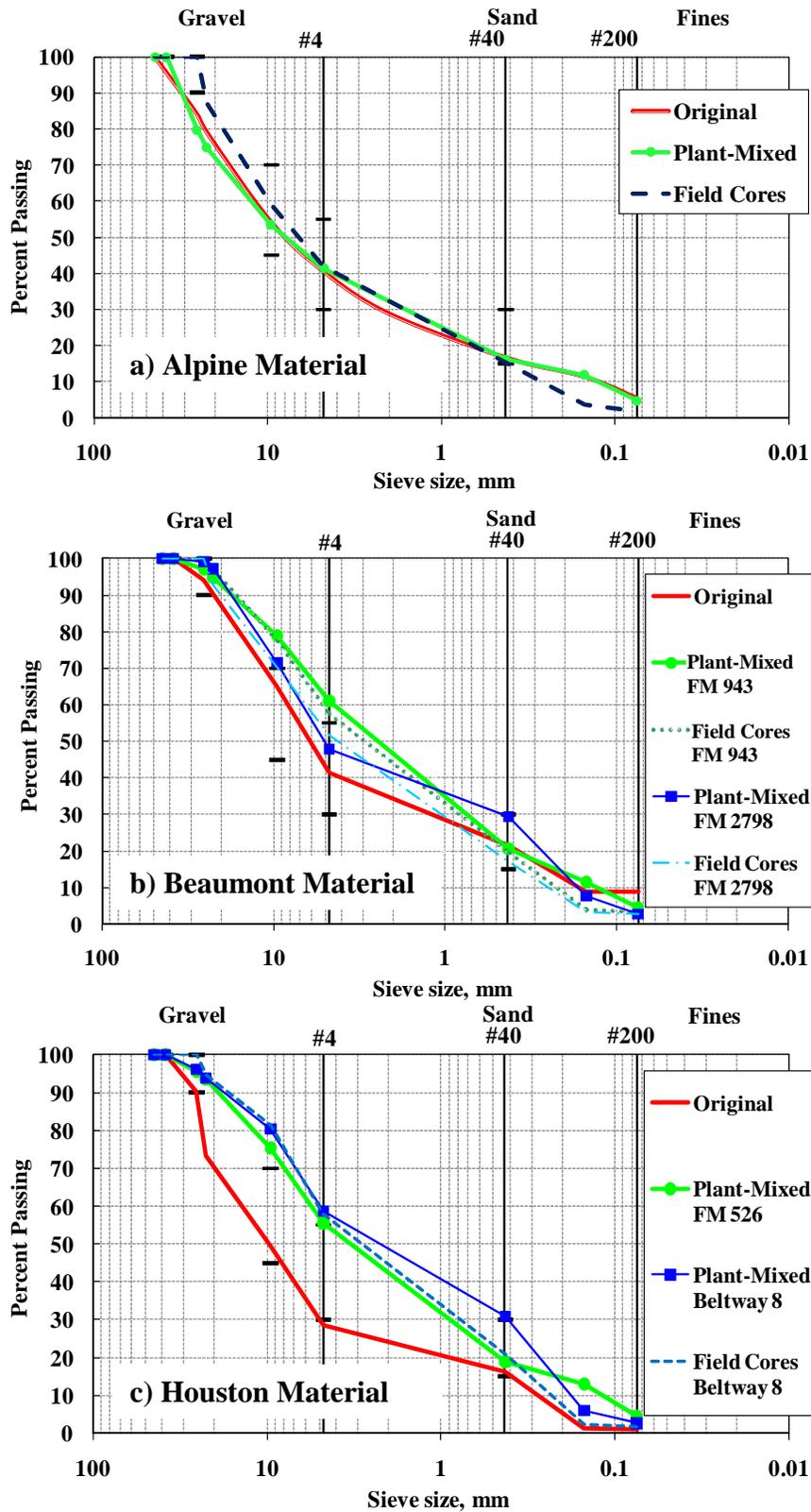
Figure 6.1 – Gradation Curves from Plant-Mixed Materials as Delivered
