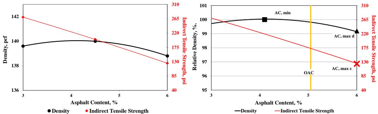
**Figure 6.6 – Density/ Strength vs. Asphalt Content for Beaumont Material**
