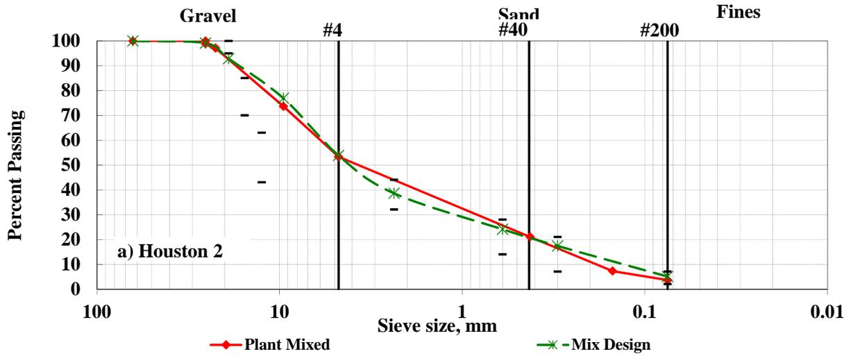
**Figure 7.1 – Gradation Curves from Type B Materials**
