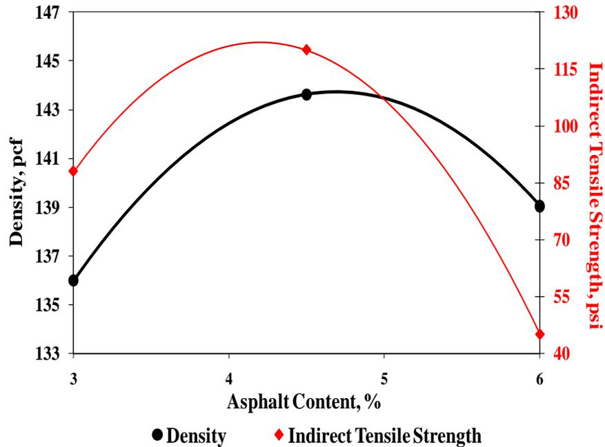
Figure 5.38 – Density/IDT Asphalt Content Combined Curves
