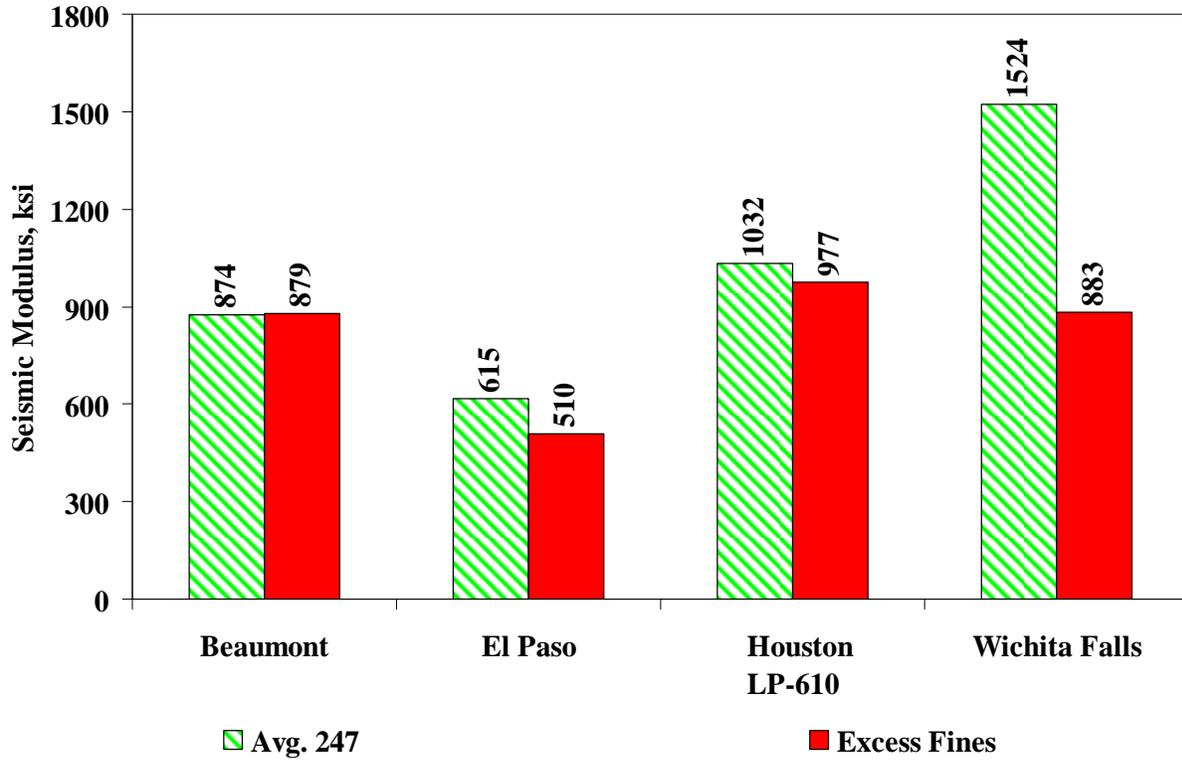
Figure 5.33 – Impact of Fines Content Variation on Modulus for Tex-126-H Protocol.
