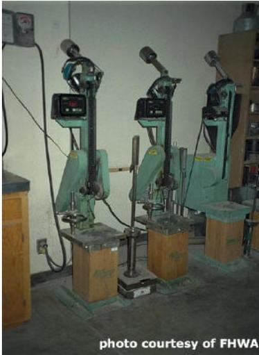
**Figure 2.3 – Marshall Hammer**
