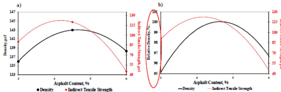
Figure 1 – Asphalt Content/Density/IDT Curve
