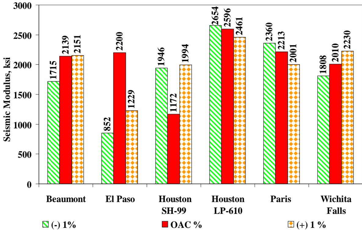
Figure 5.27 – Impact of Asphalt Content Variation on Modulus for Tex-126-H Protocol
