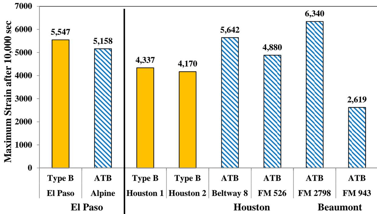
Figure 7.6 – Comparison of Flow Time Tests for ATB and Type B Specimens
