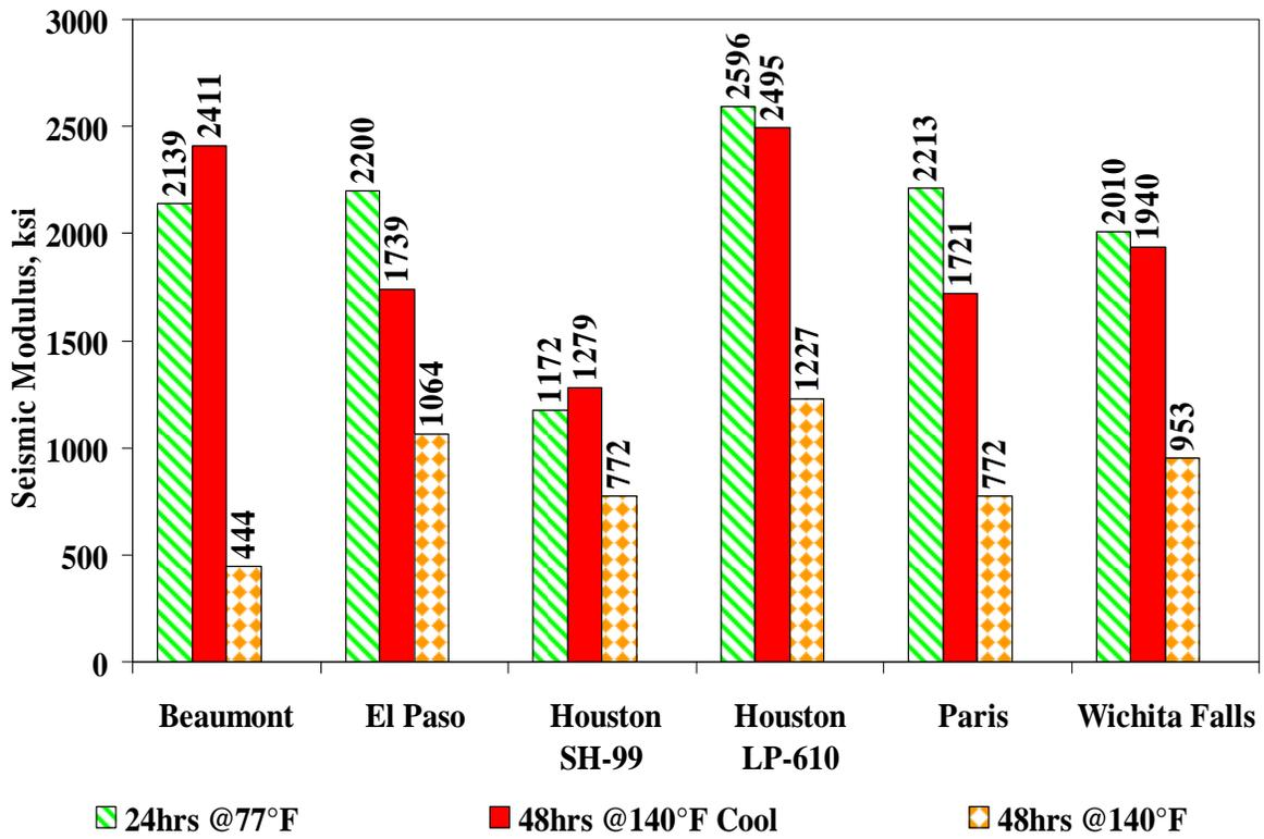
Figure 5.13 – Impact of Curing Temperature on Modulus for Tex-126-H Protocol
