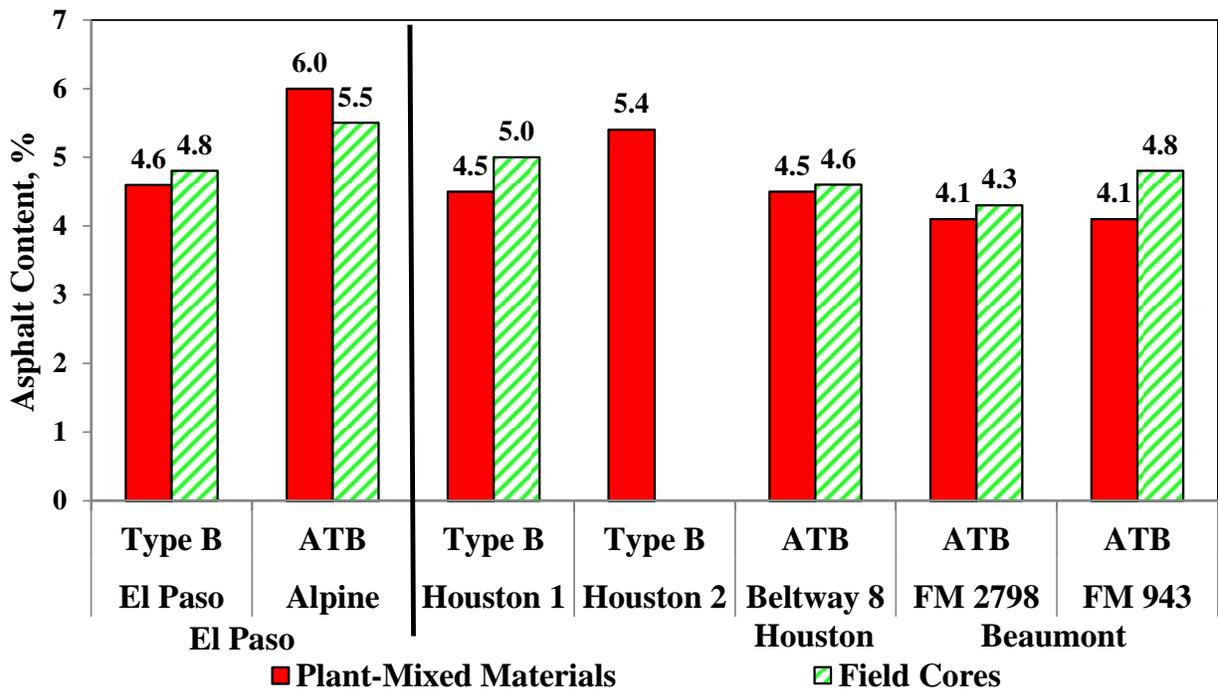
Figure 7.2 – Comparison of Asphalt Content for ATB and Type B Specimens
