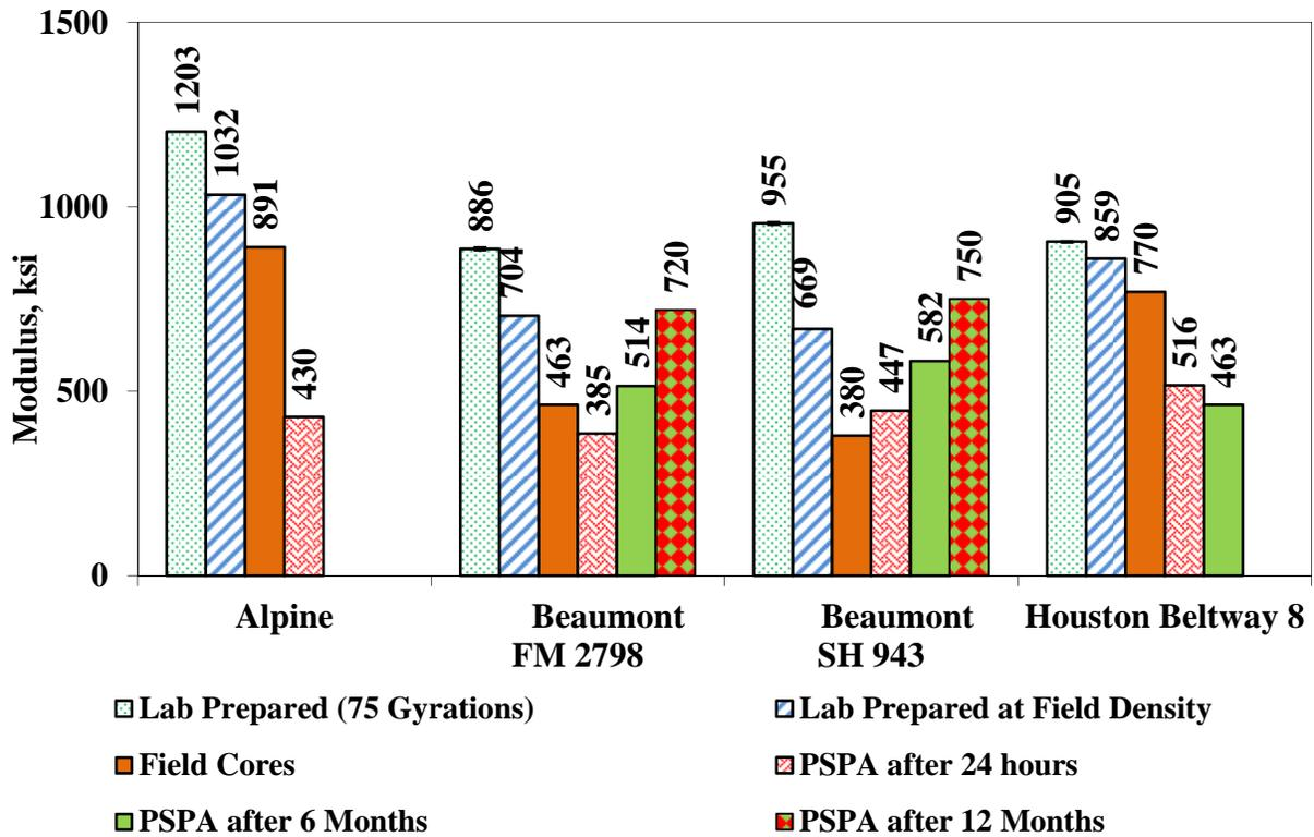
Figure 6.12 - Modulus Comparison between Laboratory and Field Specimens
