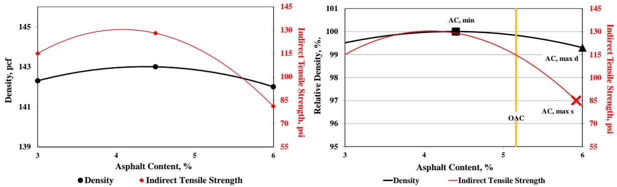
**Figure 6.5 – Density/ Strength vs. Asphalt Content for Houston Material**
