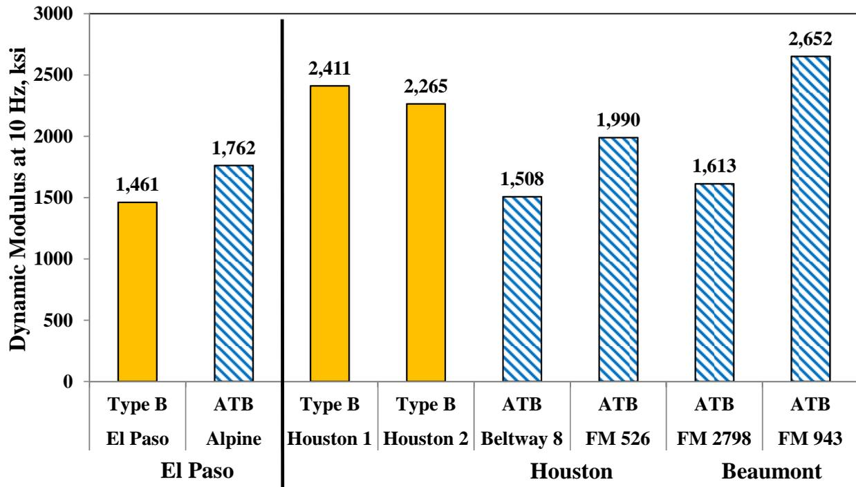
Figure 7.5 – Comparison of Dynamic Modulus for ATB and Type B Specimens
