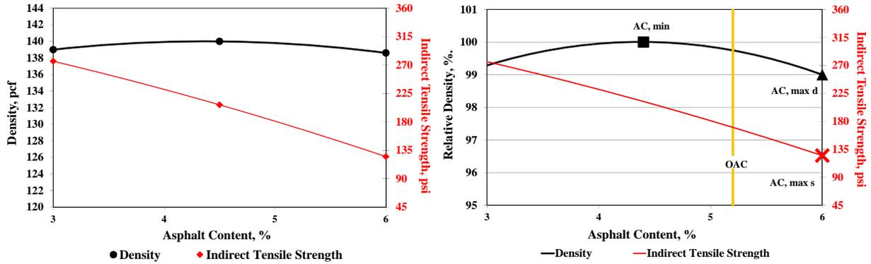
**Figure 6.4 – Density/ Strength vs. Asphalt Content for Alpine Material**
