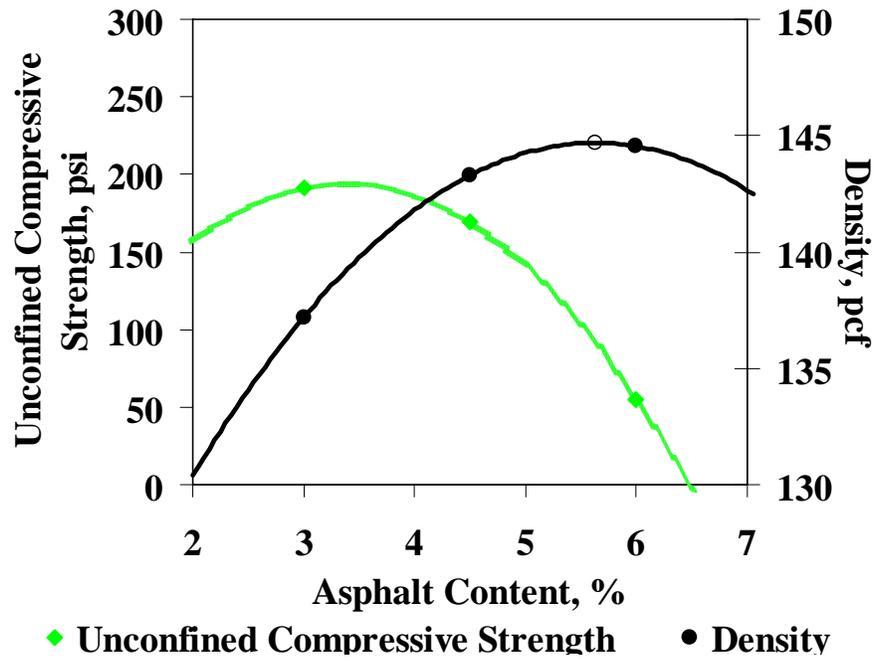
b) Asphalt Content-Density/Strength Curves
