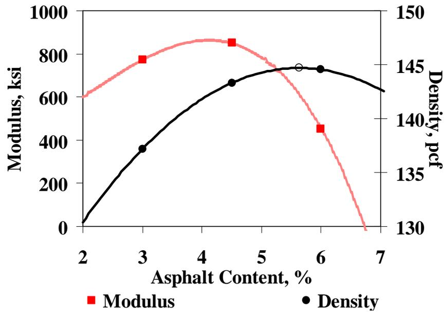
a) Asphalt Content–Density/Modulus Curves
