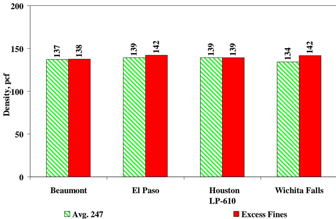
Figure 5.35 – Impact of Fines Content Variation on Density for Tex-204-H.
