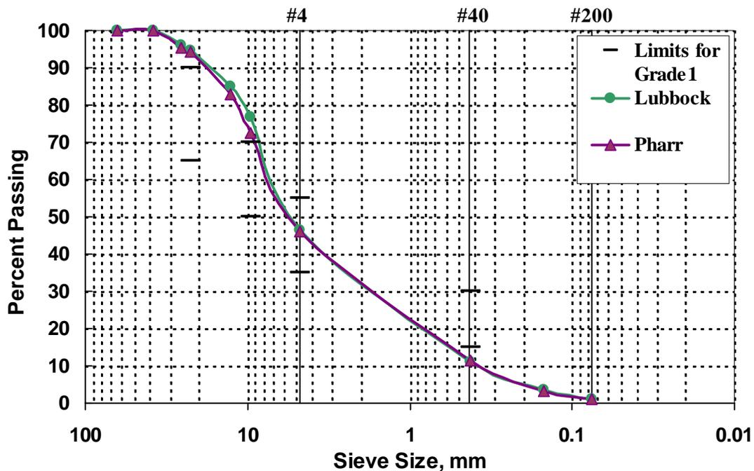
The gradation of the original or recovered aggregate of RAP after oven burning is a different matter. Figure 3.8 shows a comparison of gradations of recovered aggregates from Lubbock and Pharr RAP materials. The recovered aggregate from Lubbock RAP is finer than that from Pharr RAP for all particle sizes.
