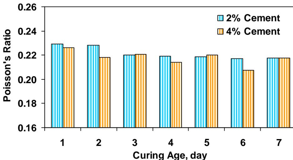
Figure 6.1 – Variations of Poisson's Ratio with Curing Age
