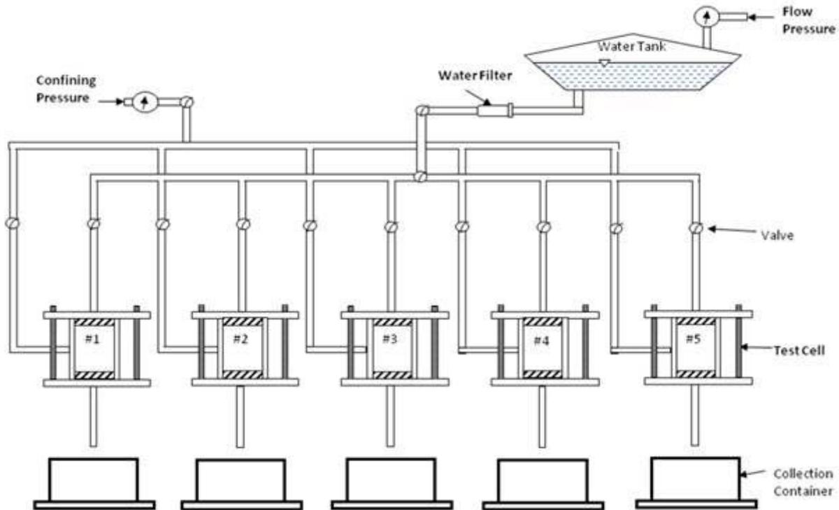
**Figure 5.2 – Schematic of Leachate Process (Chittoori, 2008)**
