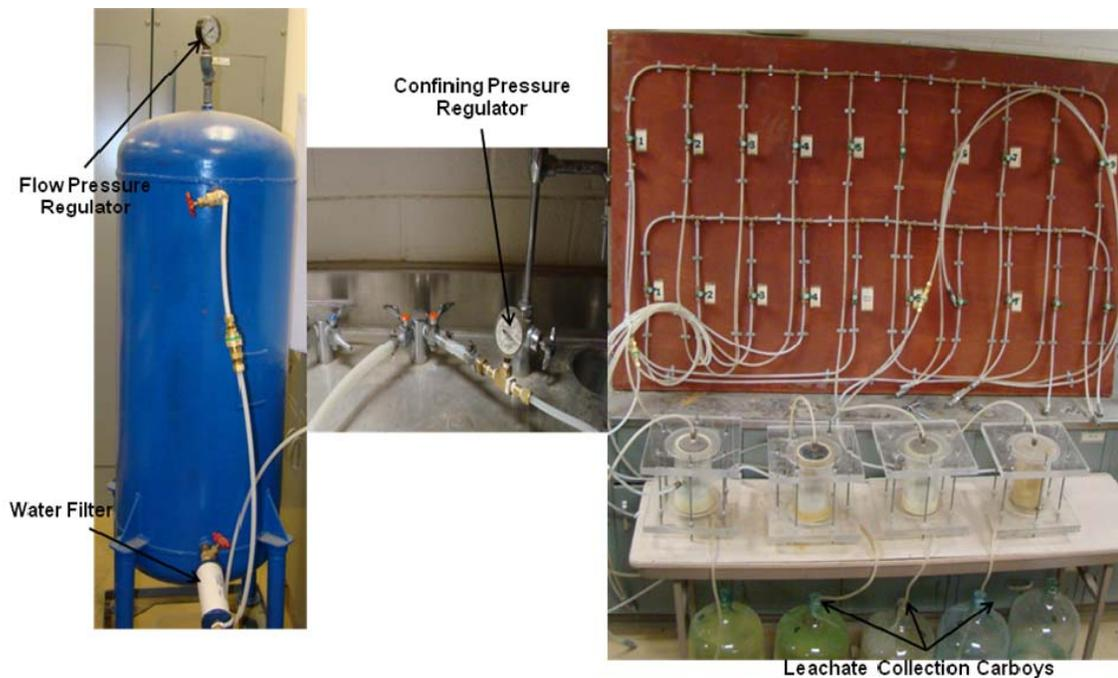
**Figure 5.4 – Test Setup for Leachate Studies (Chittoori, 2008)**
