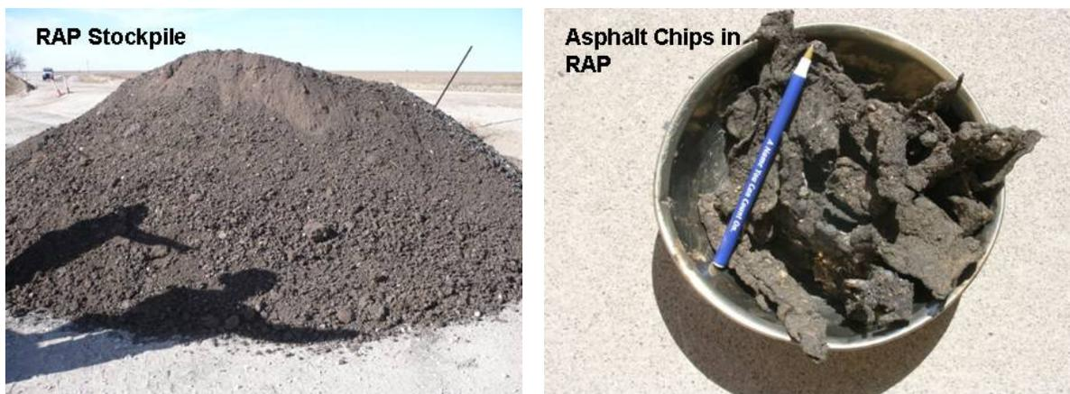
Figure 3.3 – Lubbock RAP and Asphalt Chips in RAP
