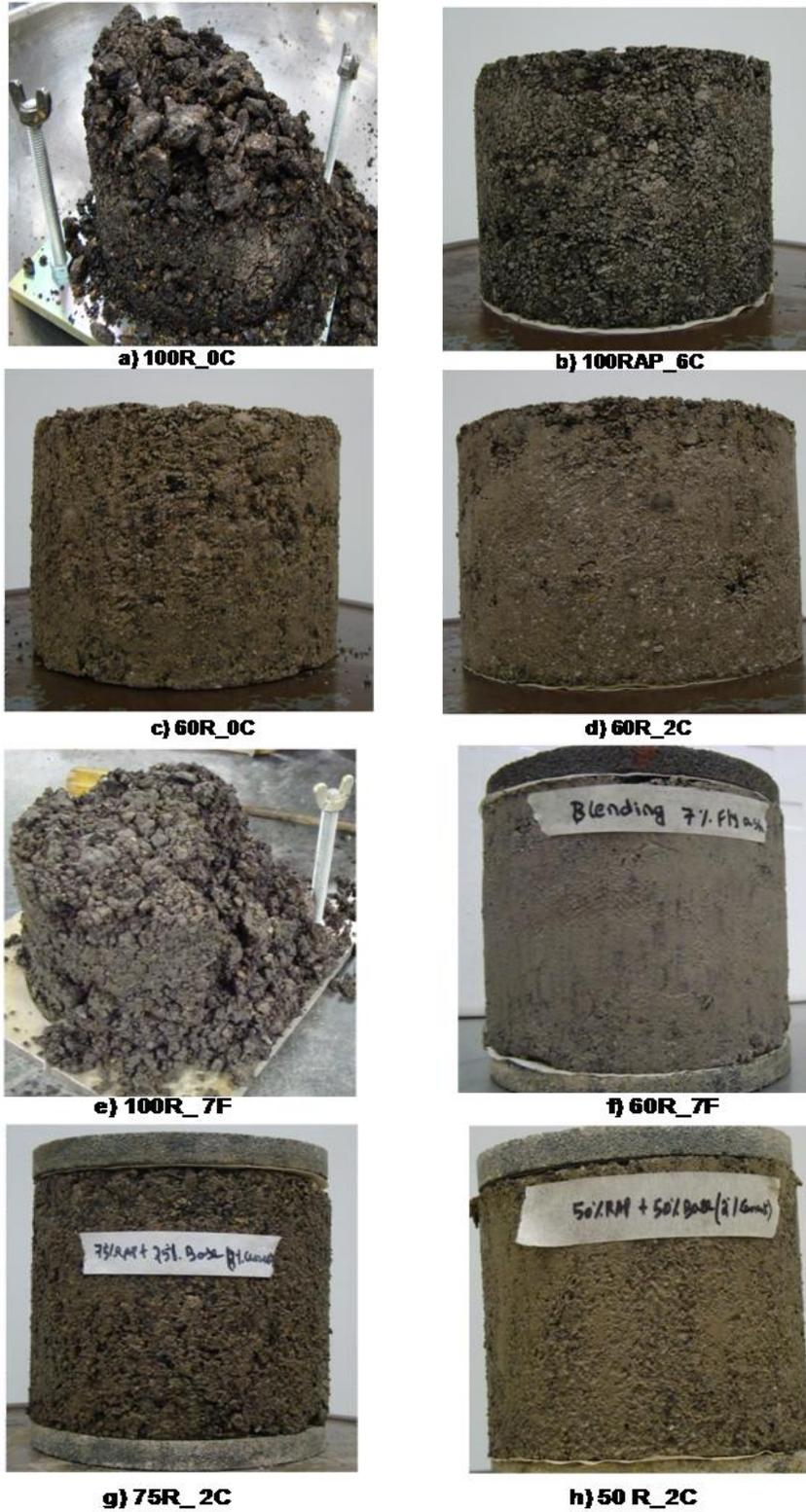
Figure 5.10 – Typical RAP and RAP Blends from El Paso District Prior to Wetting/Drying
