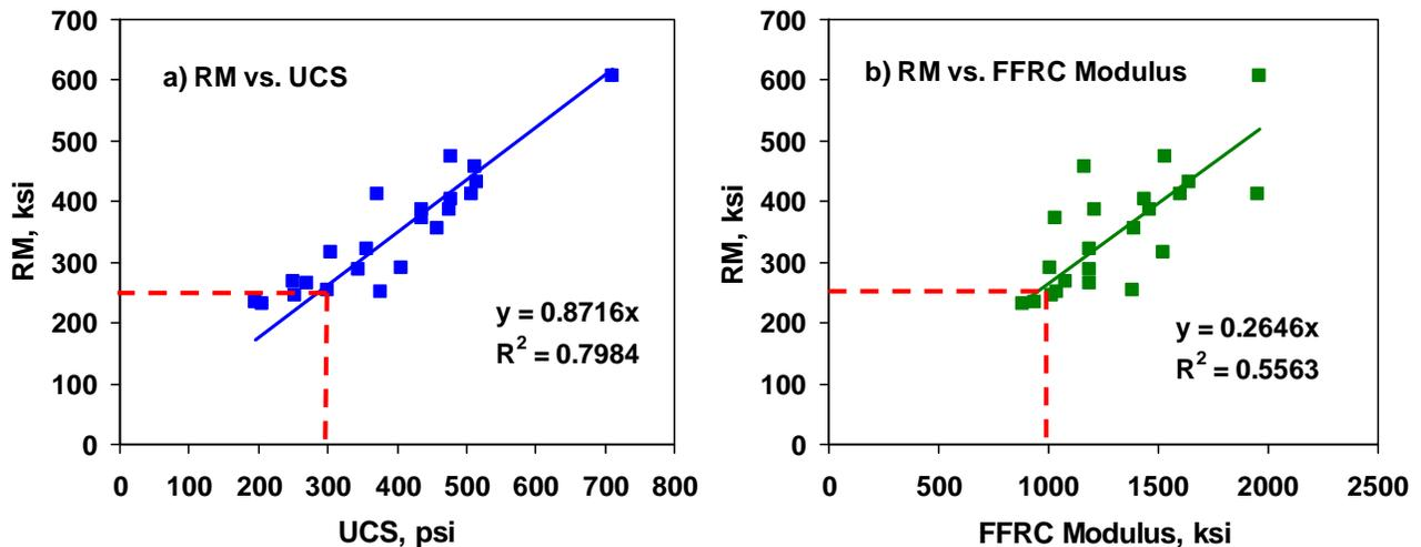
**Figure 4.9 – Resilient Modulus vs. UCS and FFRC Modulus**
