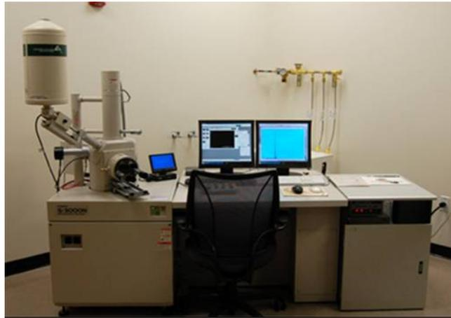
**Figure 5.8 – Scanning Electron Microscope (SEM) Test Setup**
