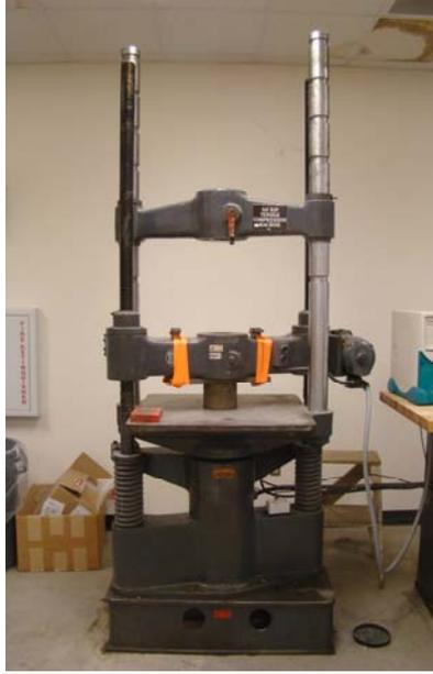
**Figure 5.5 – Unconfined Compression Test Machine**
