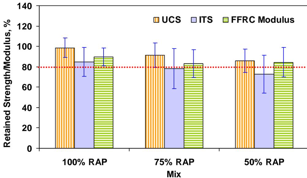
Figure 4.10 – Average Retained Strengths and Modulus
