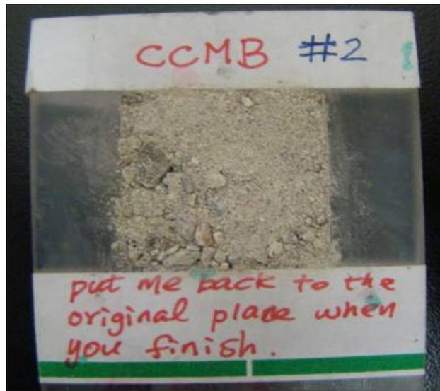
**Figure 5.6 – Sample Holder with Typical Powdered RAP Mix**
