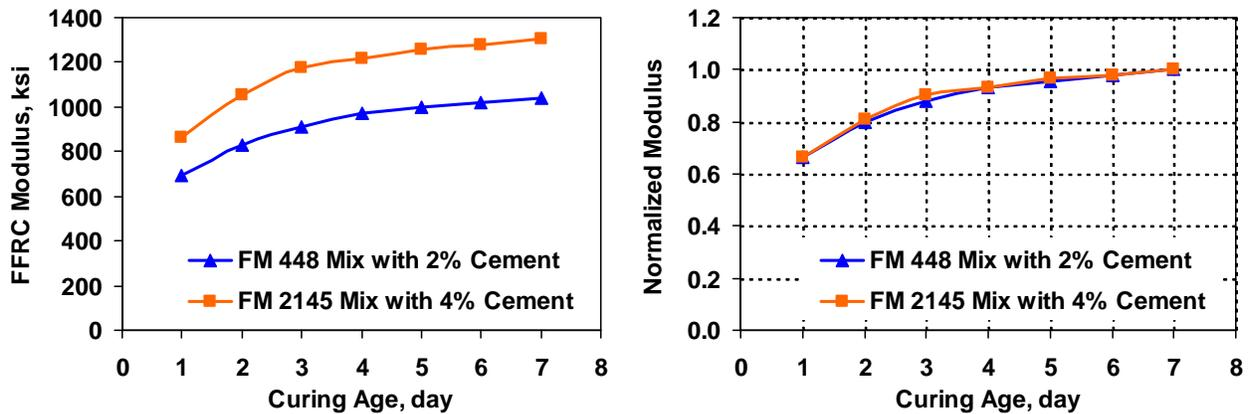
Figure 6.2 – FFRC Modulus Gain with Curing Age
