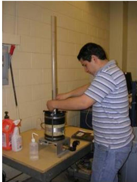
**Figure 4.3 – Setup for Hydraulic Conductivity Test**
