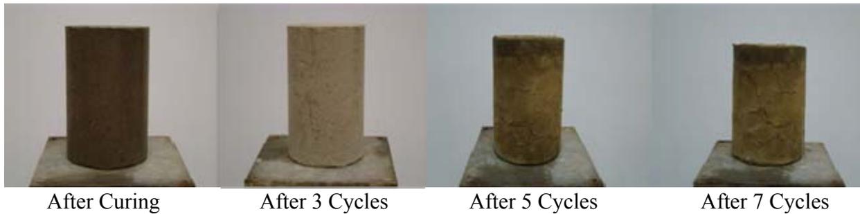
**Figure 5.13 – Changes in Paris Soil Sample (Treated) with Wetting/Drying Cycles**
