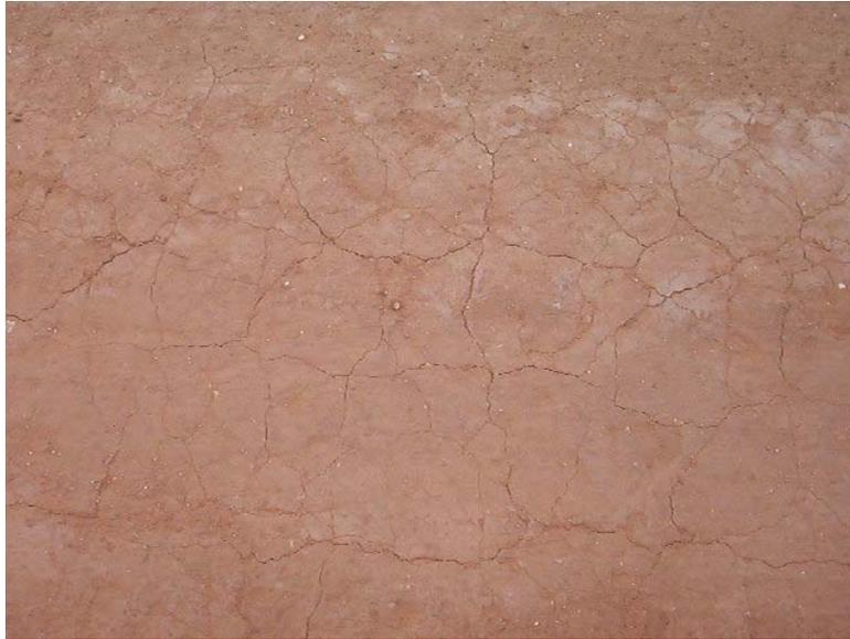
Figure 6.18 – Surface Cracking after 3 Days of Curing
