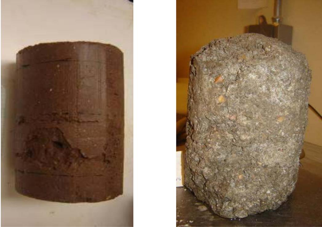
**Figure 4.8 – Submerge Test Specimens after Test**
