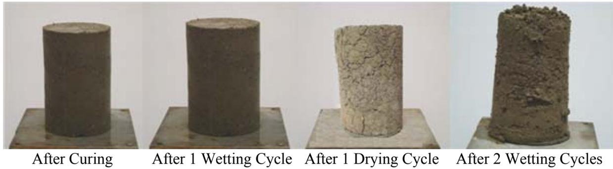
**Figure 5.12 – Changes in Paris Soil Sample (Untreated) with Wetting/Drying Cycles**
