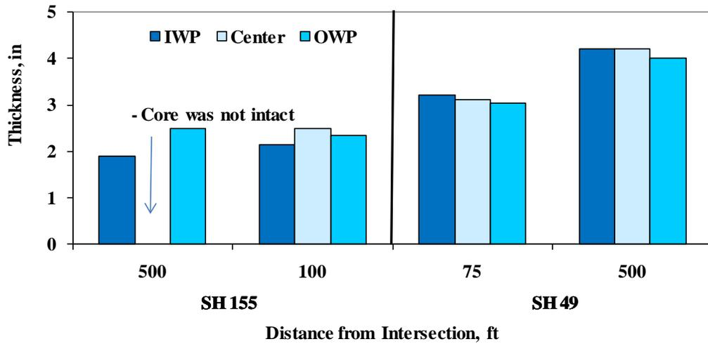
Figure 5.10 - Core Average Thicknesses as Approaching the Intersection.
