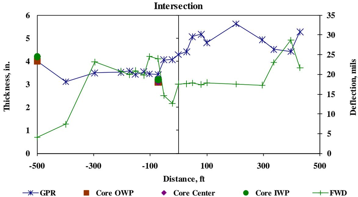
**Figure 5.17 - GPR, FWD and Cores on SH 49.**
