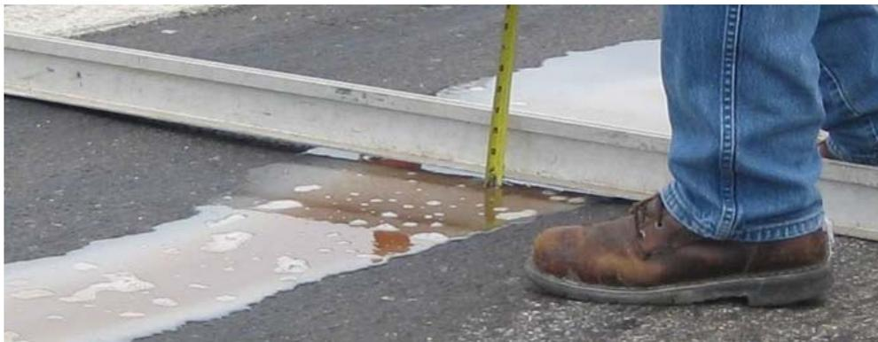
**Figure 5.5 - Rut Depth Measurement on SH 155.**
