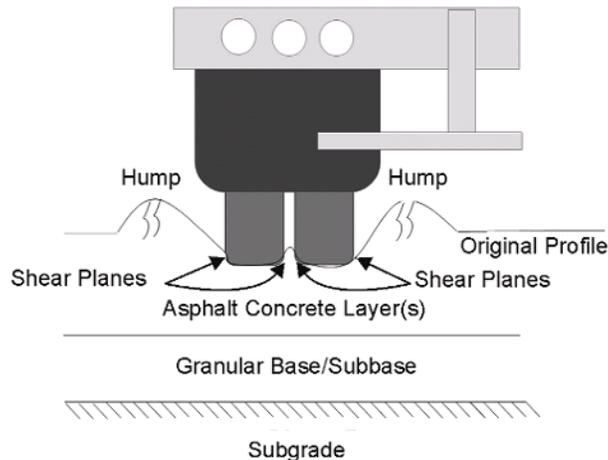
**Figure 2.4 - Instability or Plastic Flow on Asphalt Pavements (Federation of Canadian Municipalities and Canadian National Research Council 2003).**
