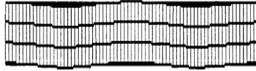
**Figure 2.3 - Surface Deformation Due to Subgrade Deformation. (Fang, 2001)**
