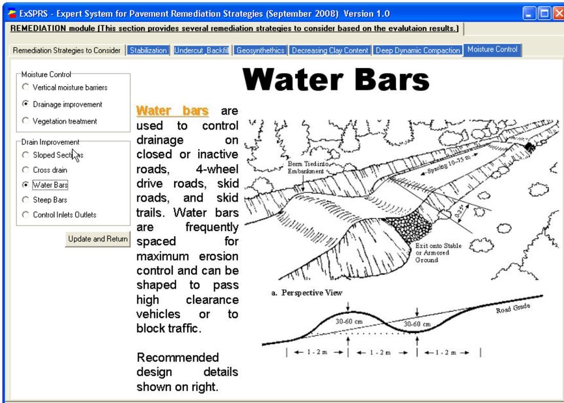
Figure 4.9—Moisture Control Method of Using Water Bars
