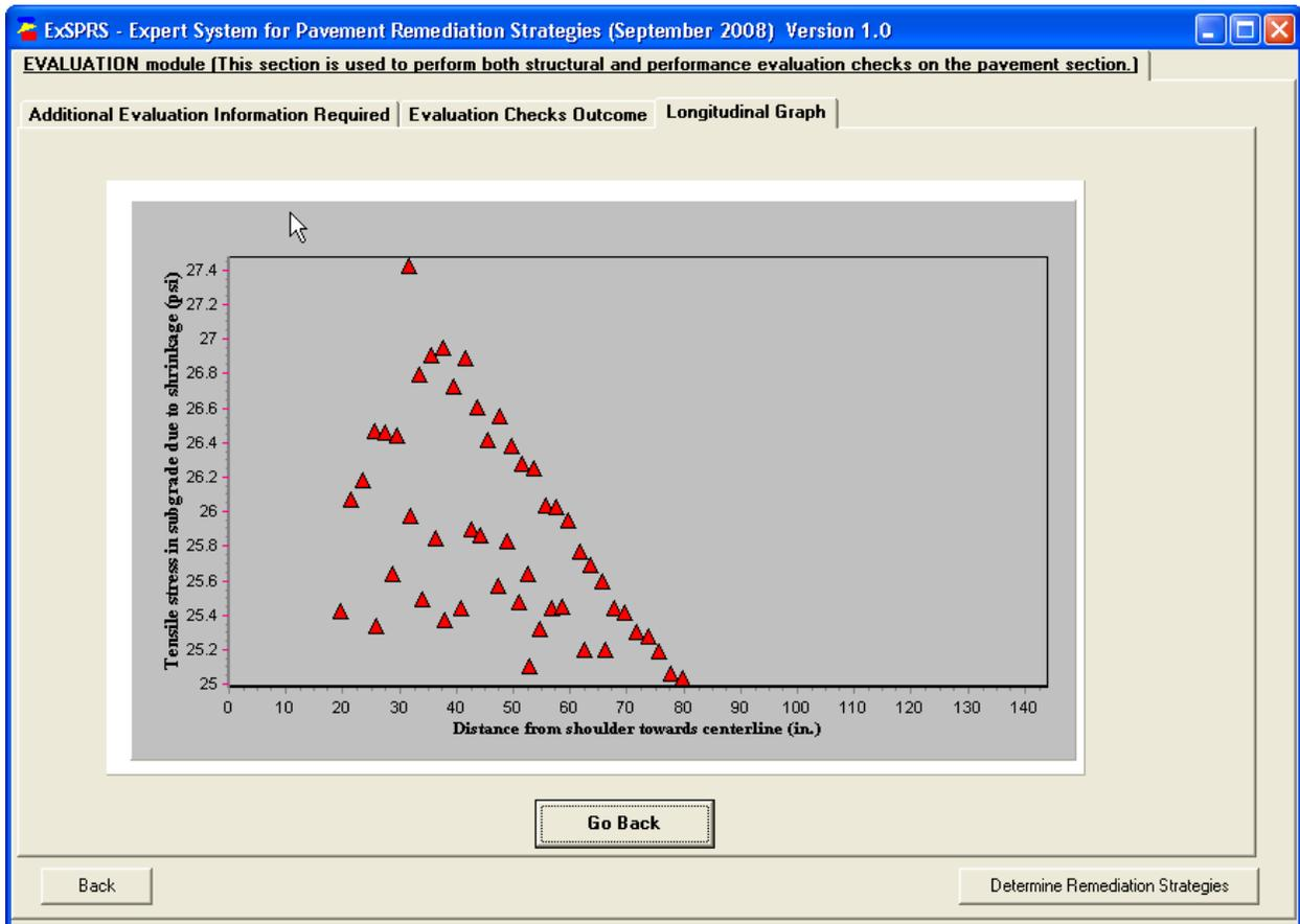
Figure 3.4—Longitudinal Cracking Check Graphical Result
