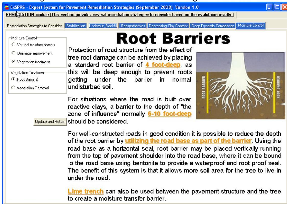
Figure 4.12—Moisture Control Method of Using Root Barriers
