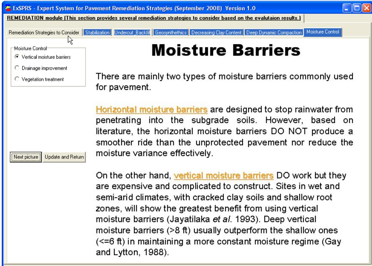
Figure 4.6—Moisture Control Method of Using Moisture Barriers
