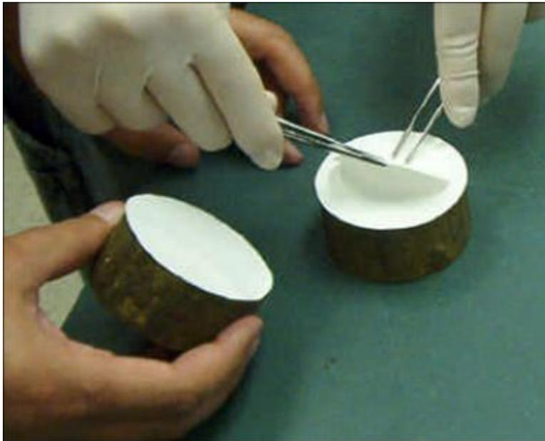
**Figure 2.13—Filter Paper Suction Measurement**
