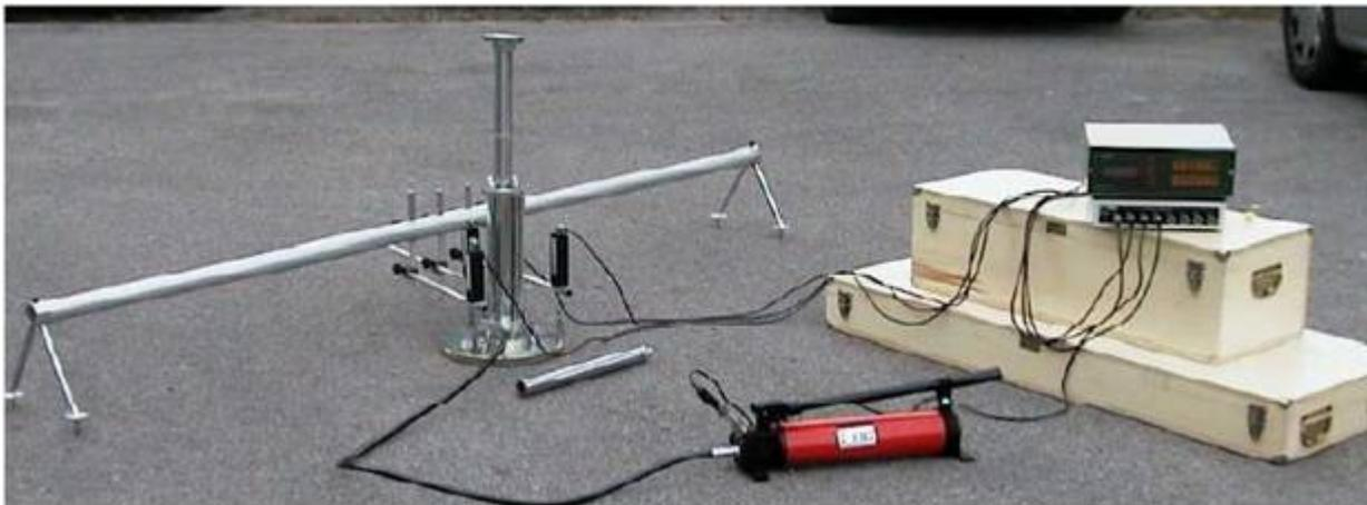
**Figure 2.8—Plate Bearing Test Apparatus**
