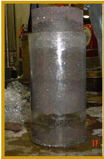
**Figure 3.3 – Clay Specimen Subjected To Wetting by *Method 3***
