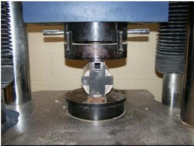
**b) Specimen Setup for IDT**
