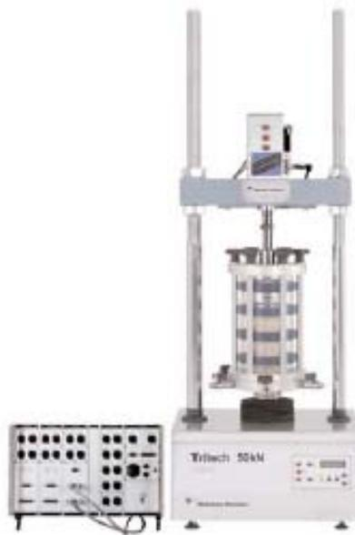
**Figure 2.6 – Cyclic Triaxial Test Apparatus**
