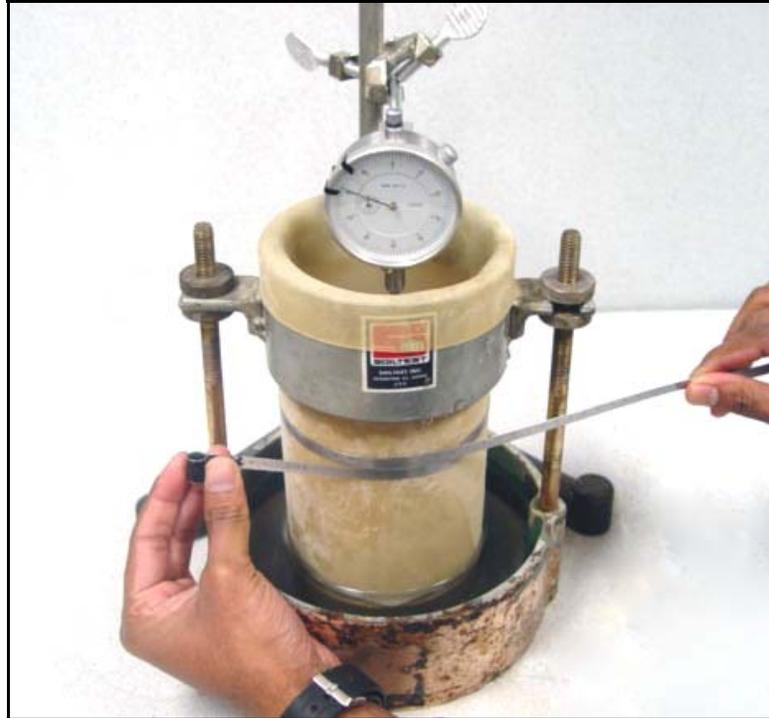
**Figure 4.11 - Three-Dimensional Free Swell Test Setup**
