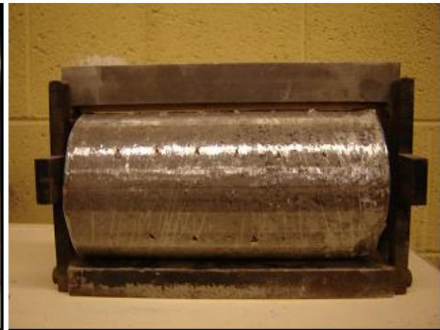
**Figure 2.5 – Indirect Tensile Strength Setup**
