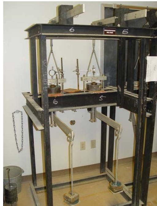
**Figure 4.12 - Modified Consolidation Test Setup for Swell Pressure Test**
