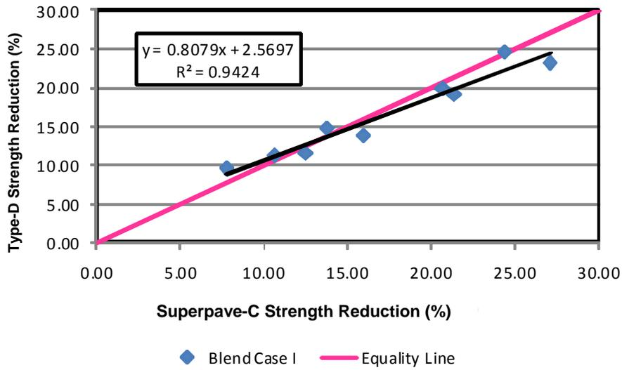
**Figure 4.13 - Superpave-C vs. Type-D Strength Reduction (Case I)**
