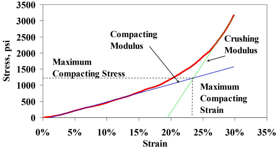
Figure 2 - Typical Results for the ACV Test
