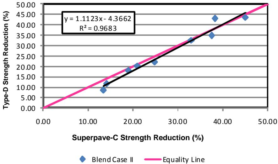
**Figure 4.14 - Superpave-C vs. Type-D Strength Reduction (Case II)**
