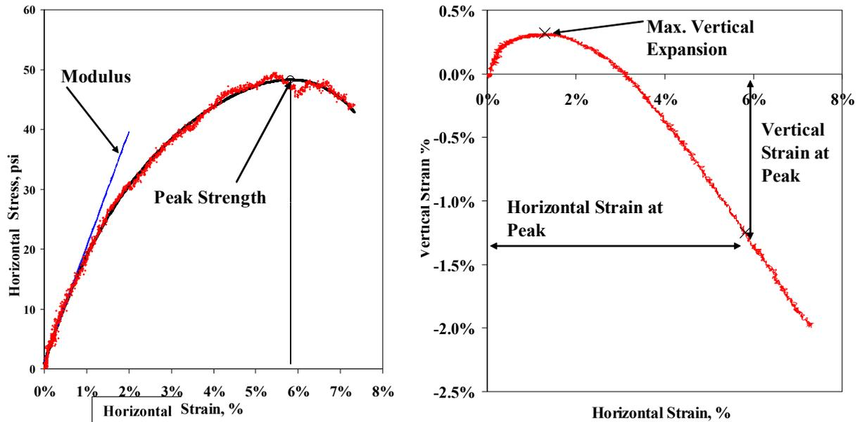
**a) Horizontal Stress vs. Horizontal Strain Plot      b) Vertical Strain vs. Horizontal Strain**
