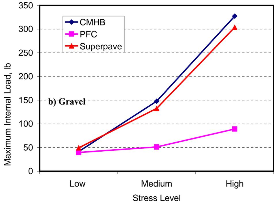
**Figure 6.8 – Internal Force Changes with Increasing Applied Load**
