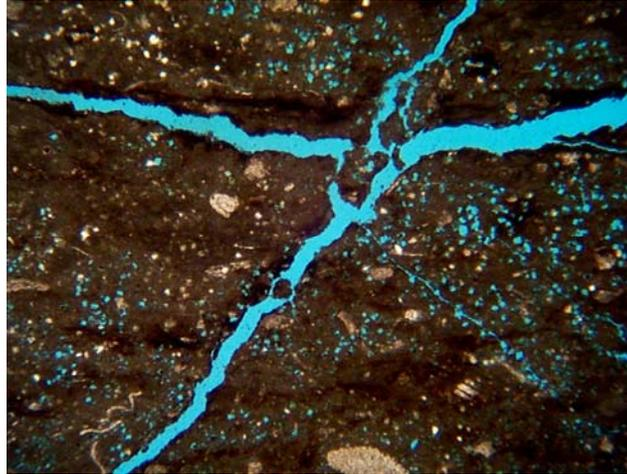
**Figure A.17 - Photomicrograph Showing Solution Widened Fractures and Micro Porosity due to Dissolution of Grains in the Dark Micrite**
