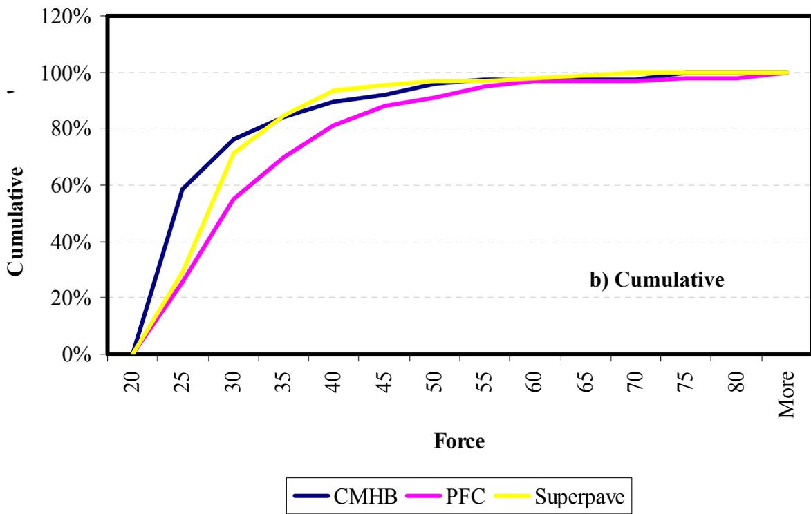
**Figure C.2 – Internal Shear Forces Distribution Results for Hard Limestone**
