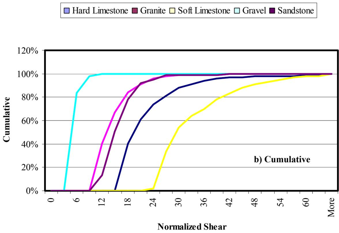
**Figure C.20 – Internal Shear Forces Distribution Results for PFC**
