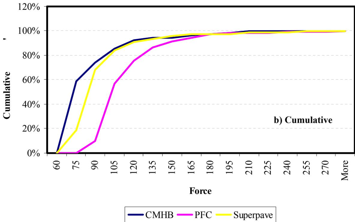
**Figure C.7 – Internal Compression Forces Distribution Results for Granite**
