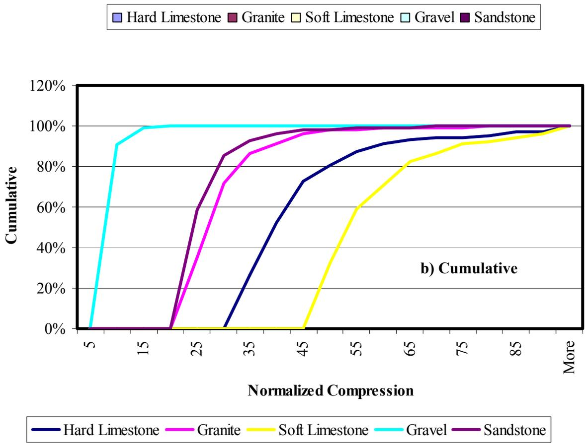
**Figure C.19 – Internal Compression Forces Distribution Results for PFC**
