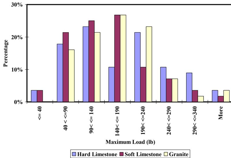
**Figure B.1 - Single Aggregate Crushing Results Distribution (Vertical)**
