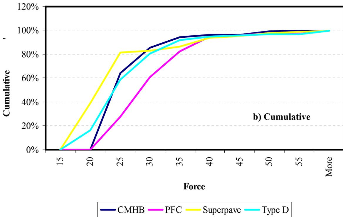
**Figure C.11 – Internal Shear Forces Distribution Results for Gravel**
