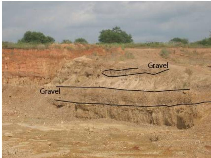
**Figure A.6 - Stratigraphy in the Gravel Quarry**
