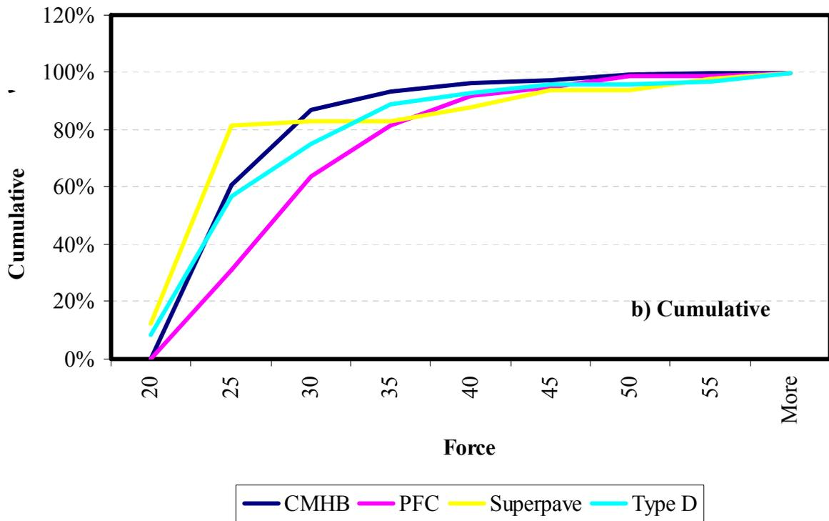
**Figure C.14 – Internal Shear Forces Distribution Results for Sandstone**
