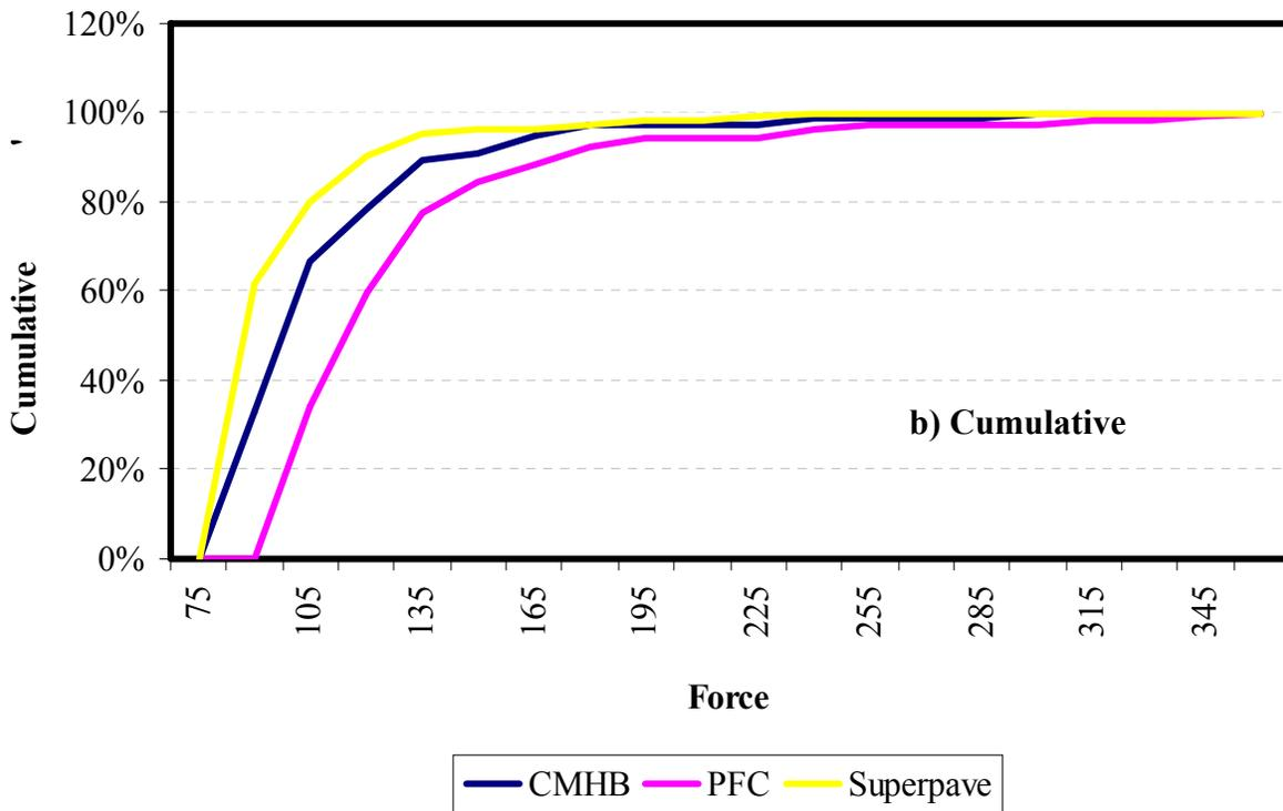
Figure C.1 – Internal Compression Forces Distribution Results for Hard Limestone
