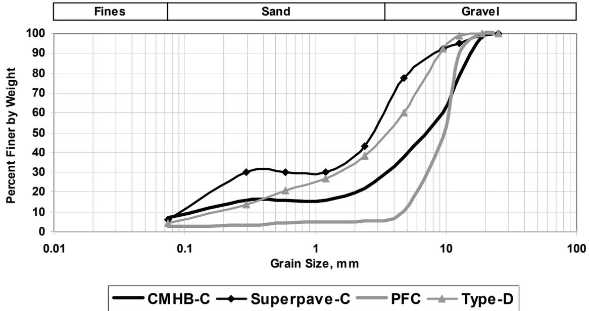
Figure 2.1 – Gradations of Mixes Used in This Study
