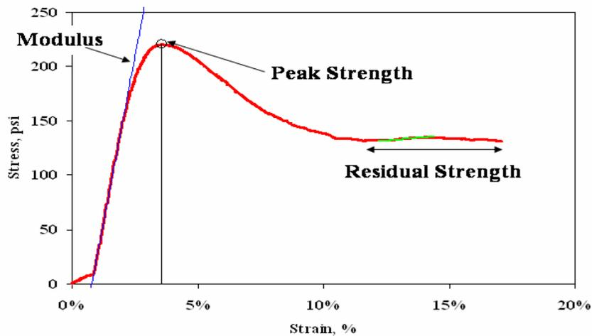
**Figure 4.2 - Typical Results from the Triaxial Test**
