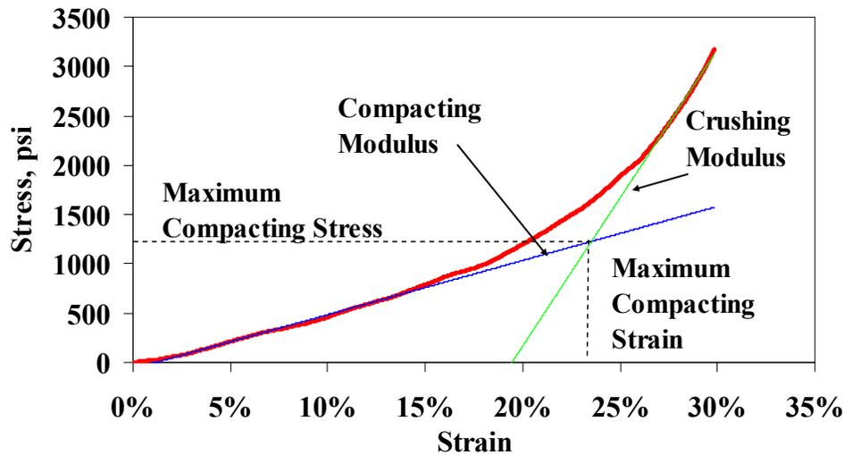
Figure 3.1 - Typical Results for an ACV Test
