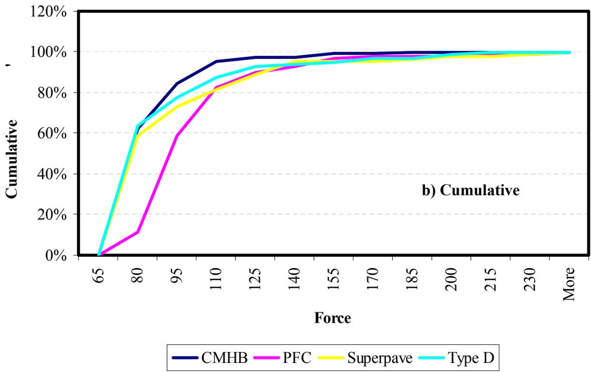
Figure C.13 – Internal Compression Forces Distribution Results for Sandstone
