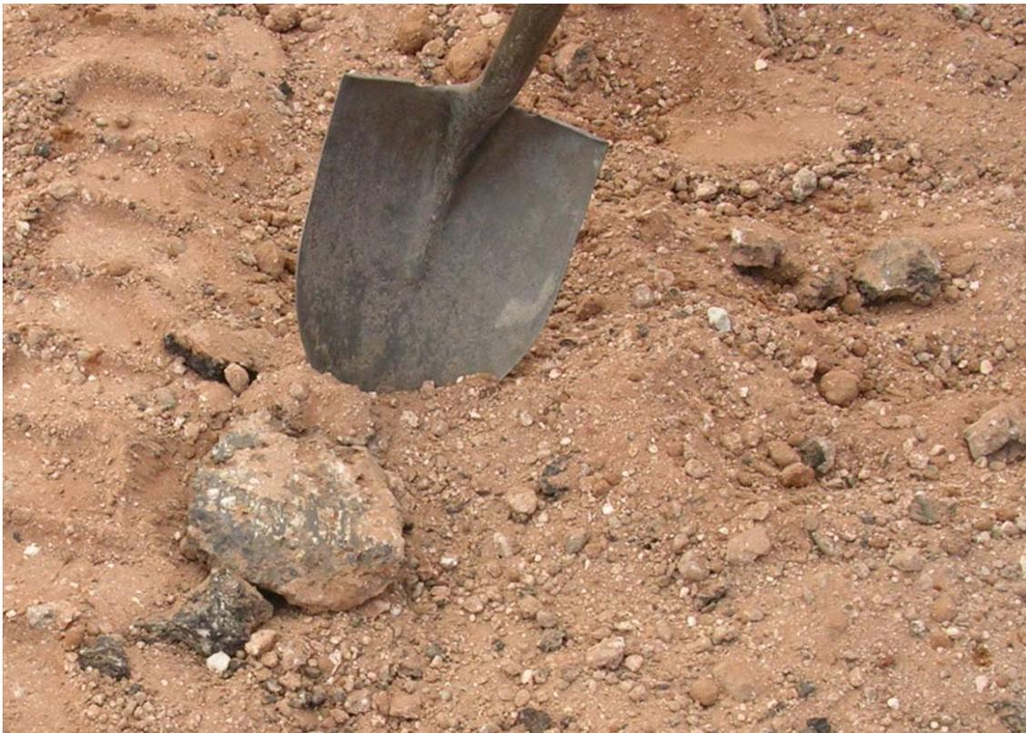
**Figure 5.7 - Large-size HMA after pulverization**
