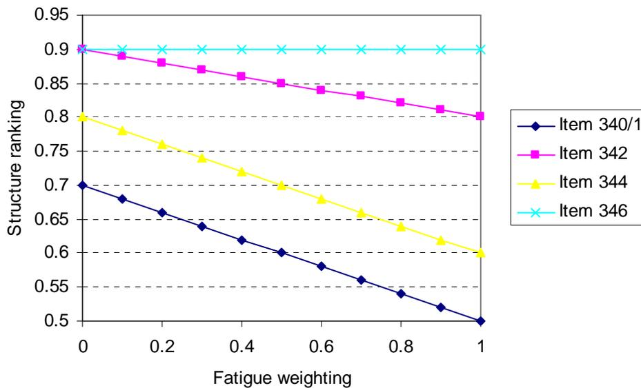
**Figure 11. Structure Ranking of HMA Mixtures in terms of Fatigue Weighting**
