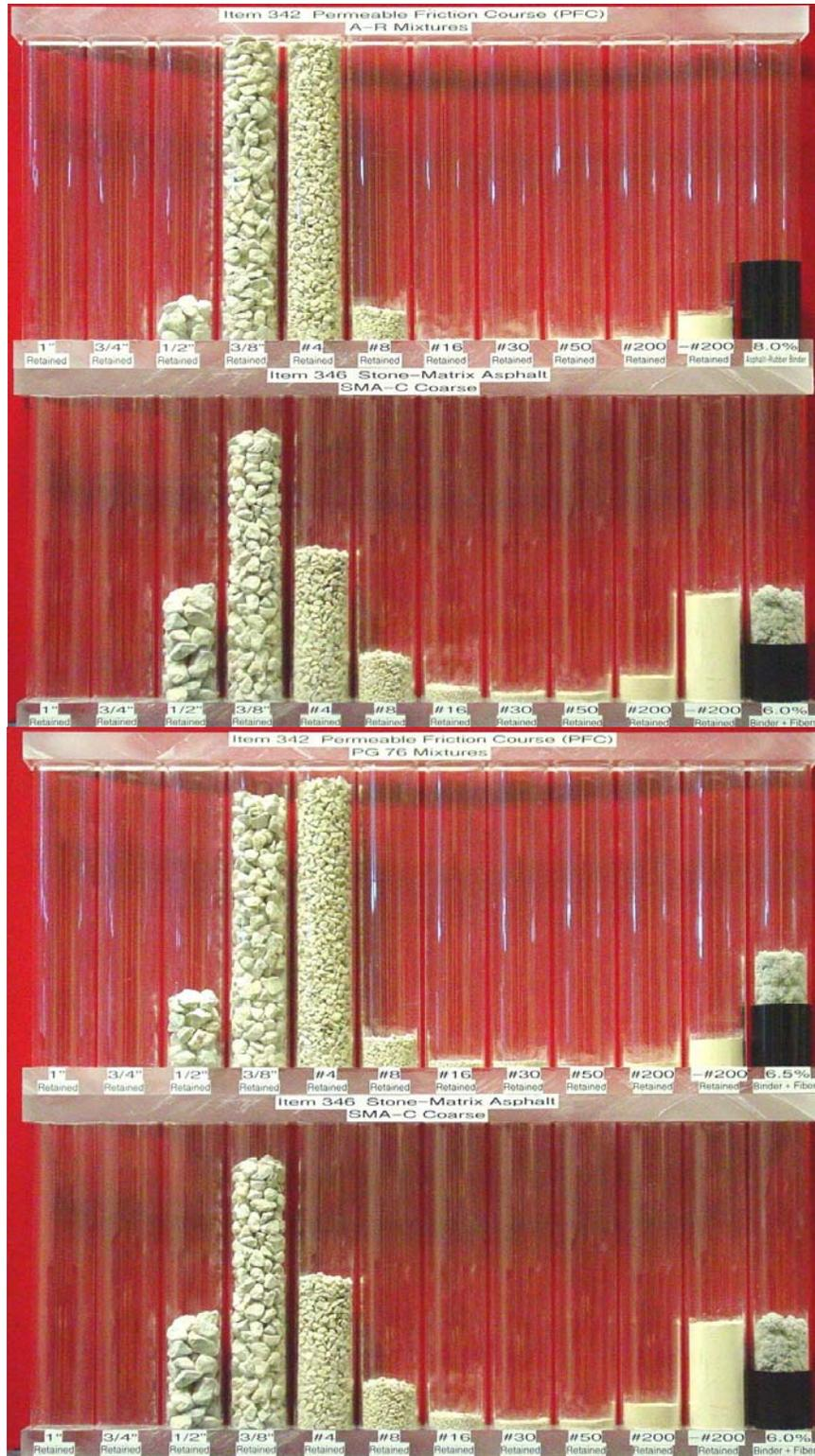
**Figure 6. Comparison Between SMA and PFC Mixes**
