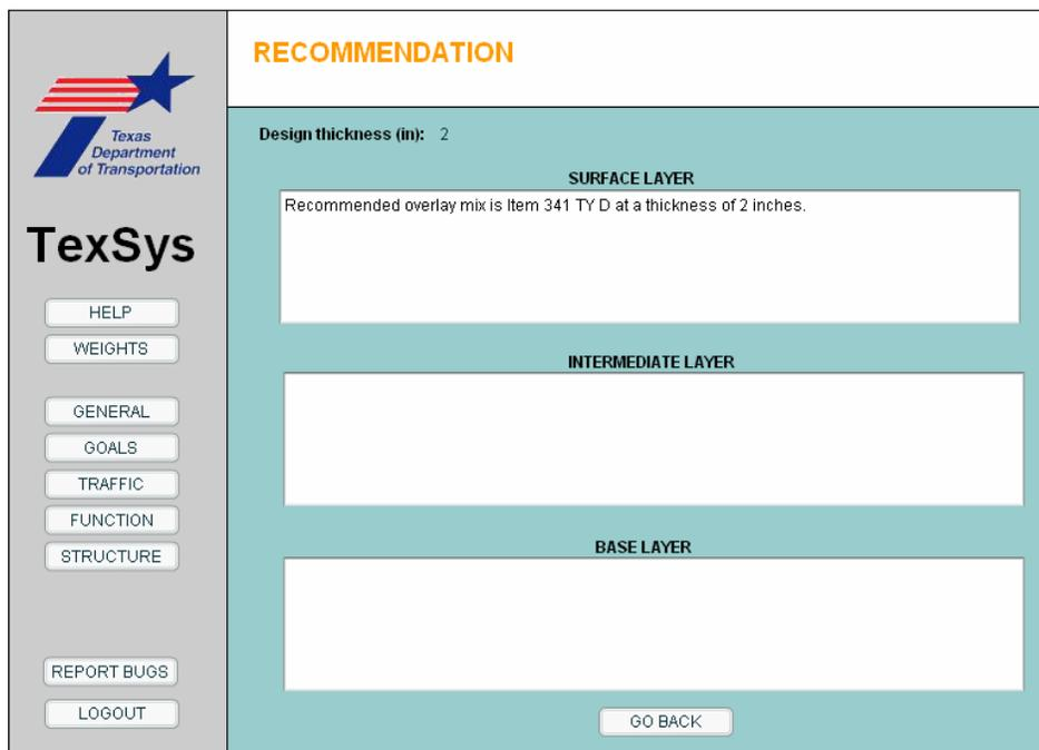
**Figure 26. TexSys Layer Thickness Recommendation for El Paso District Example.**
