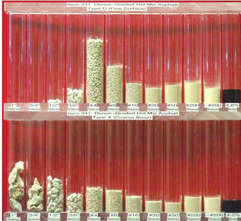
**Figure 8. Comparison Between Coarse and Fine Mixes of ITEM 341**
