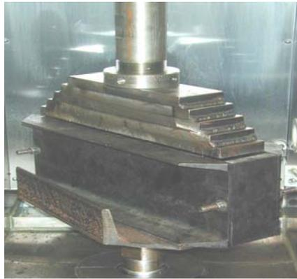
**FIGURE 20** Top Loading Platen for Compaction of Fatigue Specimens
