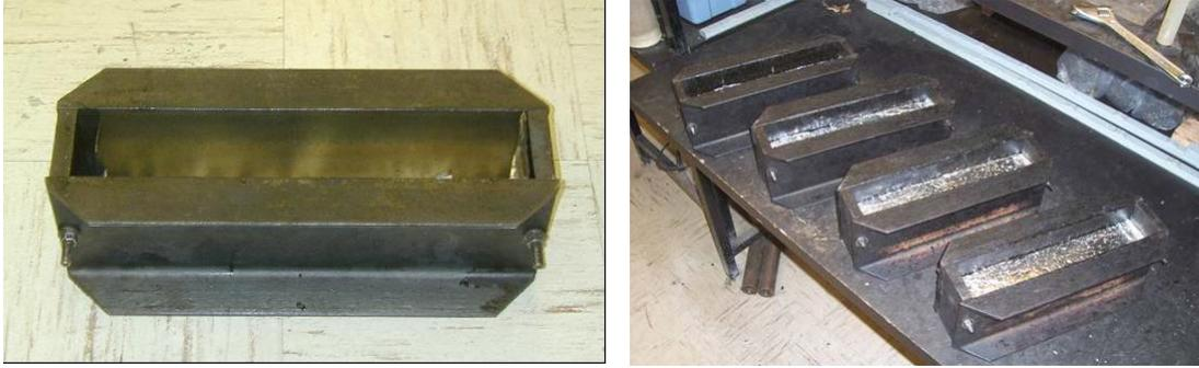
**FIGURE 19** Manufactured Mold for Beam Compaction and Compacted Specimens.
