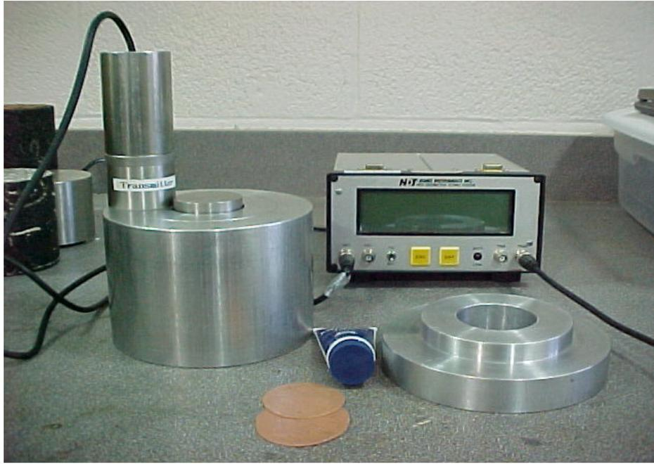
**FIGURE 21 Ultrasonic Test Device for HMAC Specimens**
