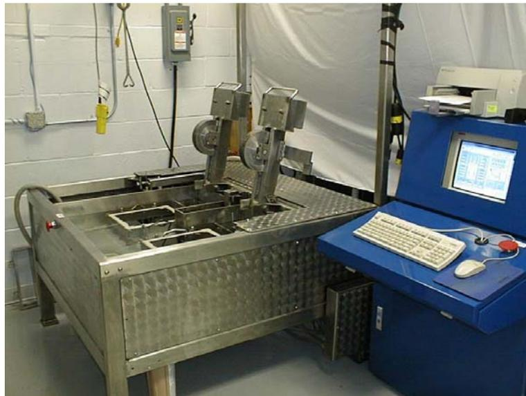
**FIGURE 2 Hamburg Wheel Tracking Device Test Set Up**
