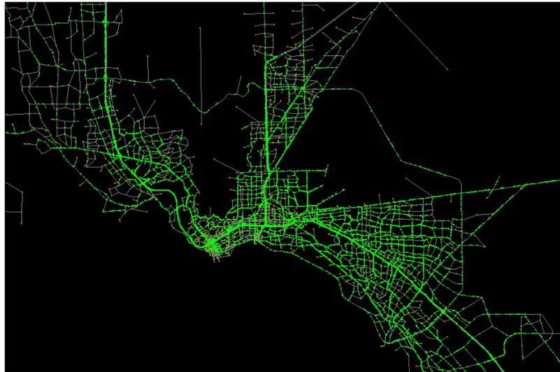
**Figure 2-2 DYNASMART-P Network Visualization**
