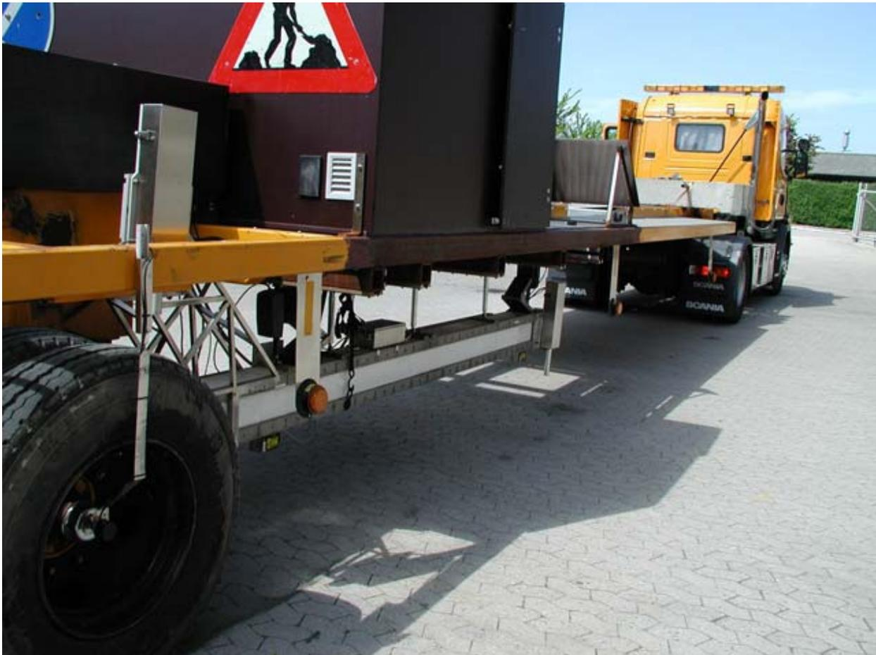
**FIGURE 4 Danish High Speed Deflectograph (Hildebrand, et. al. 2002)**
