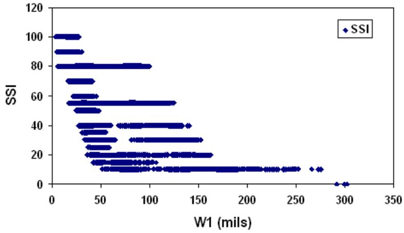
**FIGURE 29 SSI Compared with W1 for Pavement Type 5**
