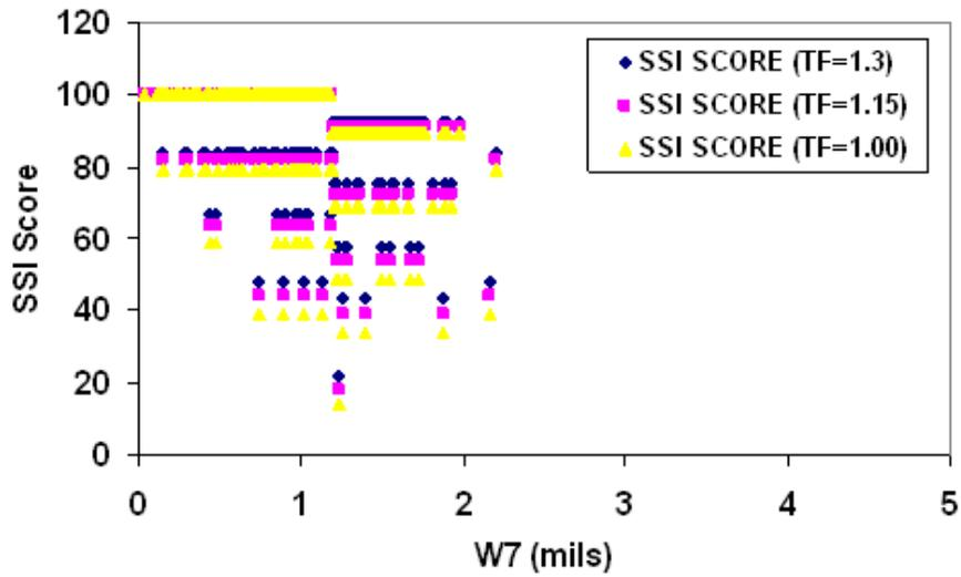
**FIGURE 25 SSI Score Compared to W7 for Pavement Type 4**
