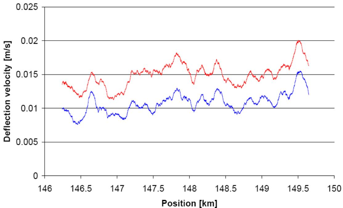
**FIGURE D. 4 Repeatability of Deflection Velocities by the HSD (Hildebrand, et. al., 2002)**
