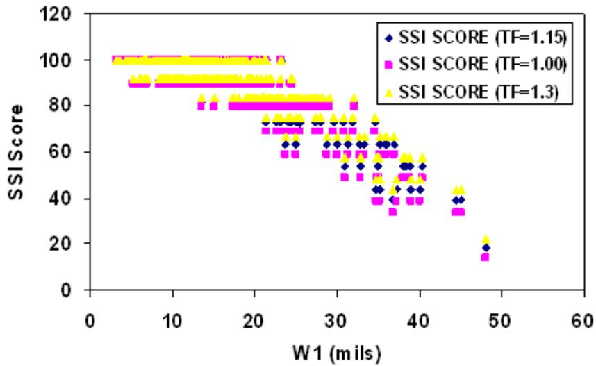
FIGURE 23 SSI Score Compared to W1 for Pavement Type 4
