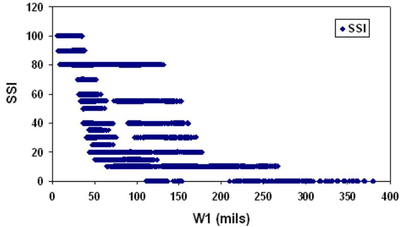
**FIGURE 31 SSI Compared with W1 for Pavement Type 10**
