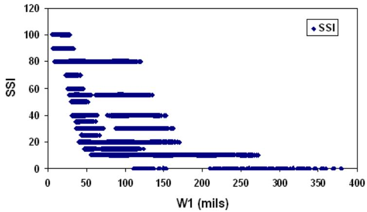
**FIGURE 30 SSI Compared with W1 for Pavement Type 6**
