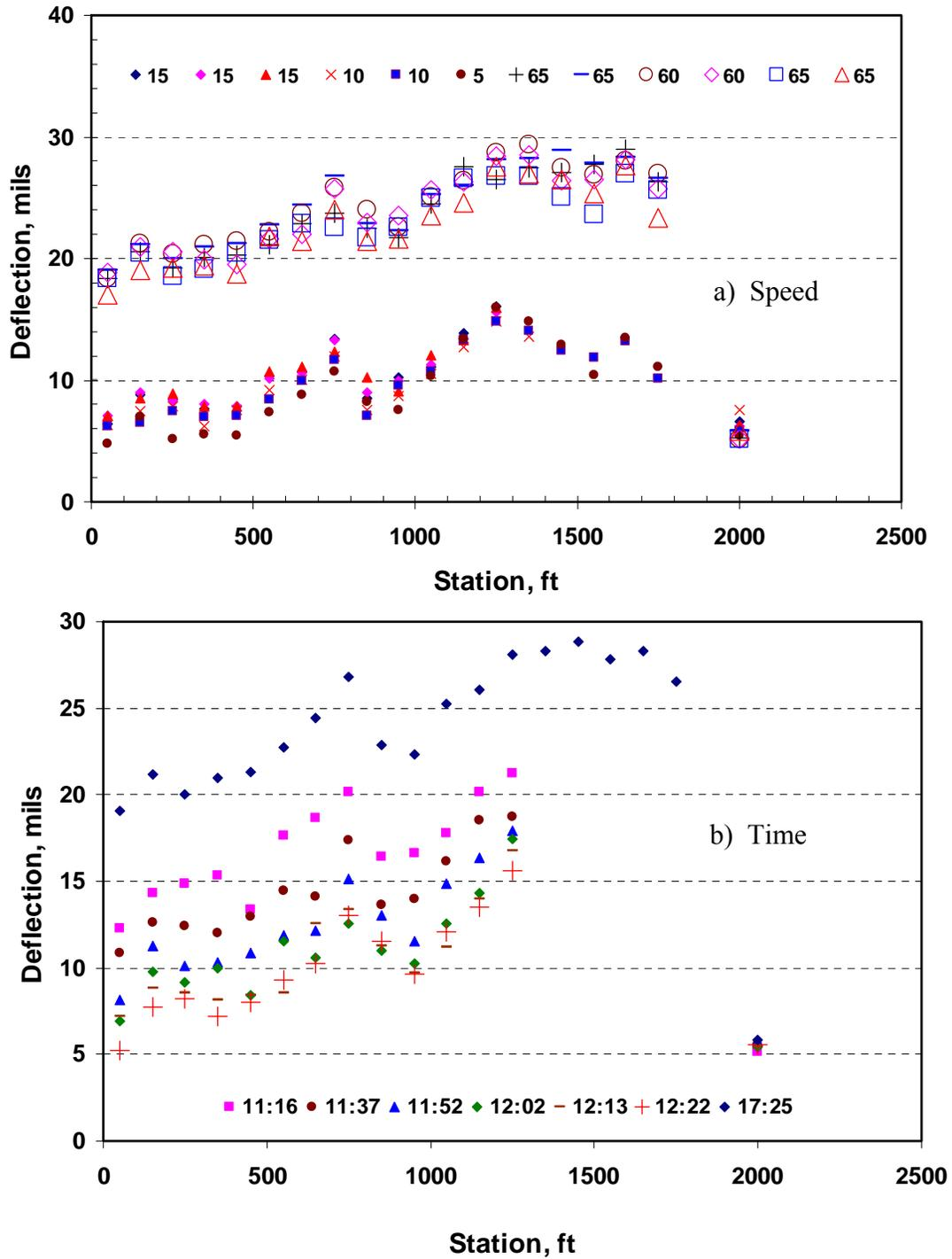
FIGURE 14 RWD and MDD Deflections from SH47 at Section R5
