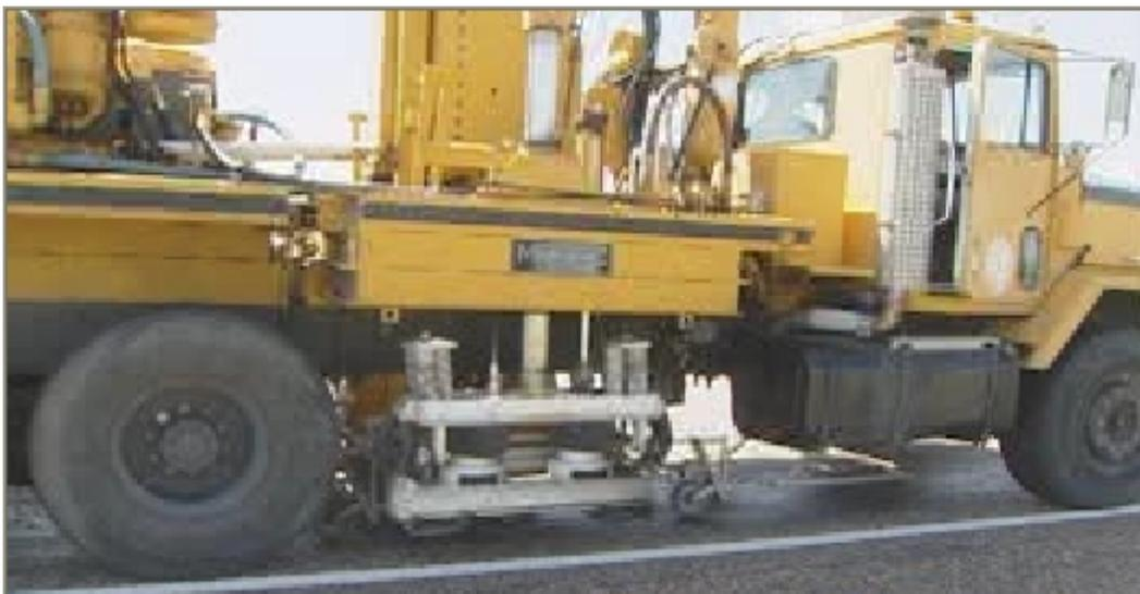
**FIGURE 3 Rolling Dynamic Deflectometer**
