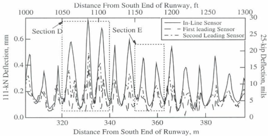
**FIGURE C.6 Transverse Deflection Profile Using All Three Sensors (Bay et. al. 2000)**
