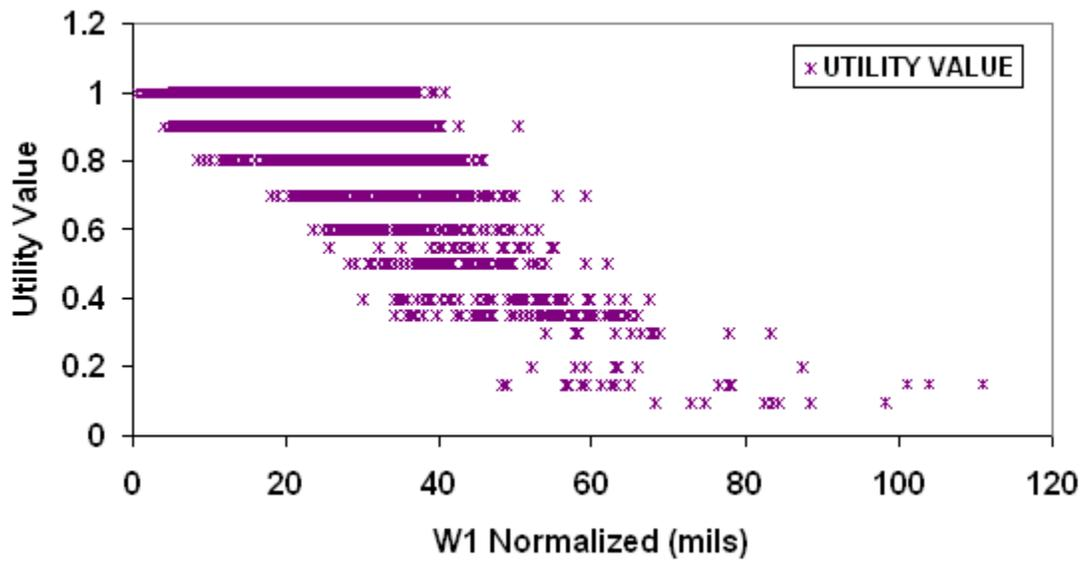
FIGURE 17 Utility Value Compared with the Center Deflection
