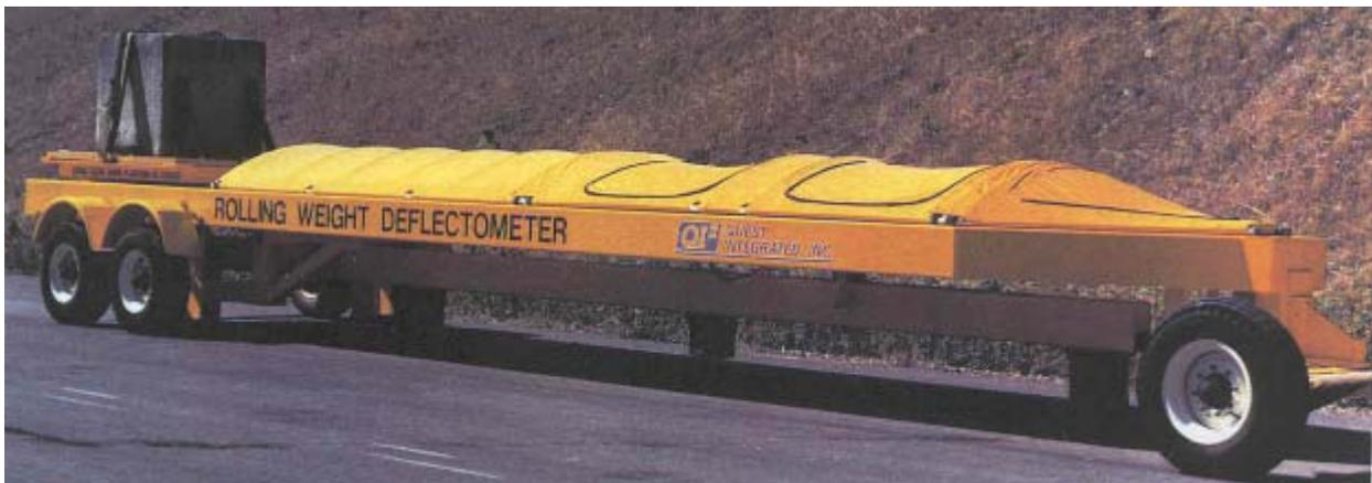
FIGURE 1 ARWD Prototype by Quest Integrated
