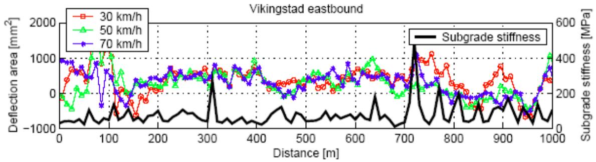
**FIGURE B.9 Relation Between Subgrade Stiffness and Deflection Area for Site 1 (Andr´en and Lenngren, 2004)**
