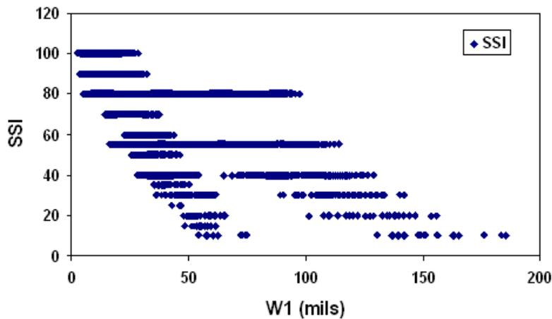
**FIGURE 28 SSI Compared with W1 for Pavement Type 4**
