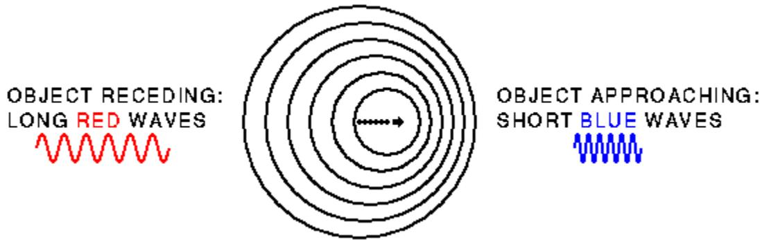
**FIGURE D. 2 Doppler Principle (Hildebrand, et. al. 2002)**
