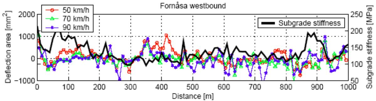
**FIGURE B.10 Relation Between Subgrade Stiffness and Deflection Area for Site 2 (Andr´en and Lenngren, 2004)**
