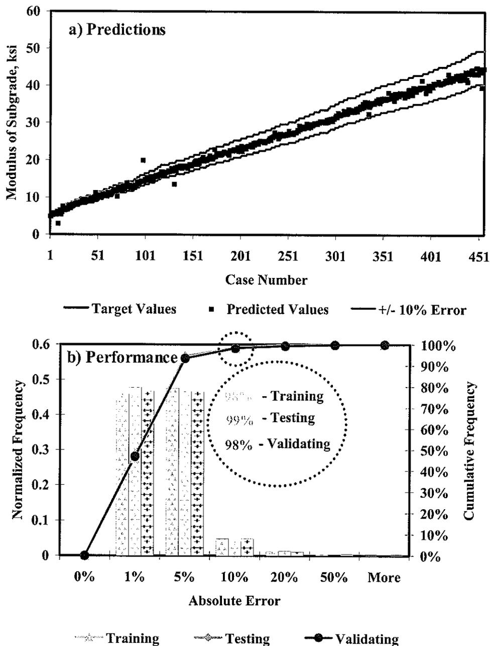
**Figure 4.4 - Quality of ANN Models Developed for Predicting Modulus of Subgrade Layer (Including Thickness of Subgrade in Input)**
