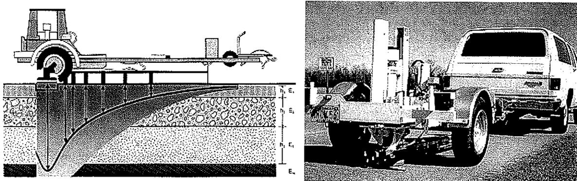
Figure 2.1 - Schematic of Falling Weight Deflectometer
