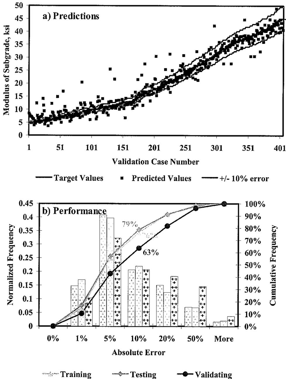
Figure 4.3 - Quality of ANN Models Developed for Predicting Modulus of Subgrade Layer
