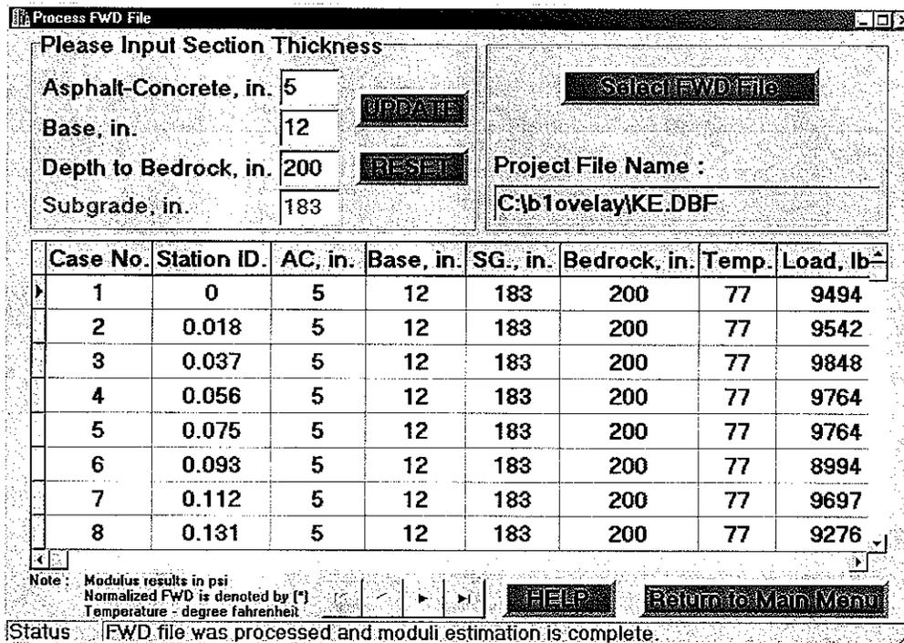
Figure 5.4 - Software Window: Process FWD File
