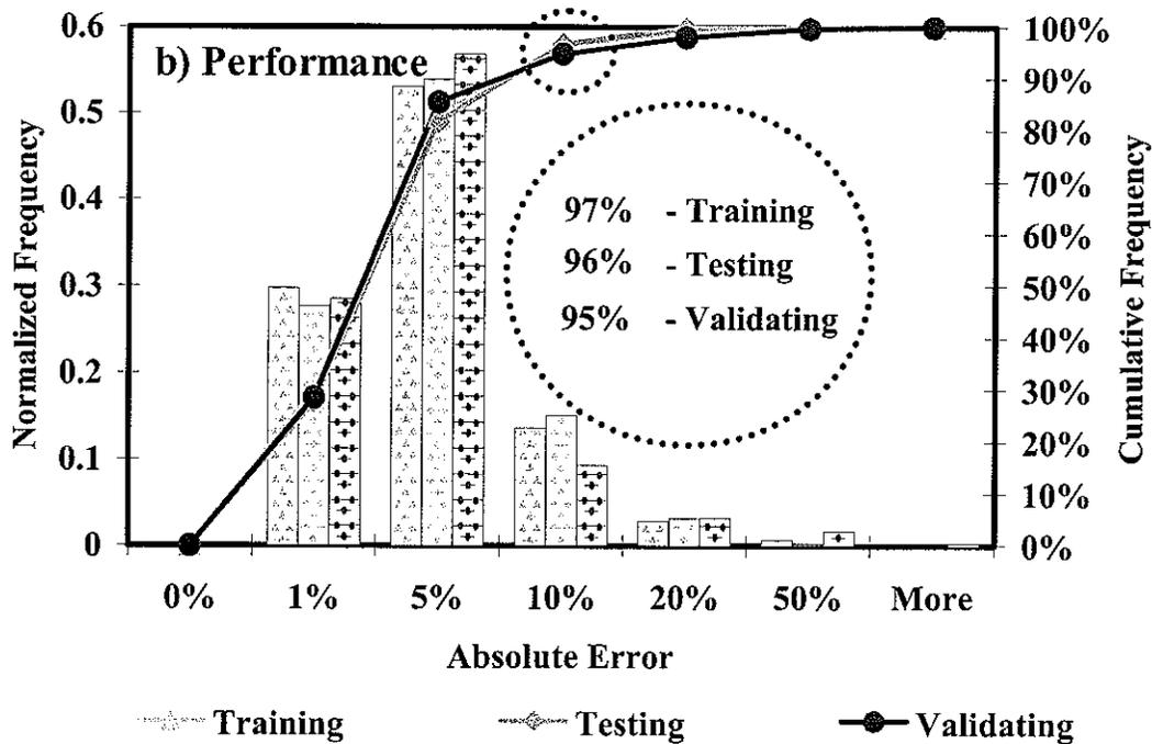
Figure 4.1 - Quality of ANN Models Developed for Predicting Modulus of AC Layer
