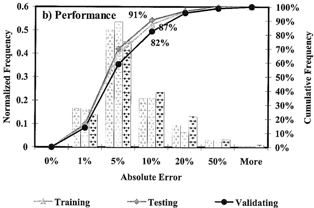
Figure 4.2 - Quality of ANN Models Developed for Predicting Modulus of Base Layer
