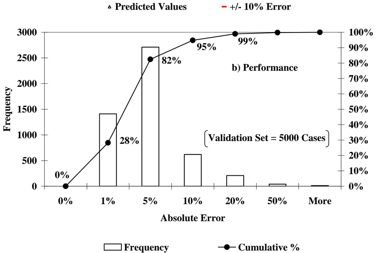
**FIGURE A.4 - ANN Model's Prediction and Performance Based on the Validation Data for the AC Modulus Parameter of a Three-Layer Pavement System with a Thick AC-Layer**
