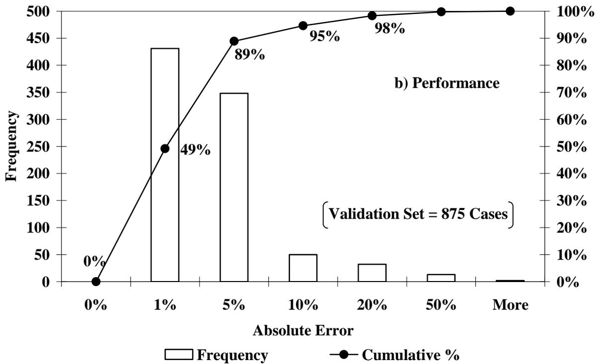
**FIGURE A.1 - ANN Model's Prediction and Performance Based on the Validation Data for the Tensile Strain Parameter of a Three-Layer Pavement System with a Thick AC-Layer**
