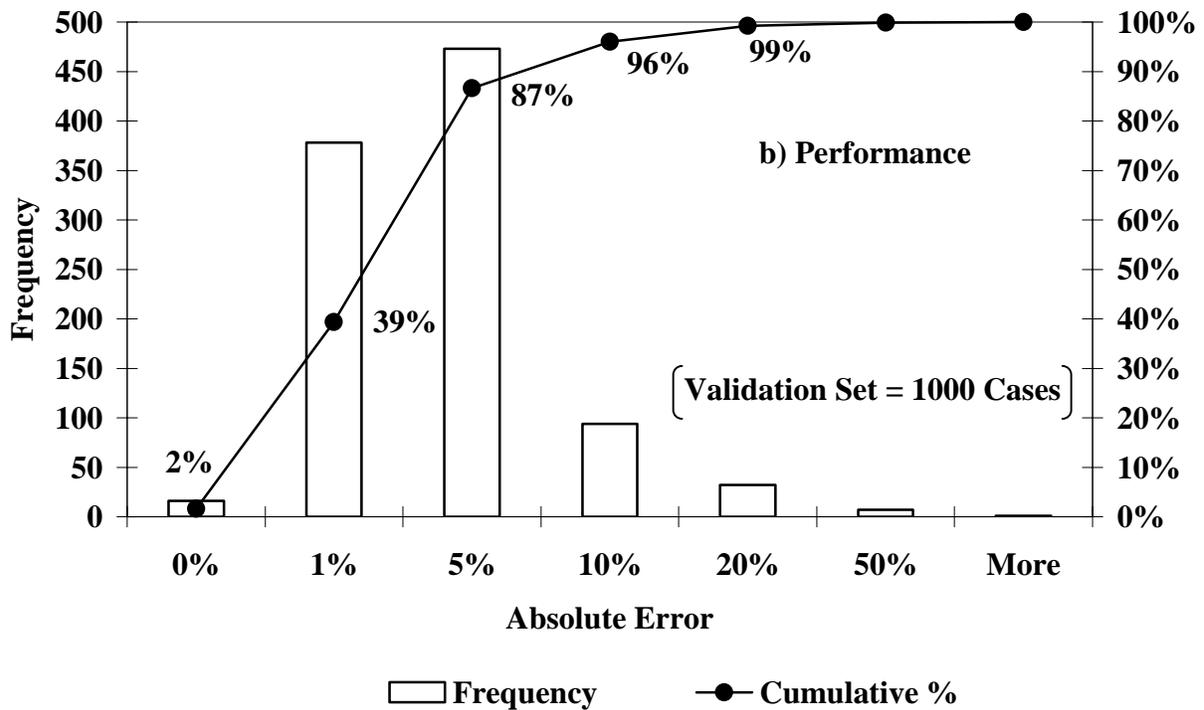
**FIGURE 3.4 - ANN Model's Prediction and Performance Based on the Validation Data for the Thickness of the Subgrade for a Three-Layer Pavement System**
