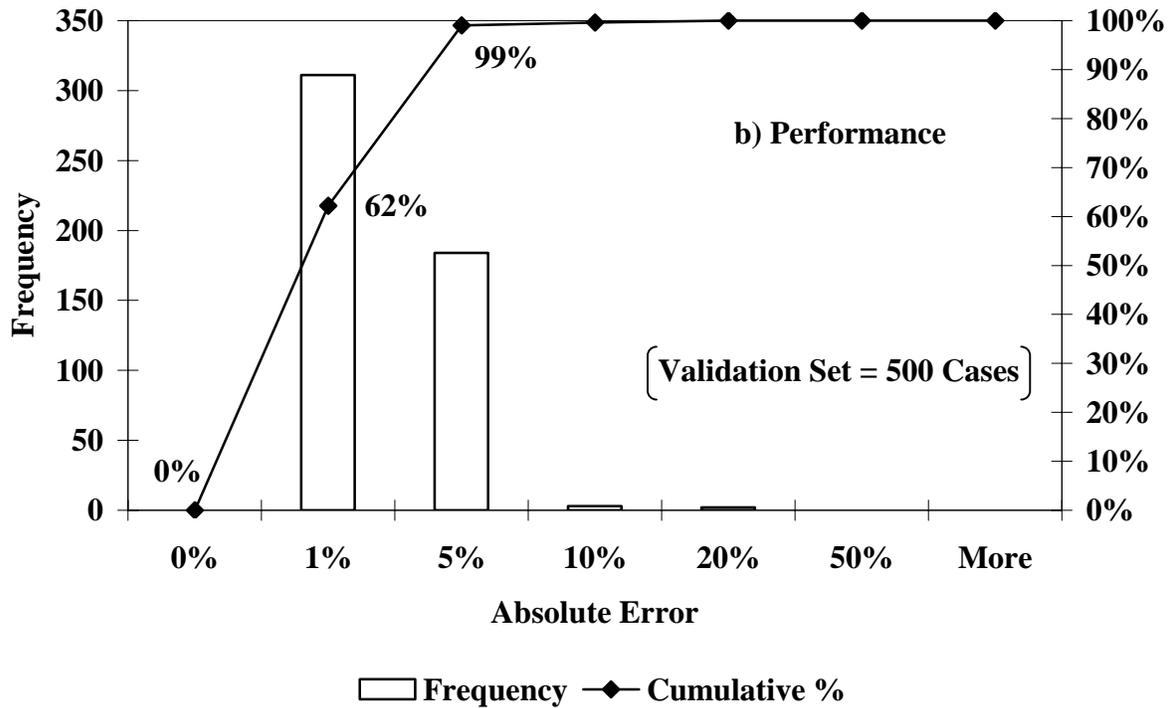
**FIGURE A.8 - ANN Model's Prediction and Performance Based on the Validation Data for the Compressive Strain Parameter of a Four-Layer Pavement System with a Thick AC-Layer**
