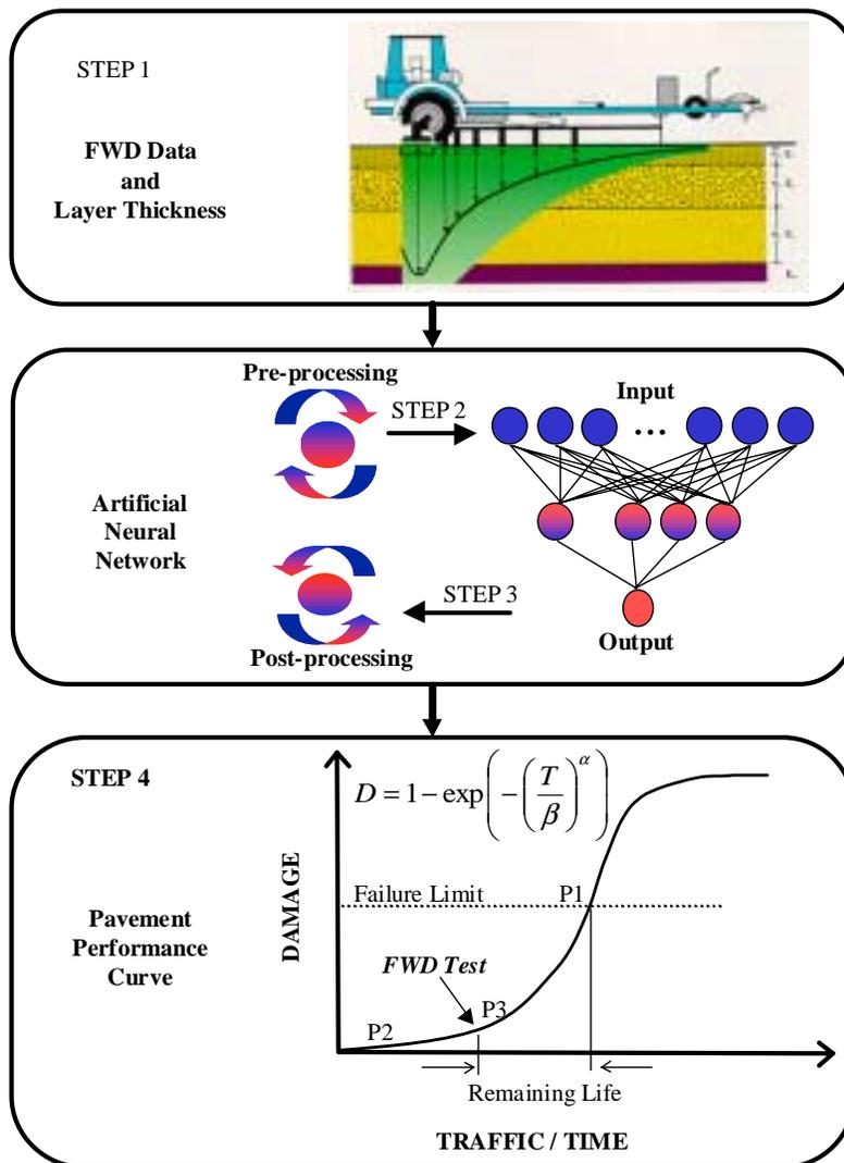
**FIGURE 2.4 - Summary of Methodology Used to Describe Service Life of a Pavement**
