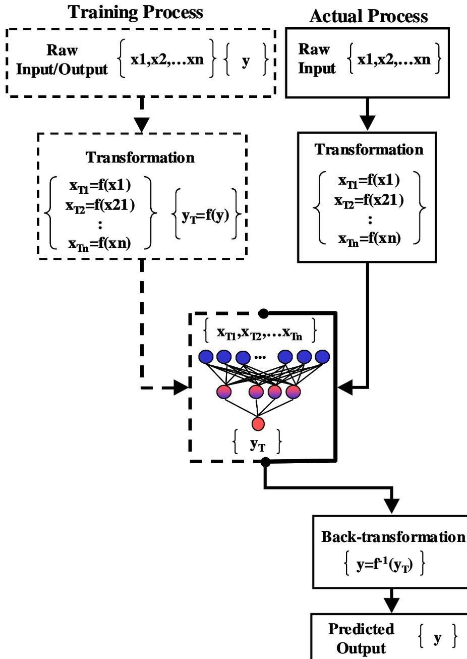
FIGURE 3.2 - Flow of Variable Transformation Process for Determining Inputs and Outputs to ANN Models
