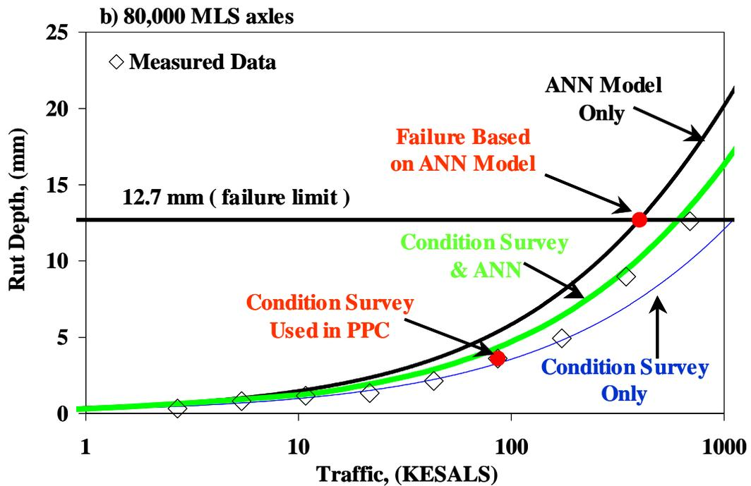
FIGURE 2.8 - Comparison of Actual Rutting Performance Curves with Calculated Ones at 20,000 and 80,000 Repetitions Using Several Strategies
