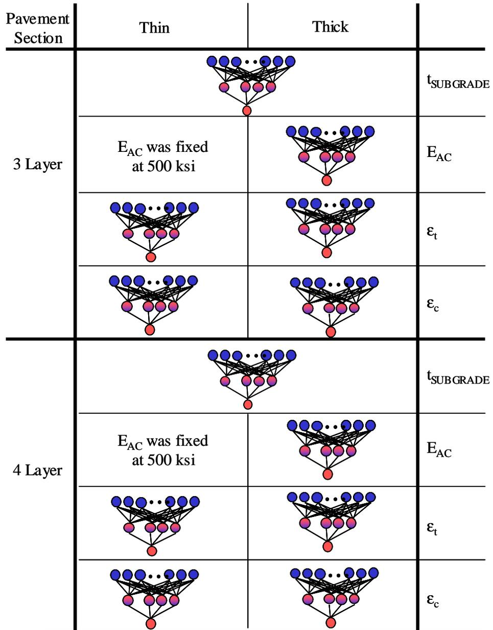
**FIGURE 3.1 - System of Artificial Neural Network Models for Three- and Four-Layer Flexible Pavements**
