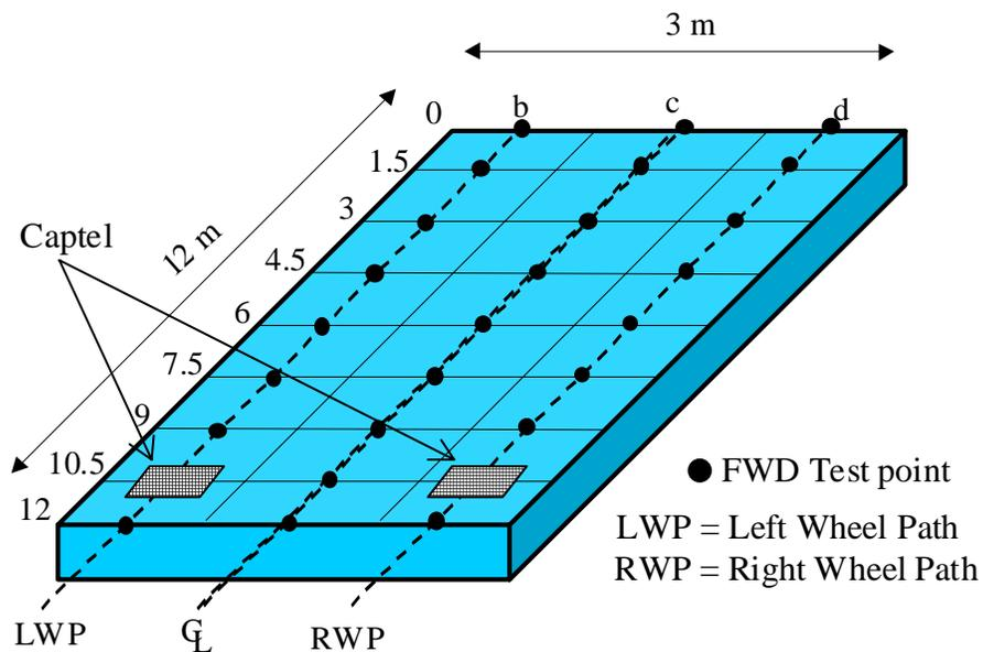
**FIGURE 2.3 - Schematic of Testing Area with TxMLS**
