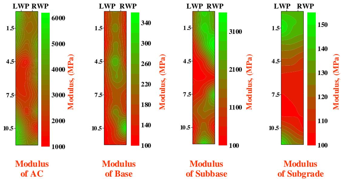
FIGURE 2.10 - Variations in Backcalculated Moduli with Location within the Test Pad
