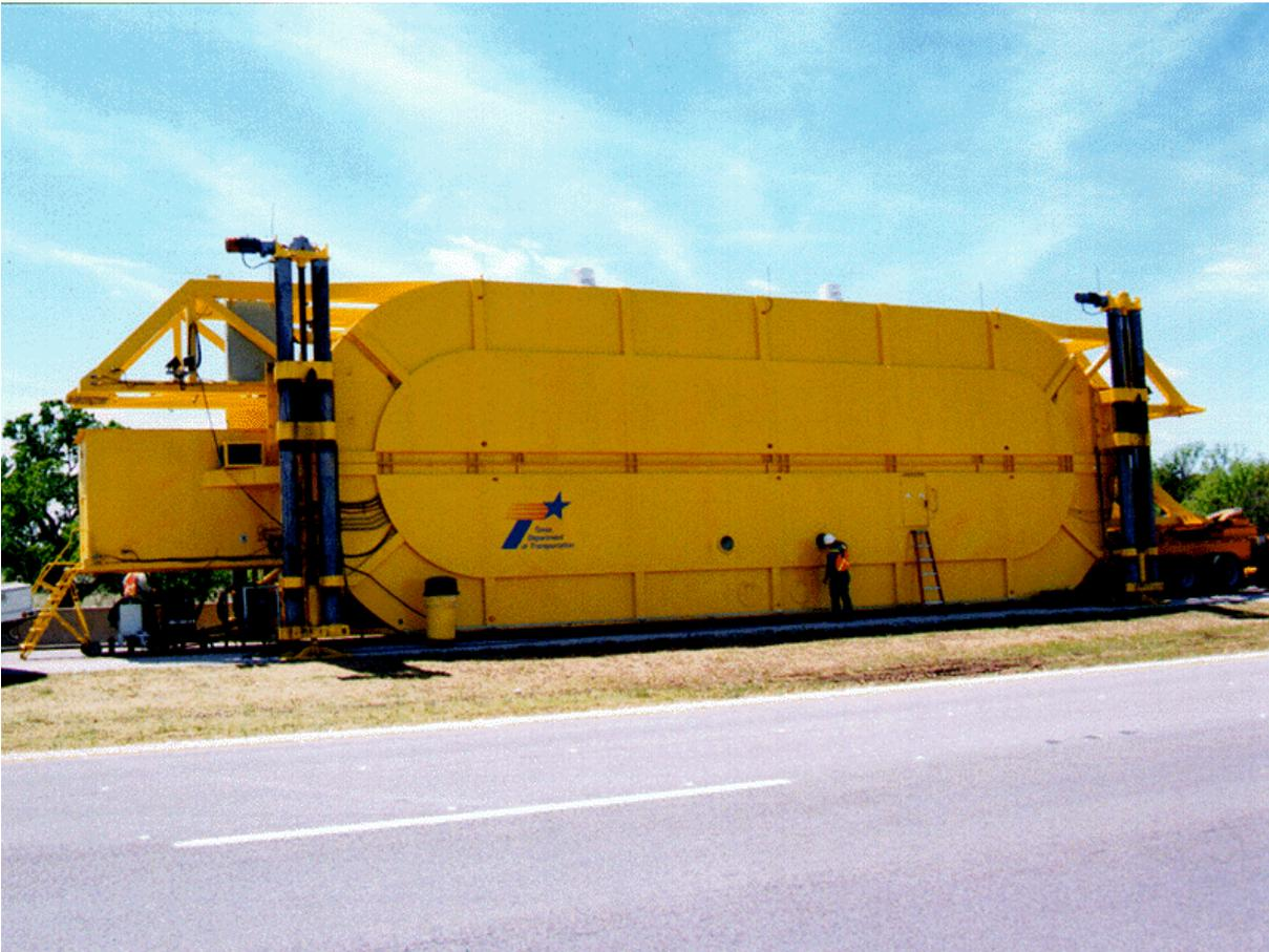
**FIGURE 2.2 - Texas Mobile Load Simulator**
