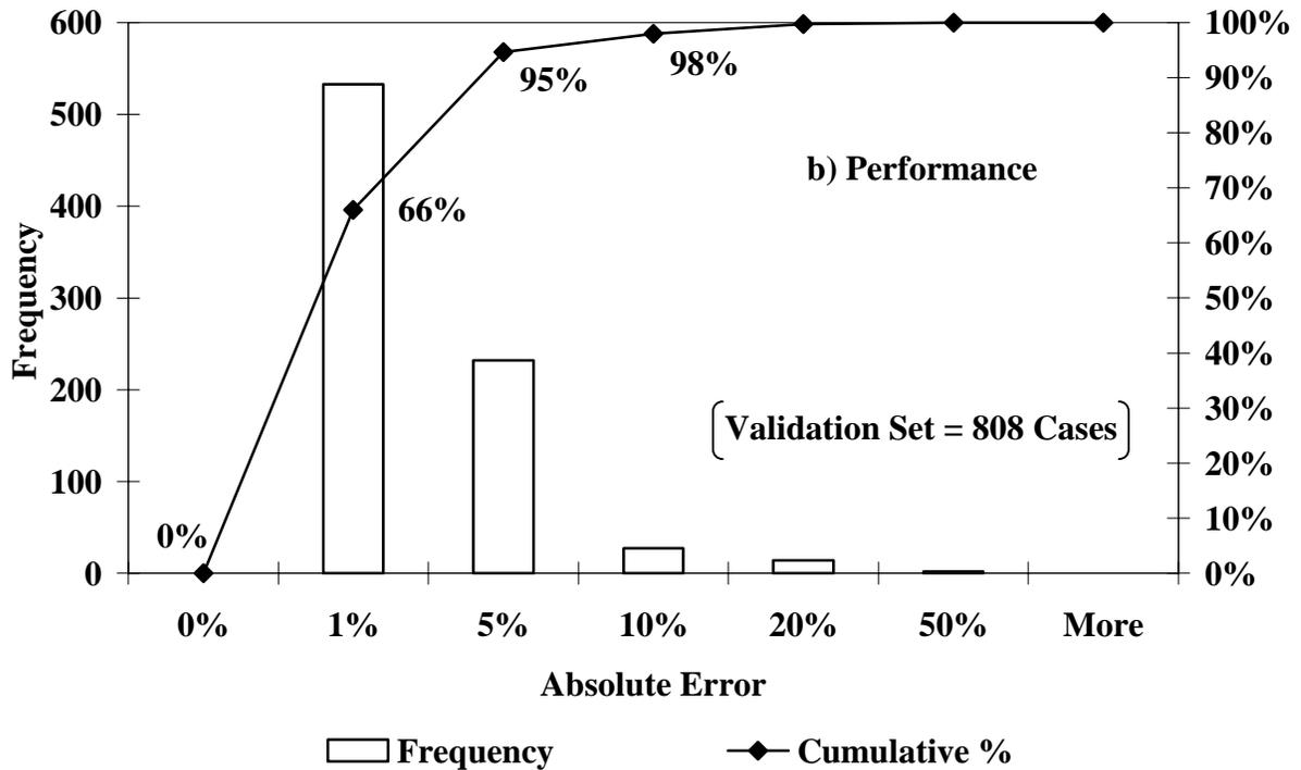
**FIGURE A.7 - ANN Model's Prediction and Performance Based on the Validation Data for the Compressive Strain Parameter of a Four-Layer Pavement System with a Thin AC-Layer**
