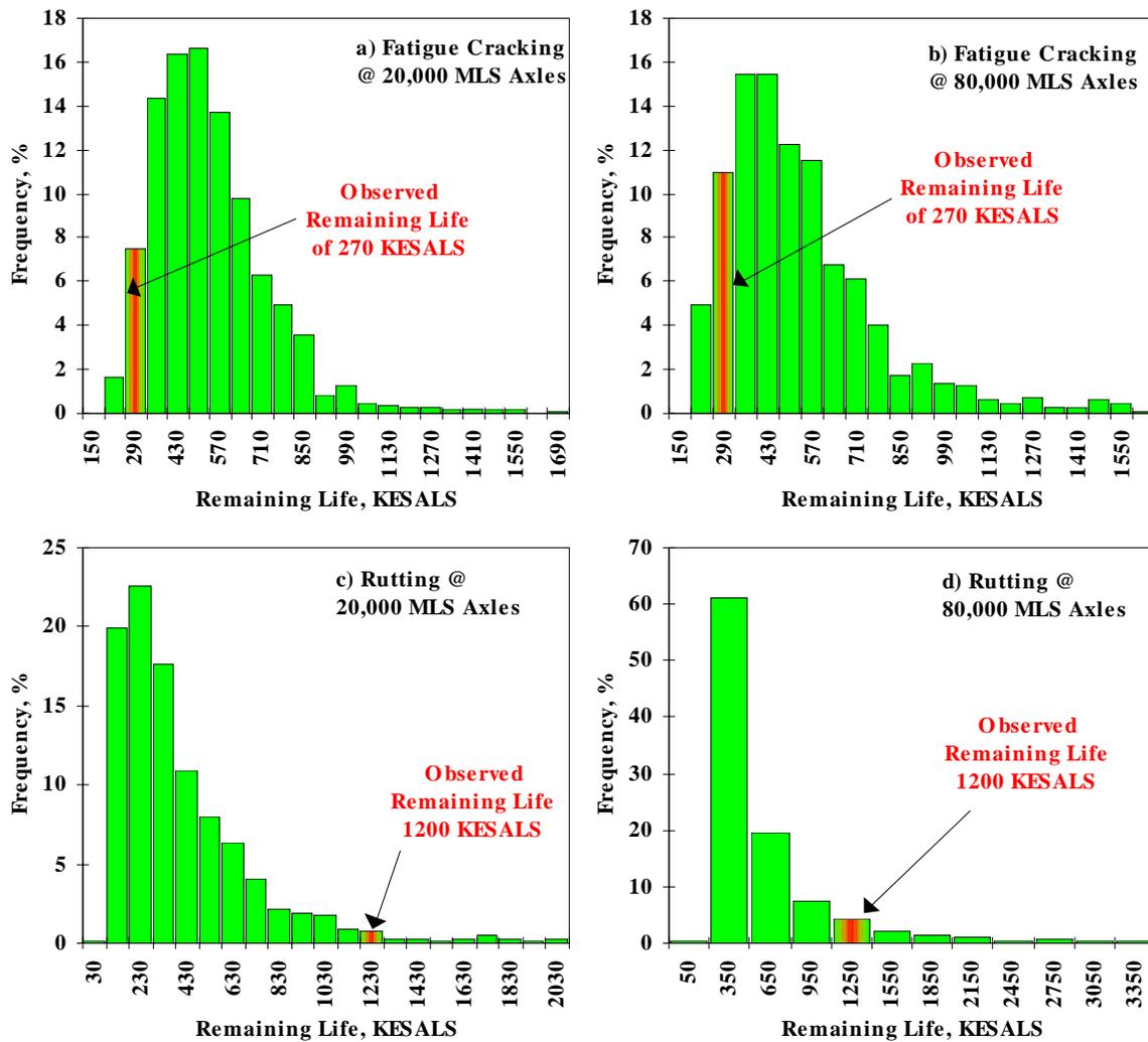
**FIGURE 2.11 - Simulated Distribution of Remaining Life Based on ANN Models vs. Observed Remaining Life of Entire Test Slab**
