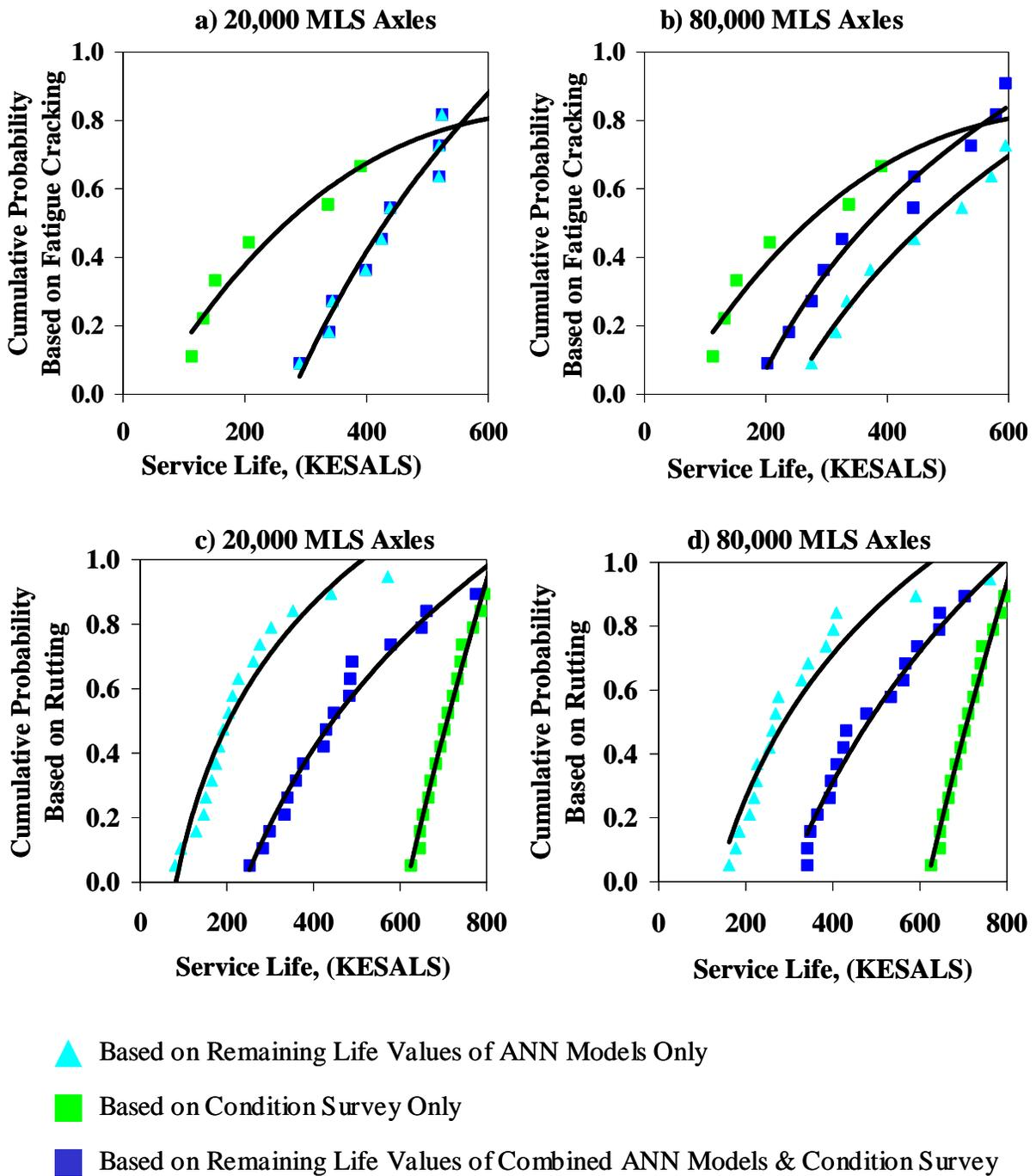
**FIGURE 2.12 - Comparison of the Pavements Service Life Based on Observed Data, Results of ANN Models, and PPC**
