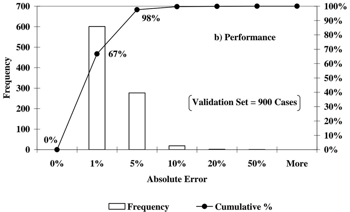
**FIGURE A.3 - ANN Model's Prediction and Performance Based on the Validation Data for the Compressive Strain Parameter of a Three-Layer Pavement System with a Thick AC-Layer**
