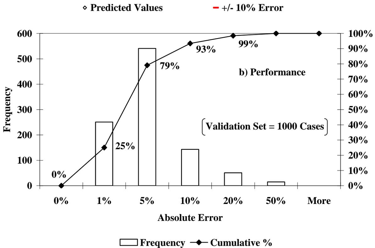
**FIGURE A.9 - ANN Model's Prediction and Performance Based on the Validation Data for the AC Modulus Parameter of a Four-Layer Pavement System with a Thick AC-Layer**
