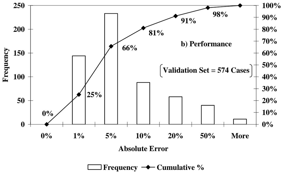
**FIGURE A.6 - ANN Model's Prediction and Performance Based on the Validation Data for the Tensile Strain Parameter of a Four-Layer Pavement System with a Thick AC-Layer**
