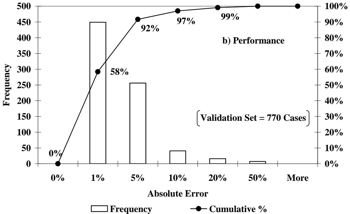
**FIGURE 3.3 - ANN Model's Prediction and Performance Based on the Validation Data for the Tensile Strain Parameter of a Three-Layer Pavement System with a Thin AC-Layer**
