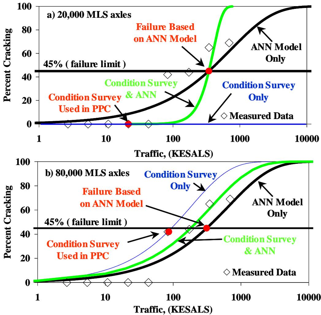
**FIGURE 2.7 - Comparison of Actual Fatigue Cracking Performance Curves with Calculated Ones Using Several Strategies**
