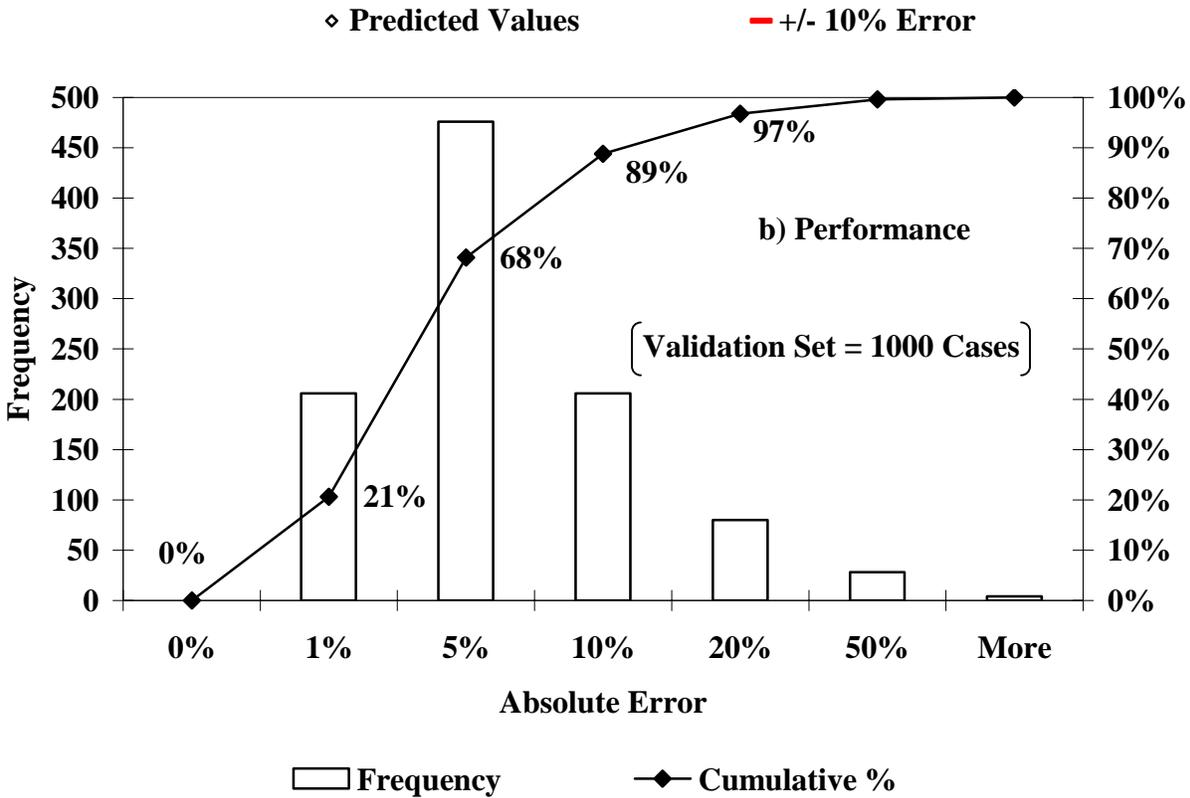
**FIGURE A.10 - ANN Model's Prediction and Performance Based on the Validation Data for the Thickness of the Subgrade for a Four-Layer Pavement System**
