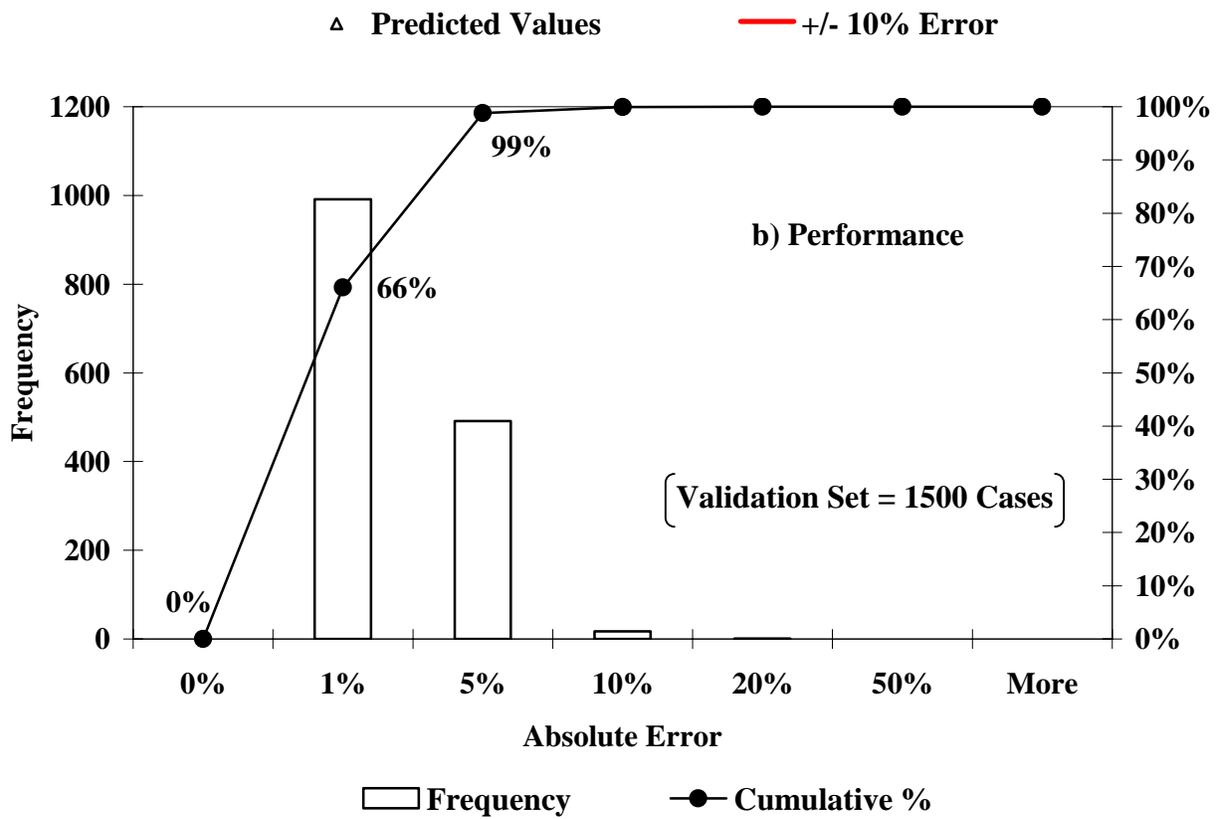
**FIGURE A.2 - ANN Model's Prediction and Performance Based on the Validation Data for the Compressive Strain Parameter of a Three-Layer Pavement System with a Thin AC-Layer**
