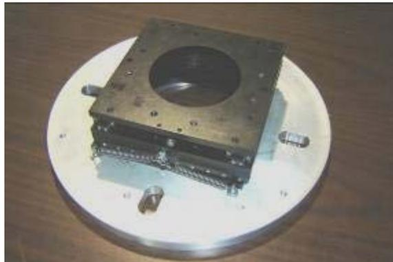
This pole interface plate serves an additional, important function—which is to house features to prevent slide over travel. These may be implemented as hard rubber pegs or rubber-coated posts, providing a positive stop for the slide at each end; one such stop is shown in orange in the next picture. In optimized implementations, the stopping mechanisms may incorporate springs or dampers to absorb impact energy resulting
