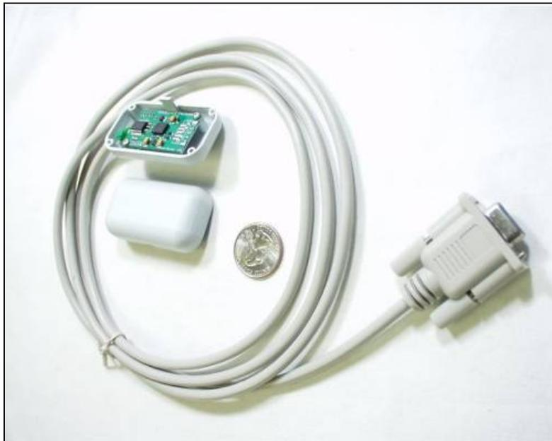
Figure 4.15 Tri-Axis serial accelerometer.
