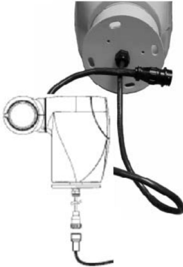
Figure 4.10 Pigtail connector for typical CCTV cameras.
