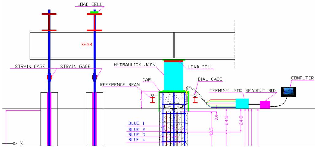
**Fig. 3 Schematic Side View of the Pile Load Test Setup**
