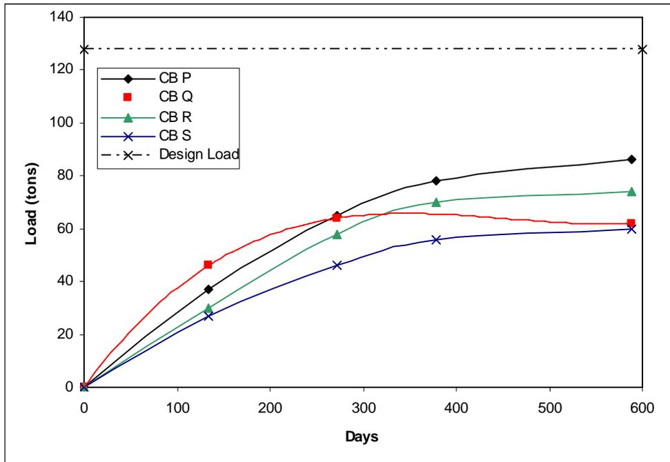
**Fig. 8 Load carried by the CB service piles**
