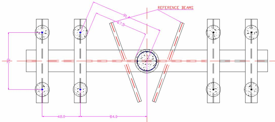
**Fig. 4 Schematic Plan View of the Pile Load Test Setup**
