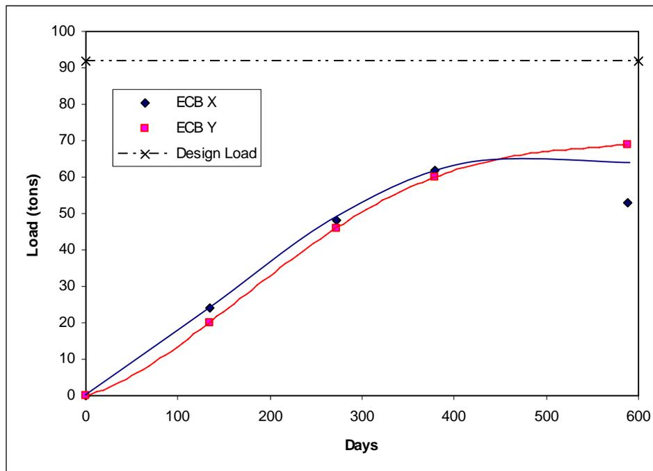
**Fig. 7 Loads carried by the ECB Service Piles**
