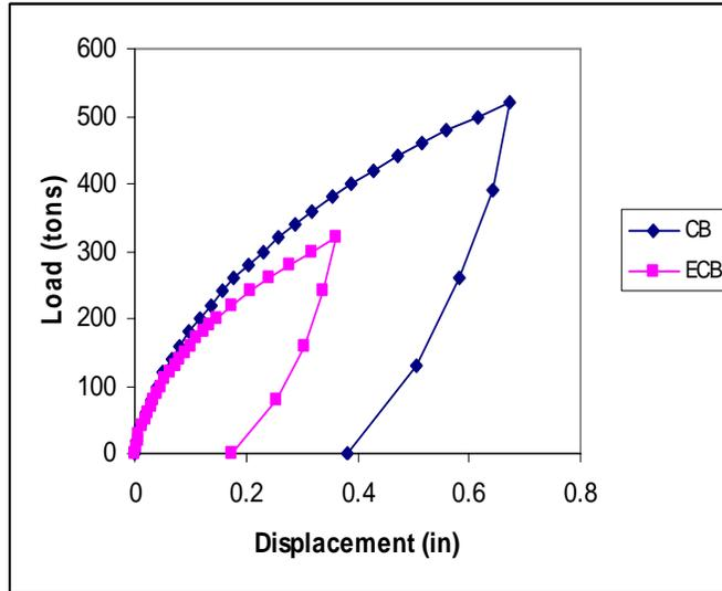
**Fig. 5 Load-Displacement Behavior of the ACIP Pile at both sites**
