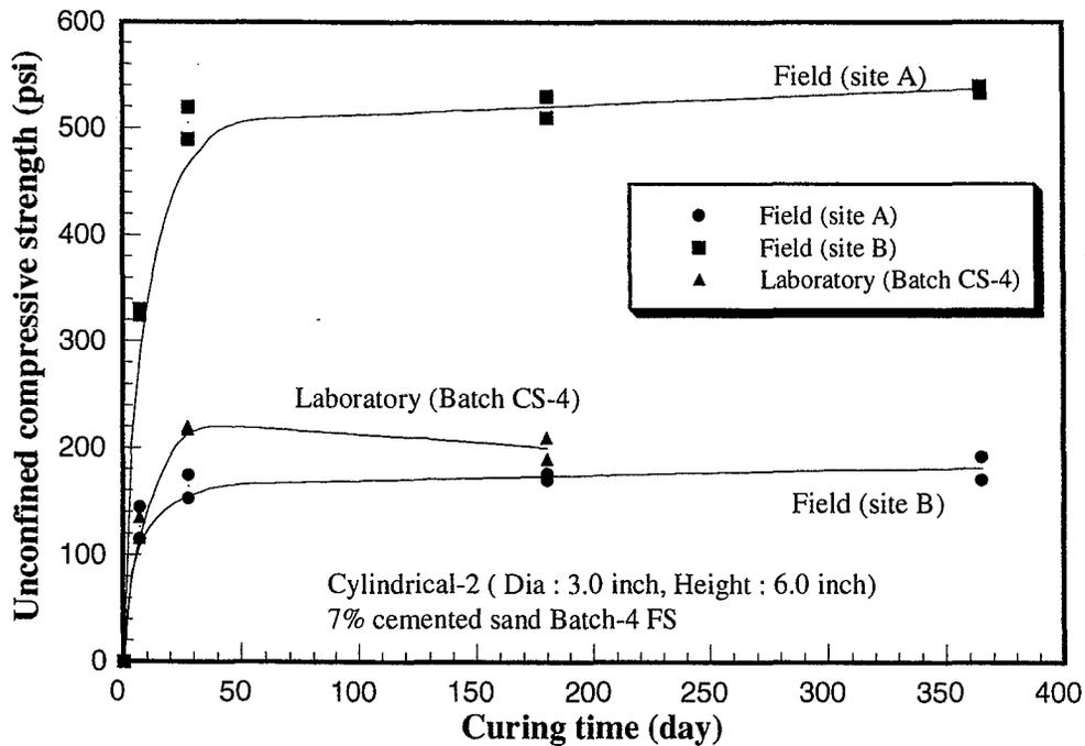
Figure 5.29 Comparison of the unconfined compressive strength with laboratory and field data (cylindrical-2 specimen)
