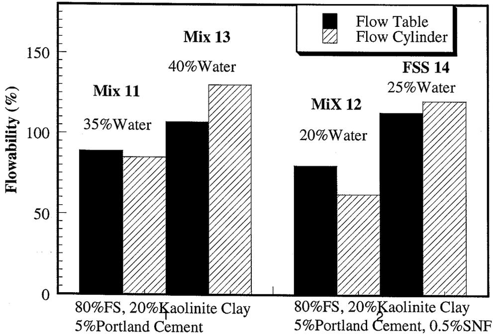
Figure 4.29 The flowability of FS-cement-kaolinite flowable fill with and without superplasticizer (SNF)
