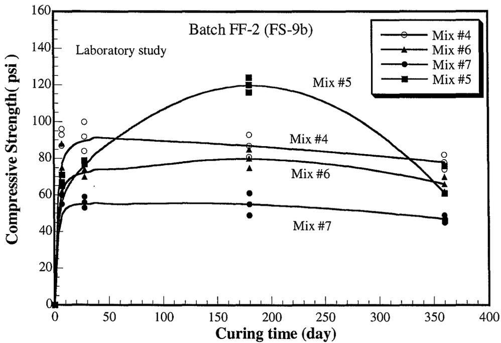
Figure 4.22 Variation of compressive strength with curing time for Batch FF-2
