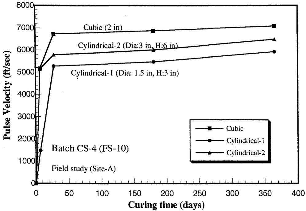
**Figure 5.18** Variation of pulse velocity with curing time
