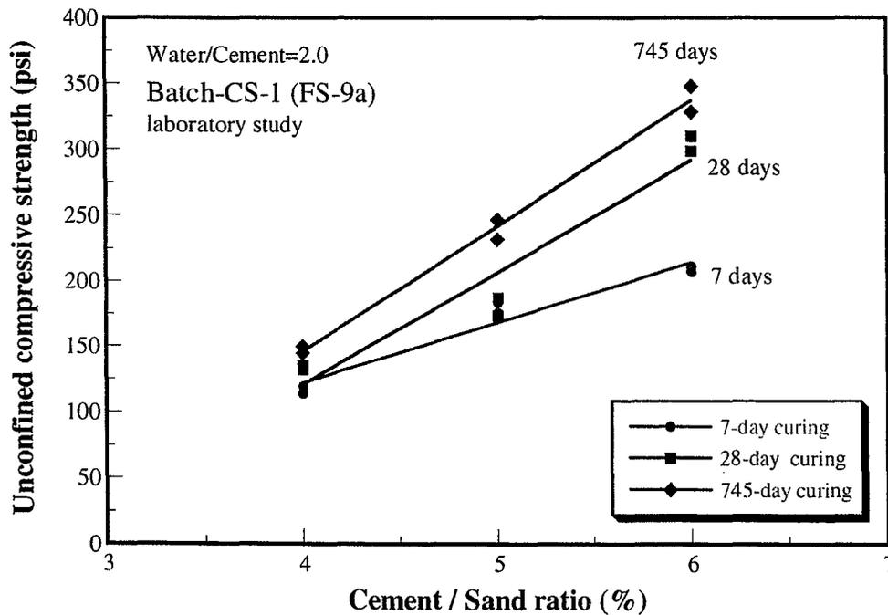
Figure 5.5 Variation of unconfined compressive strength with curing time (Batch CS-1, laboratory study)
