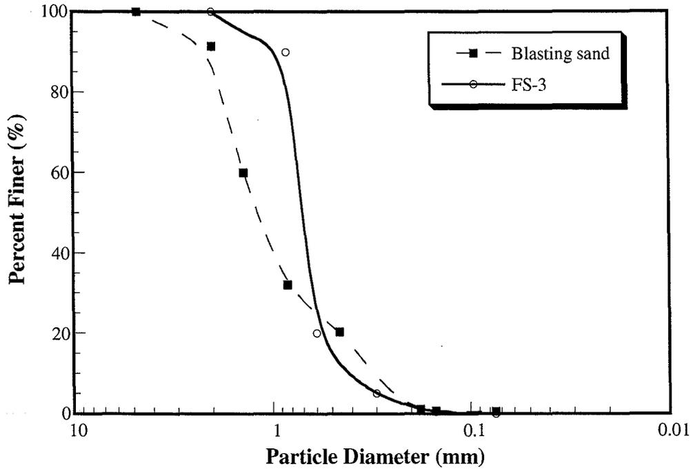
Figure 4.27 The particle size distribution of blasting sand and FS-3
