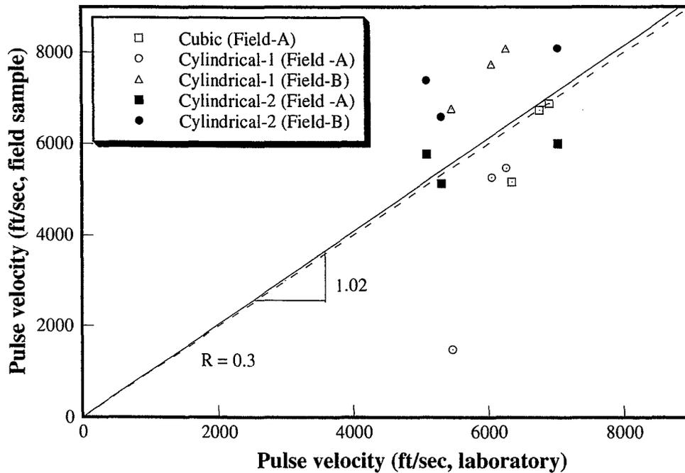
Figure 5.25 Comparison of the pulse velocity with laboratory and field samples
