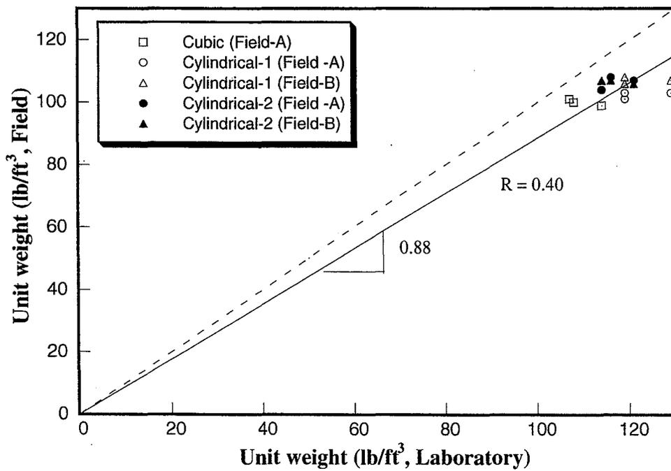
Figure 5.23 Comparison of the unit weight with laboratory and field samples
