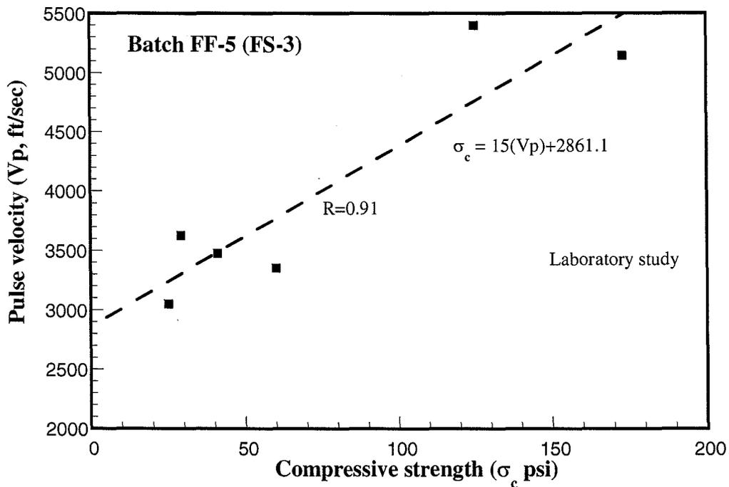
Figure 4.37 Relationship between compressive strength and pulse velocity
