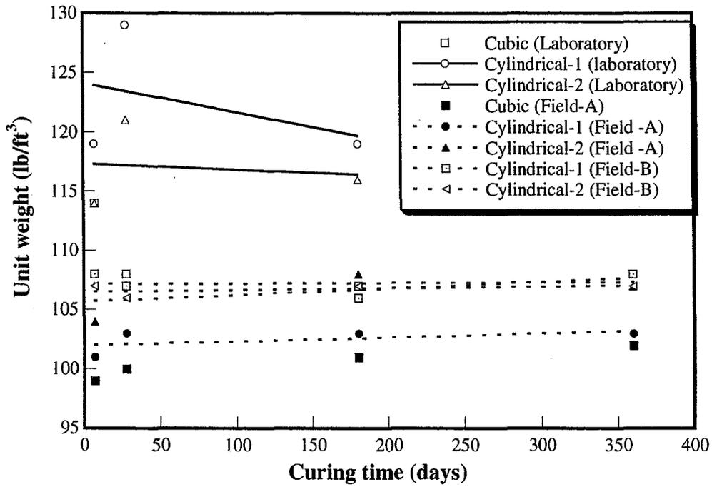
Figure 5.22 Comparison of the unit weight with laboratory and field samples
