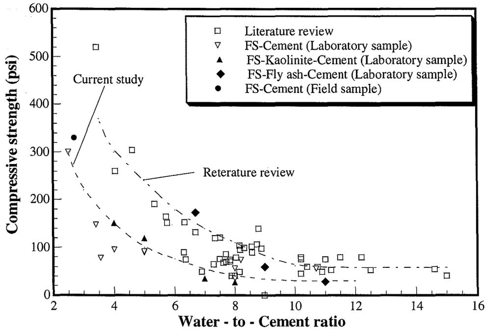
Figure 4.52 Strength versus water-to-cement ratio for FS mixes
