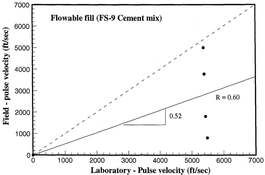
**Figure 4.47 Comparison of pulse velocity (Laboratory and Field sample)**
