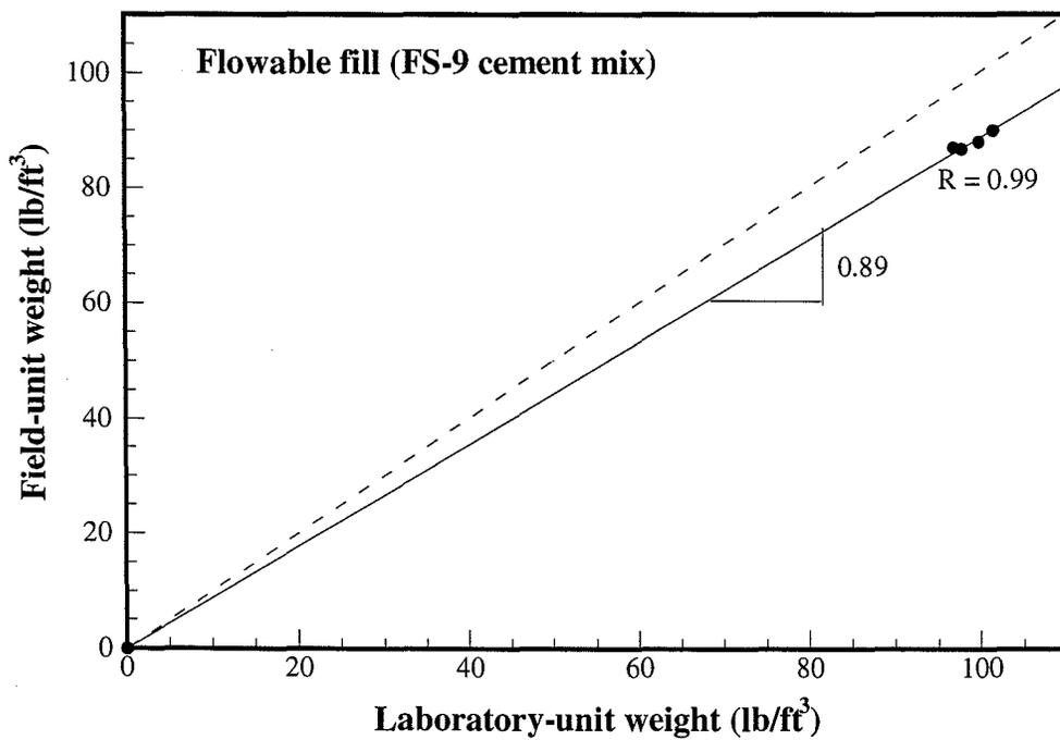
Figure 4.45 Comparison of unit weight (laboratory and field sample)
