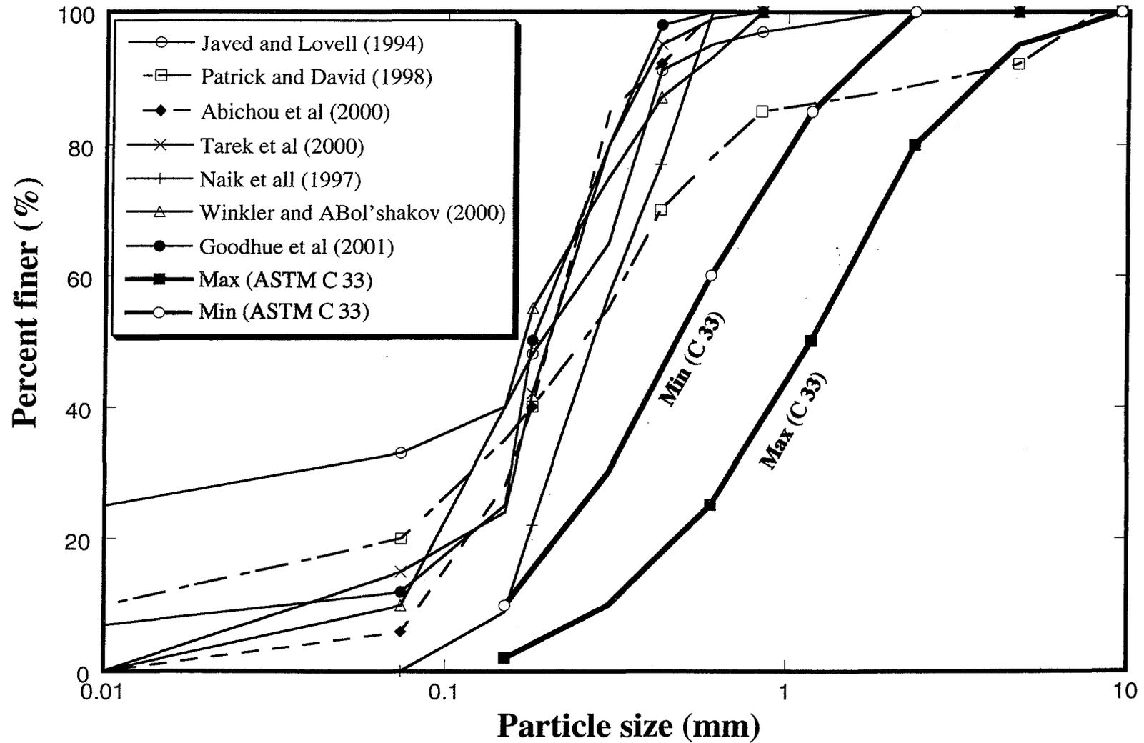
**Figure 2.1** Particle Size Distributions of foundry sands are compared to the ASTM C 33 Sand used for Making Concrete.
