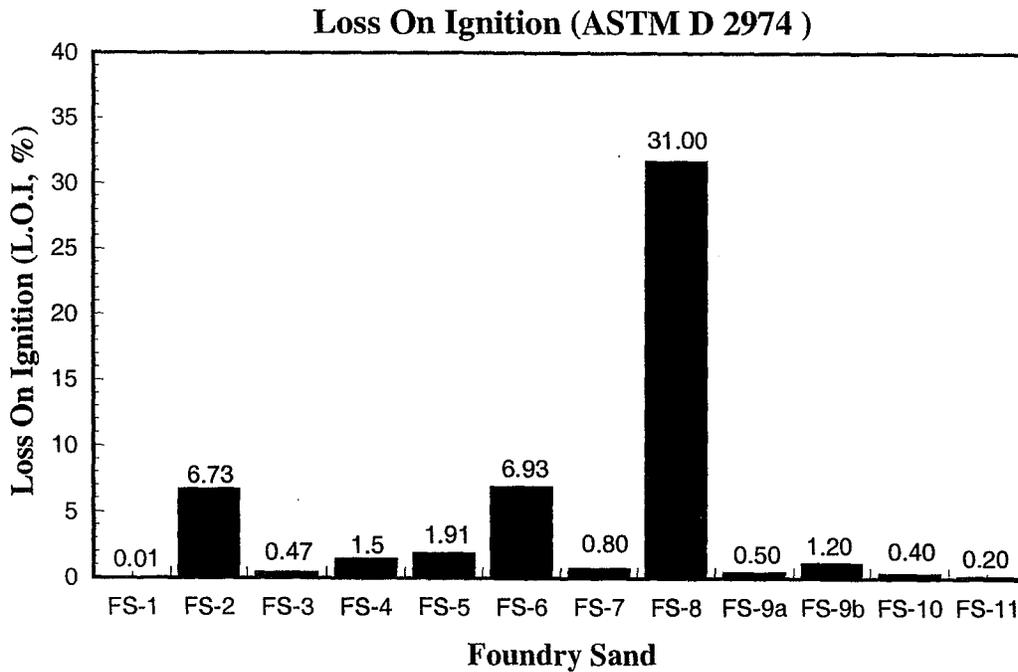
**Figure 3.8. Distribution of Loss on Ignition (LOI) of Texas Foundry Sands Tested During this Study.**
