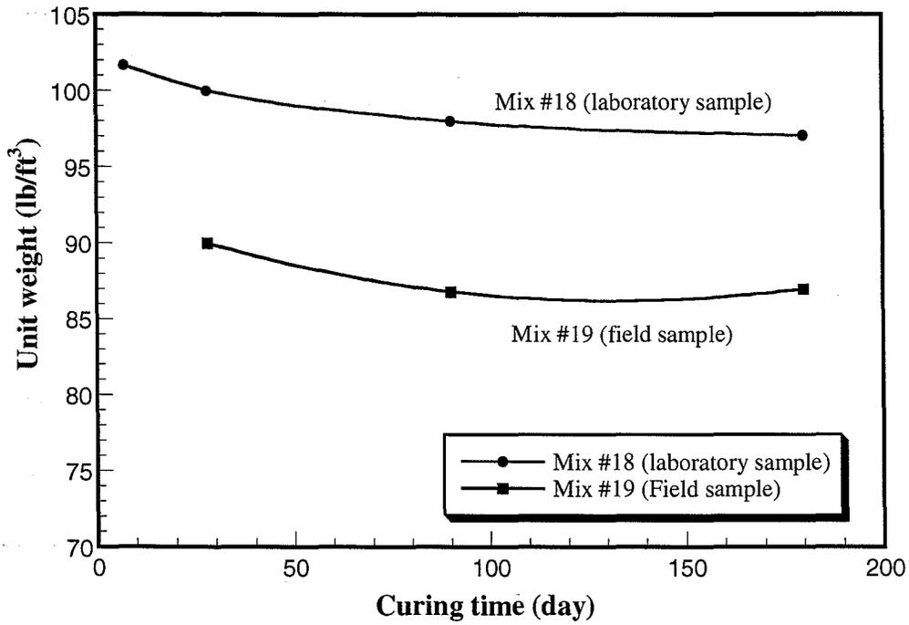
Figure 4.44 Variation of unit weight with curing time (laboratory and field sample)
