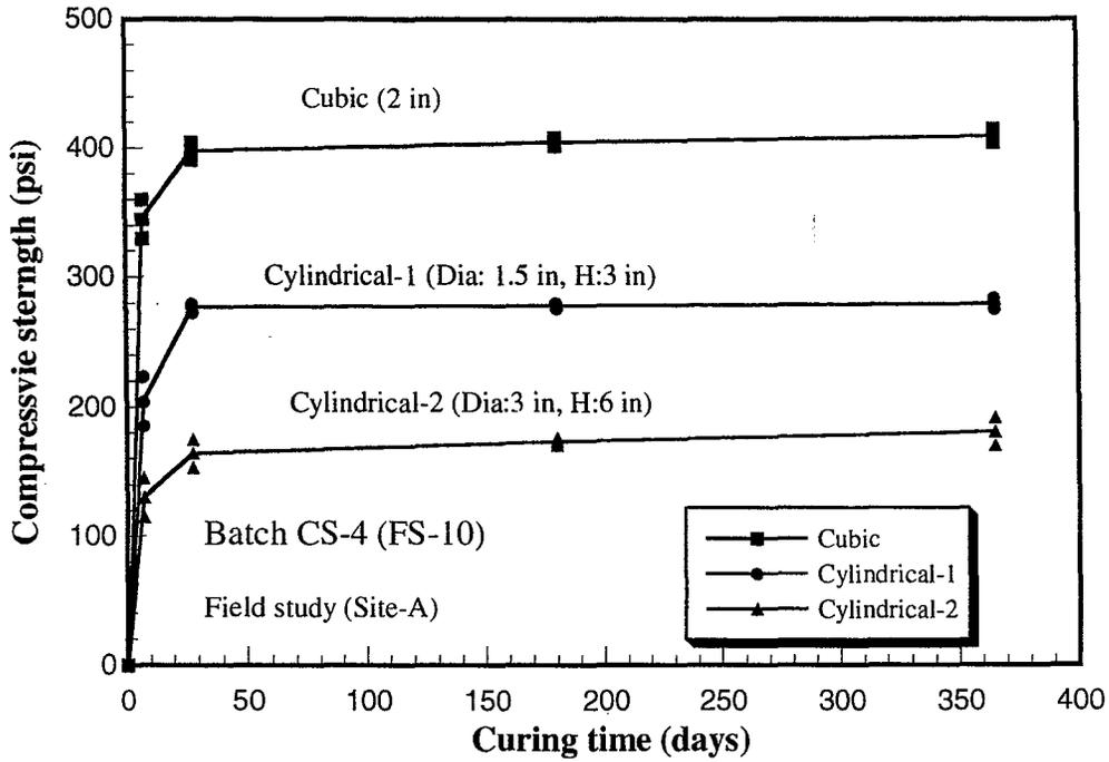
Figure 5.20 Unconfined compressive strength with varying specimen size, shape, and curing time (Batch CS-4. field study, Site-A)
