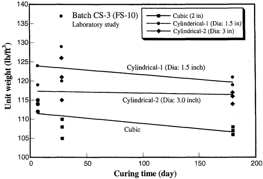
Figure 5.2 Variation of unit weight with curing time (Batch CS-3, laboratory study)
