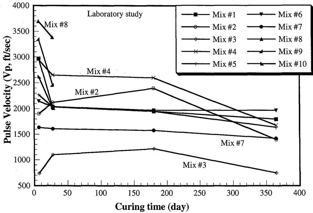
Figure 4.17 Variation of pulse velocity versus curing time for various mixes
