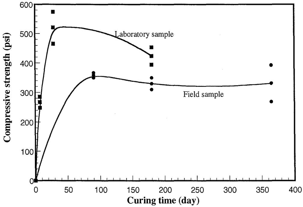
Figure 4.48 Variation of compressive strength with curing time (laboratory and field sample)
