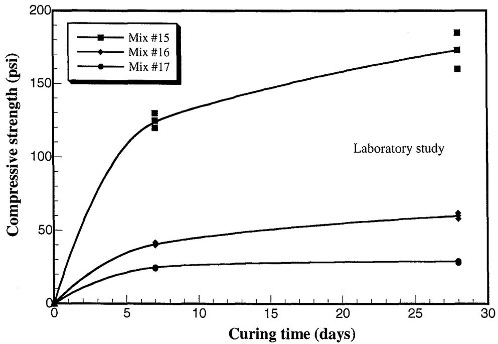
Figure 4.35 Variation of compressive strength with curing time
