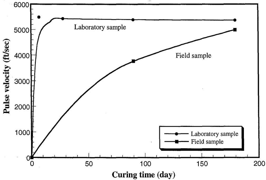
**Figure 4.46 Variation of pulse velocity with curing time (laboratory and field sample)**
