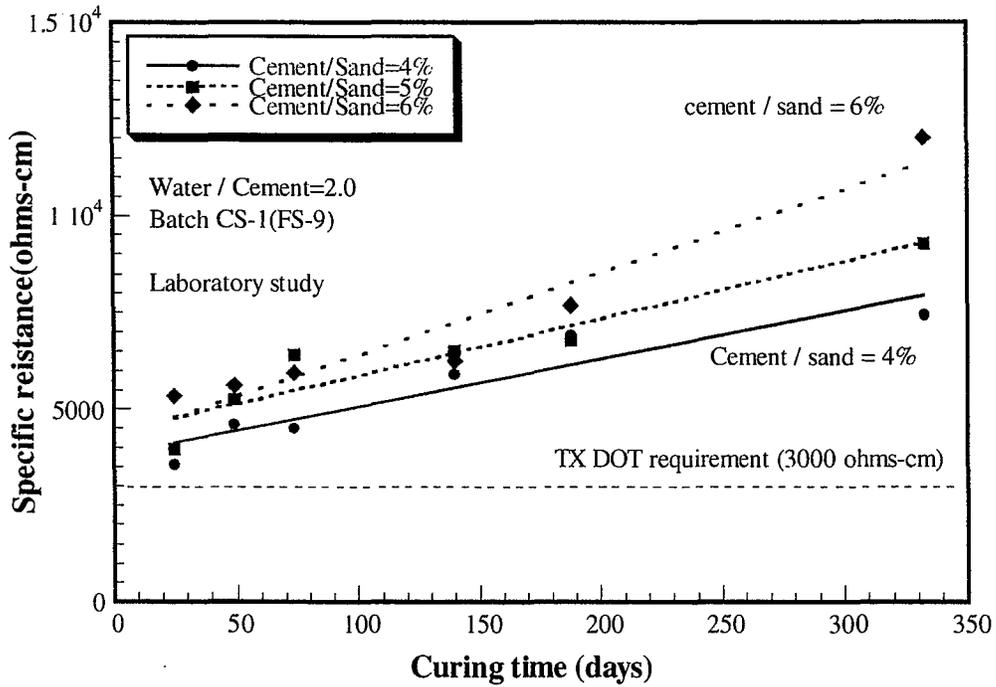
Figure 5.3 Variation of specific electrical resistivity of cemented sand with curing time and cement content (Batch CS-3, laboratory study)
