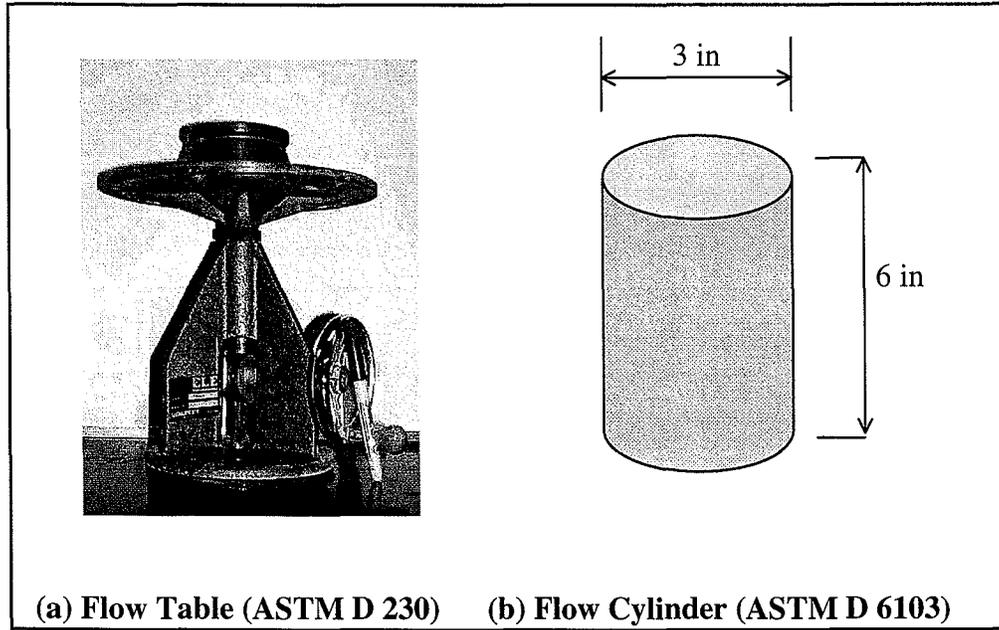
Figure 4.7 Flowability equipments used in this study
