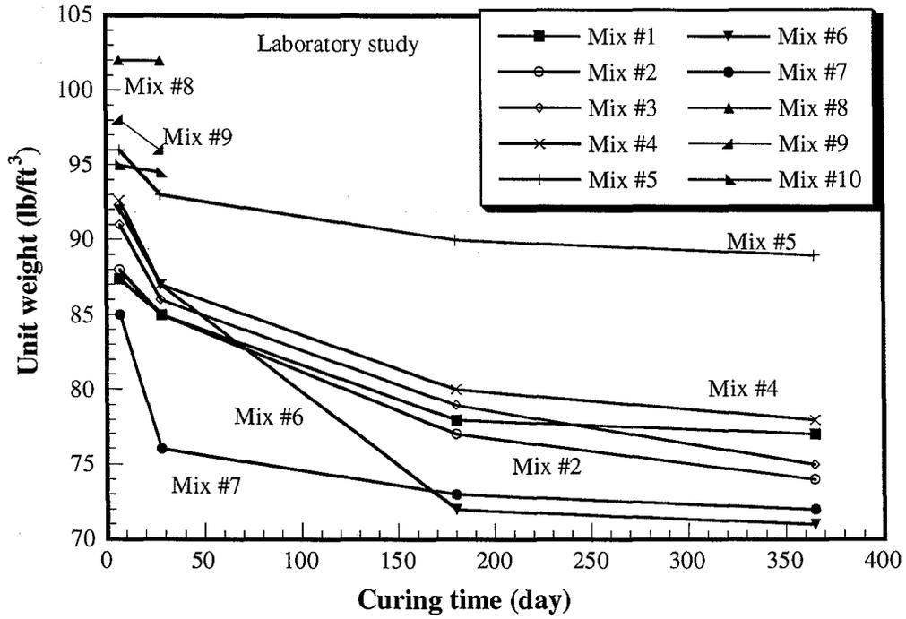
Figure 4.15 Variation of unit weight versus curing time for flowable fill mixtures
