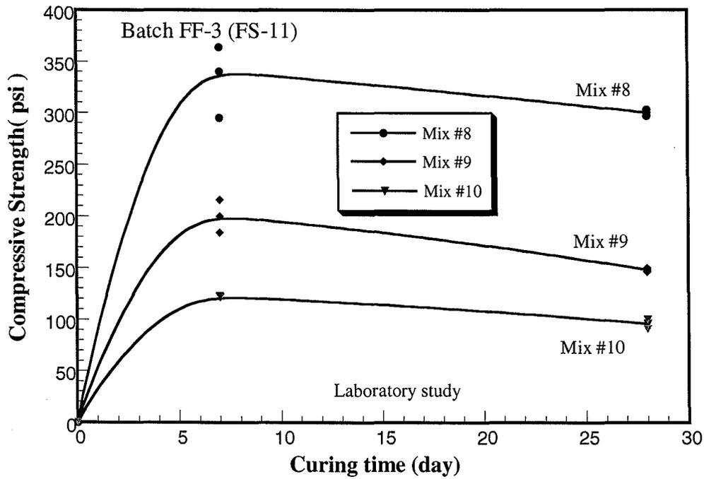
Figure 4.24 Variation of compressive strength with curing time for Batch FF-3
