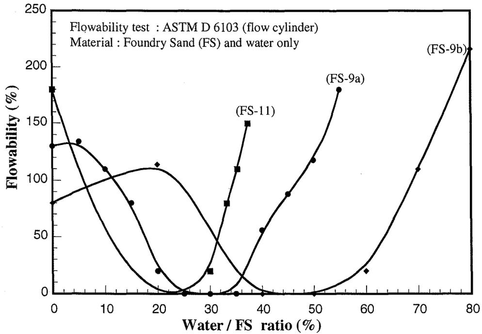
Figure 4.12 Flowability of FS with varying water/FS ratio
