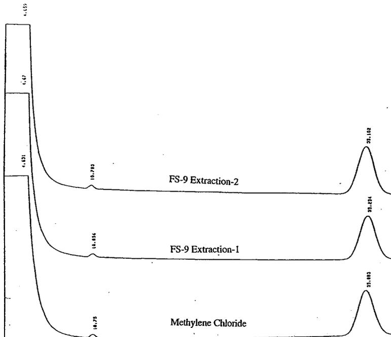
**Figure 3.9. GC Analysis after Methylene Chlorides Extraction with and without Foundry Sand (FS-9a).**
