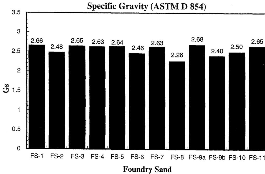
**Figure 3.4. Distribution of Specific Gravity ( $G_s$ ) of Texas Foundry Sands Tested During this Study.**
