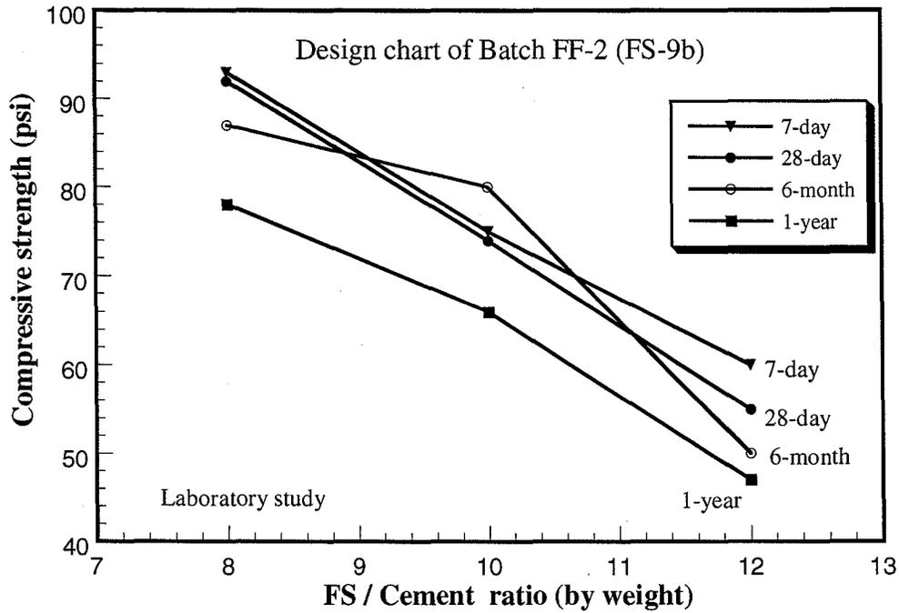
Figure 4.21 FS/cement ratio on the compressive strength of flowable fill (FF-2)
