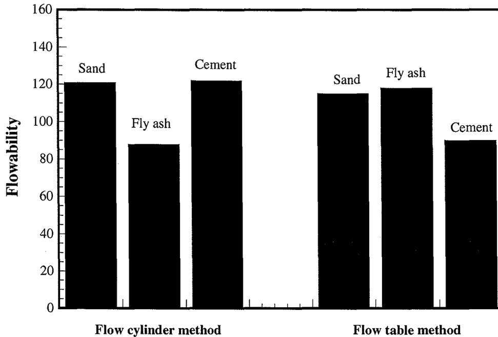
**Figure 4.31. Flowability of dry materials using the Flow cylinder and Flow table tests.**
