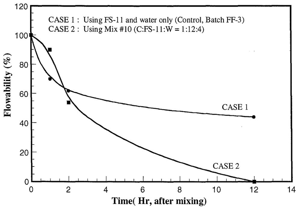
Figure 4.13 Flowability versus time for Batch FF-3
