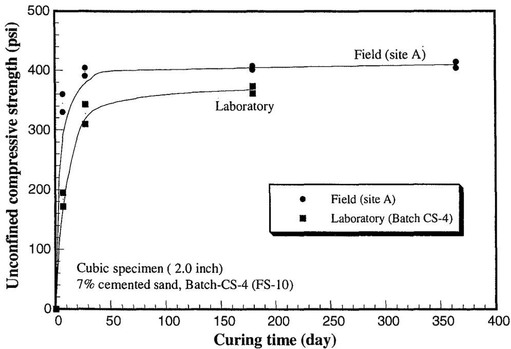
Figure 5.27 Comparison of the unconfined compressive strength with laboratory and field data (cubic specimen)
