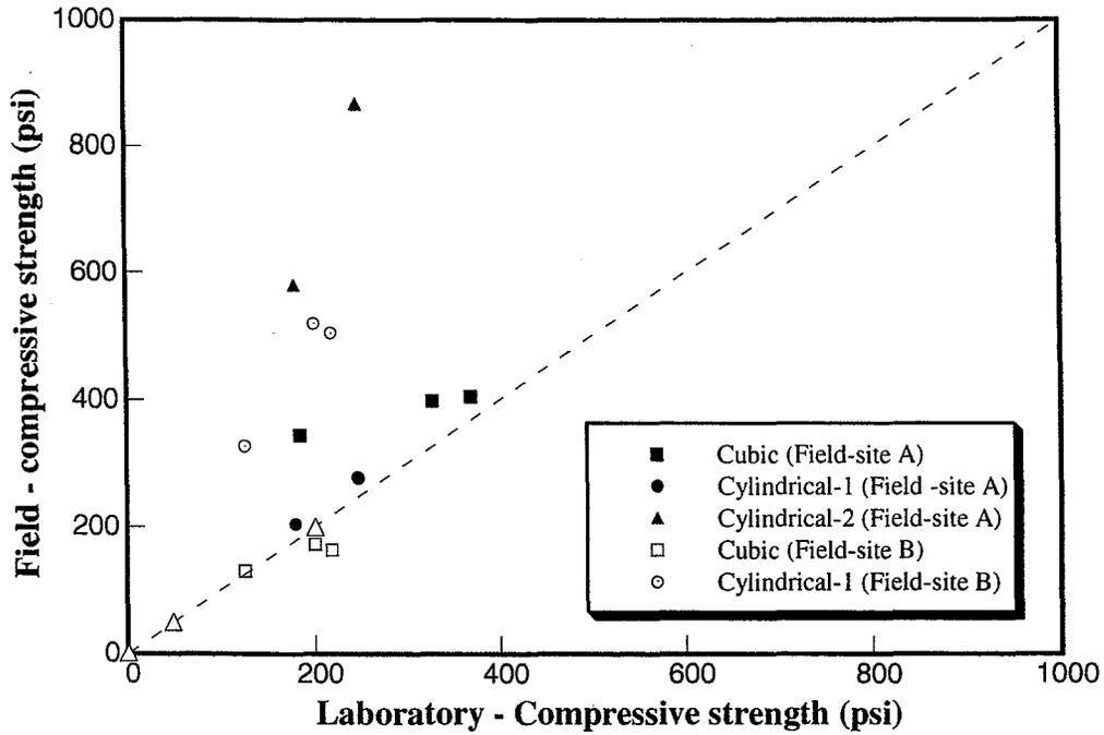
Figure 5.26 Comparison of the unconfined compressive strength with laboratory and field data
