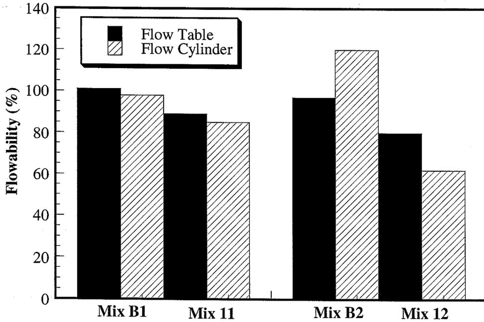
Figure 4.28 The flowability of kaolinite flowable fill with blasting sand and FS-3
