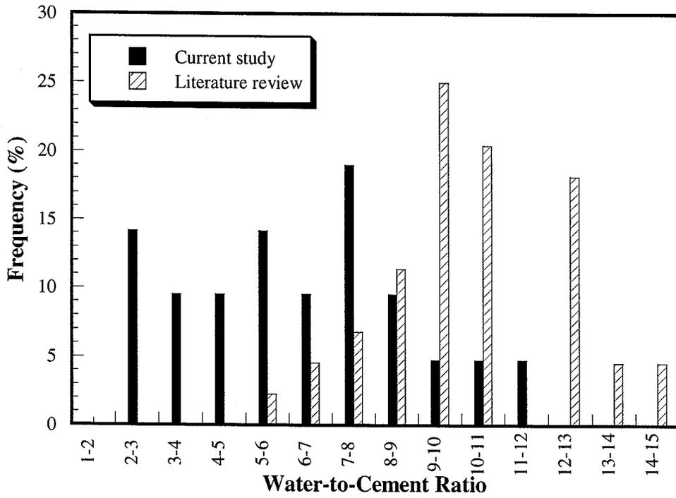
Figure 4.50 Variation of water-to-cement ratio used for flowable fill mixes
