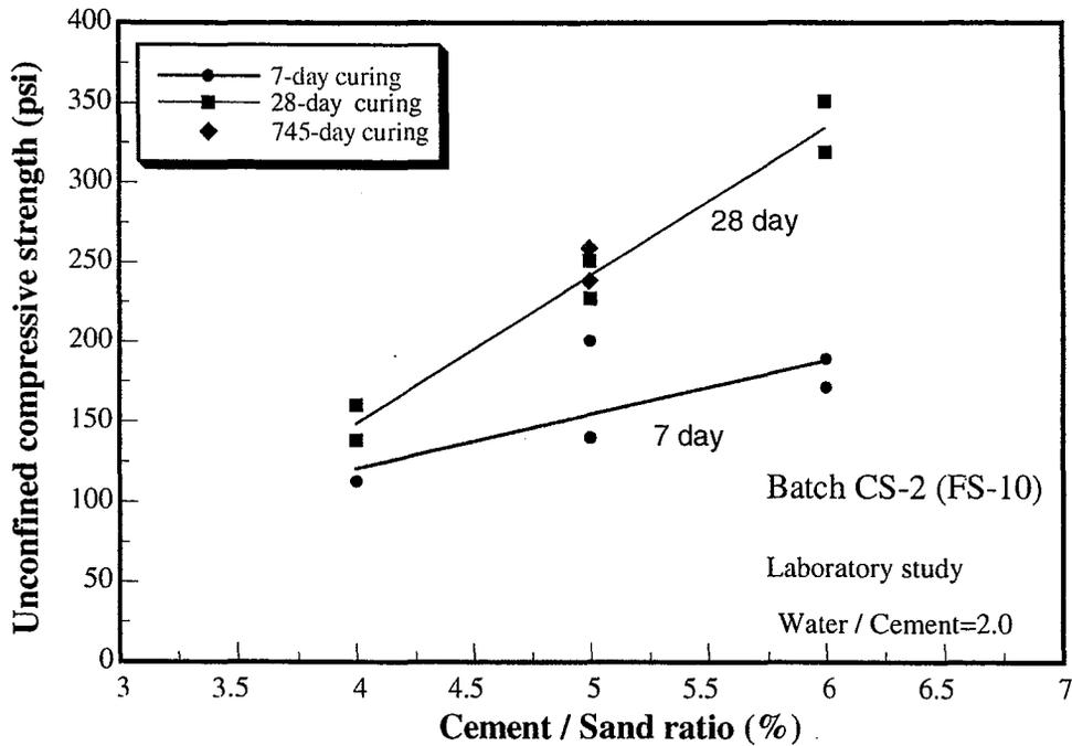
Figure 5.7 Variation of unconfined compressive strength with curing time (Batch CS-2. laboratory study)
