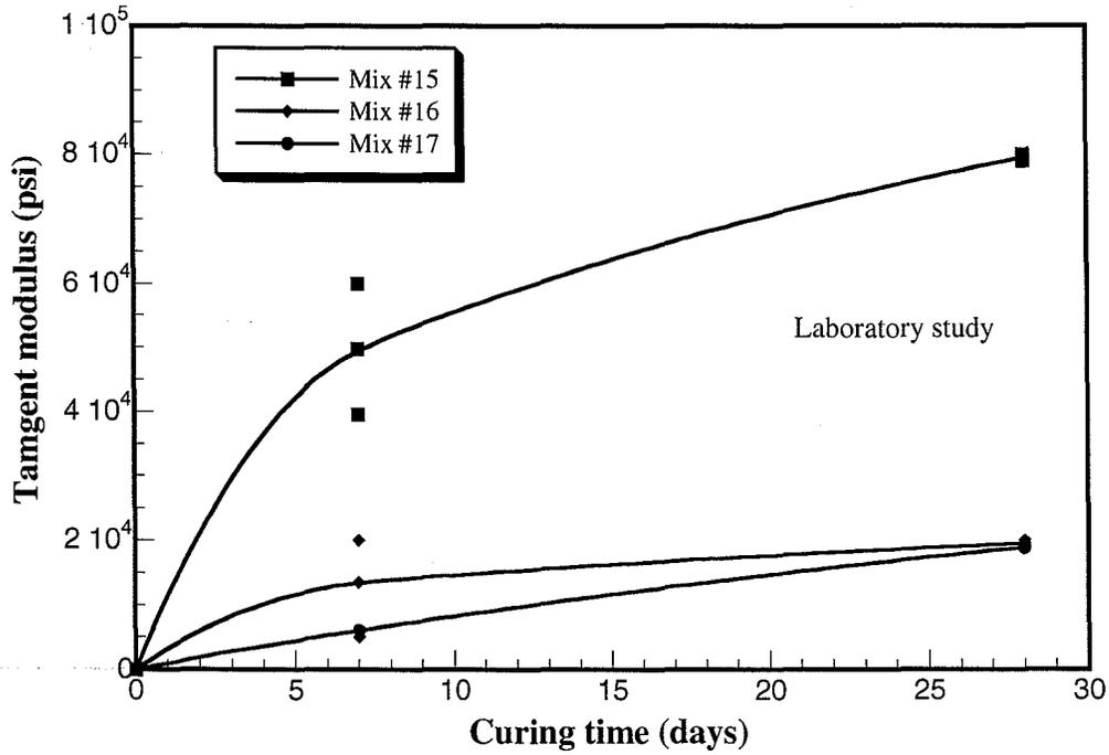
Figure 4.36 Variation of modulus with curing time
