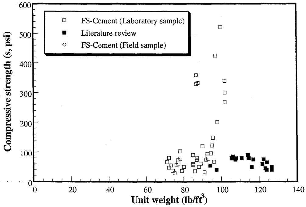
Figure 4.54 Strength versus unit weight
