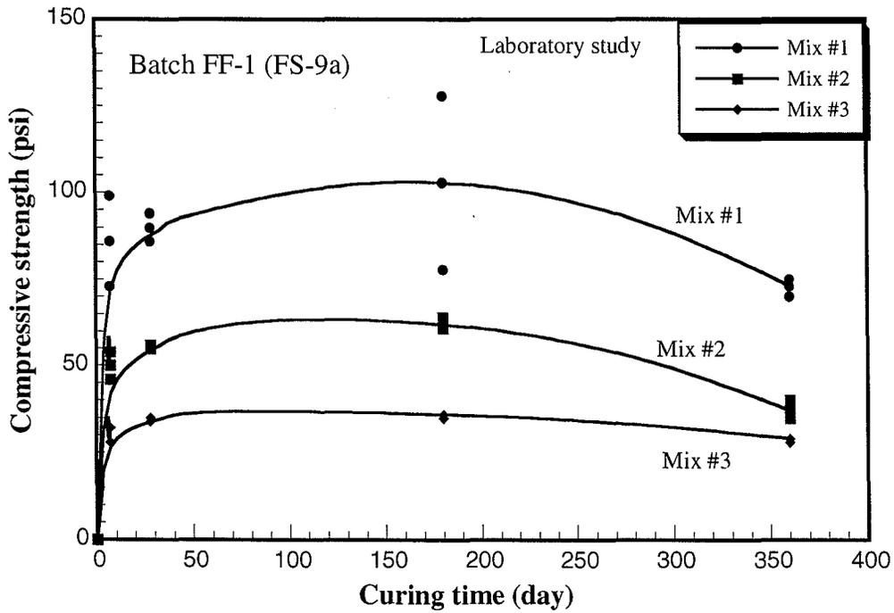
Figure 4.20 Variation of compressive strength with curing time for Batch FF-1
