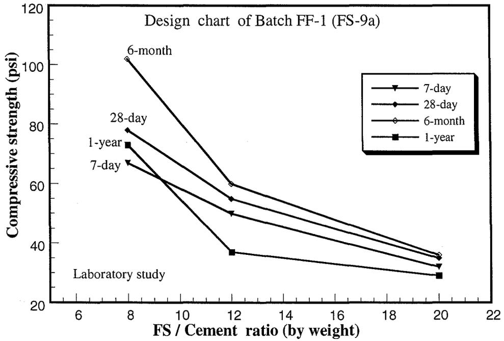
Figure 4.19 FS/cement ratio on the compressive strength of flowable fill (FF-1)
