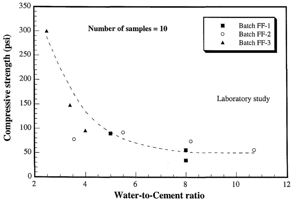
Figure 4.26 Strength versus water-to-cement ratio
