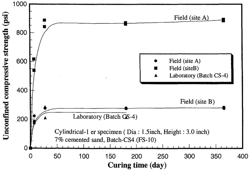
Figure 5.28 Comparison of the compressive strength with laboratory and field data (cylindrical-1 specimen)
