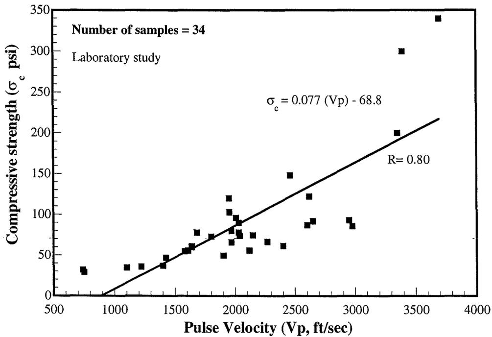
Figure 4.18 Pulse velocity versus compressive strength relationship
