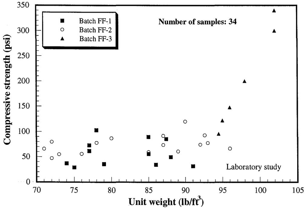
Figure 4.25 Relationship between compressive strength and unit weight
