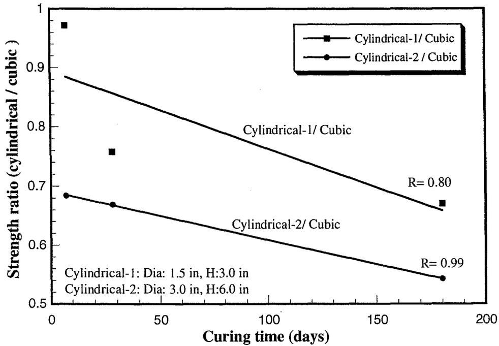
**Figure 5.10 Strength ratio of cubic and cylindrical specimen (Batch CS-3. laboratory study)**
