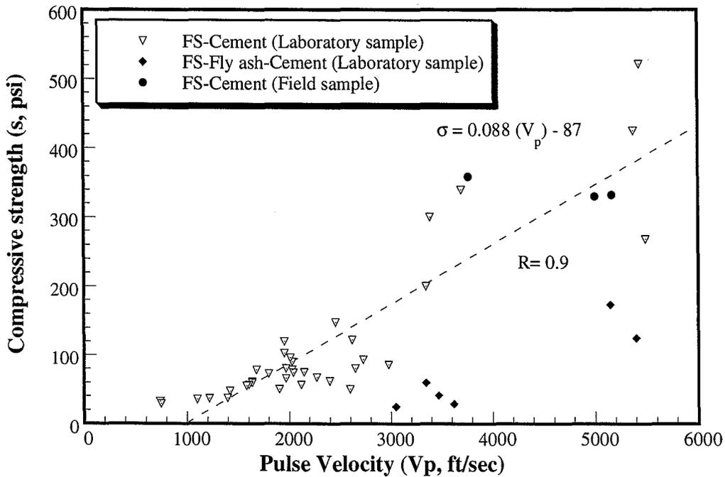
Figure 4.53 Pulse velocity versus compressive strength for flowable fill with FS
