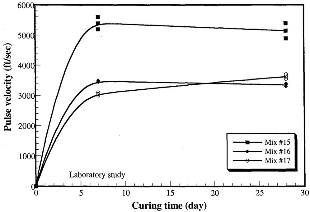
Figure 4.34 Variation of pulse velocity with curing time
