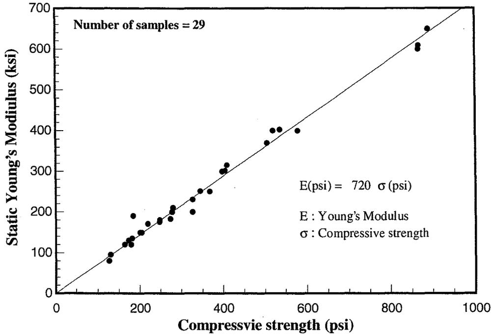
Figure 5.32 Comparison of unconfined compressive strength with modulus
