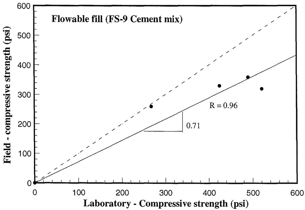
Figure 4.49 Comparison of compressive strength (laboratory and field sample)
