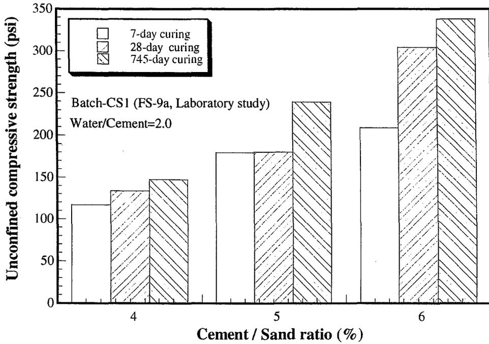
Figure 5.6 Unconfined compressive strength with varying cement / sand ratio and curing time (Batch CS-1. laboratory study)
