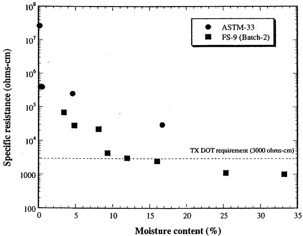
**Figure 3.10. Variation of Specific Resistivity with Moisture Content for Foundry Sand (FS-9a) and ASTM C 33 Sand.**
