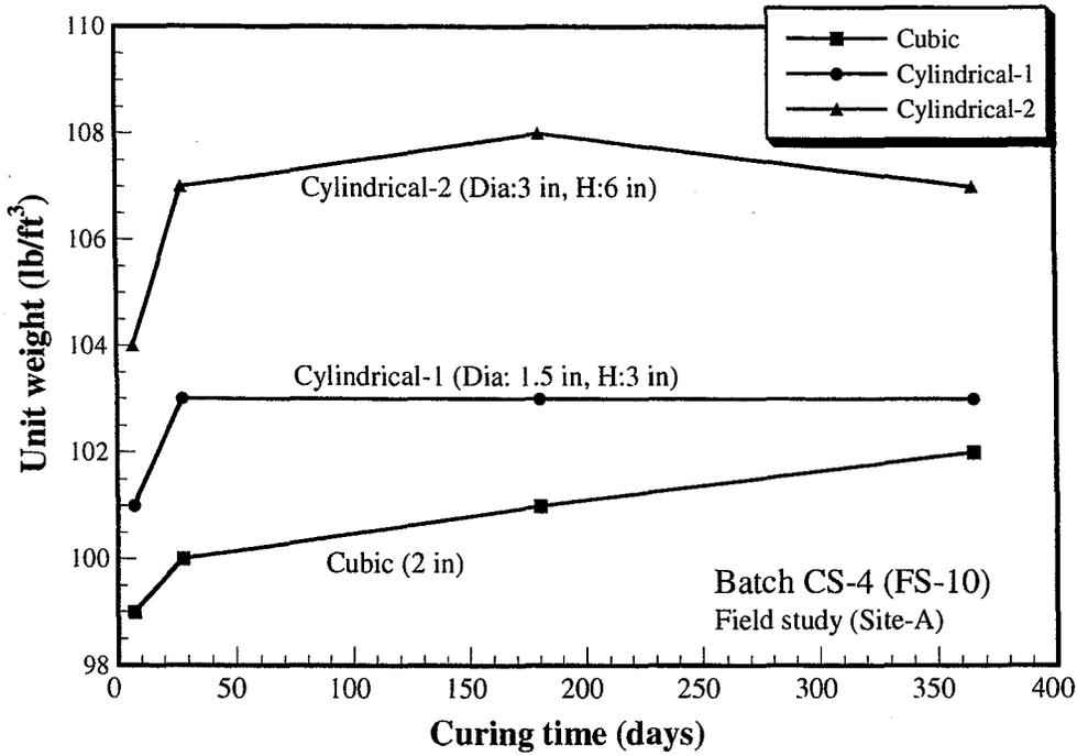
Figure 5.16 Variation of unit weight with curing time (Batch CS-4, field study, Houston, Texas)
