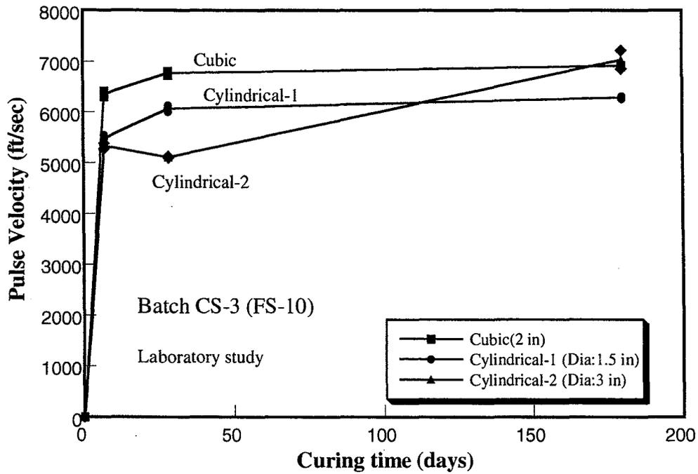
Figure 5.4 Variation of pulse velocity with curing time (Batch CS-3, laboratory study)
