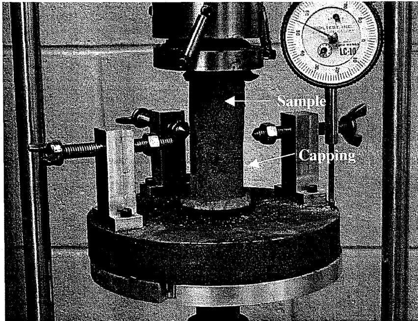
**Figure 4.11 Unconfined compressive strength test**
