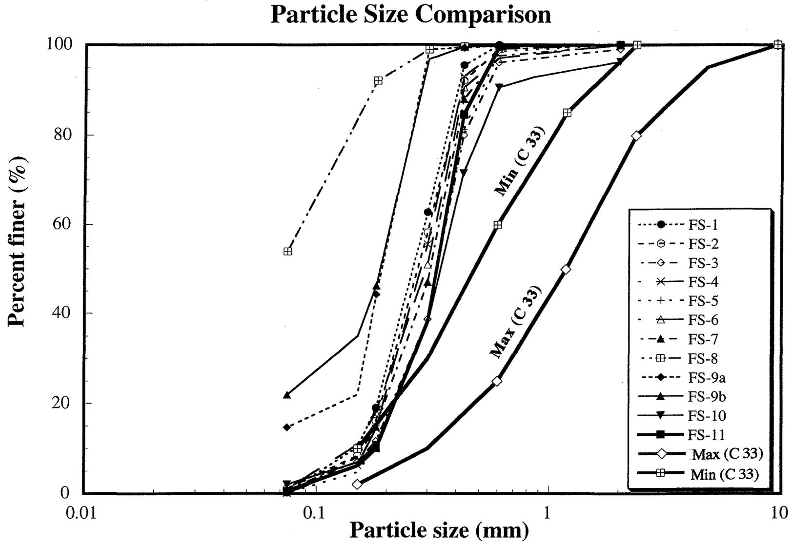
**Figure 3.6. Particle Size Distribution of Texas Foundry Sands Tested During this Study.**
