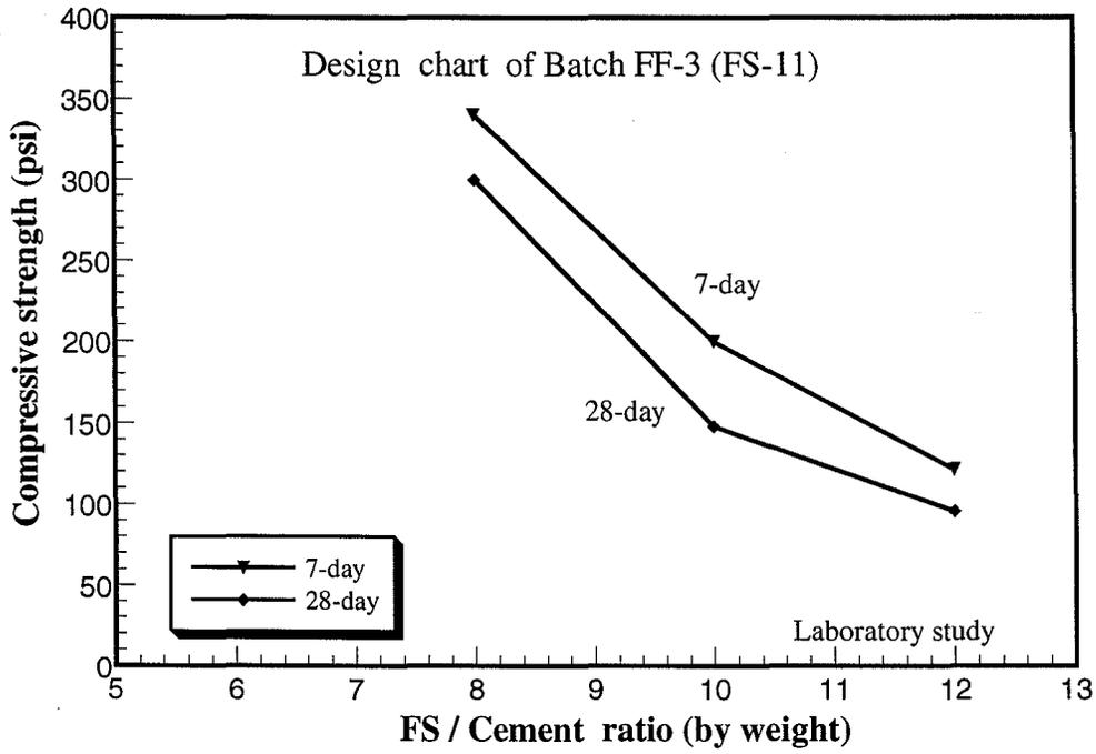
Figure 4.23 FS/cement ratio on the compressive strength of flowable fill (FF-3)
