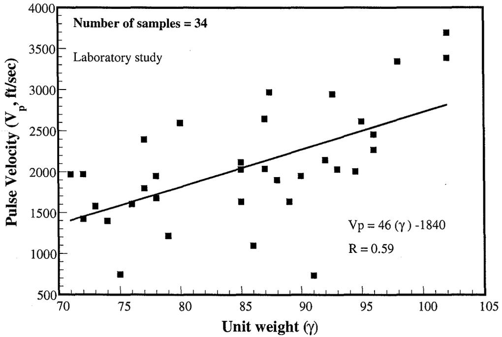
Figure 4.16 Variation of pulse velocity with unit weight
