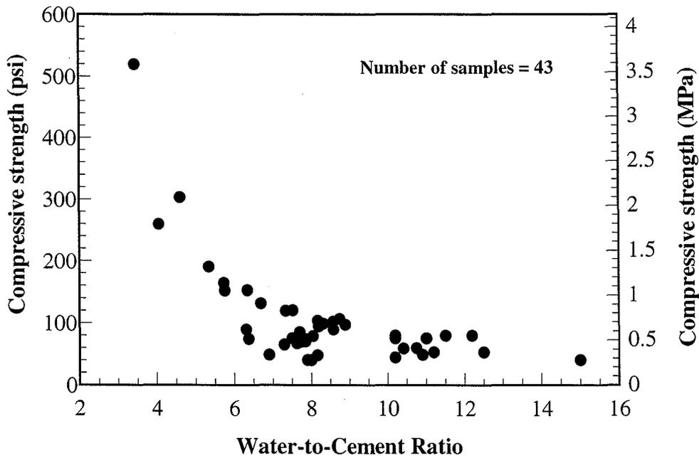
Figure 4.4 Strength versus water-to-cement ratio for the flowable fill with FS (Literature review)
