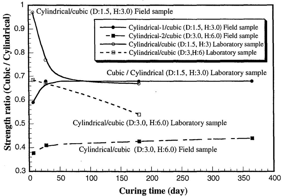
Figure 5.33 Unconfined compressive strength ratio of cubic and cylindrical specimen
