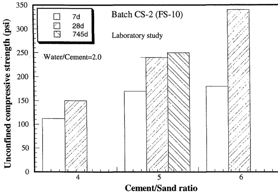
**Figure 5.8 Unconfined compressive strength with varying cement / sand ratio and curing time (Batch CS-2. laboratory study)**
