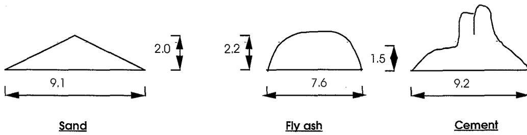
Figure 4.32 Flow shapes of different dry materials after flow cylinder test
