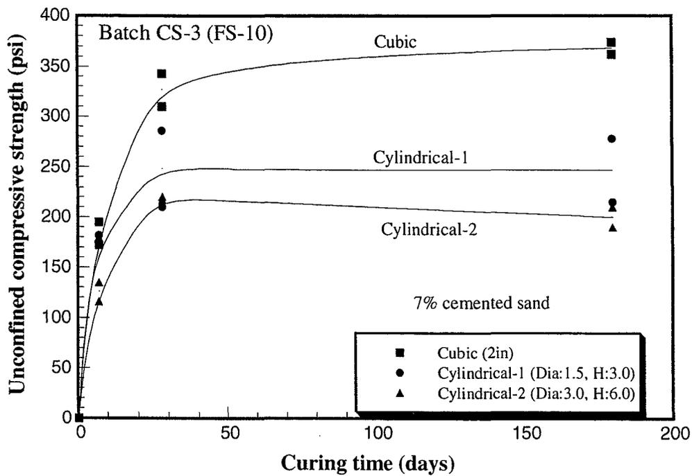
**Figure 5.9 Unconfined compressive strength with varying specimen size, shape, and curing time (Batch CS-3. laboratory study)**
