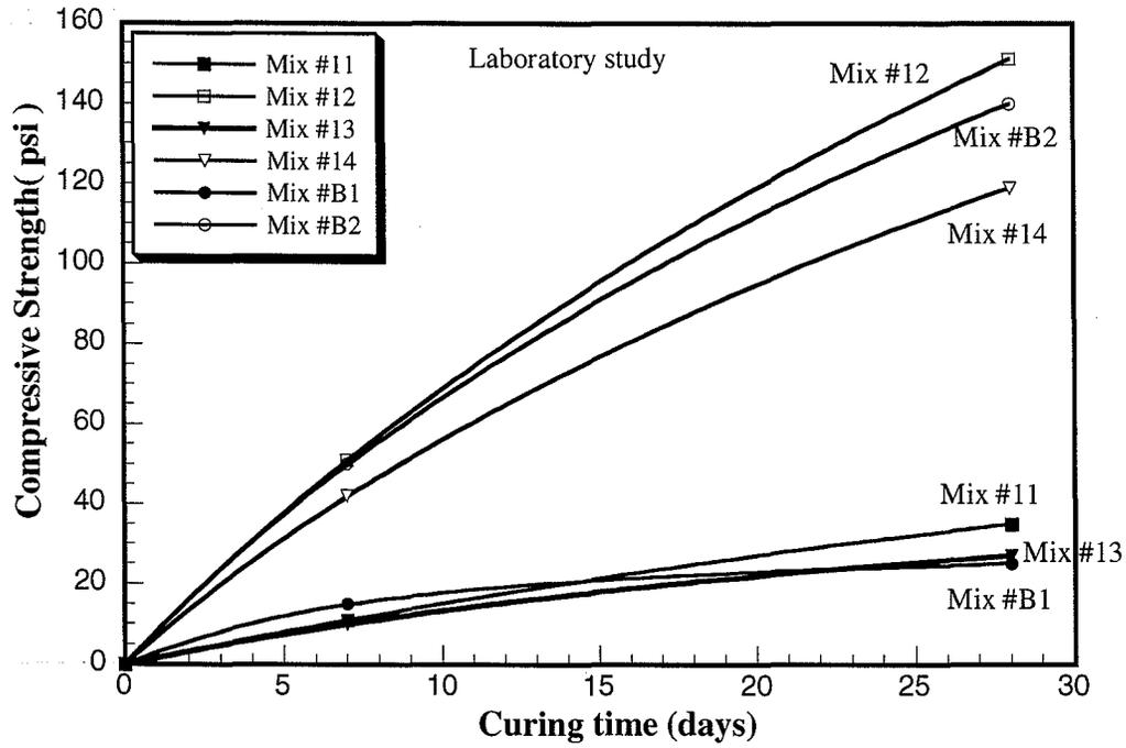
Figure 4.30 The strength versus curing time of for FS-cement-kaolinite flowable fill
