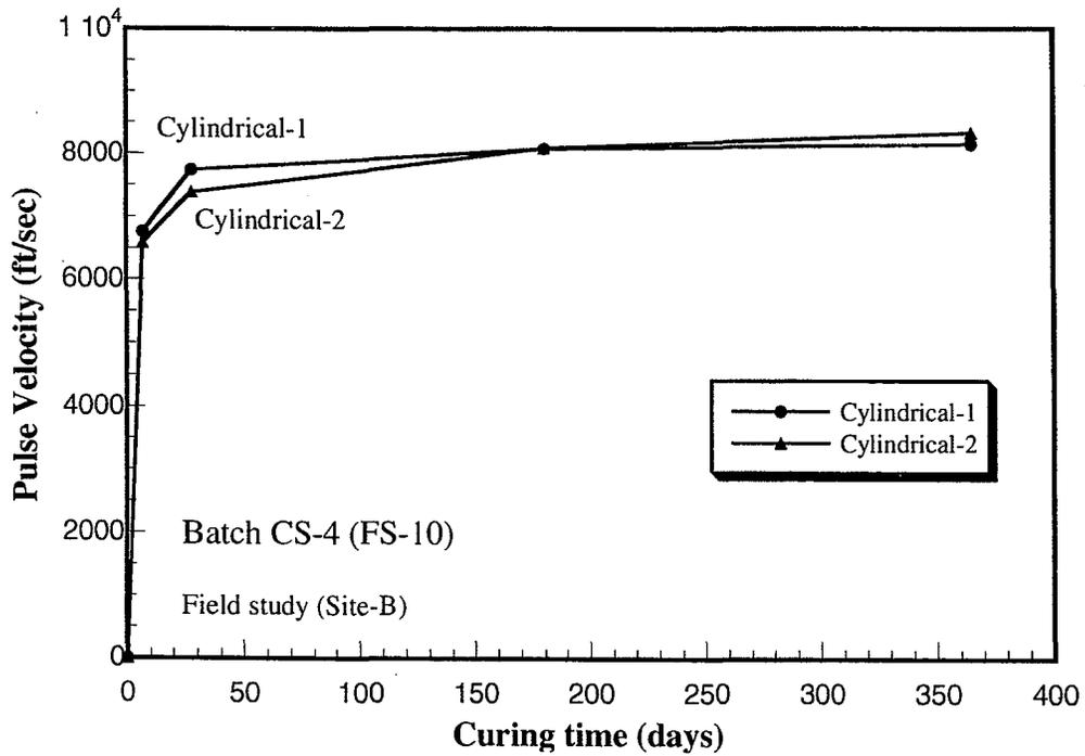
**Figure 5.19** Variation of pulse velocity with curing time
