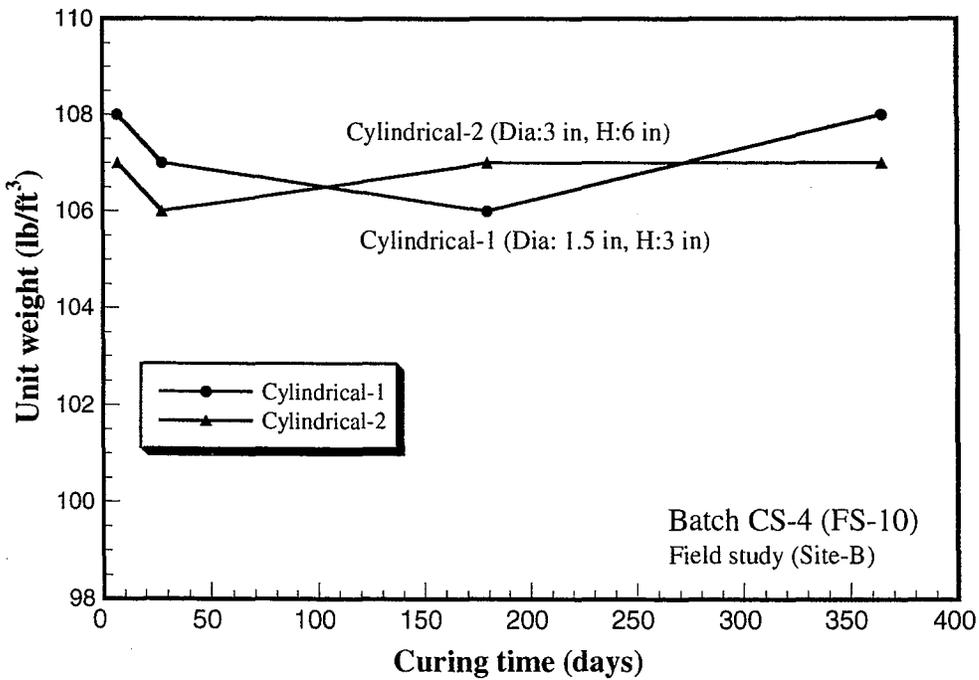
Figure 5.17 Variation of unit weight with curing time (Batch CS-4, field study, Houston, Texas)
