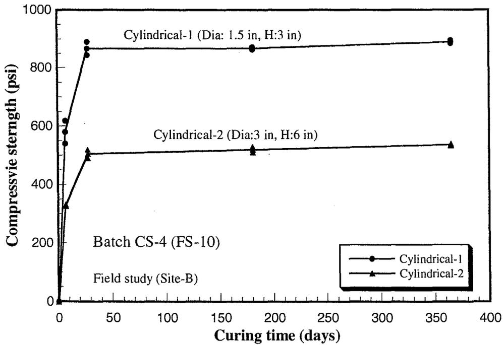
Figure 5.21 Unconfined compressive strength with varying specimen size, shape, and curing time (Batch CS-4. field study, Site-B)
