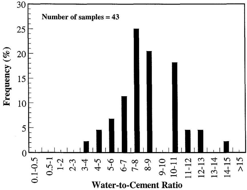
Figure 4.1 Variation of water-to-cement ratio for flowable fill with FS (Literature review)
