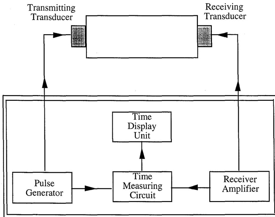
**Figure 4.9 Schematic of the pulse velocity testing set up**
