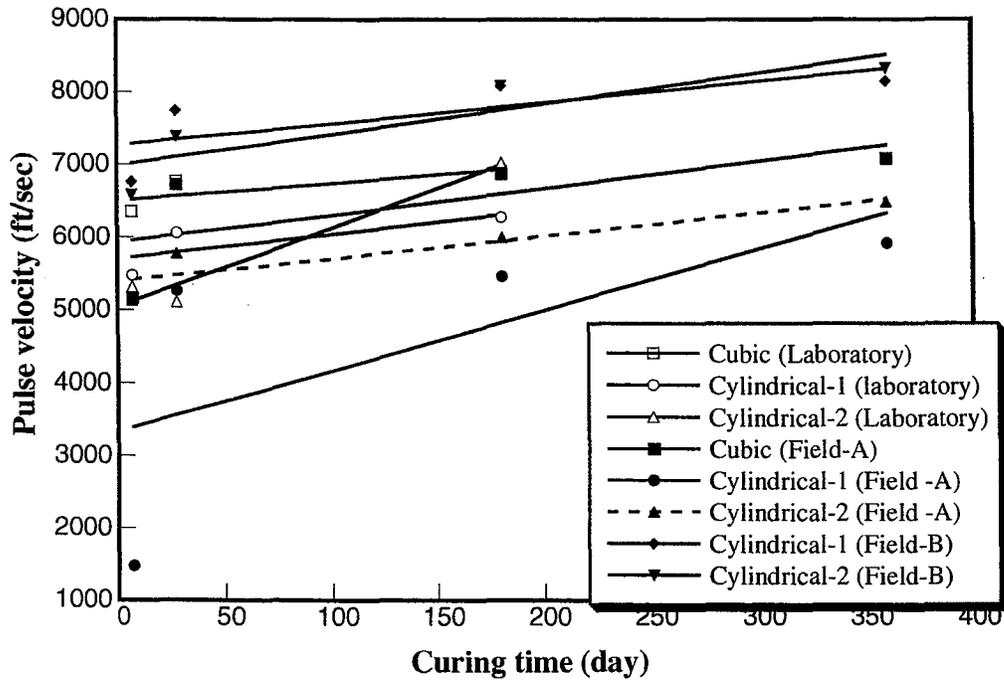
Figure 5.24 Comparison of the pulse velocity with laboratory and field samples
