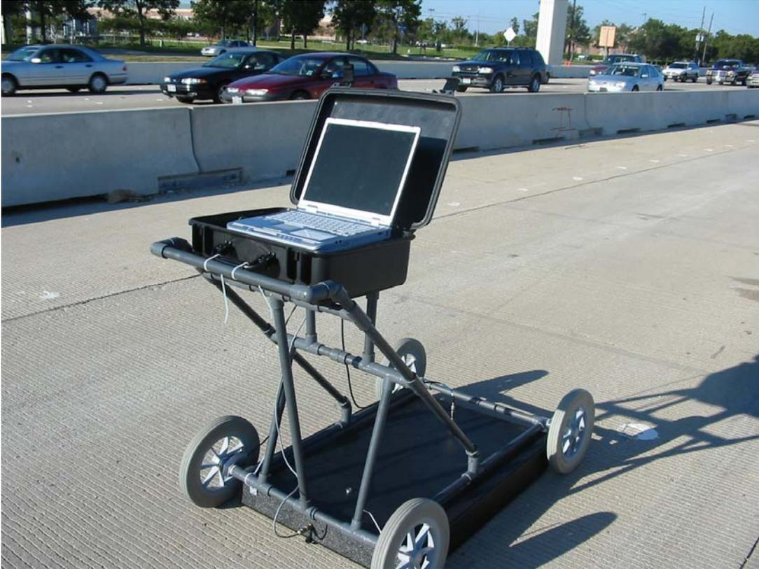
**Figure 2.2 GPR system in measurement configuration.**
