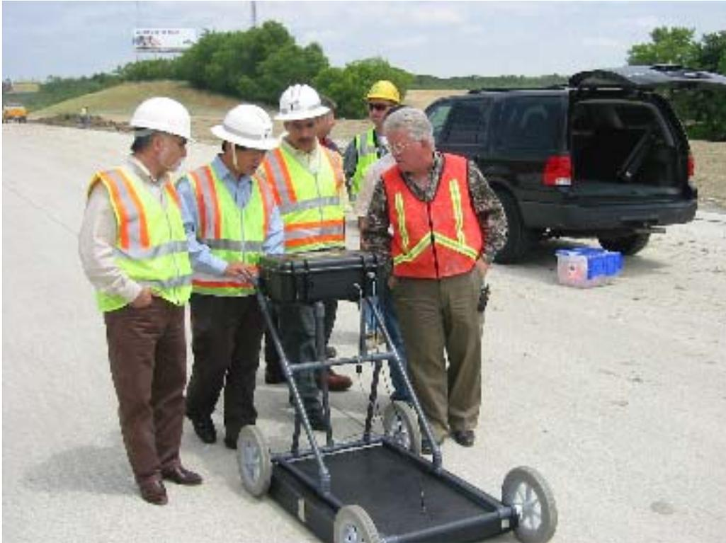
**Figure 3.5 The thickness is displayed on top the GPR enclosure.**
