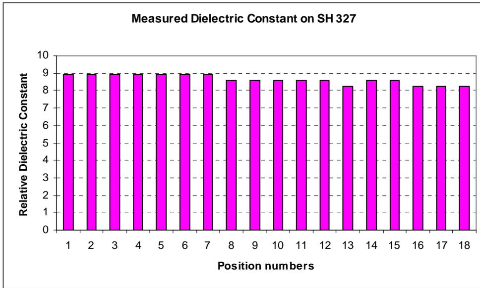
**Figure 4.6 Measured dielectric constants on SH 327.**
