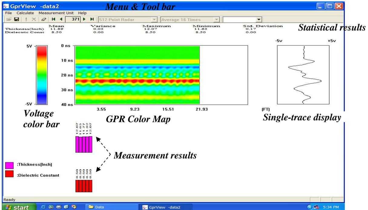
**Figure 2.3 GPR software interface.**
