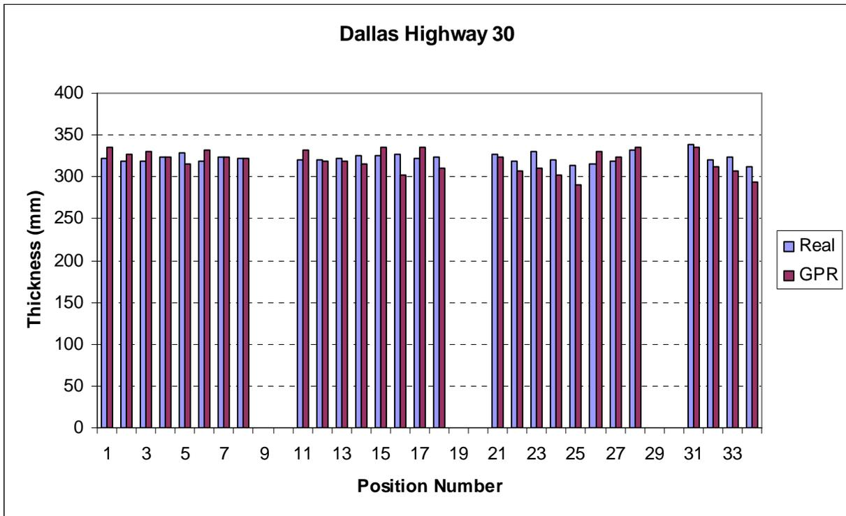
**Figure 4.2 Comparison of the GPR measured thickness with real thickness on Highway 30, Dallas.**
