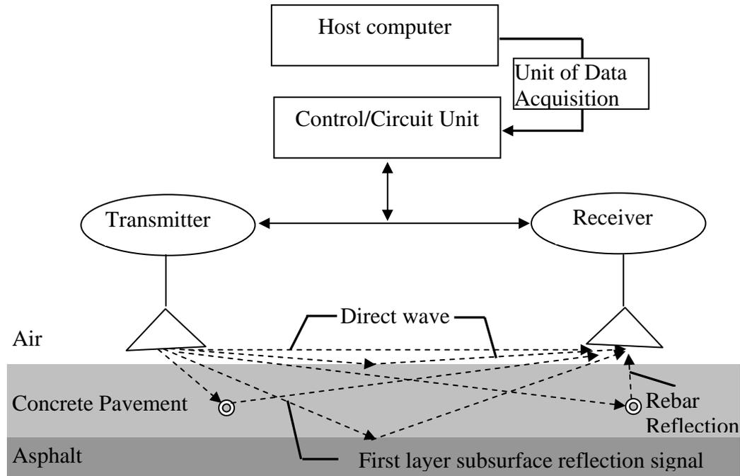
**Figure 2.1** Block diagram of the CPT-GPR system.
