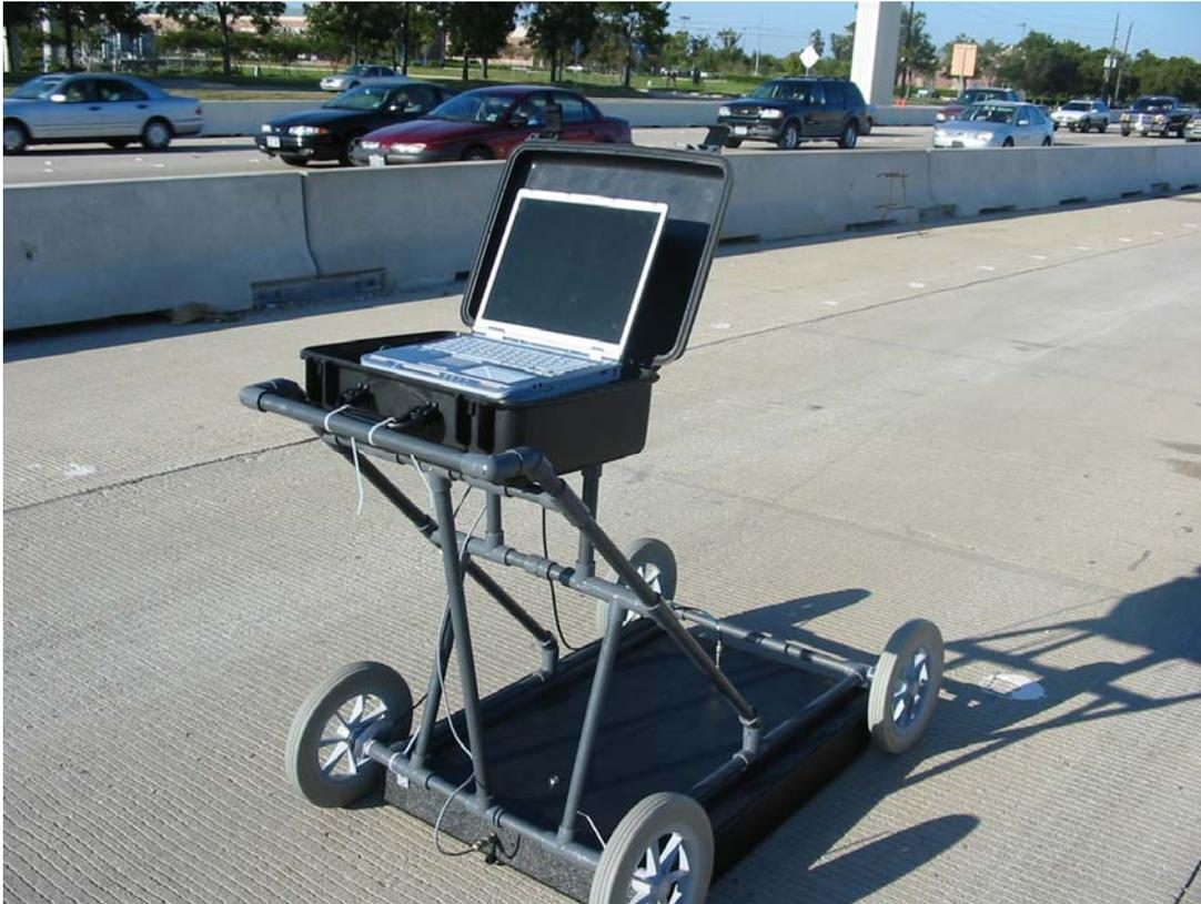
Fig 1.2 GPR system in measurement configuration
