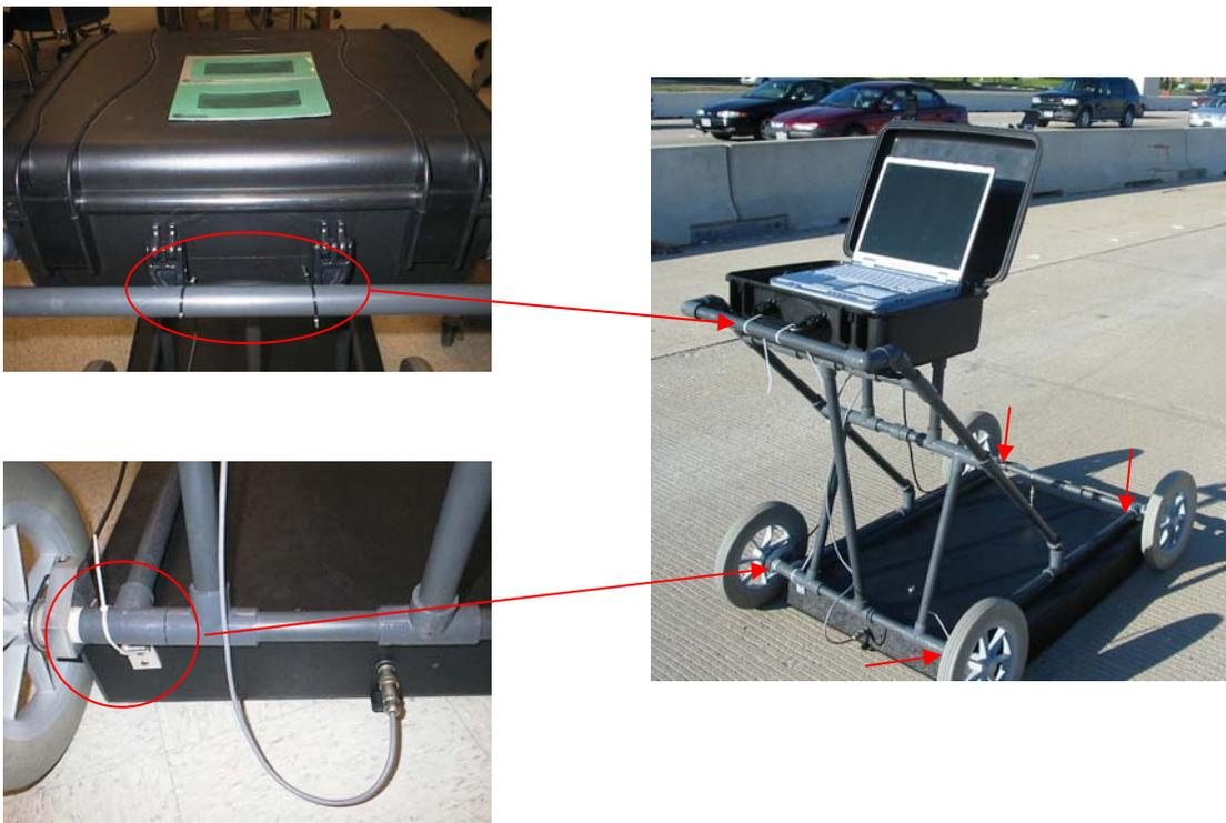
Fig 2.4 Attach the antenna box and circuit box to the cart with cable ties
