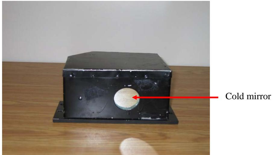
Figure 4 The laser device based on triangulation method.
