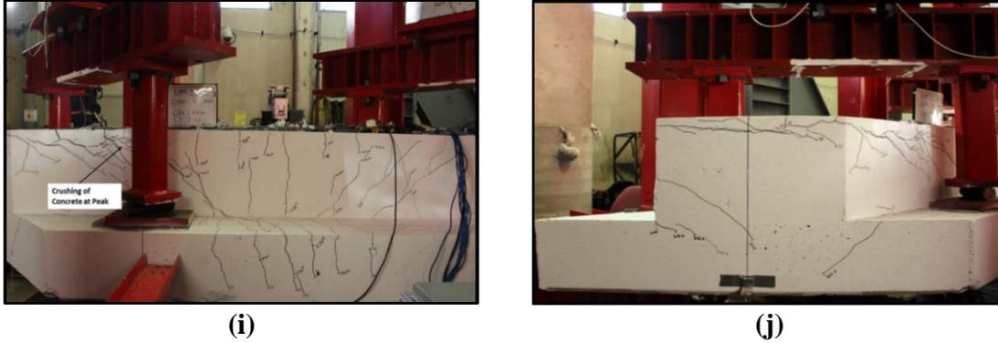
**Figure 4.30. Cracking of Specimen ITBC-45-S-M:**
