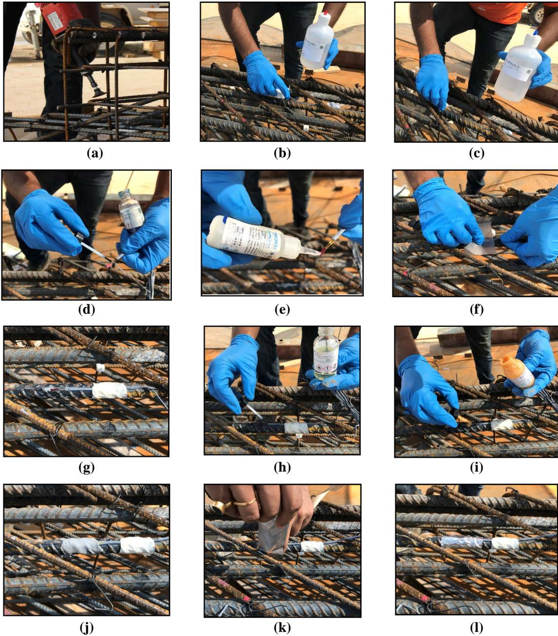
**Figure 3.14. Strain Gauge Installation:**
