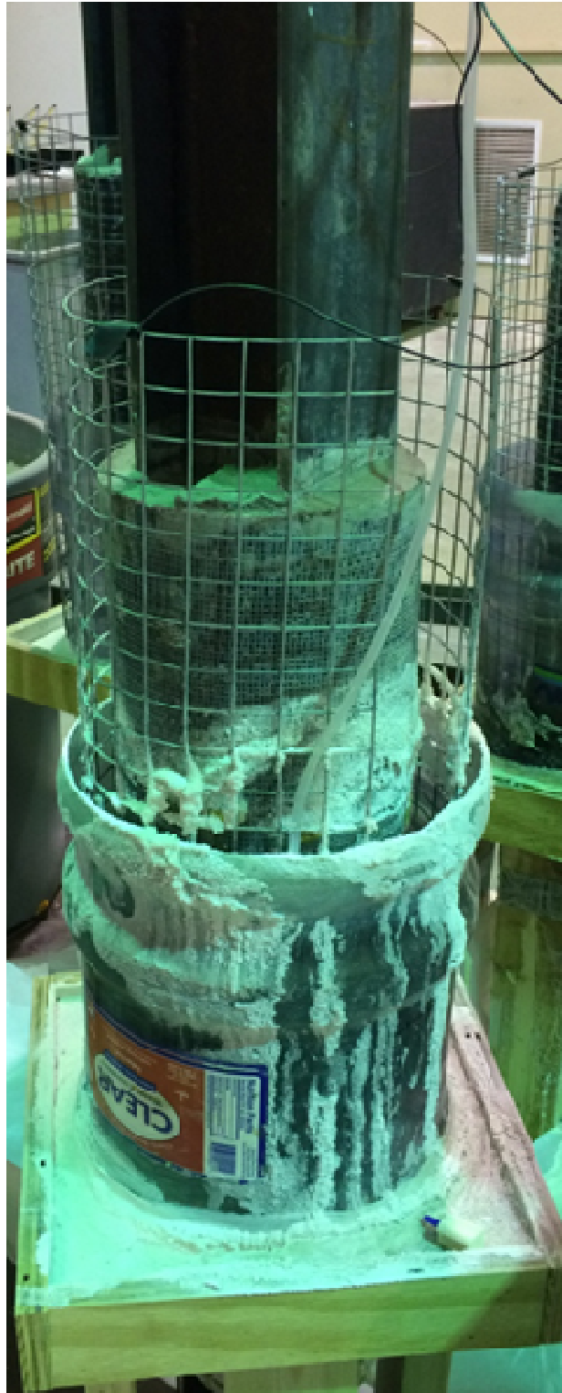
Figure 10.42: A damaged pile repaired with Repair System 1 (S1-4-Cor) showing no evidence of corrosion
