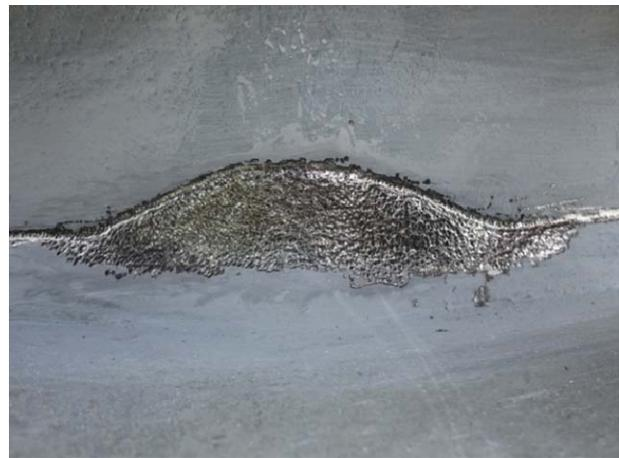
(d) Repair weld after application of UIT to both the face of the weld and toe
