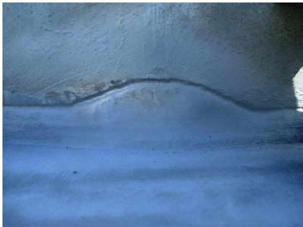
(c) Repair weld made to improve fatigue life. The profile meets the requirements of AWS D1.1. Toe dressing has been performed at the weld toe
