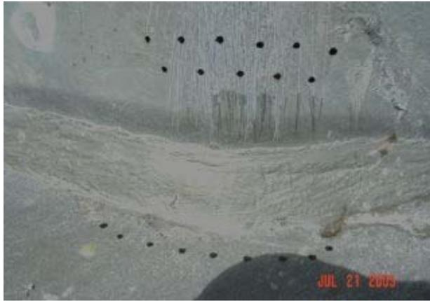
(a) Visual appearance of apex with UT indication of lack of weld fusion (no visible fracture)
