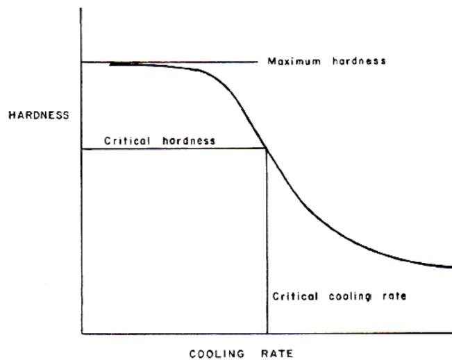
**Figure 7. Typical Hardening Curve of Steel (Graville, 1975).**
