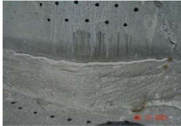
(b) After removal of galvanization by grinding at weld toe (no visible fracture)
