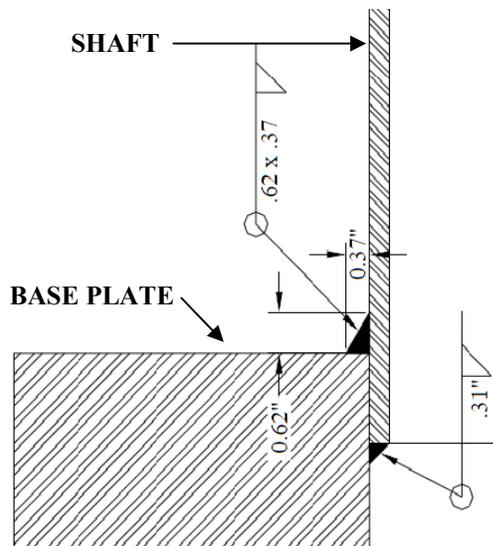
**Figure 5. Fillet Welded Socket Connection Weld Detail (Rios, 2007).**
