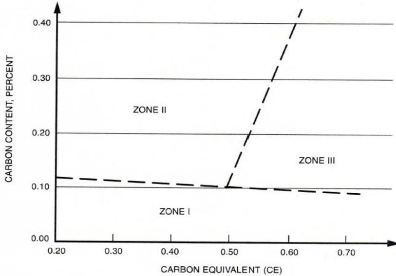
[CE = C + (Mn+Si)/6 + (Cr + Mo + V)/5 + (Ni + Cu)/15, where C = % Carbon, Mn = % Manganese, Si = % Silicon, Cr = % Chromium, Mo = % Molybdenum, V = % Vanadium, Ni = % Nickel and Cu = % Copper]
