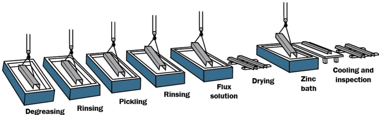
**Figure 10. Galvanizing Process (AGA—[www.galvanizeit.org](http://www.galvanizeit.org)).**
