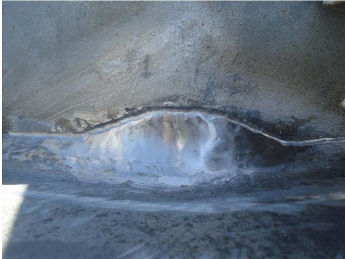
(a) Weld repair with toe dressing (prior to UIT)
