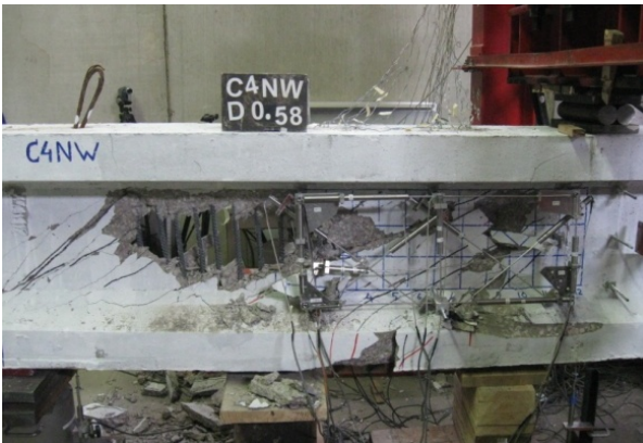
(e) Shear failure at 194 kips
