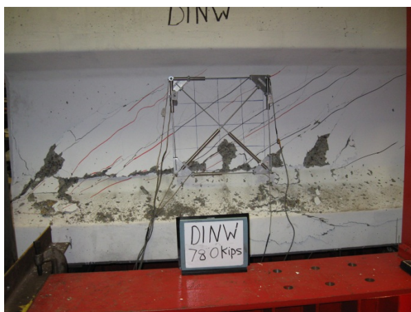
(e) Shear failure at 779.80 kips
