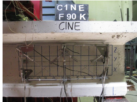
(b) First shear crack at 75 kips
