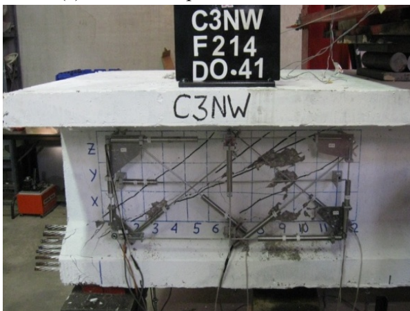
(e) Shear failure at 214.44 kips
