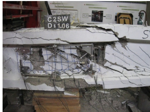
(f) Shear failure at 164.60 kips
