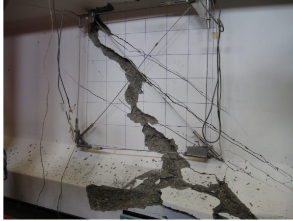
(c) Shear failure at 756.42 kips
