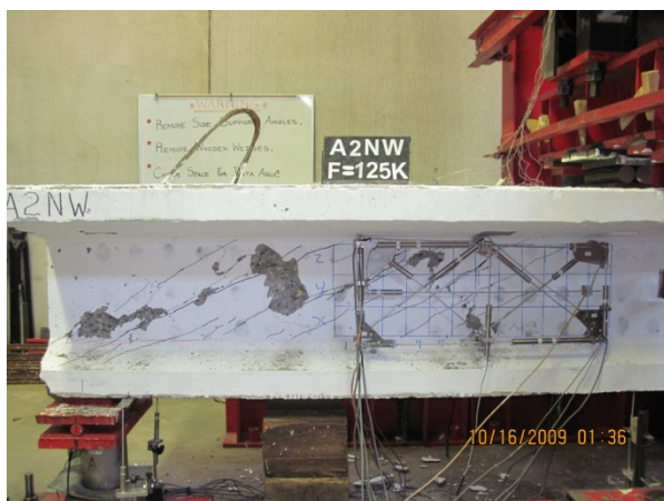
(e) Shear failure at 125.60 kips
