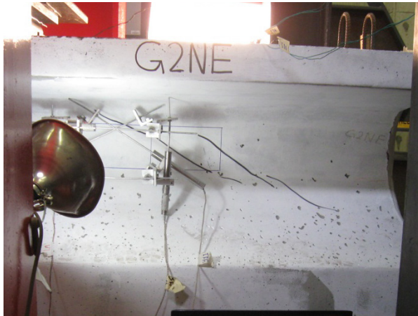
(a) First shear crack at 206 kips
