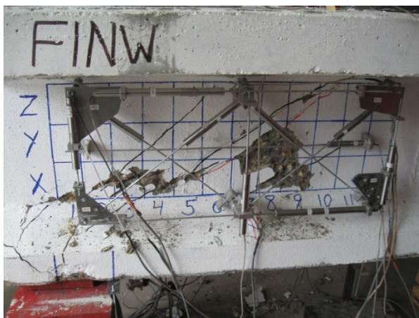
(e) Shear failure at 202.90 kips
