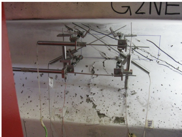
(e) Shear failure at 457.22 kips
