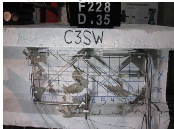
(f) Shear failure at 228.24 kips
