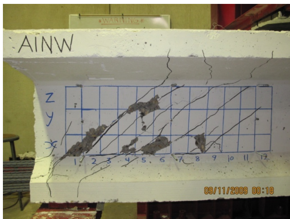
(e) Shear failure at 138.21 kips
