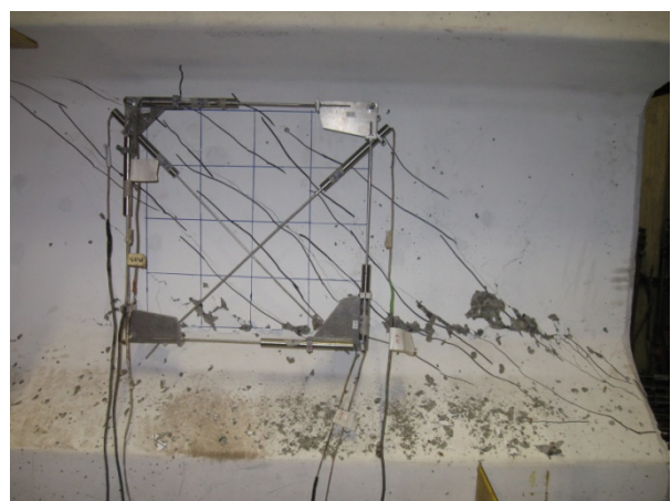
(f) Shear failure at 912.78 kips
