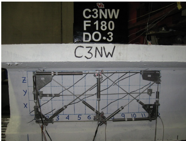
(c) Shear crack pattern before failure
