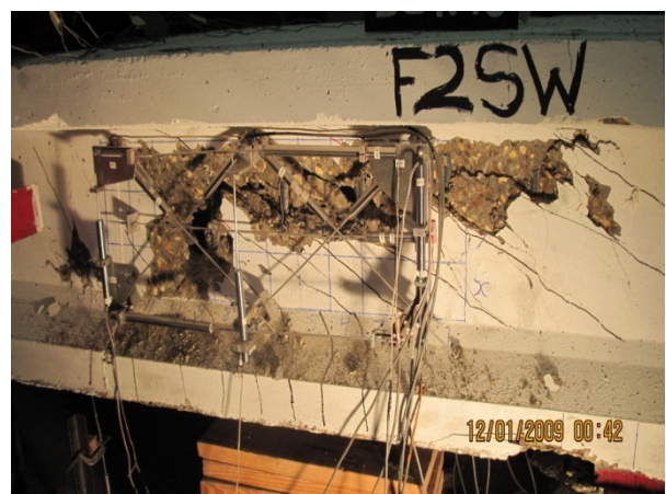
(f) Shear failure at 185.35 kips
