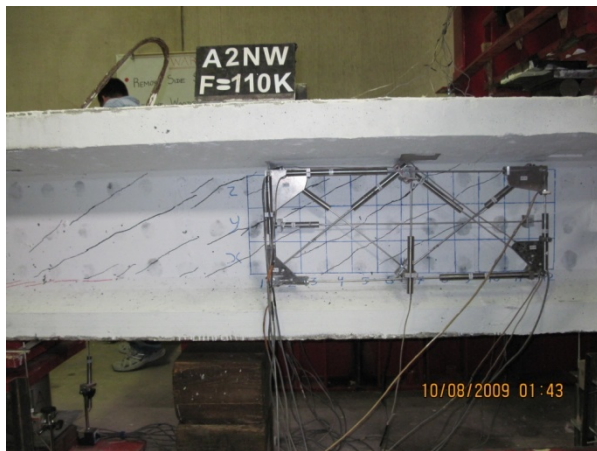
(c) Shear crack pattern before failure
