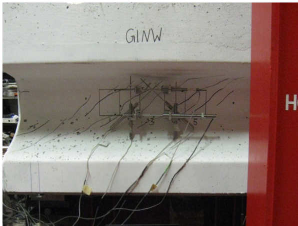
(c) Shear crack pattern before failure
