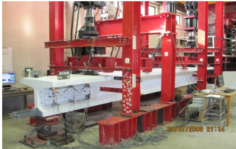
Fig. 3.21 Test Setup for Girders
