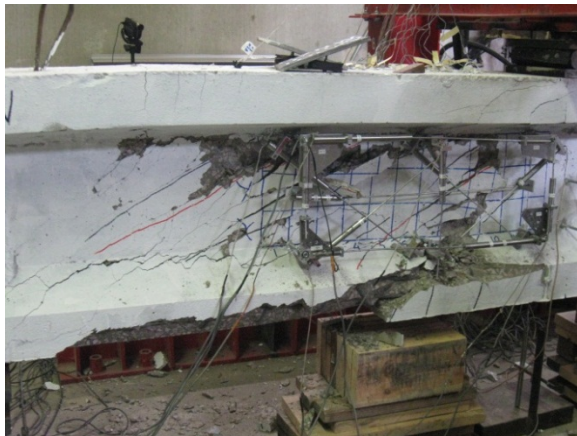
(e) Shear failure at 190.10 kips
