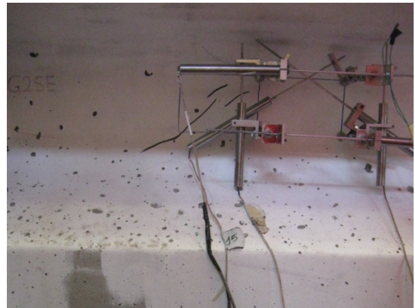
(b) First shear crack at 213 kips
