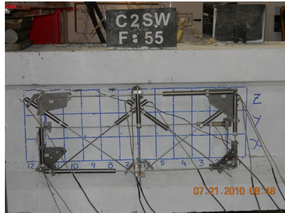
(b) First shear crack at 53 kips
