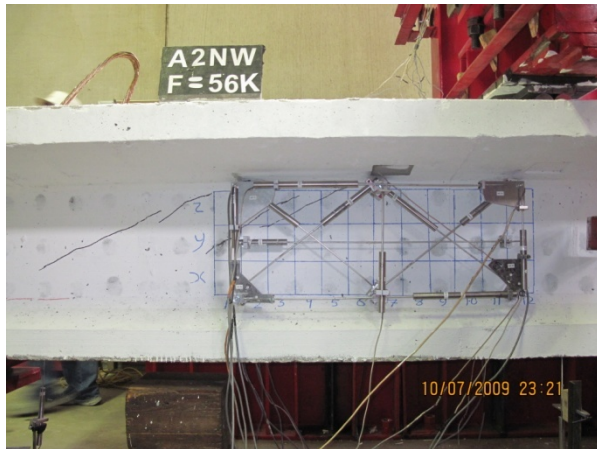
(a) First shear crack at 56 kips
