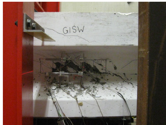
(f) Shear failure at 789.66 kips
