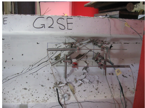
(f) Shear failure at 524.64 kips
