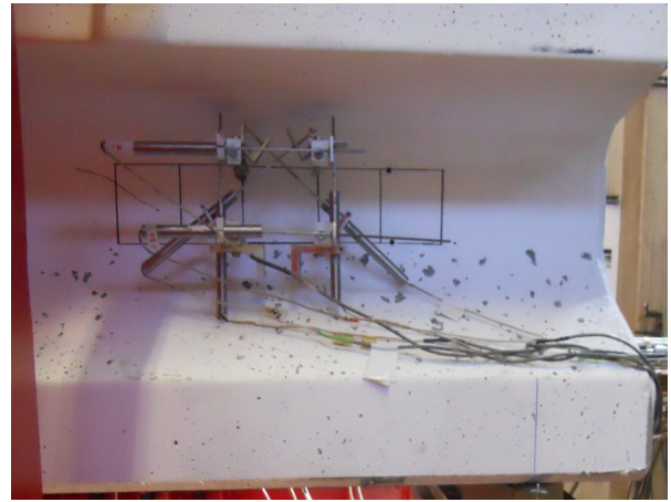
(b) First shear crack at 213 kips
