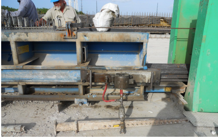
Fig. 6.16 Bed Vibrator Attached to Steel Forms
