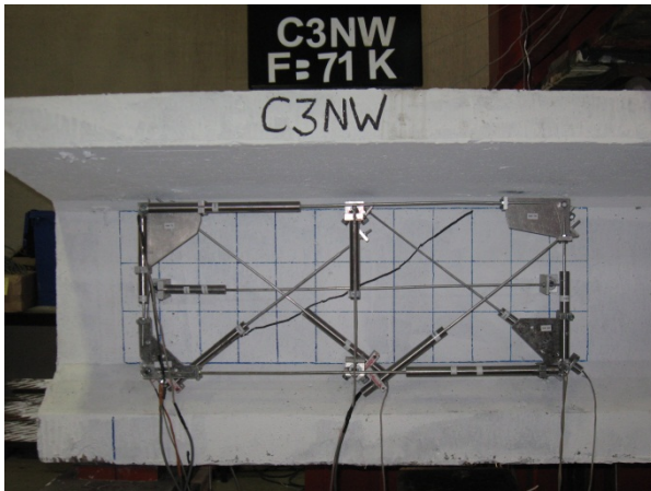
(a) First shear crack at 71 kips
