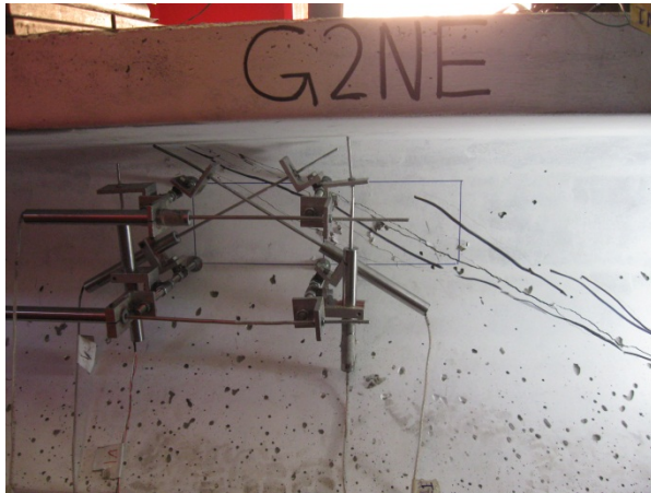
(c) Shear crack pattern before failure
