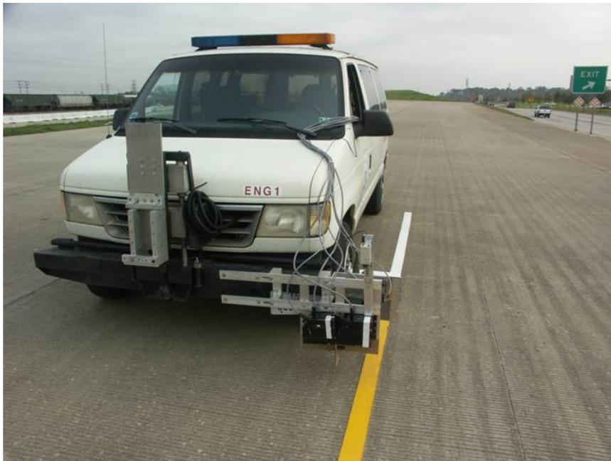
Figure 1 Designed vehicle-mounted device.
