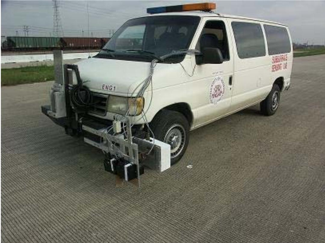
Figure 7 Measurement device mounted on the left side of the vehicle.
