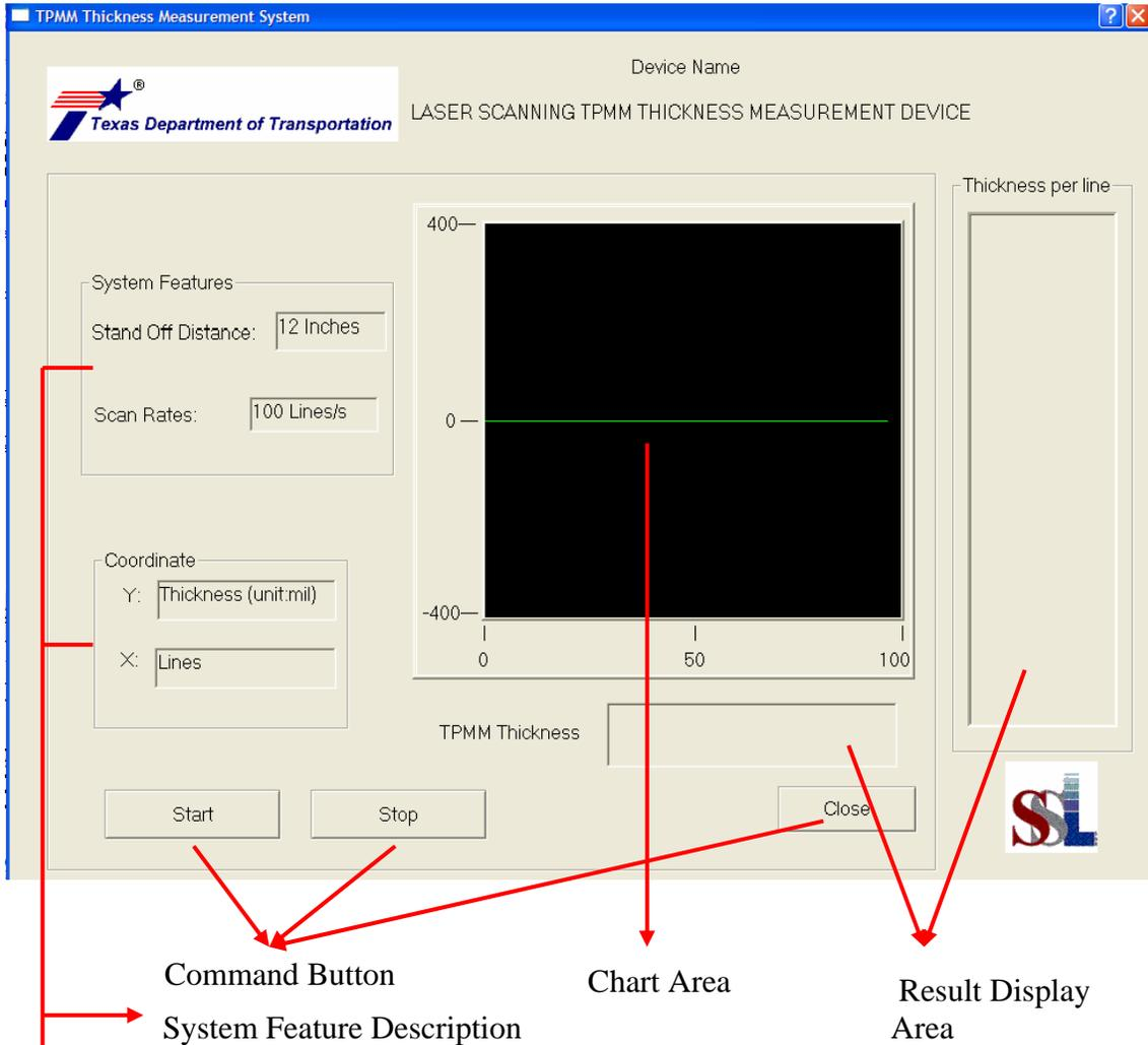
Figure 12 The interface of TPMM measurement software.
