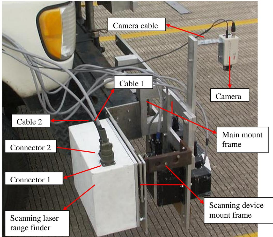
Figure 9 Configuration of vehicle-mounted TPMM measurement system.
