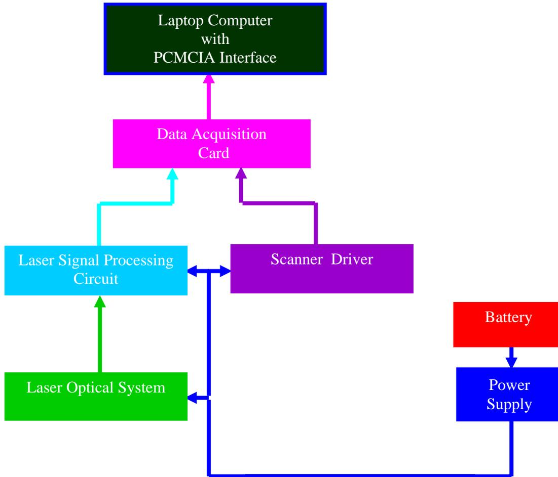
Figure 2 Hardware design block diagram.
