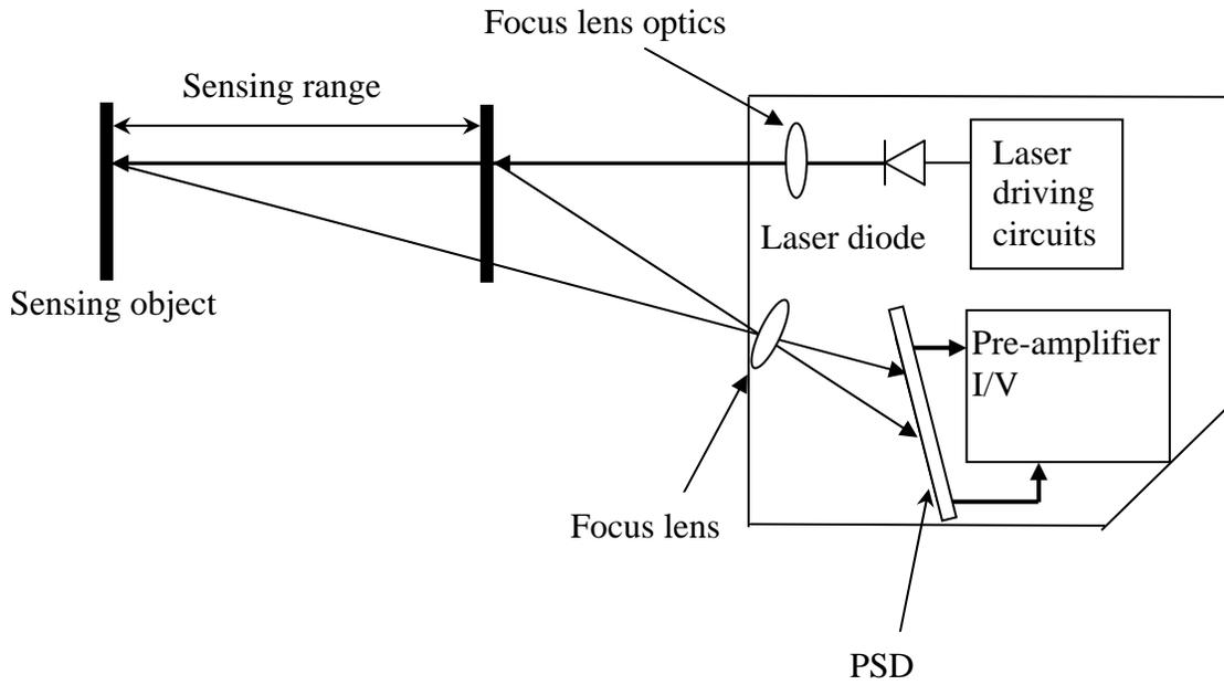
Figure 4 The laser-based triangulation optical system.
