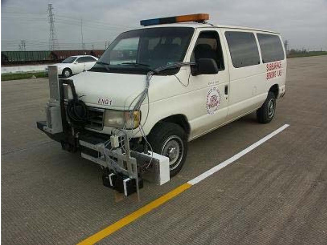
Figure 6 Scanning laser device in measurement.
