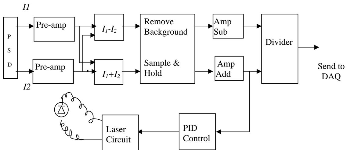
Figure 4 Block diagram of signal processing circuit.
