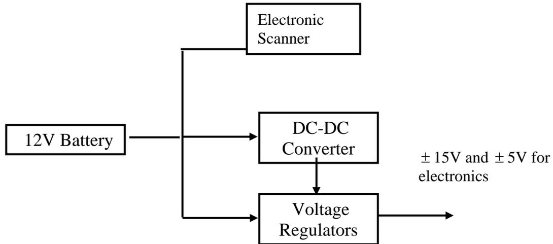
Figure 5 Block diagram of power supply system.
