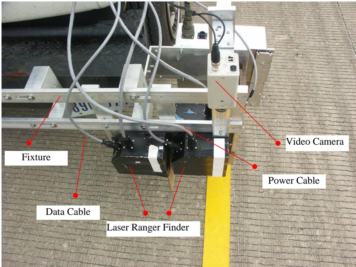
Figure 7 Vehicle-mounted measurement system components.
