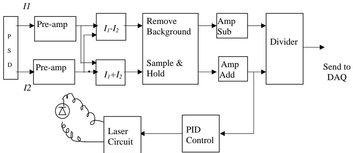
Figure 5 Block diagram of signal processing circuit.
