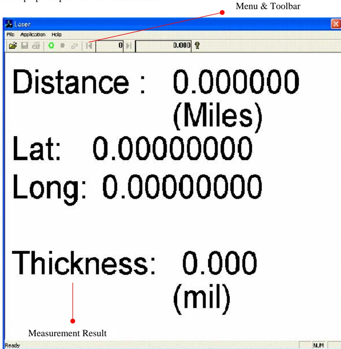
Figure 9 The interface of TPMM measurement software.
