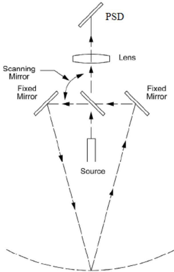
Figure 3 Auto-synchronized triangulation optical system.
