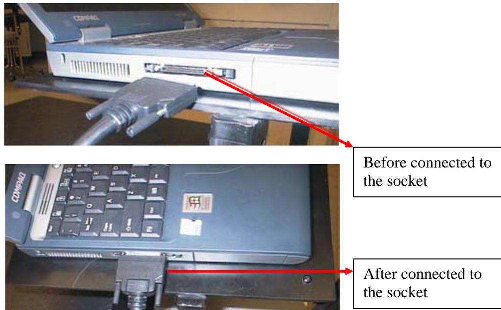
Figure 10 Connection of the data acquisition cable to the socket.
