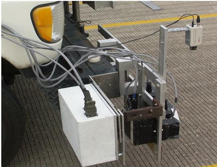
Figure 53 Measurement device mounted on the right side of the vehicle.
