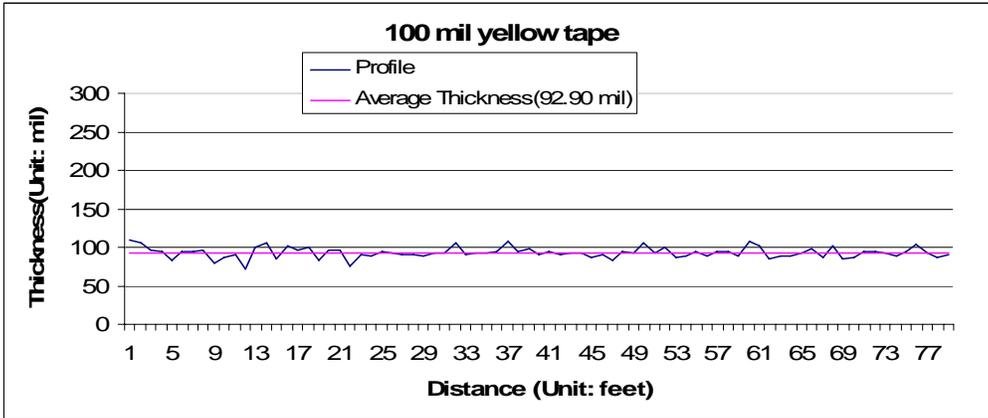
Figure 54 Thickness measurement result for the 100 mil yellow tape.
