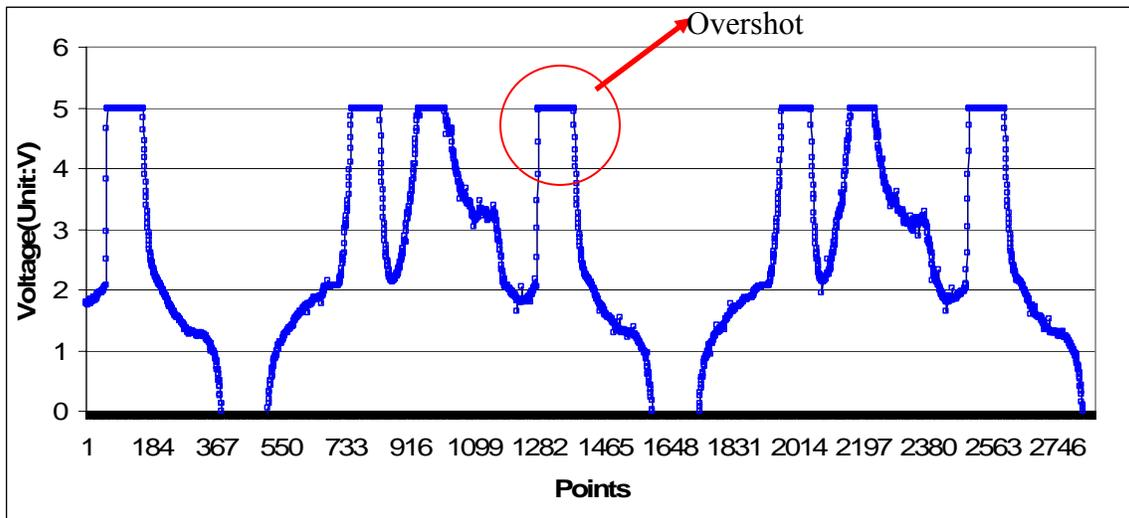
Figure 18 Output electronic signal under sunshine without filter.
