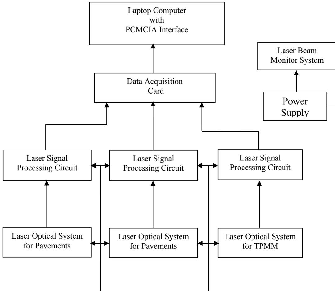
Figure 2 Block diagram of the vehicle-mounted device.
