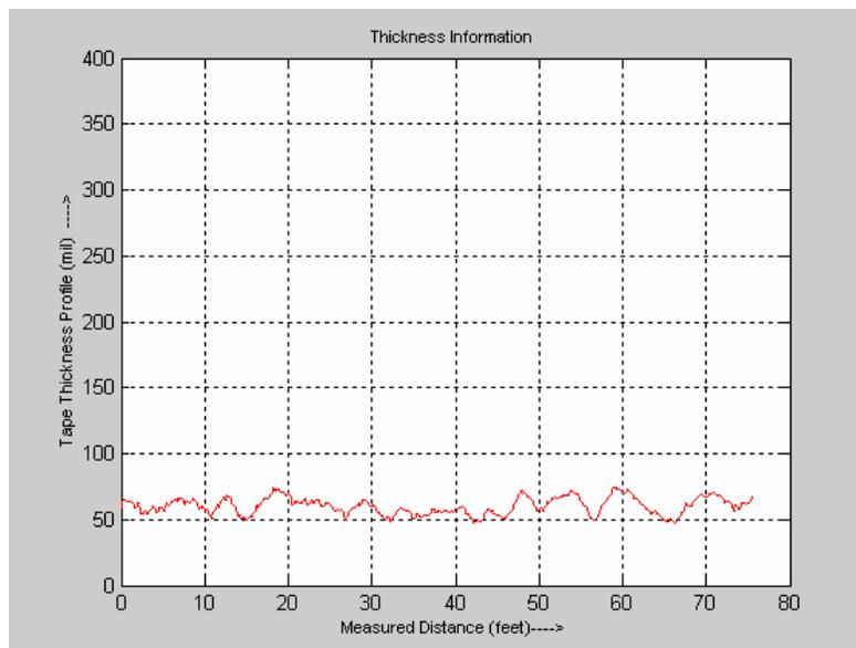
Figure 37 Thickness profile of TPMM (marked with 60 mils).
