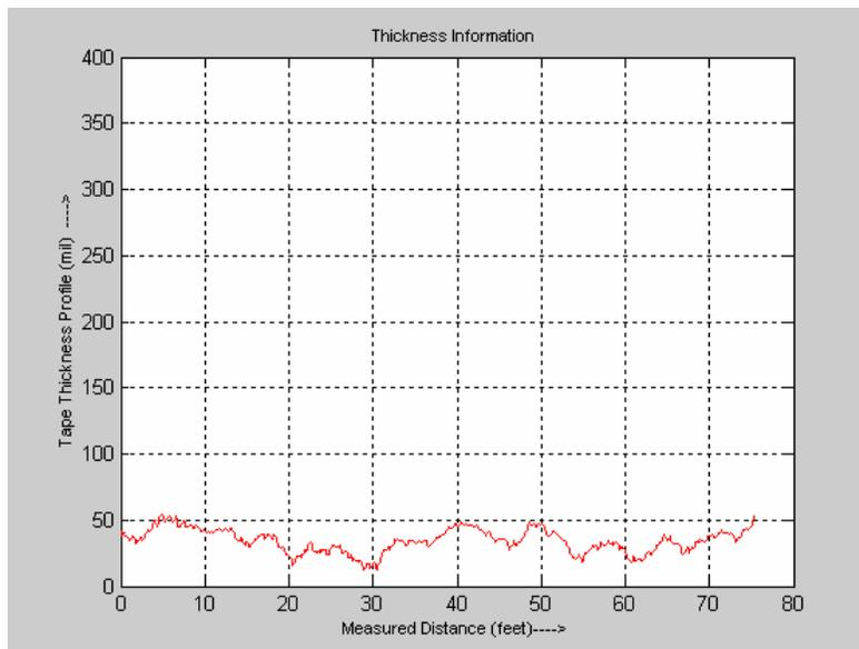
Figure 39 Thickness profile of TPMM (marked with 40 mils).
