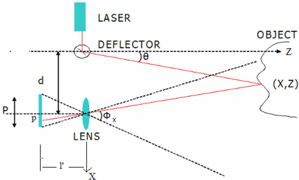
Figure 10 Geometrical principle of laser scanning triangulation.
