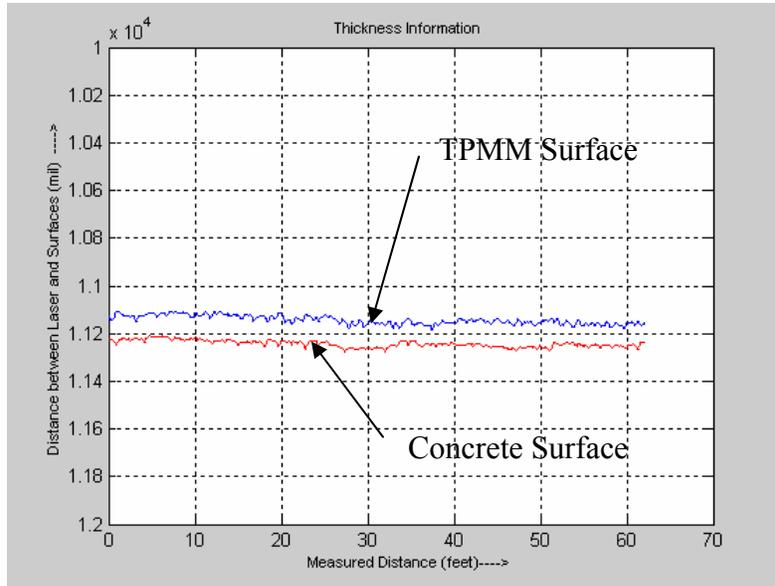
Figure 27 Test results of the TPMM (marked with 100 mils) on highway.
