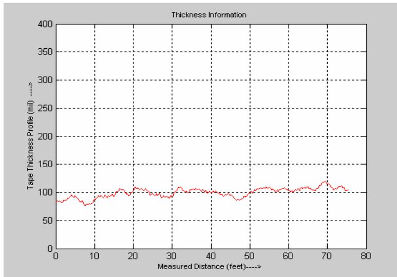
Figure 35 Thickness profile of TPMM (marked with 100 mils).
