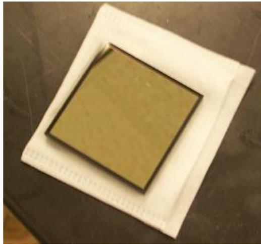
Figure 16 Laser bandpass filter.
