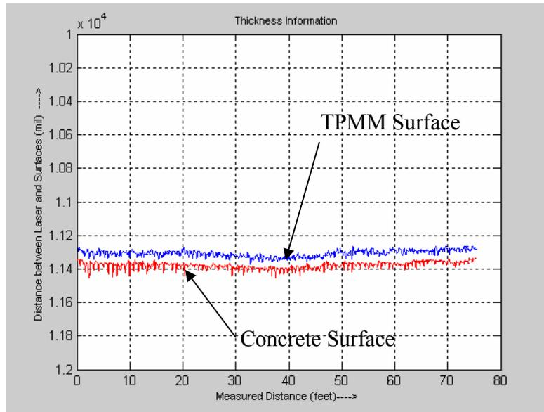
Figure 36 Test results of the TPMM (marked with 60 mils) on highway
