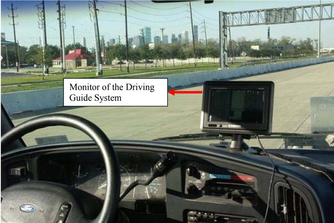
Figure 22 LCD monitor for the driving guide system.
