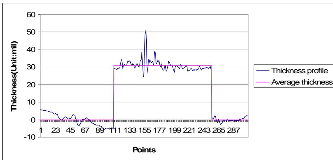
Figure 49 Thickness Profile of the Flex-O-Line thickness of 30 mil tape.
