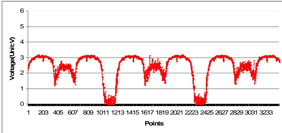
Figure 19 Output electronic signal under sunshine with bandpass filter.
