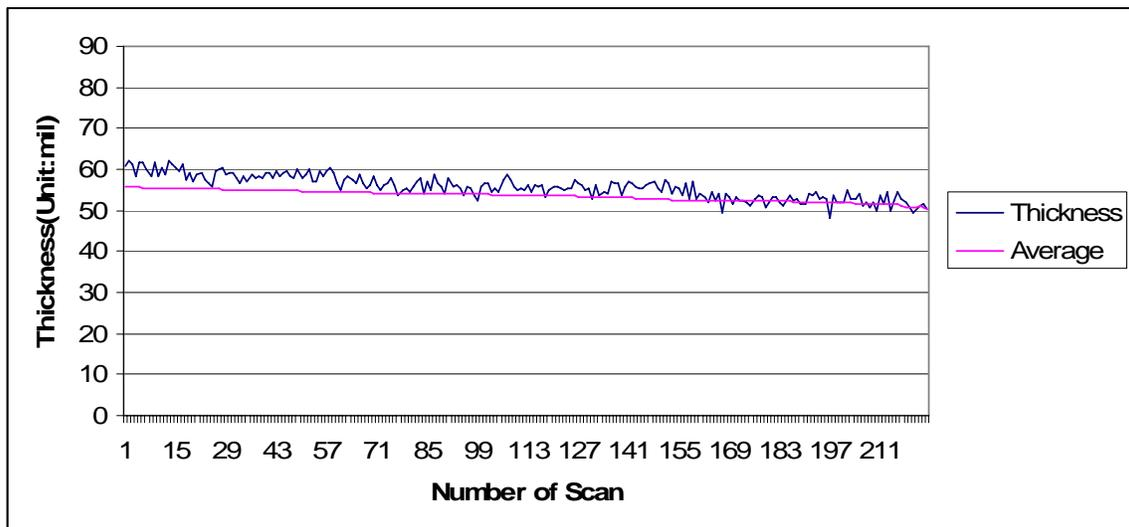
Figure 46 Test result on the 60 mil yellow tape by scanning laser device.
