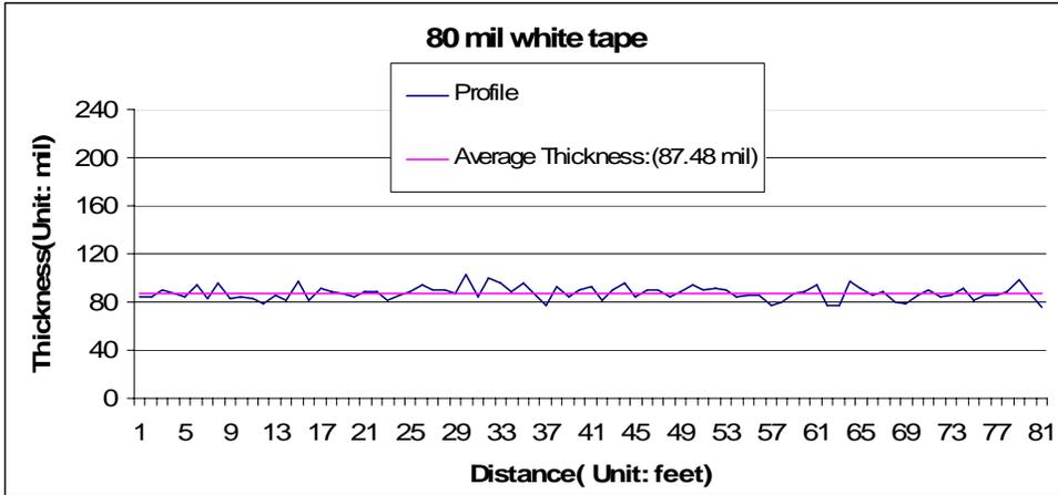
Figure 56 Thickness measurement result of 80 mil white tape.
