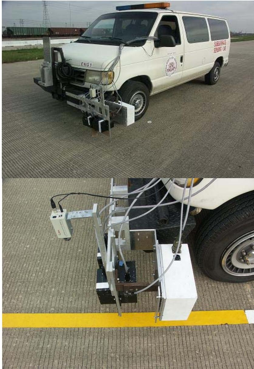
Figure 50 Measurement device mounted on the left side of the vehicle.
