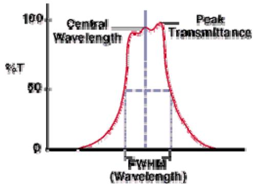
Figure 17 Transmittance chart of the bandpass filter.
