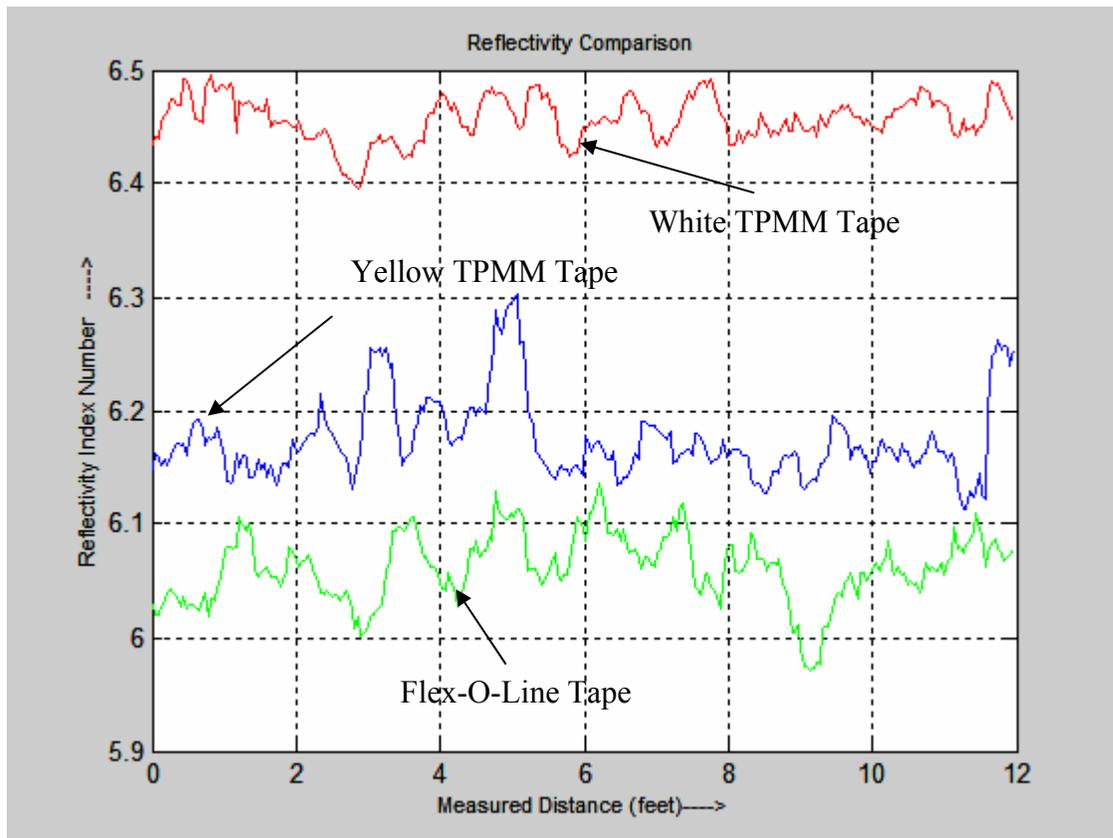
Figure 41 Retroreflectivity comparison of different marking materials.
