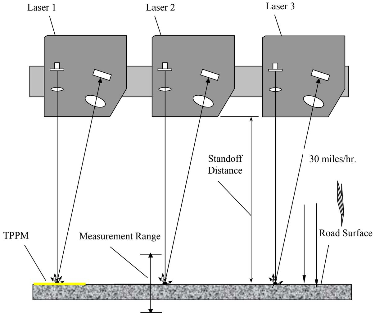
Figure 3 Using three independent laser devices to measure the thickness of TPMM.
