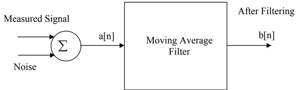
Figure 6 Signal through a moving average filter.
