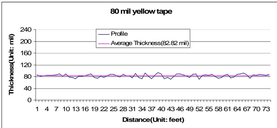
Figure 55 Thickness measurement result for the 80 mil yellow tape.
