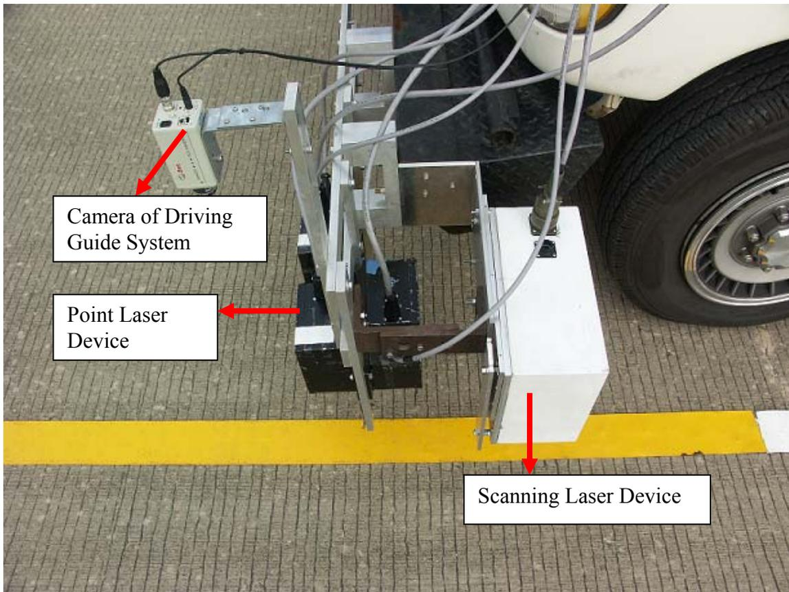
Figure 21 Scanning laser device mounted on the left (driver) side of the vehicle.
