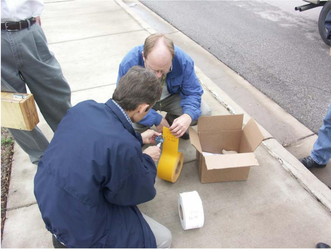
Figure 45 TPMM tape measured by caliper in the field test at Austin.
