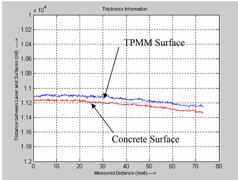
Figure 30 Test results of the TPMM (marked with 60 mils) on highway.
