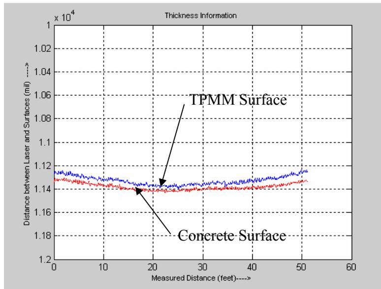
Figure 32 Test results of the TPMM (marked with 40 mils) on highway.
