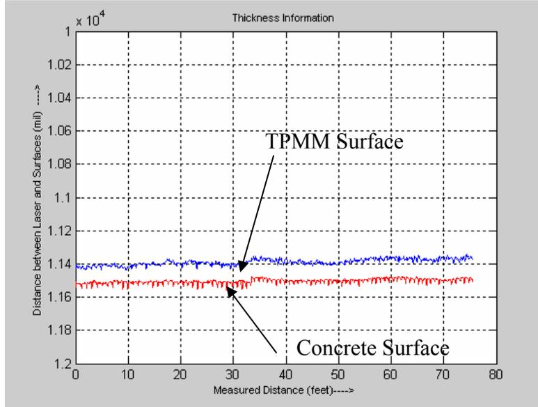
Figure 34 Test results of the TPMM (marked with 100 mils) on highway.
