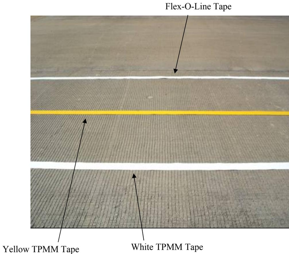
Figure 40 Retroreflectivity experiment setup.
