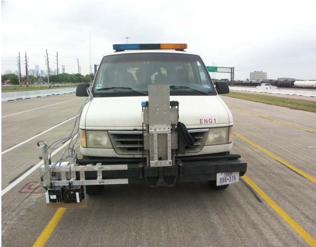
Figure 25 Point laser device mounted on the right (passenger) side.
