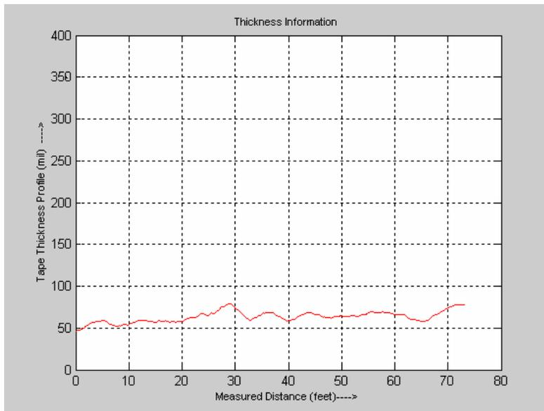
Figure 31 Thickness profile of TPMM (marked with 60 mils).
