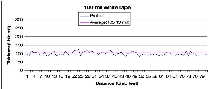
Figure 51 Thickness measurement result of 100 mil white tape.
