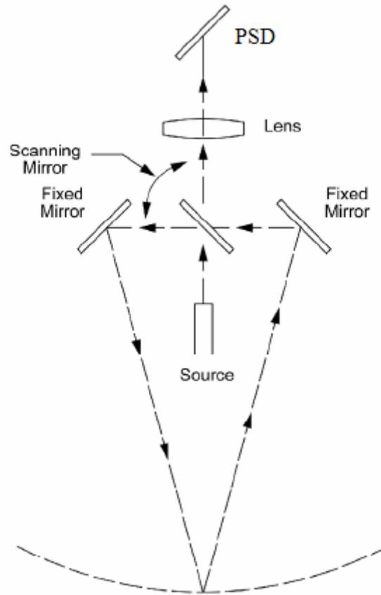
Figure 12 Optical configuration of auto-synchronized laser scanning.
