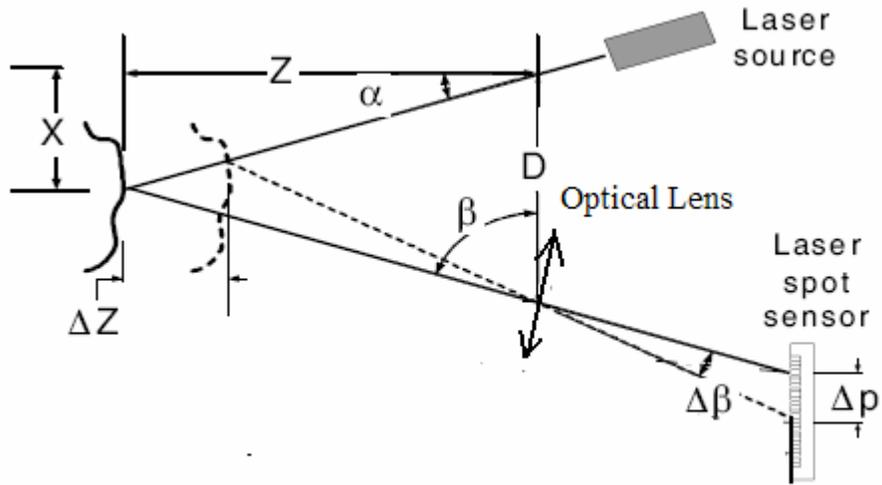
Figure 9 Geometrical principle of triangulation.
