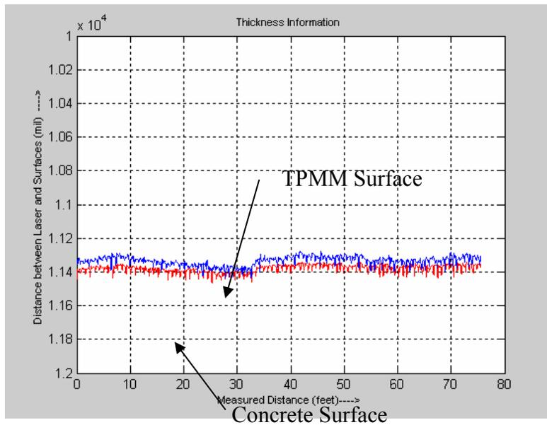
Figure 38 Test results of the TPMM (marked with 40 mils) on highway.
