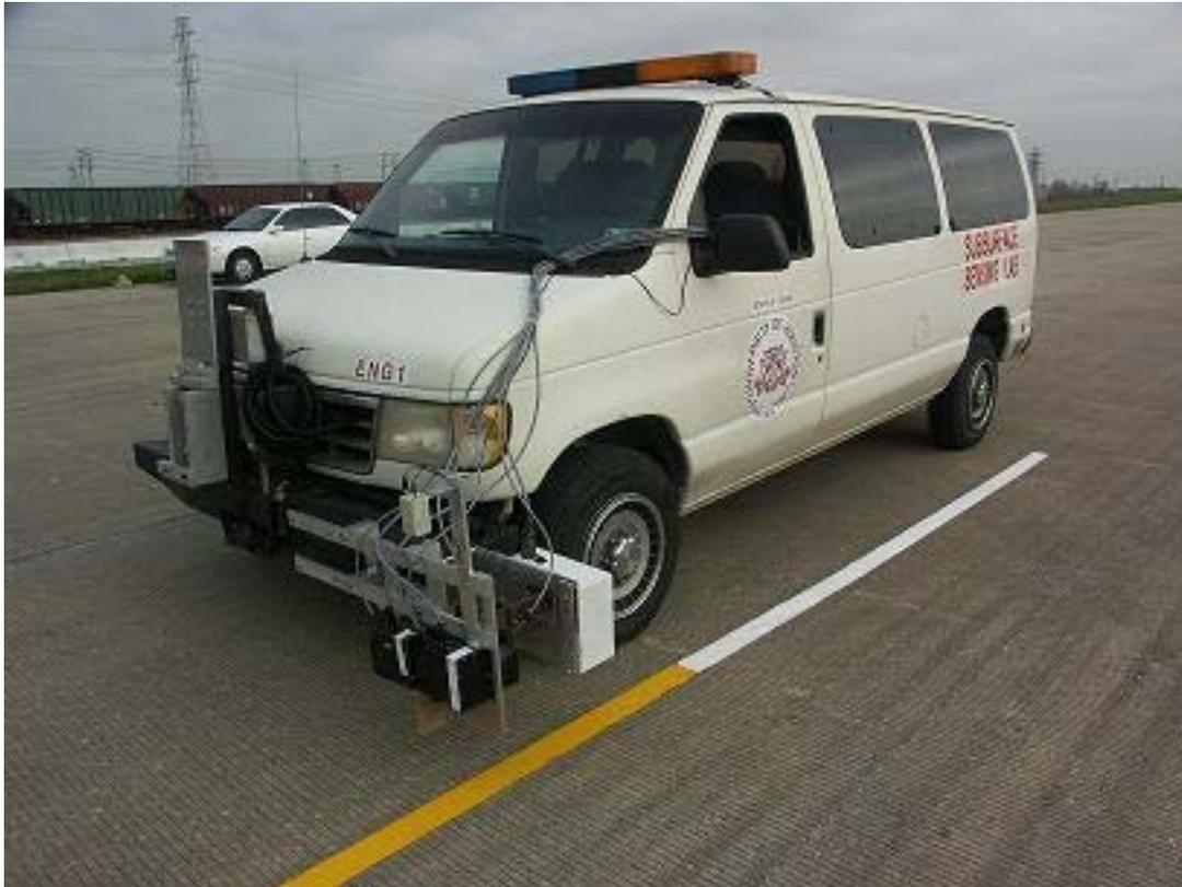
Figure 47 Field test of laser scanning device on spur 5.
