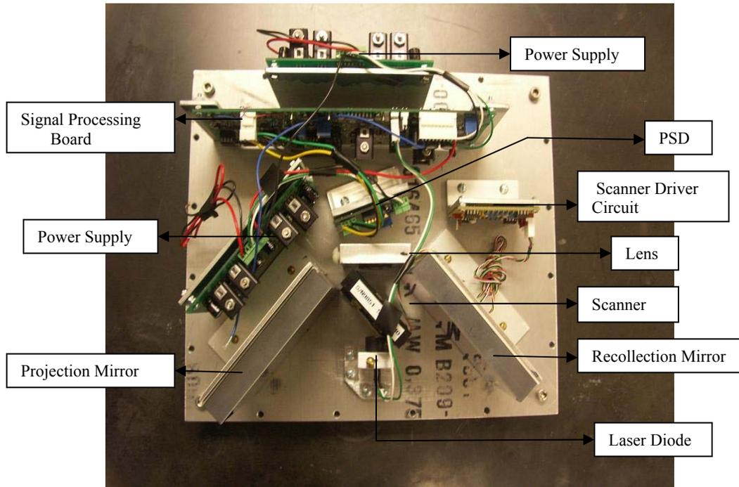
Figure 15 Internal structure of the scanning laser device.
