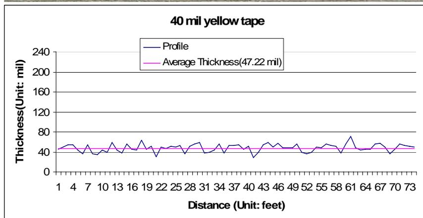
Figure 52 Thickness measurement result of 40 mil yellow tape.
