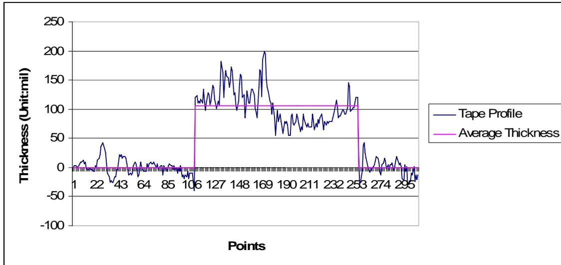
Figure 48 Thickness Profile of the 100 mil Thickness Tape.
