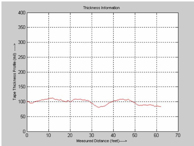
Figure 28 Thickness profile of TPMM (marked with 100 mils).
