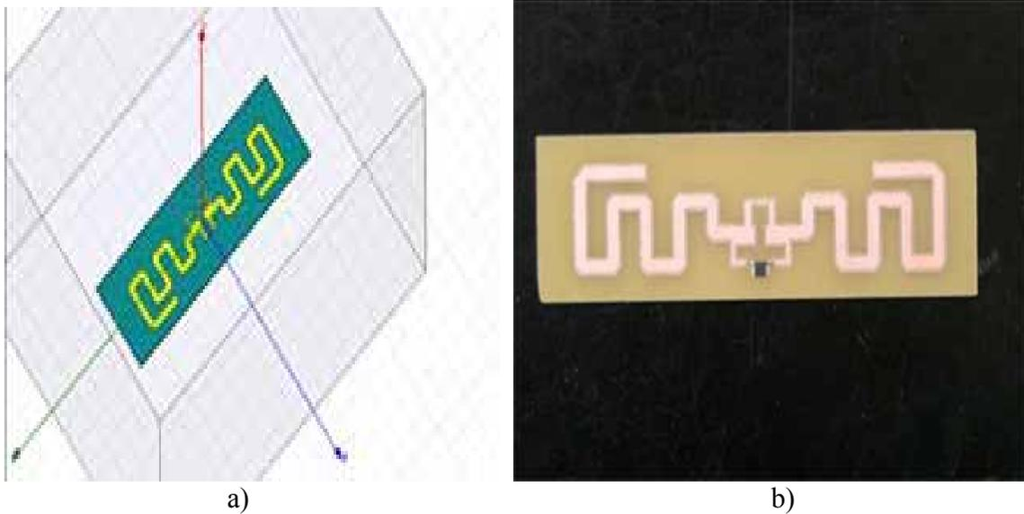
Fig 2-3 Meander Dipole Antenna for Passive RFID Tag: a) HFSS Simulation Model; b) RFID Prototype
