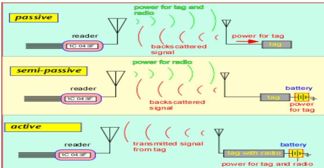
Fig 1-2 Principles of Active, Semi-passive and Passive RFID
