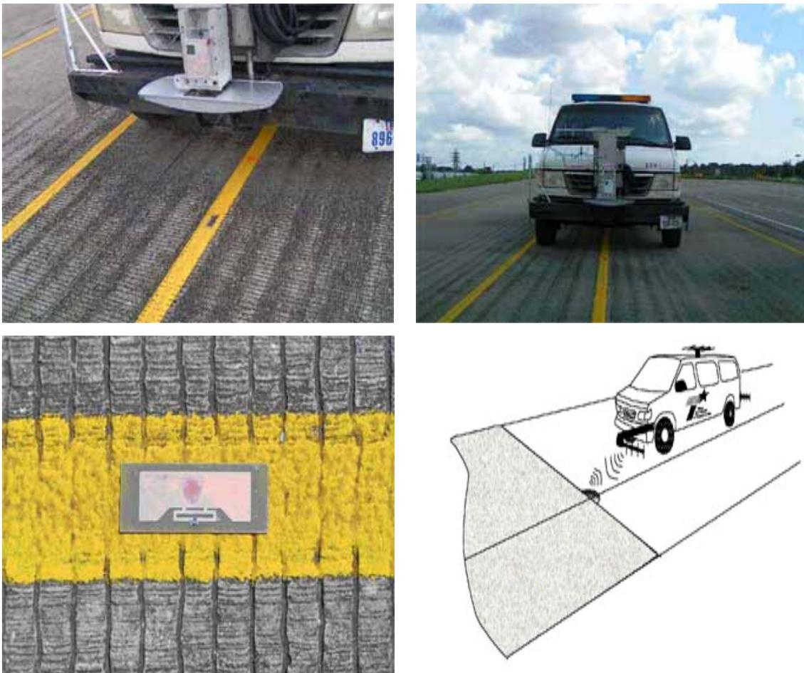
Fig 5-1 RFID For Highway Surface Mount Application
