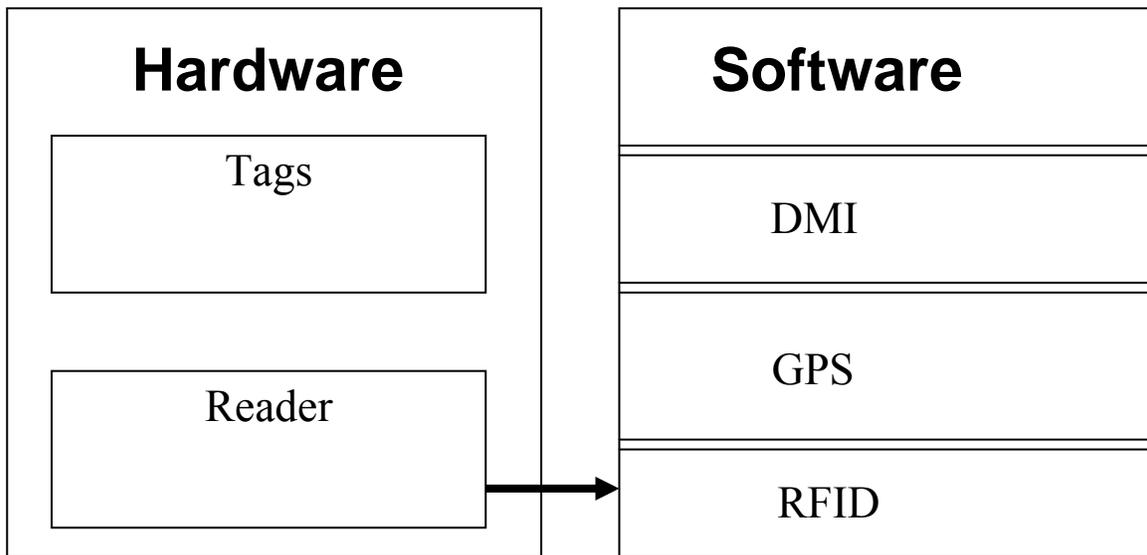
Fig 1-3 Highway Reference Marker Locating RFID System
