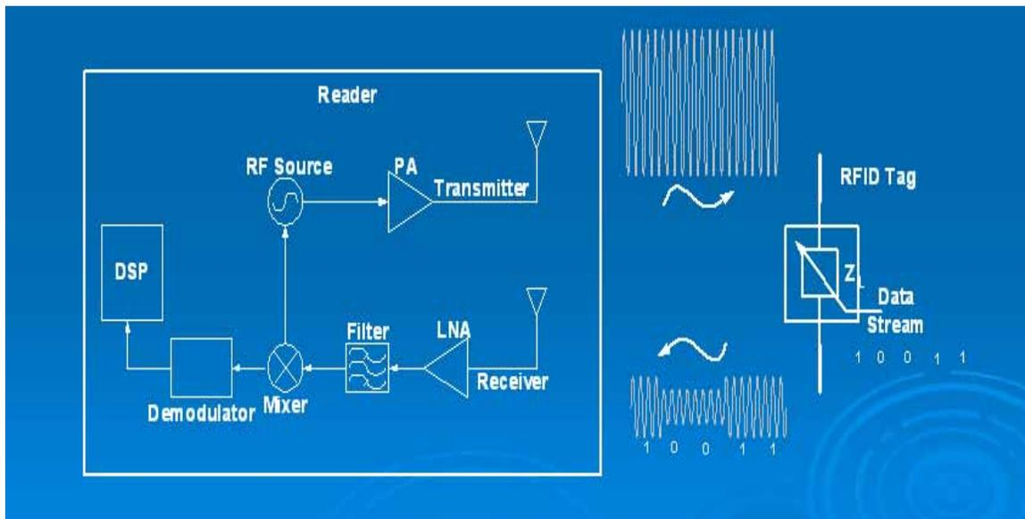
Figure 2-1 Block Diagram of Backscattering RFID System
