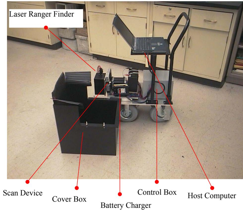
Figure 2.3 TPMM measurement system components
