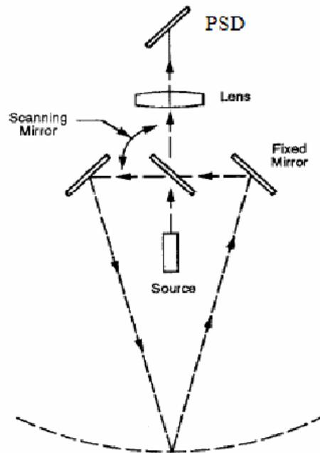
Figure 4.3 Basic principle of the longitudinal auto-synchronization technique using a double-sided coated mirror [5]
