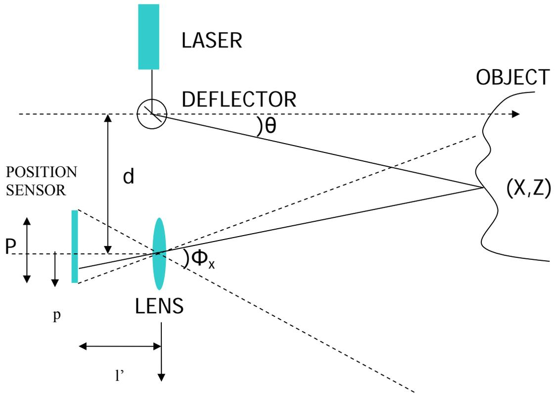
Figure 4.1 Classical laser triangulation methods
