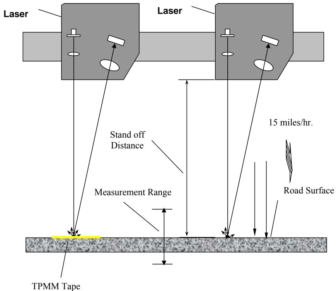
Figure 3.1 Two synchronized laser devices used to the TPMM thickness
