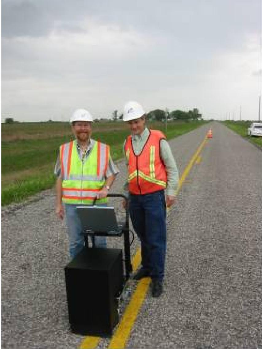
Figure 2.7 TPMM thickness pushcart in field test
