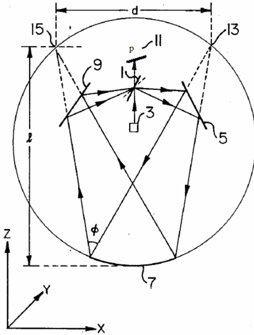
Figure 4.4 A single point on the position sensor defines a surface in the object space [6]
