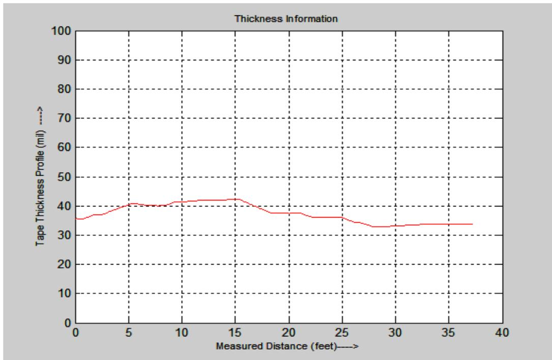
Figure 6.10. Measured FLEX\_O\_LINE thickness of 30 mils tape by mobile device
