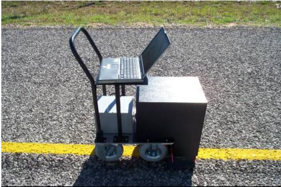
Figure 1.1 New version of pushcart TPMM thickness measurement system
