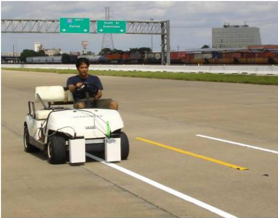
Figure 1.2 Vehicle-mount TPMM thickness measurement system
