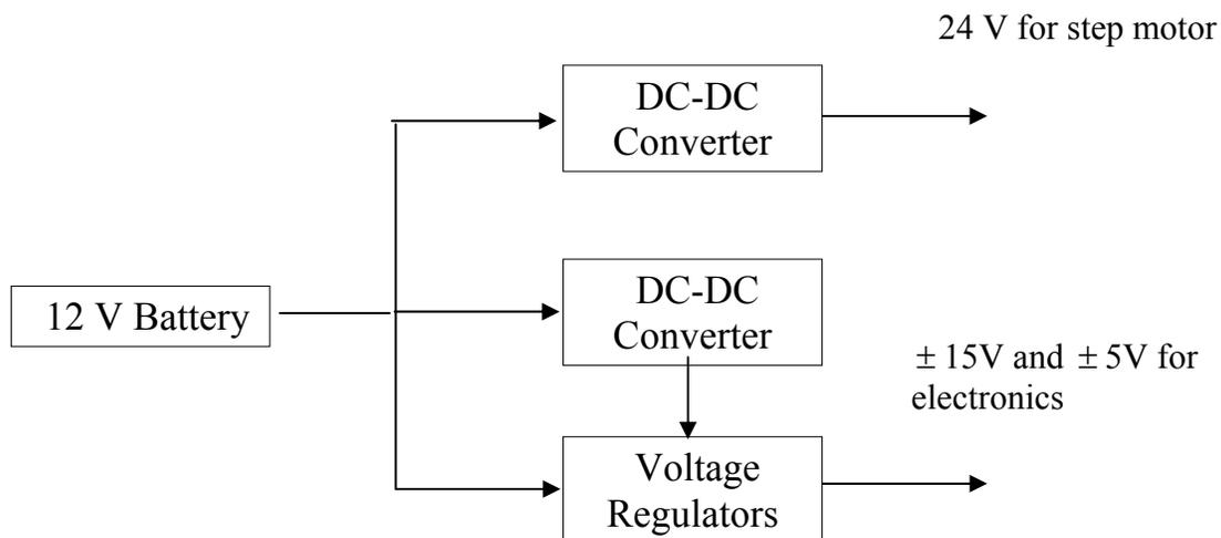
Figure 2.6 Block diagram of power supply system
