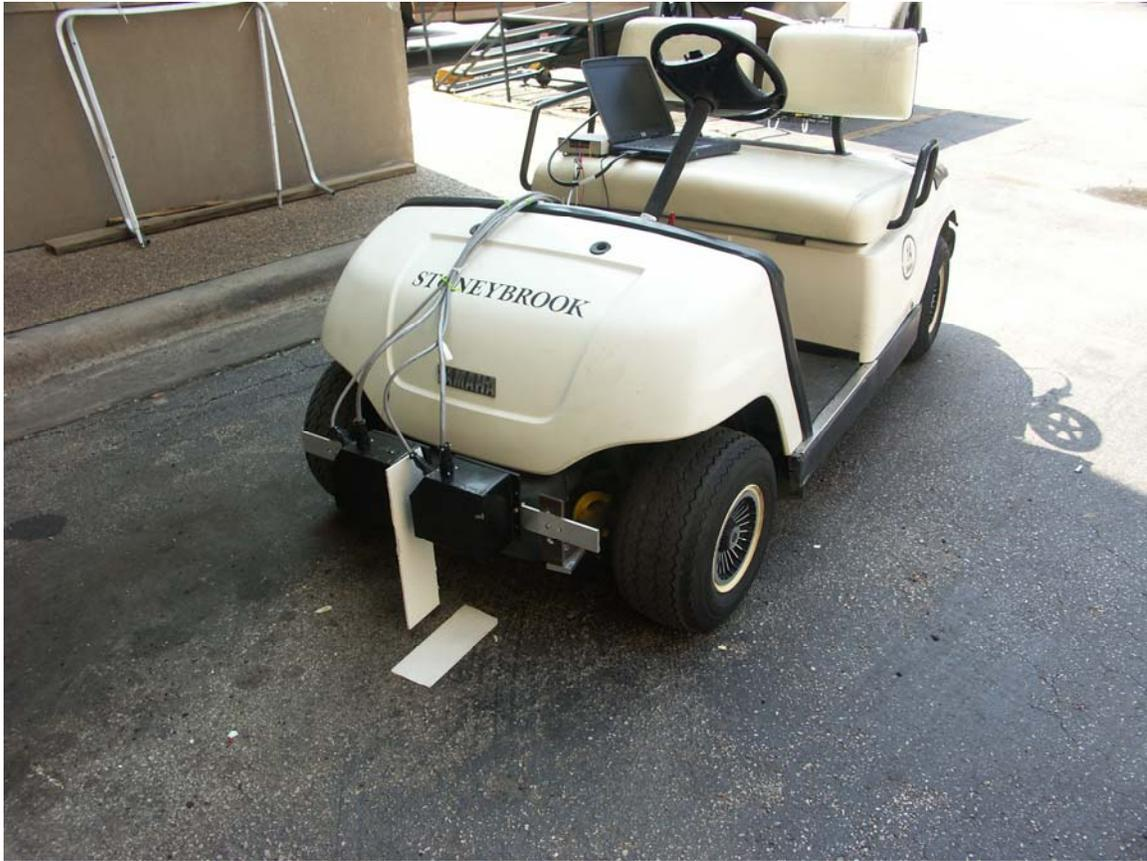
Figure 3.2 Measurement on pavement surface by using golf cart version
