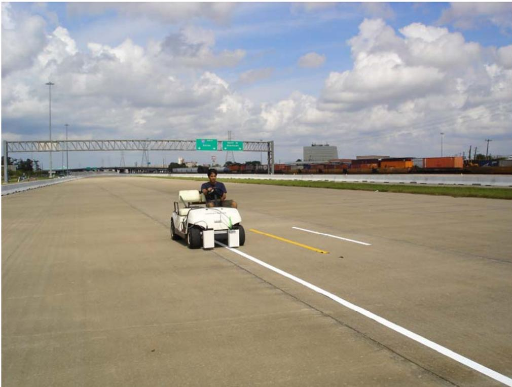
Figure 6.8. Field tests of the vehicle mount TPMM tape thickness measurement device
