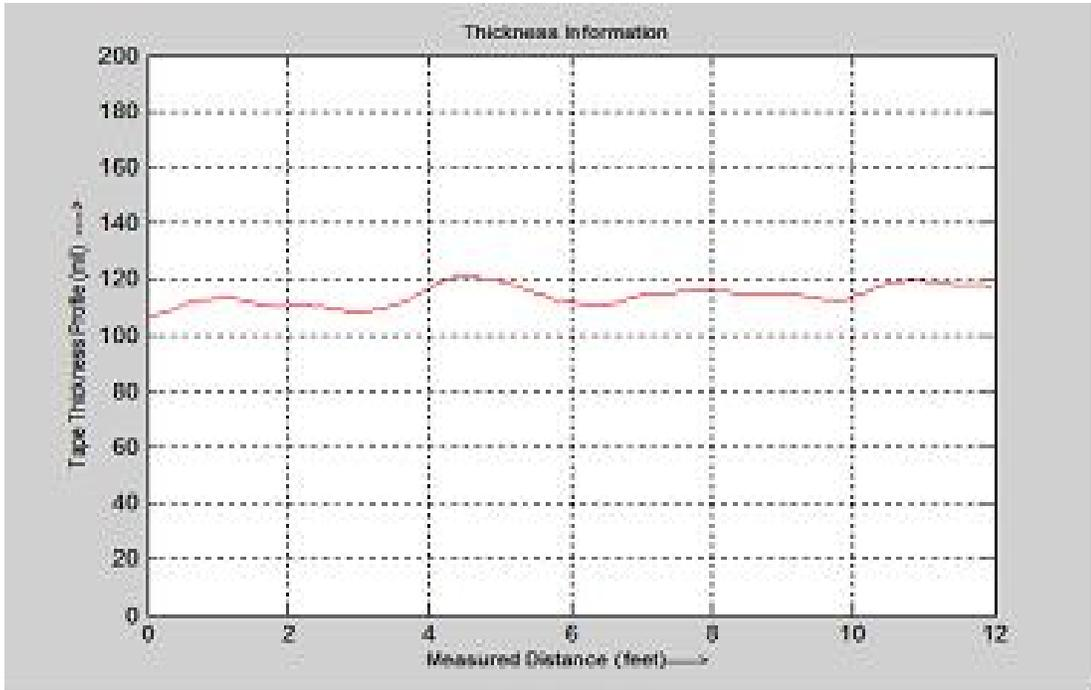
Figure 6.9. Measured TPMM thickness of 100 mils yellow tape by mobile device
