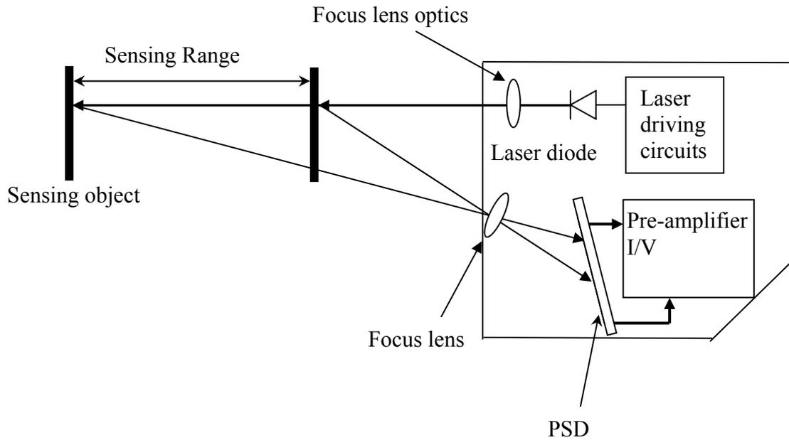
Figure 2.4 Laser-based triangulation optical system
