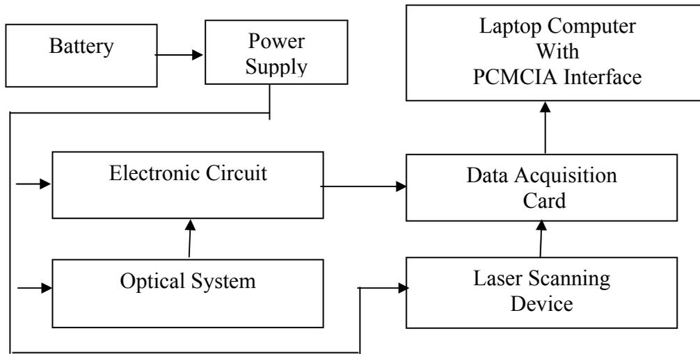
Figure 2.2 Block diagram of hardware system
