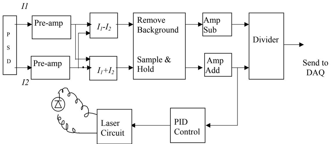
Figure 2.5 Block diagram of signal processing circuit
