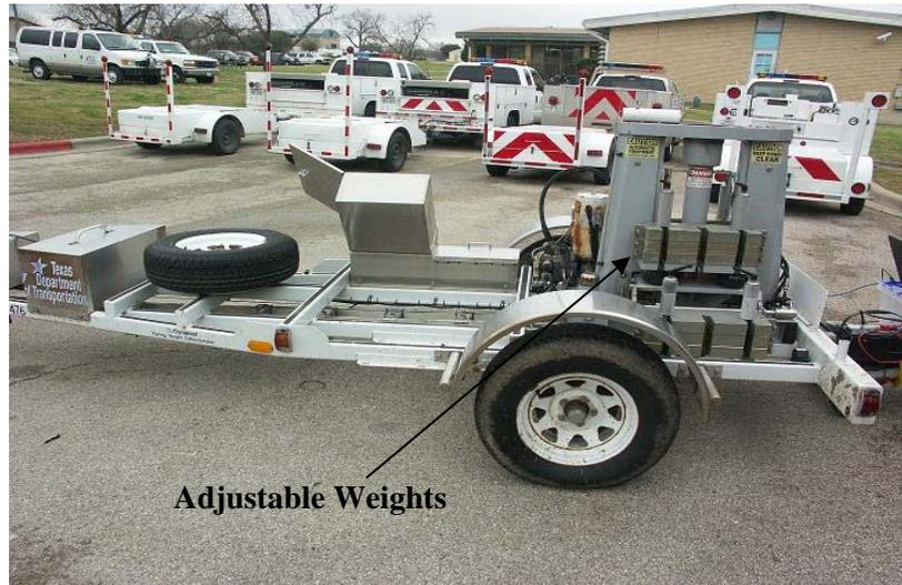
**Figure 2-1 Falling weight deflectometer**
