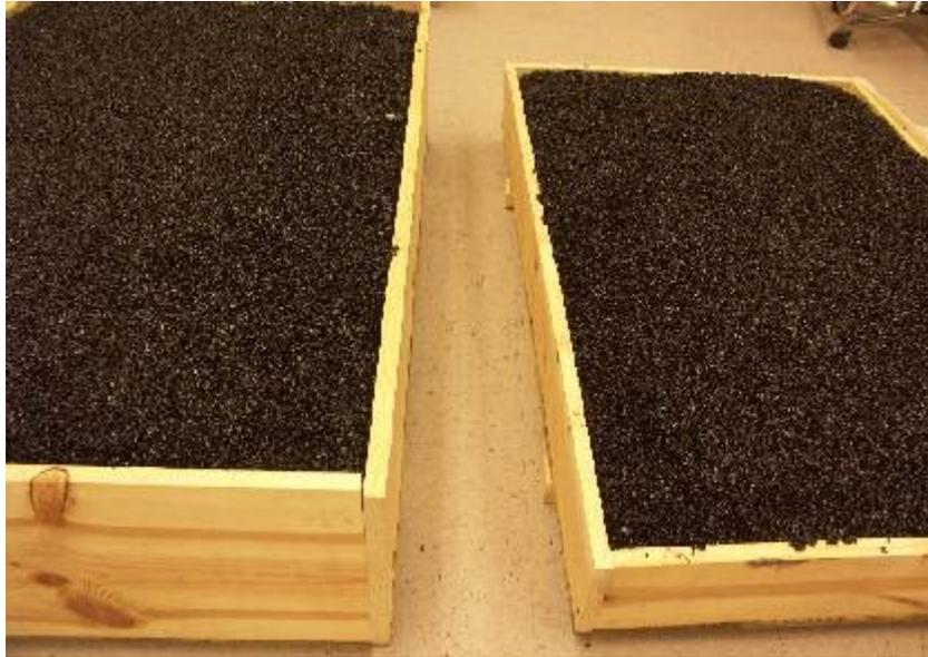
**Figure 4-1 Asphalt slabs for lab experiment**
