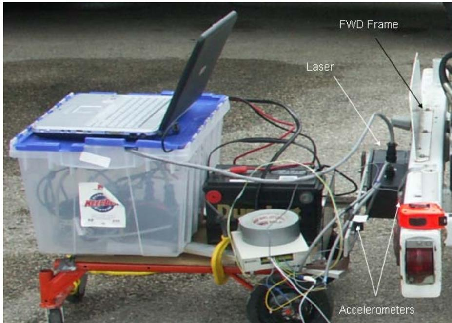
**Figure 2-6 Laser device setup**
