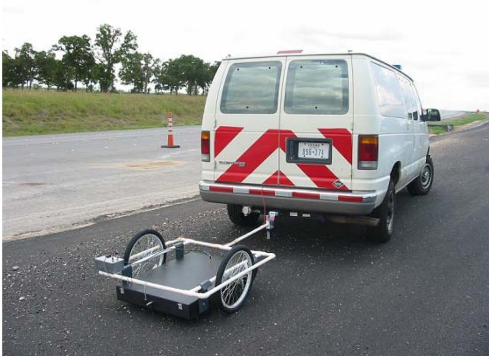
**Figure 3-2 Pushcart version of the pulse GPR**
