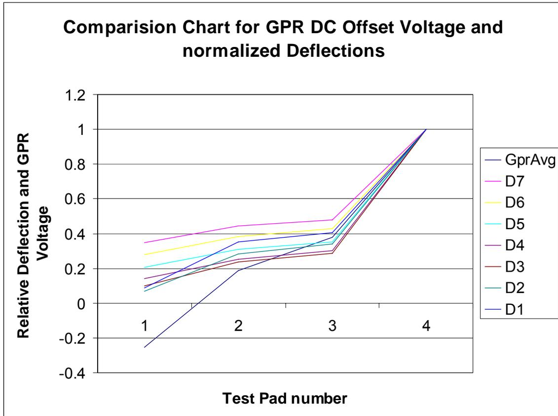
**Fig. 3-19 Correlation between GPR data and FWD data**
