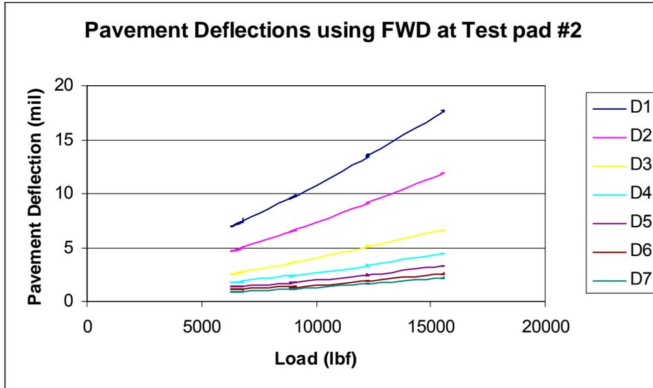
**Fig. 3-13 Pavement deflection data obtained with the FWD at pad 2**
