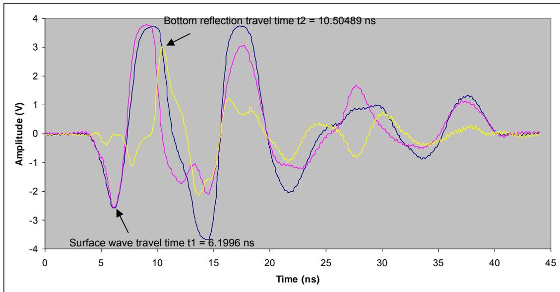
**Fig. 3-8 Test 3 of the pulse GPR, slab thickness being pressed to 10.75 Inch**
