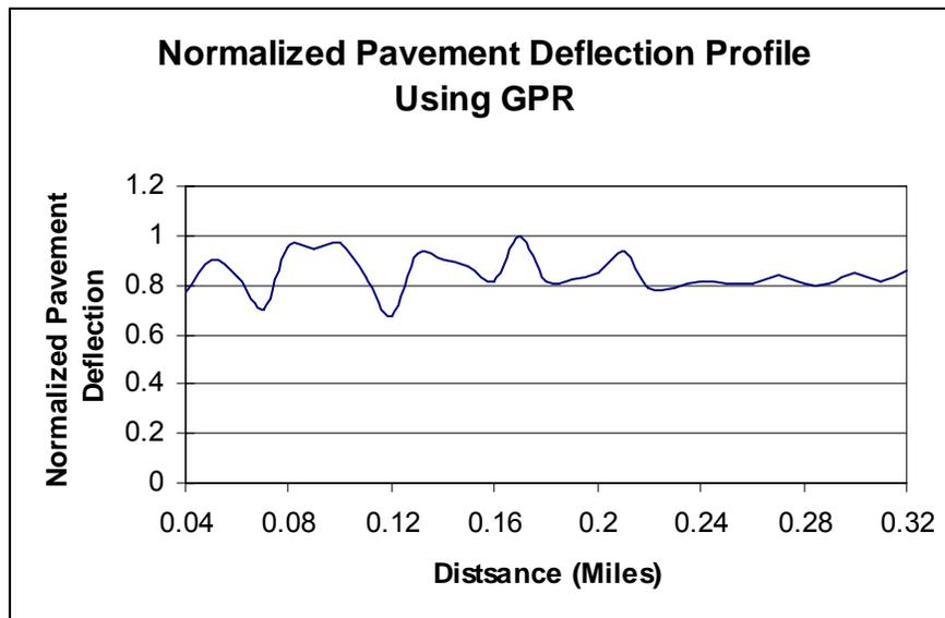
Fig. 3-24 Pavement deflections calculated using GPR
