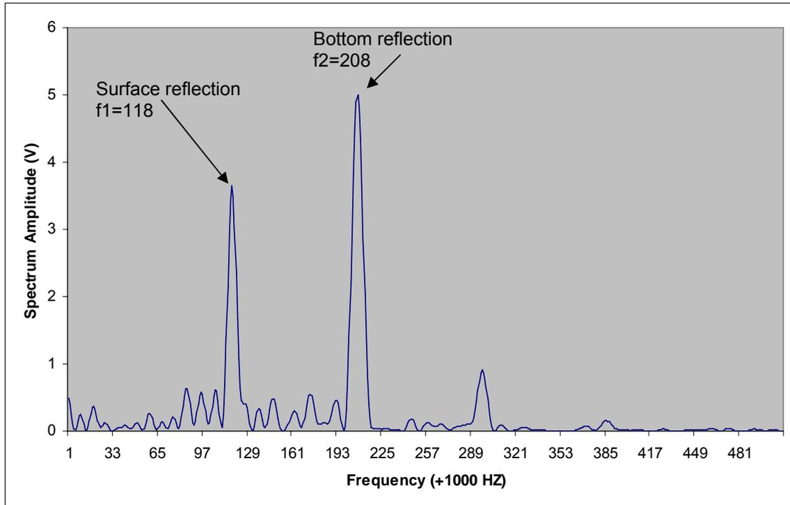
**Fig. 3-7 Test 3 of the FMCW radar, slab thickness being pressed to 10.75 Inch**
