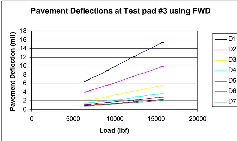
Fig. 3-15 Pavement deflection data obtained with the FWD at pad 3
