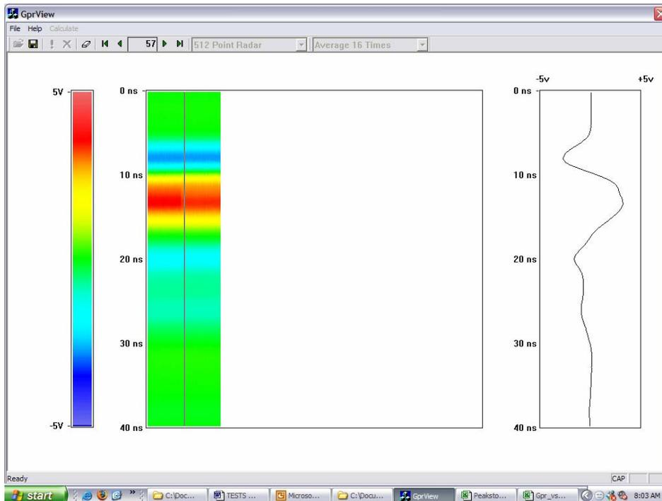
Fig. 3-12 GPR trace color-map obtained at pad 2
