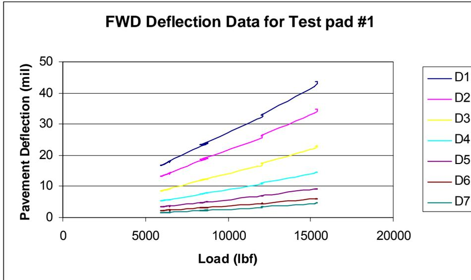
Fig. 3-11 Pavement deflection data obtained with the FWD at pad 1
