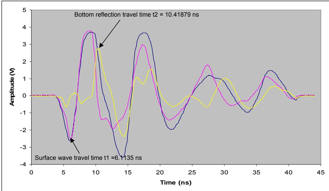
**Fig. 3-6 Test 2 of the pulse GPR, slab thickness being pressed to 11 Inch**
