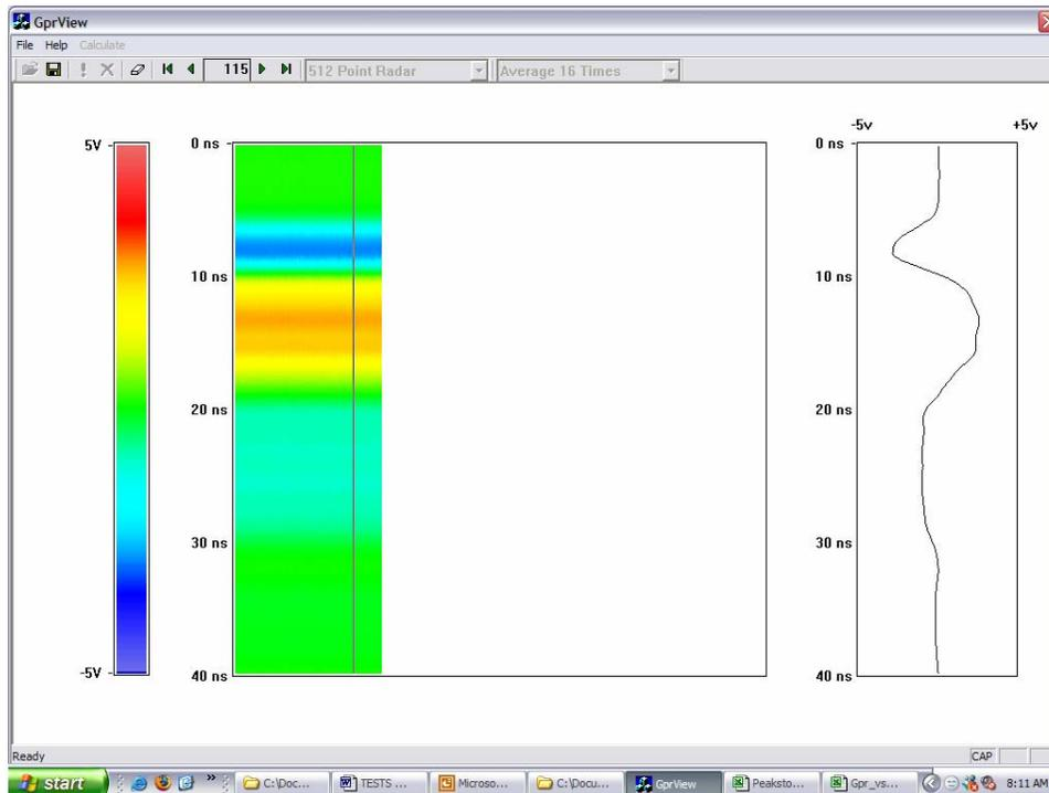
**Fig. 3-14 GPR trace color-map obtained at pad 3**
