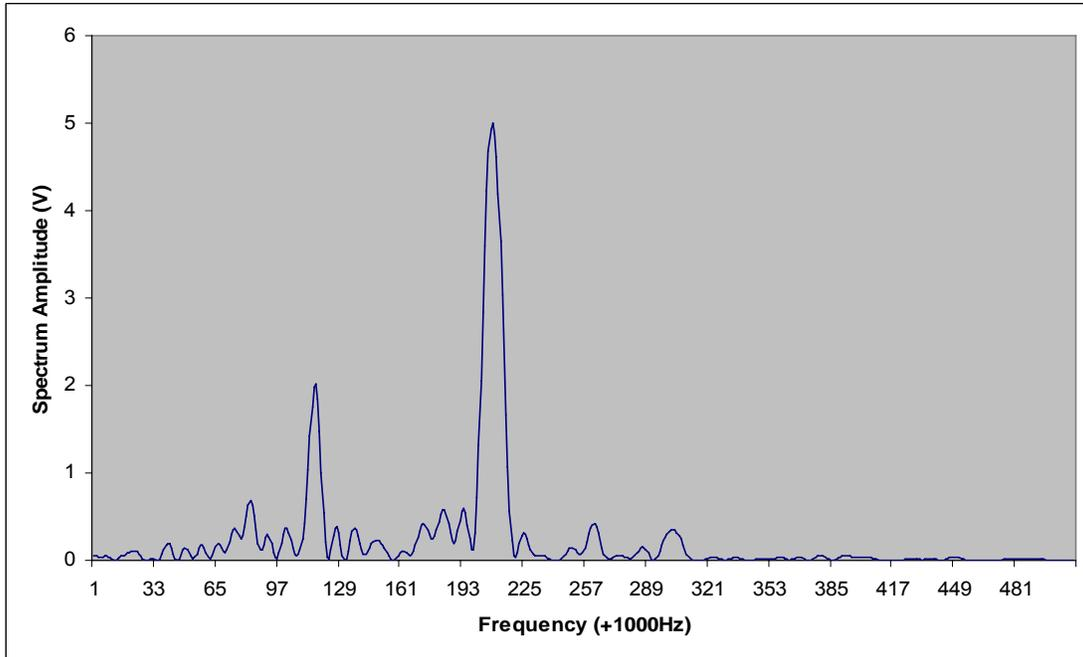
**Fig. 3-3 Test 1 using the FMCW radar, slab thickness 11.5 Inch**
