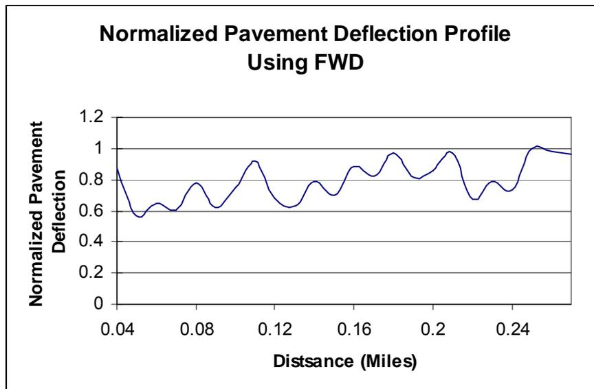
**Fig. 3-25 Normalized pavement deflections using FWD**
