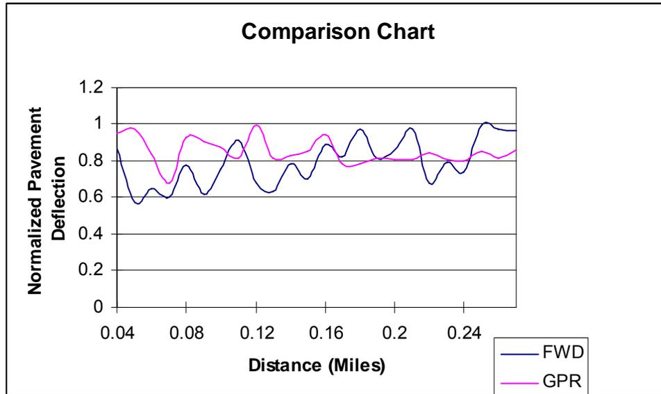
**Fig. 3-26 Comparison between results obtained using the GPR and the FWD**
