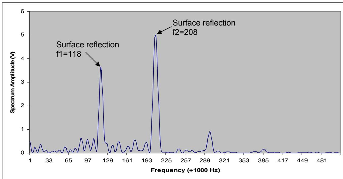
**Fig. 3-5 Test 2 of the FMCW radar, slab thickness being pressed to 11 Inch**
