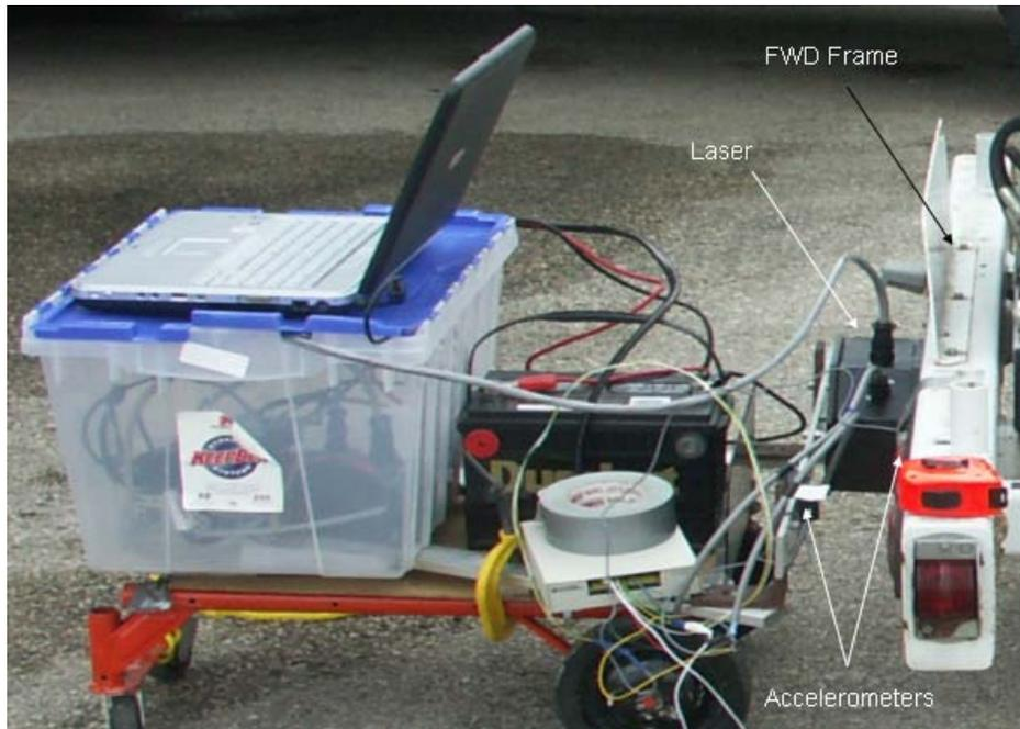
**Fig. 2-2 Laser device setup**
