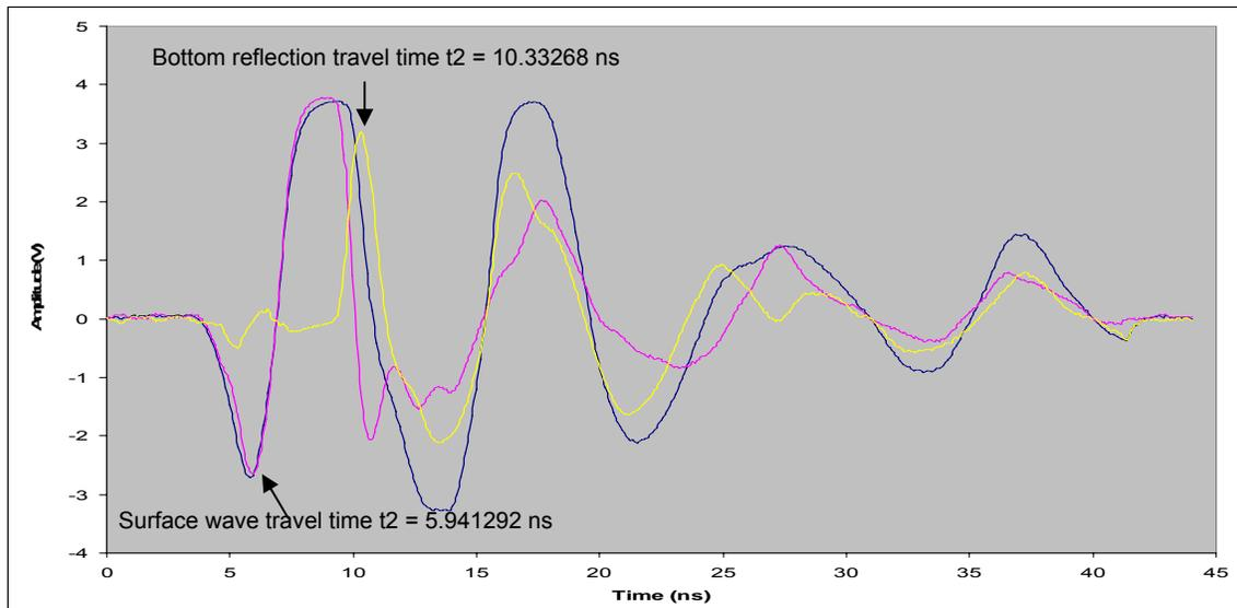
**Fig. 3-4 Test 1 using the pulse GPR, slab thickness 11.5 Inch**
