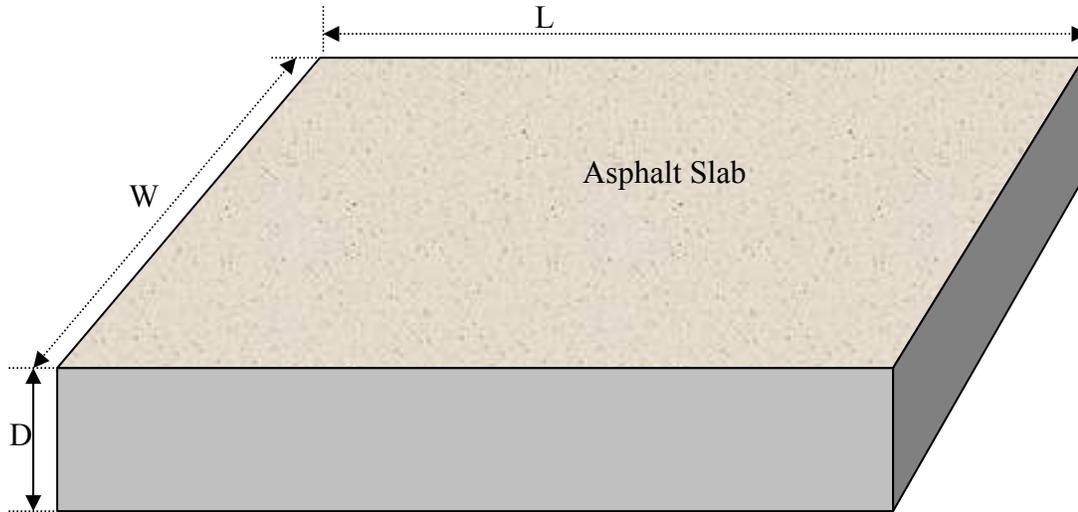
**Fig. 3-2 Asphalt slab in the lab, where  $L = 64$  Inch and  $W = 30.75$  Inch**
