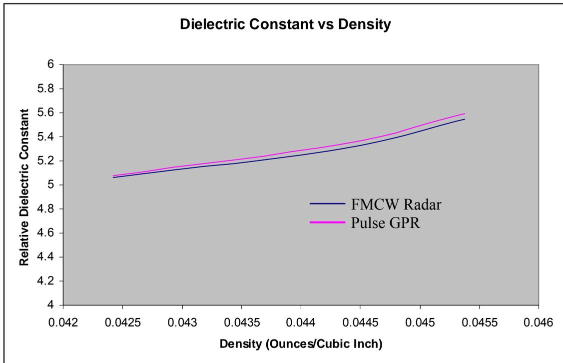
**Fig. 3-9 The relation between dielectric constant and density of asphalt material**
