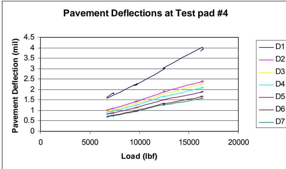
**Fig. 3-17 Pavement deflection data obtained with the FWD at pad 4**
