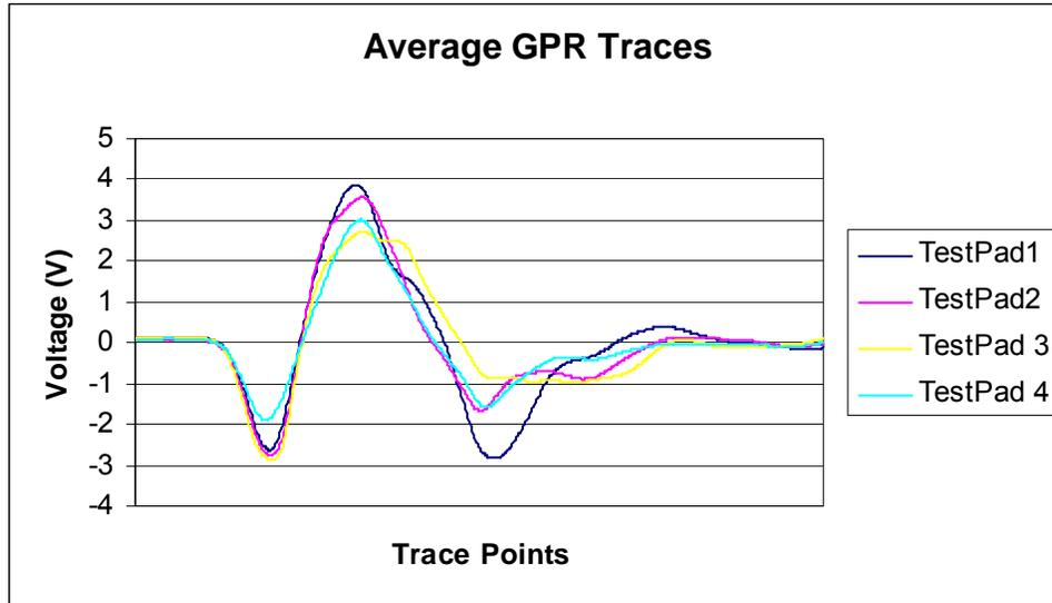
**Fig. 3-18 Average GPR traces for all test pads**
