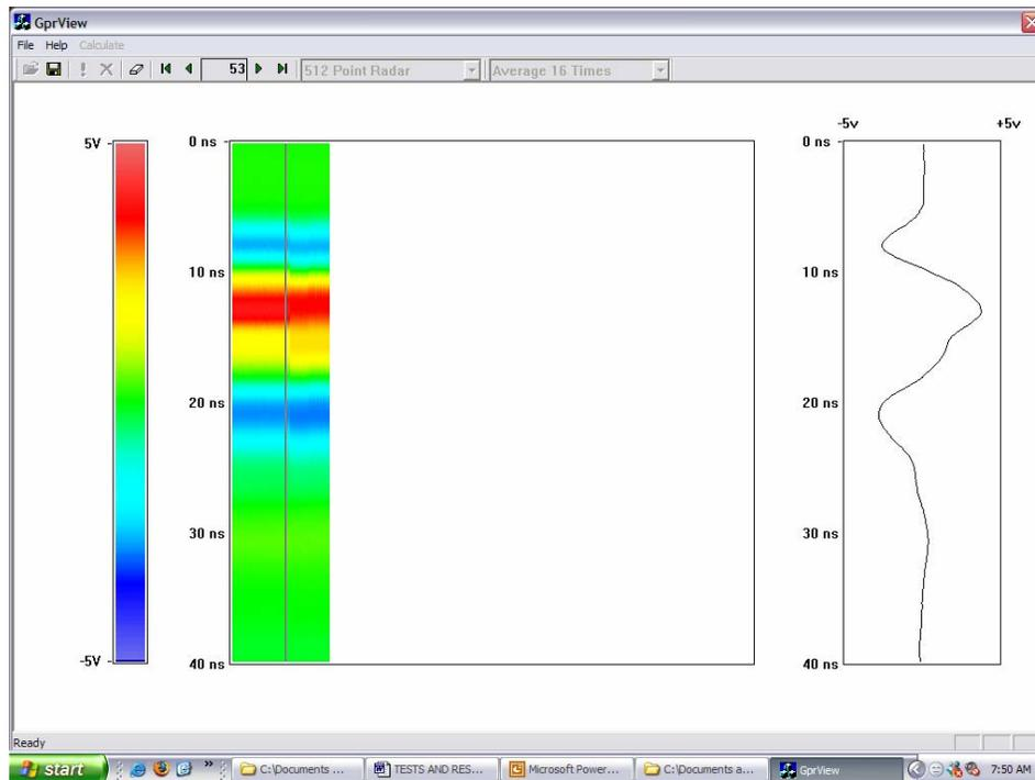
Fig. 3-10 GPR trace color-map obtained at pad 1
