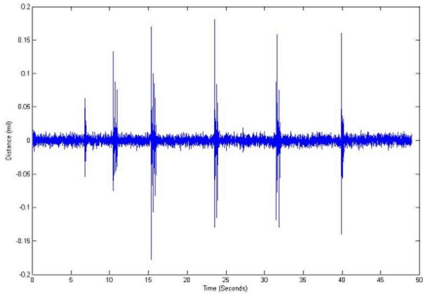
**Fig. 2-4 Frame vibrations measured by accelerometer**
