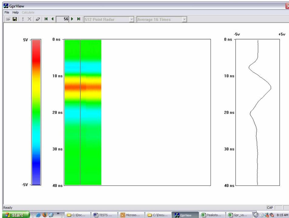
Fig. 3-16 GPR trace color-map obtained at pad 4
