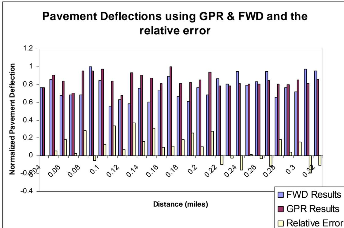
**Fig. 3-27 Pavement deflection results with relative error**
