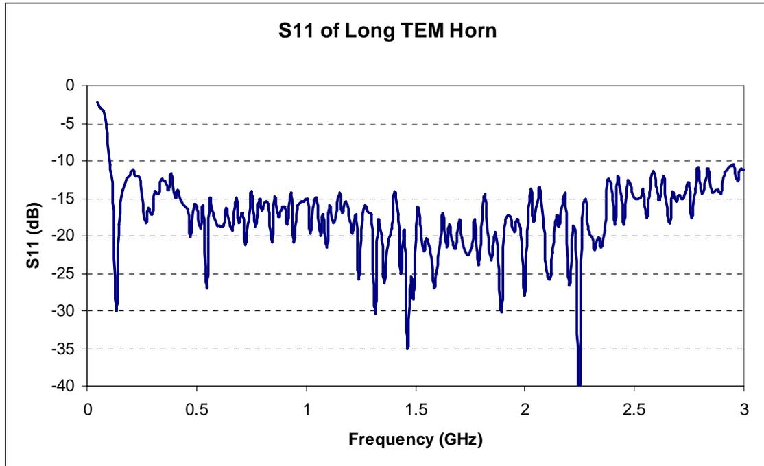
Fig. 2-4 Measured S11 of the developed TEM Horn antenna
