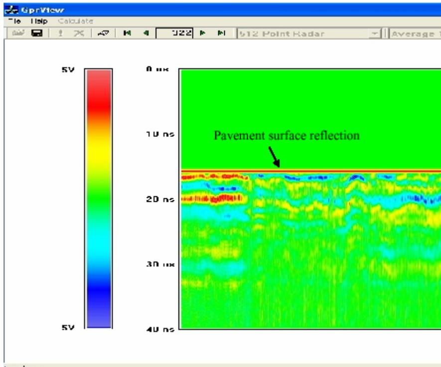
Fig. 3-3 The measured color map of Fig. 3-1 after signal processing
