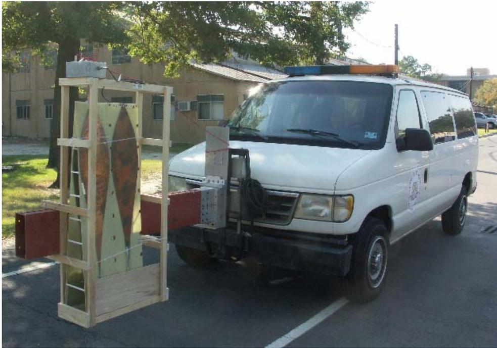
Fig. 2-5 Air-coupled version of the pulse GPR
