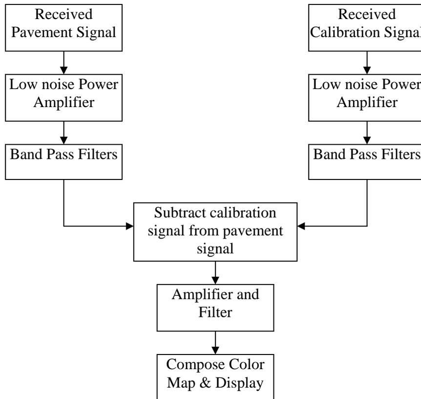
Fig. 3-2 Data processing procedures for air-coupled GPR
