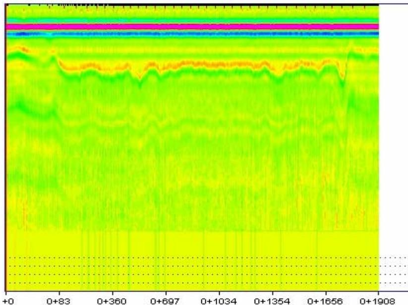
Fig. 4-1 Measured color map at TTI Annex by Air-coupled GPR
