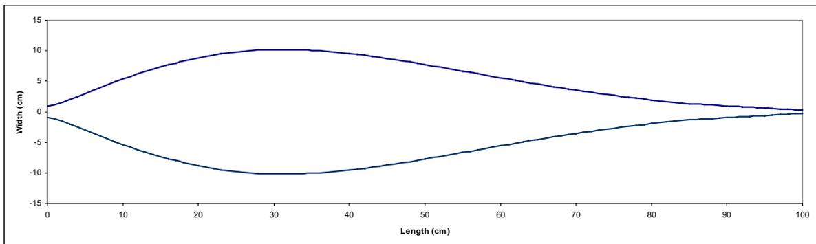
Fig. 2-3 Dimensions of the antenna plate
