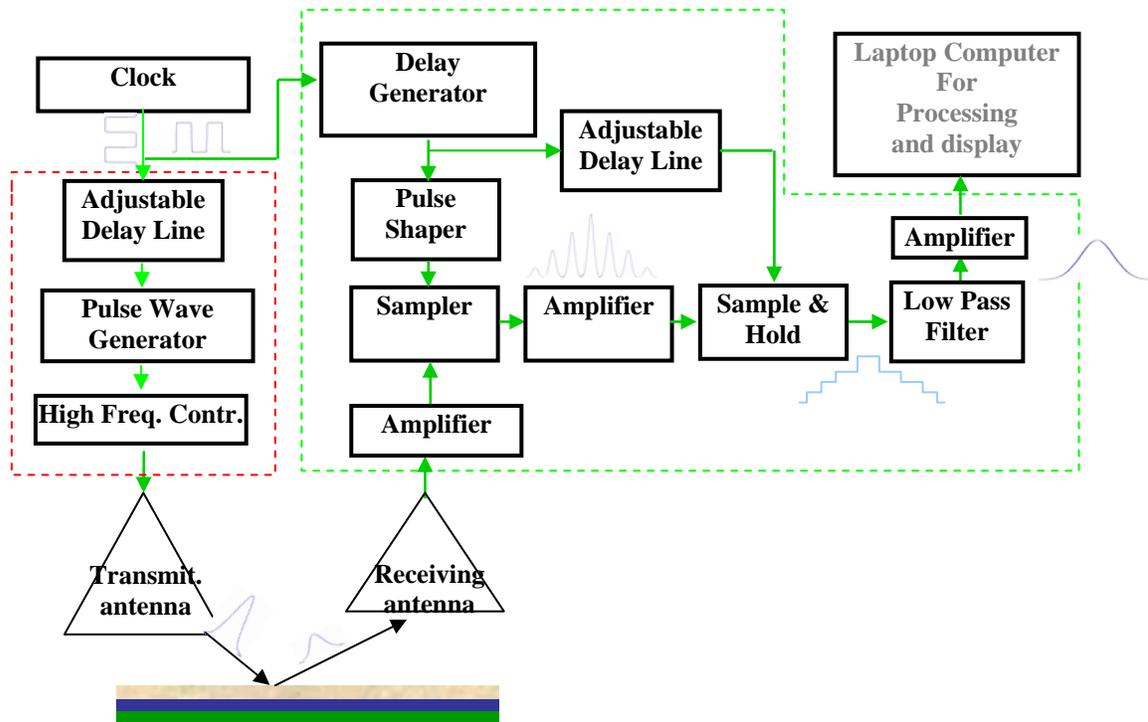
**Fig. 2-1 Block diagram of the pulse GPR system**
