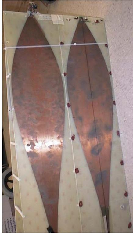
Fig. 2-2 two TEM horn antennas
