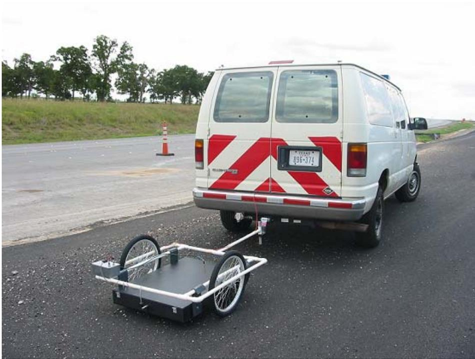
Fig. 2-8 Ground-coupled version of the pulse GPR
