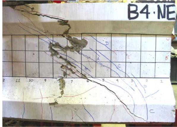
(b) Shear Failure of Beam B4-North End
