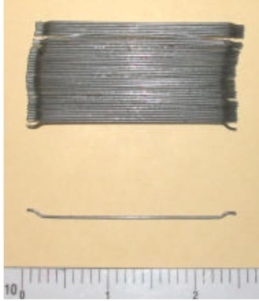
**Fig. 2.5.1 Steel Fiber RC80/60BN**
