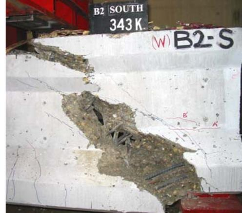
(b) Shear Failure of Beam B2-South End
