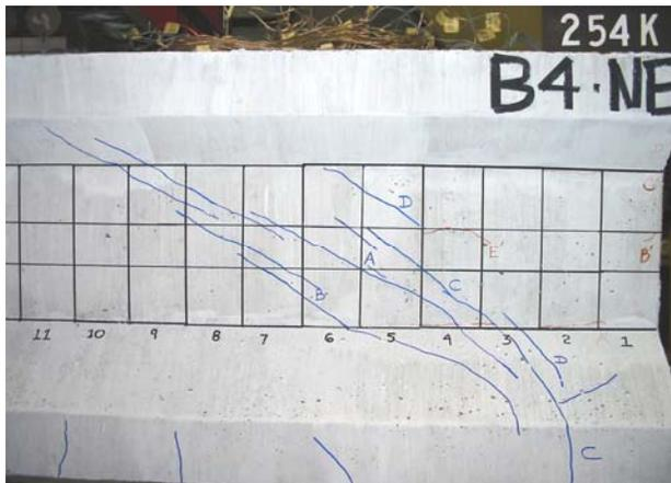
(a) Cracking of Beam B4-South End
