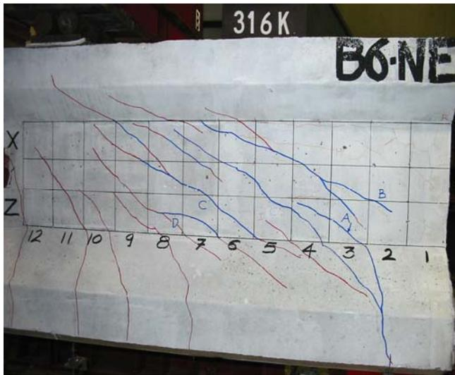
(a) Cracking of Beam B6-North End
