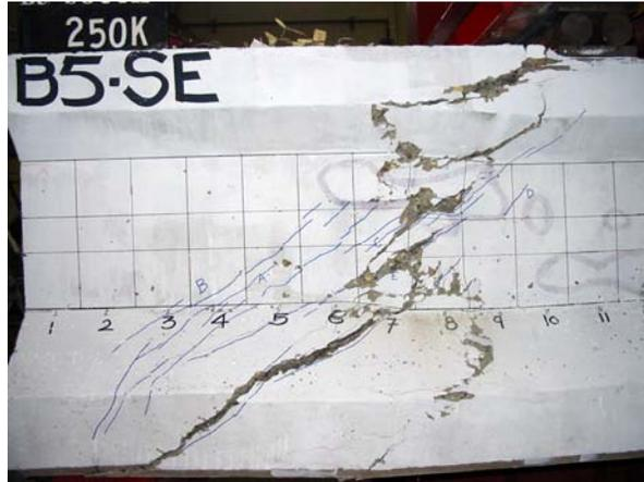
(b) Shear Failure of Beam B5-South End
