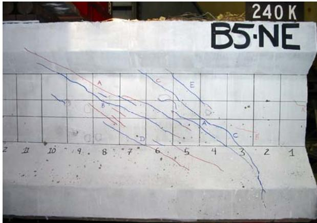
(a) Cracking of Beam B5-North End
