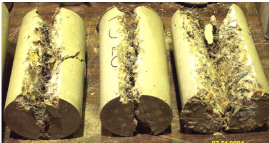
**Fig. 2.9.2 Split Cylinder Test Specimens**
