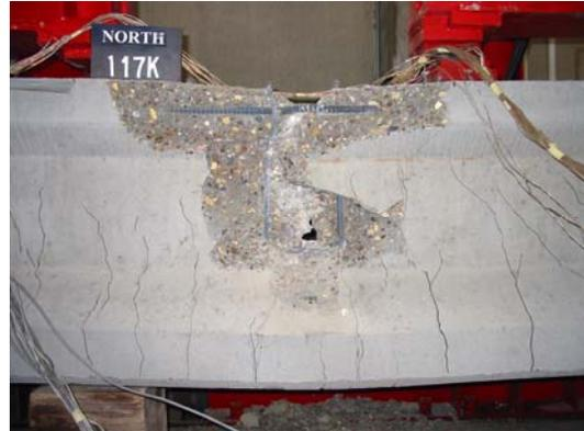
(b) Flexure Failure of Beam B1-North End
