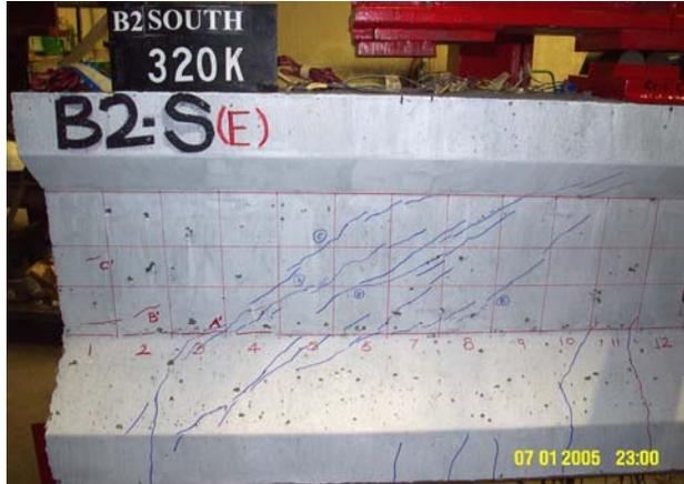
(a) Cracking of Beam B2-South End
