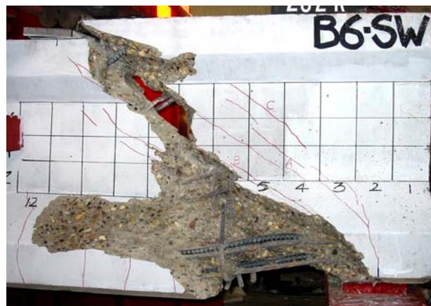
(b) Shear Failure of Beam B6-South End
