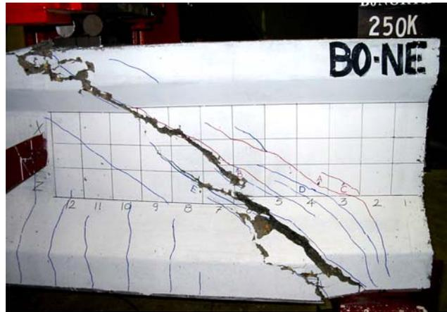
(b) Shear Failure of Beam B0-North End
