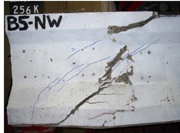
(b) Shear Failure of Beam B5-North End
