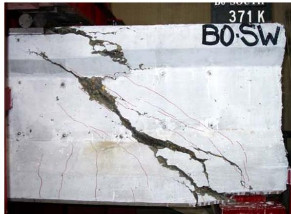
(b) Shear Failure of Beam B0-South End
