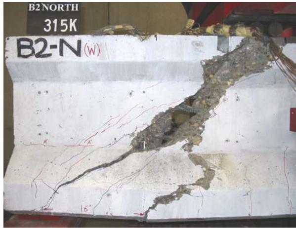
(b) Shear Failure of Beam B2-North End
