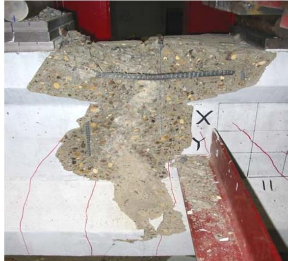
(b) Flexure Failure of Beam B6-North End
