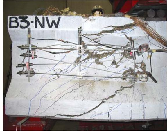
(b) Shear Failure of Beam B3-North End
