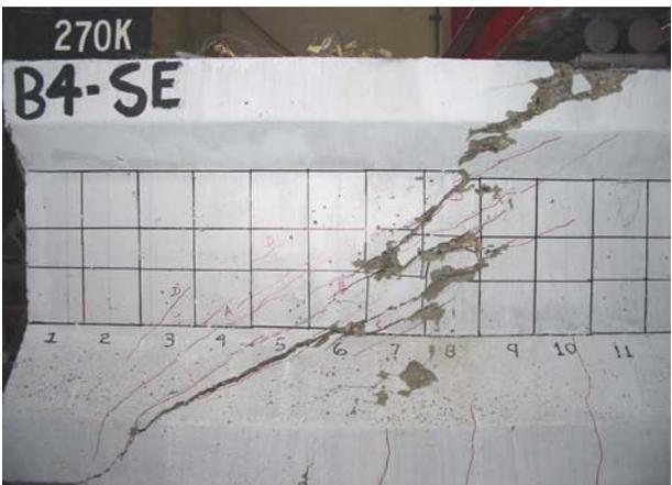
(b) Shear Failure of Beam B4-South End
