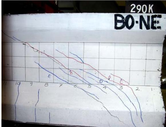
(a) Cracking of Beam B0-North End
