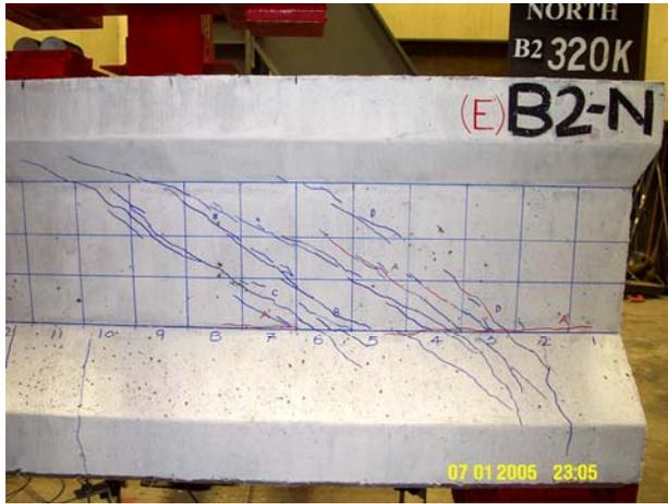
(a) Cracking of Beam B2-North End
