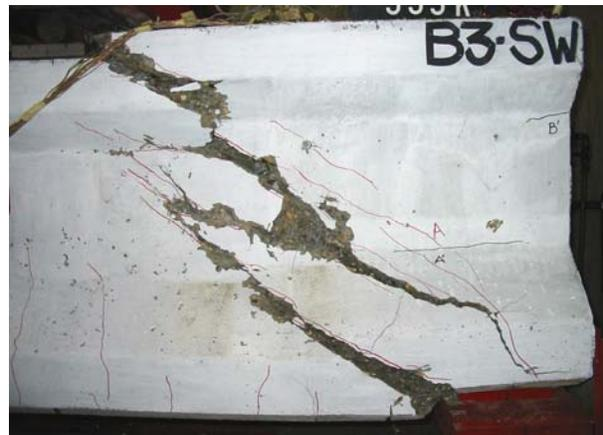
(b) Shear Failure of Beam B3-South End
