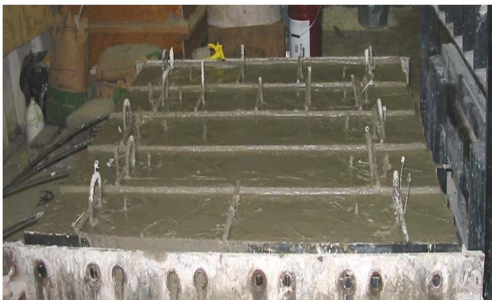
Fig. 3.3.4 Specimens after Casting Concrete
