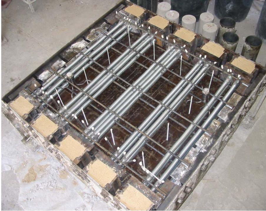
(c) Formwork of Panel TE-7
