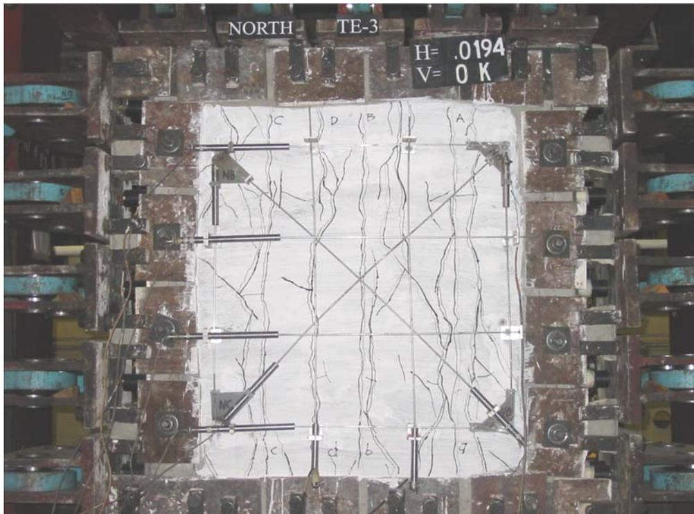
Fig. 4.8.4 Crack Pattern of Panel TE-3
