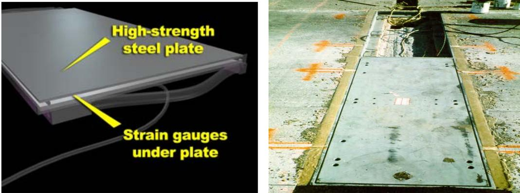
Figure 2-5: Bending Plate.
