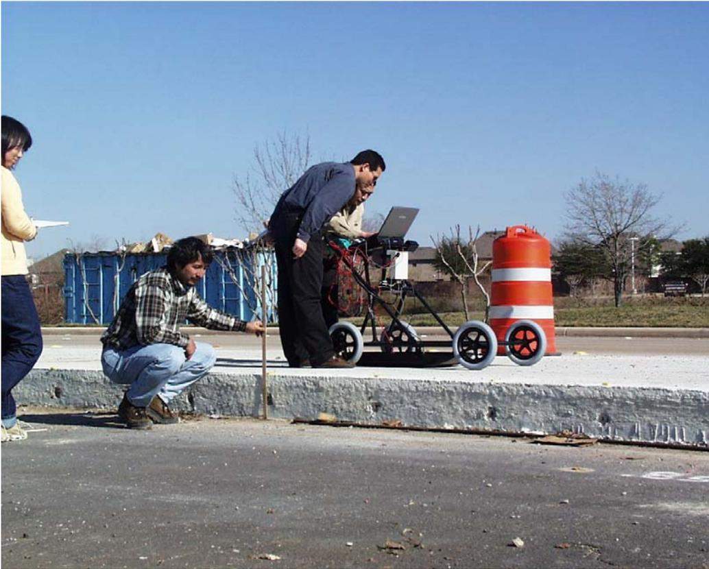
[Figure 5.1](#). Field test of the developed thickness radar over new pavement with steel rebar (Picture taken by Ed Oshinsky).
