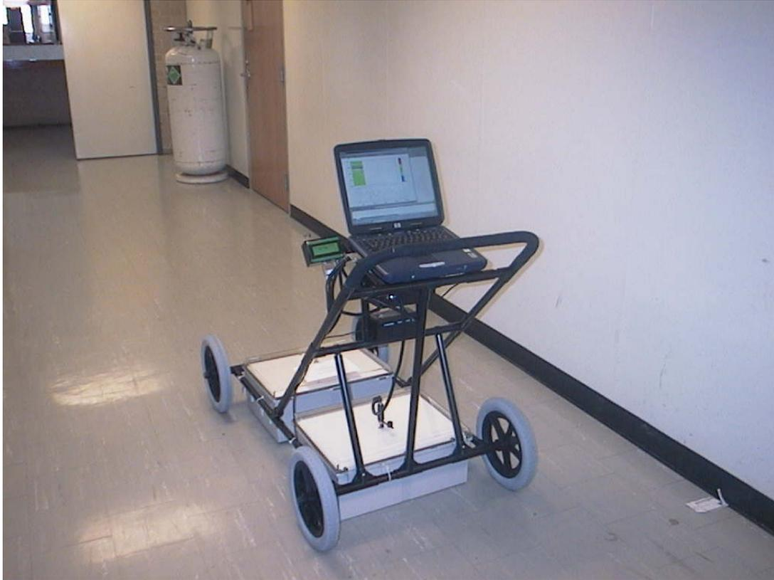
Figure 2.7. The Finalized GPR thickness measurement system
