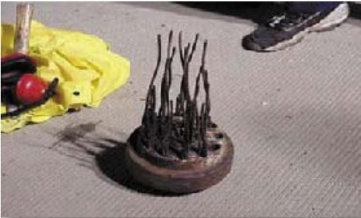
*Tendon Corrosion at Anchorage.*
