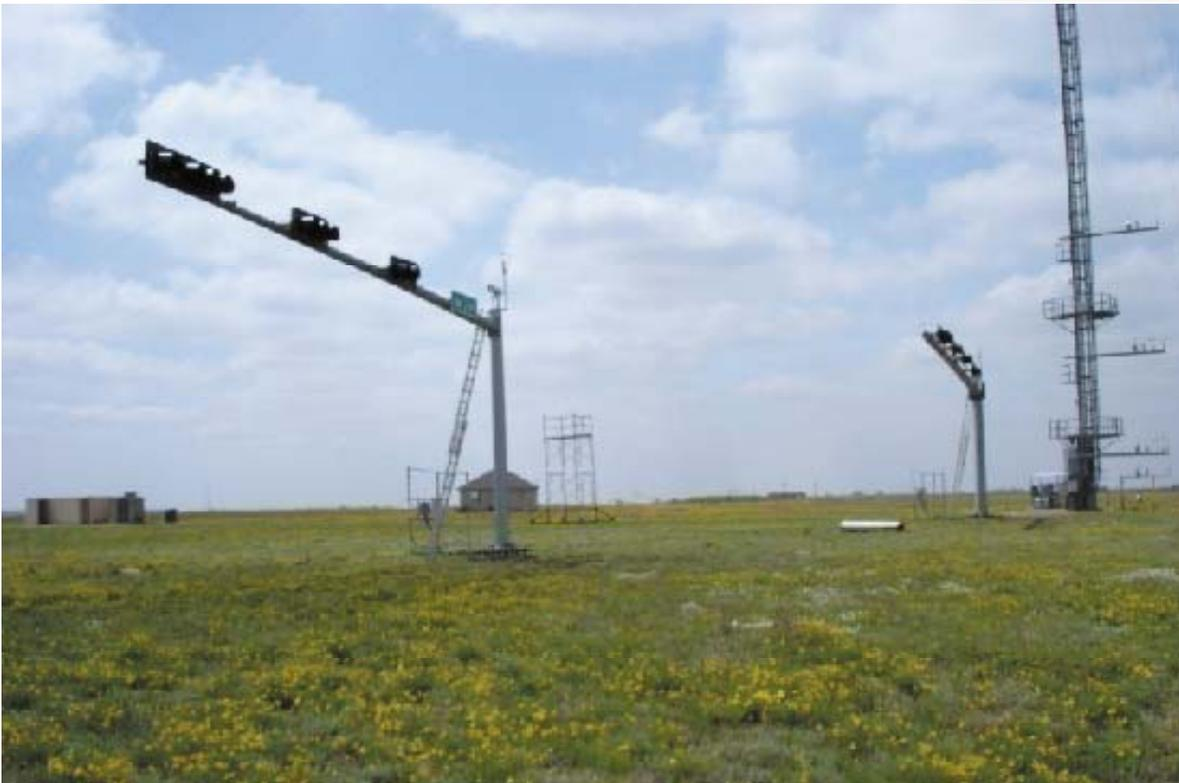
*Two Cantilever Traffic Signal Structures Tested at Reese Technology Center.*
