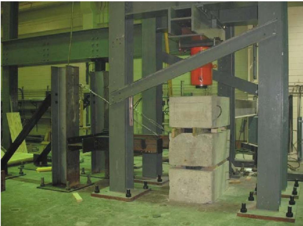
*Elevation View of Testing Frame: The test frame was composed of three separate smaller frames, allowing for the bearing to be loaded in three directions simultaneously.*
