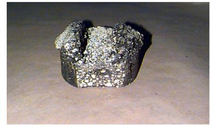
Figure 4. Specimen after HWTD Test (intermediate degradation)
