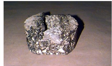
Figure 5. Specimen after HWTD Test (rough surface-low degradation)
