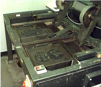
Figure 1. Hamburg Wheel Tracking Device
