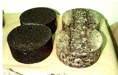
Figure 2. Specimens before and after HWTD Test
