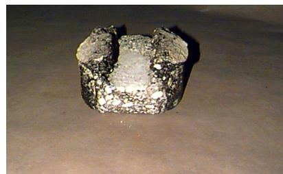
Figure 3. Specimen after HWTD Test (smooth surface-high degradation)
