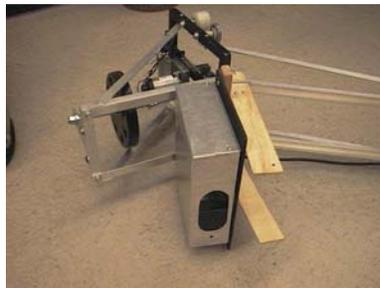
Figure 1. Laser texture sensor with mounting hardware
