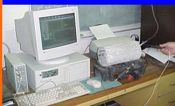
Portable Seismic Pavement Analyzer for Field Testing
